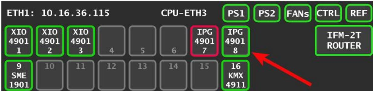
To access the menu for this IPG-4901, touch the virtual button corresponding to the card (identified by card type and slot number) in the home screen.
