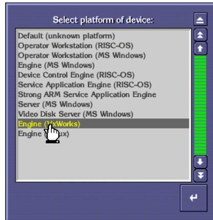
In the case of a system controller, choose **Engine (VxWorks)**.
