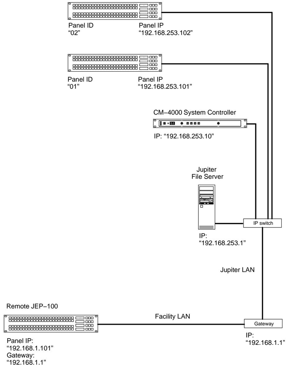
Configuration is similar to that just described, except that the address of the gateway must be entered on the web page for the remote JEP-100.
