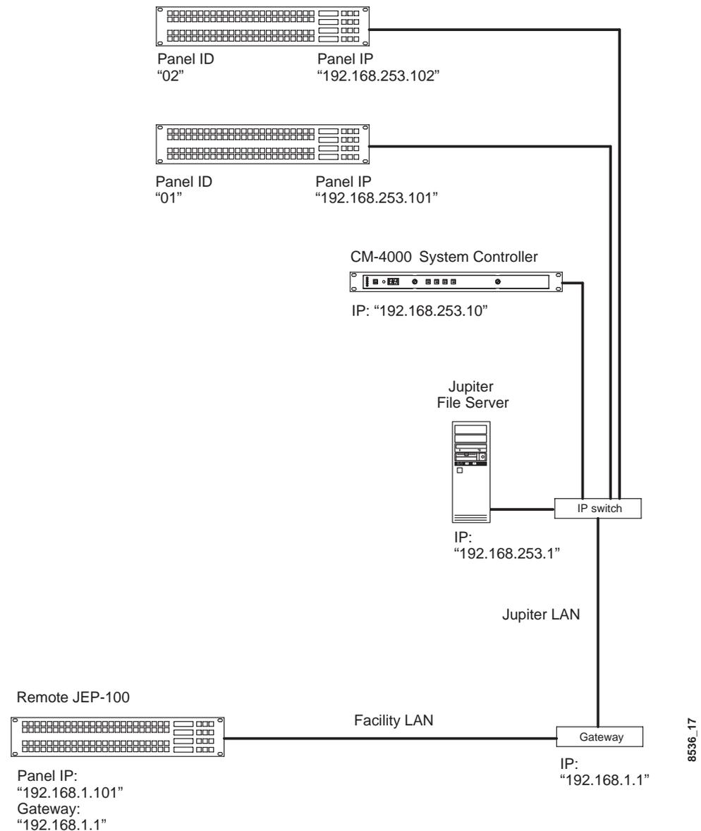
Configuration is similar to that just described, except that the address of the gateway must be entered on the web page for the remote JEP-100.
