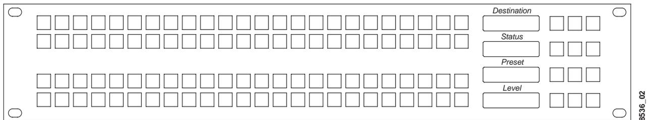
The JEP-100 Jupiter/Encore Control Panel is a locally-programmable, eight-character mnemonic, full-matrix control, multiple level break away panel designed especially for use in television production vans.
