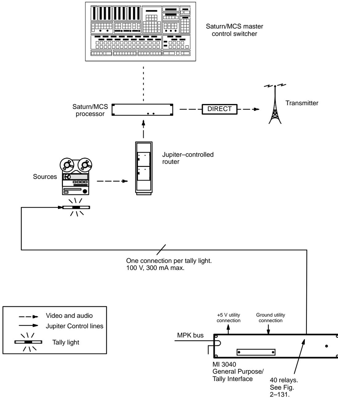
Figure 2-124. Tally system with Jupiter-controlled router, Saturn/MCS master control, and direct feed to transmitter.
