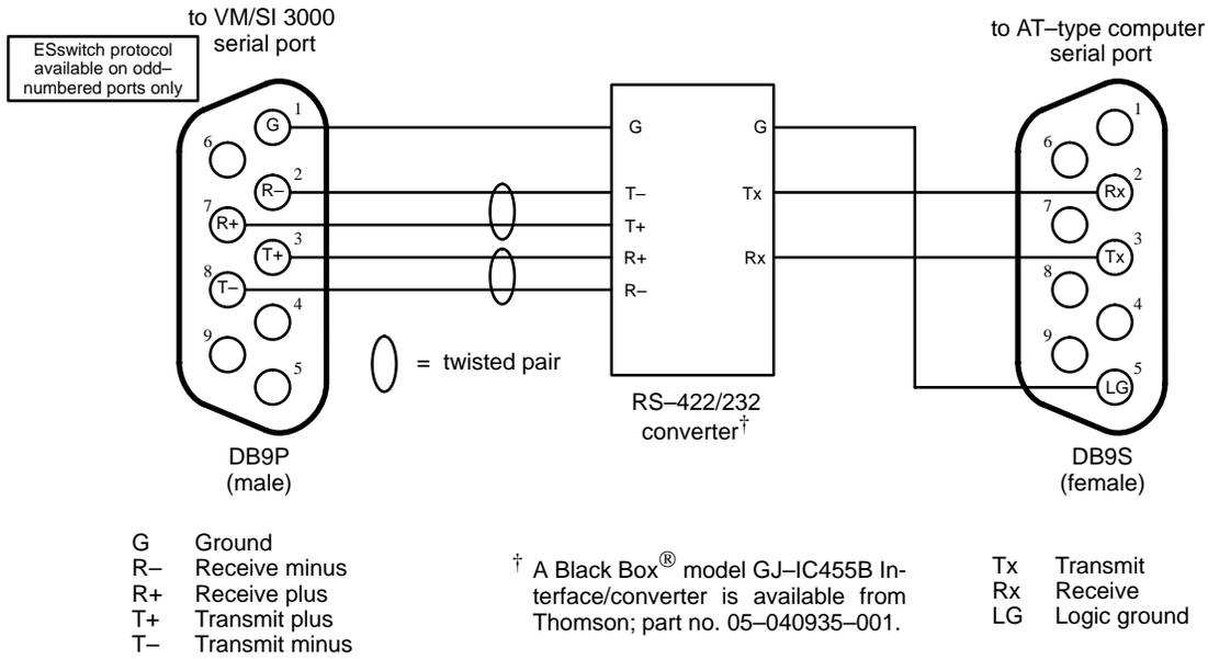
Figure 2-94. Cable for connecting VM/SI 3000 to AT-type computer.
