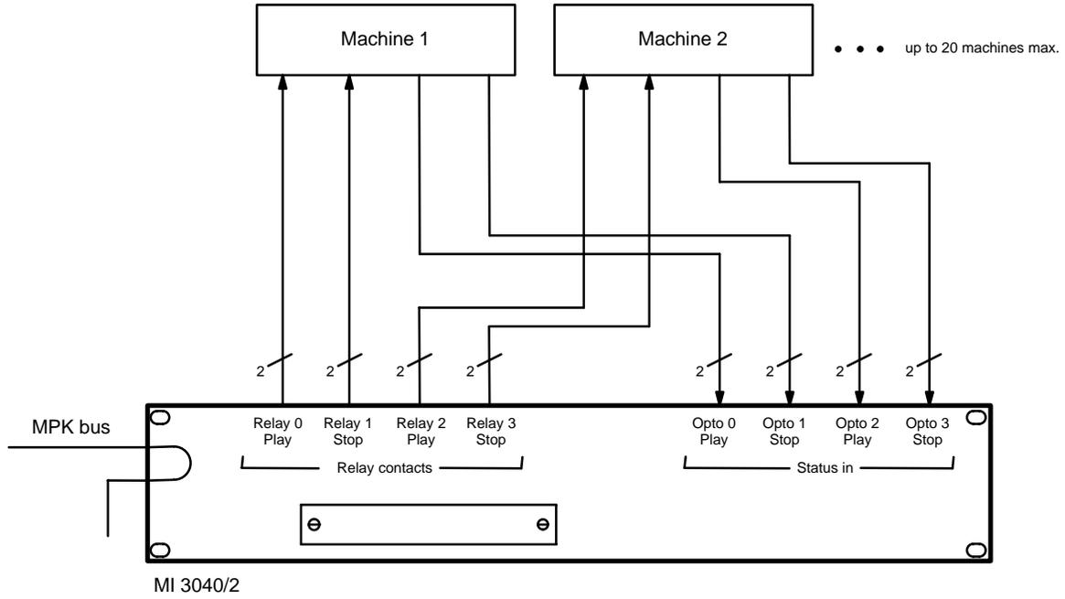
Figure 2-109. Example of MI 3040/2 connections.
