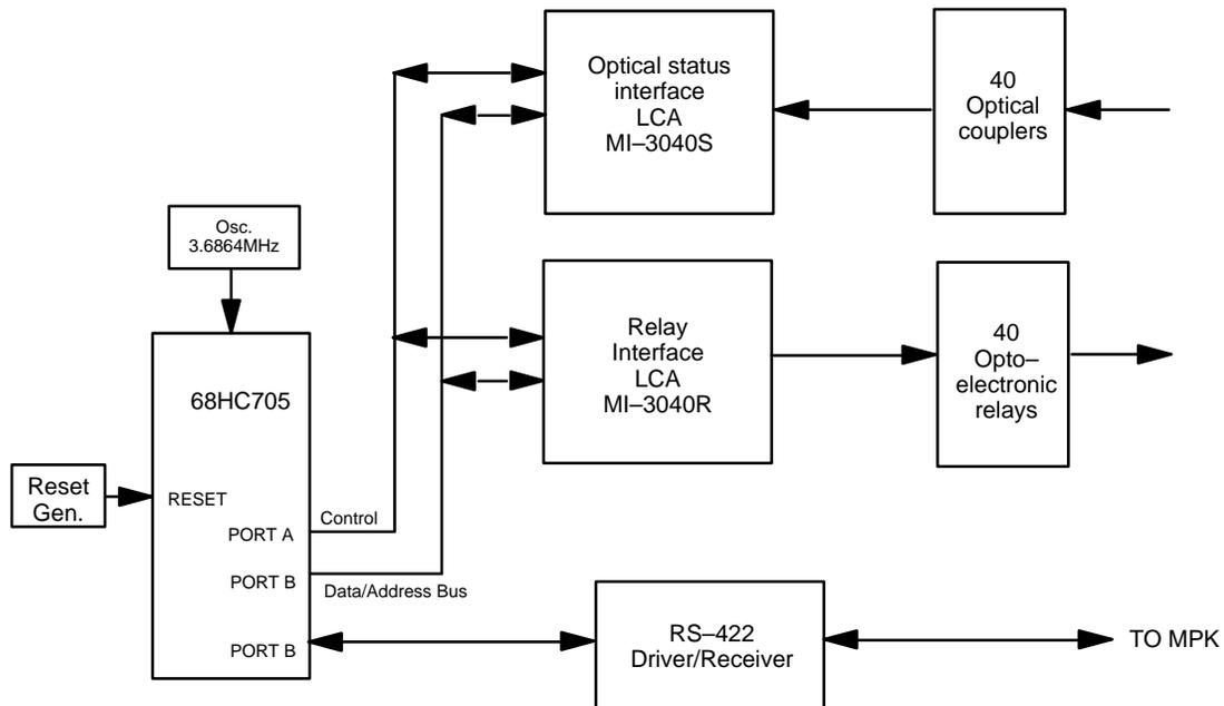
Figure 2-130. MI/MC 3040 interface block diagram.
