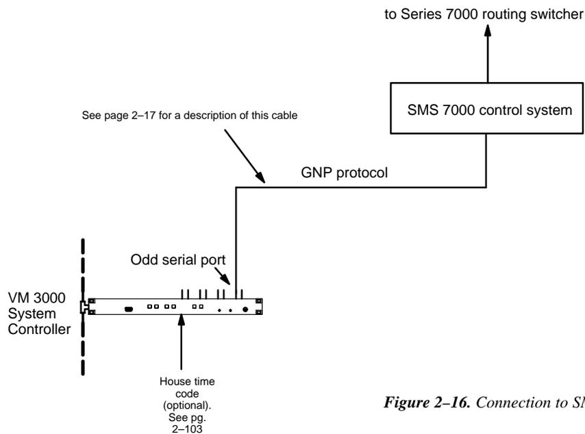
**Figure 2–16.** Connection to SMS 7000 Control System.
