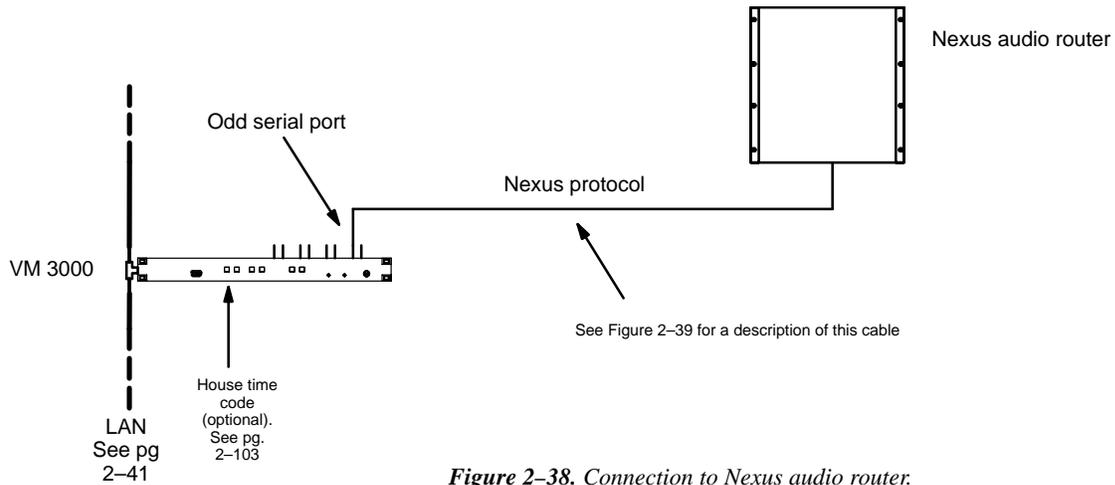
Figure 2-38. Connection to Nexus audio router.
