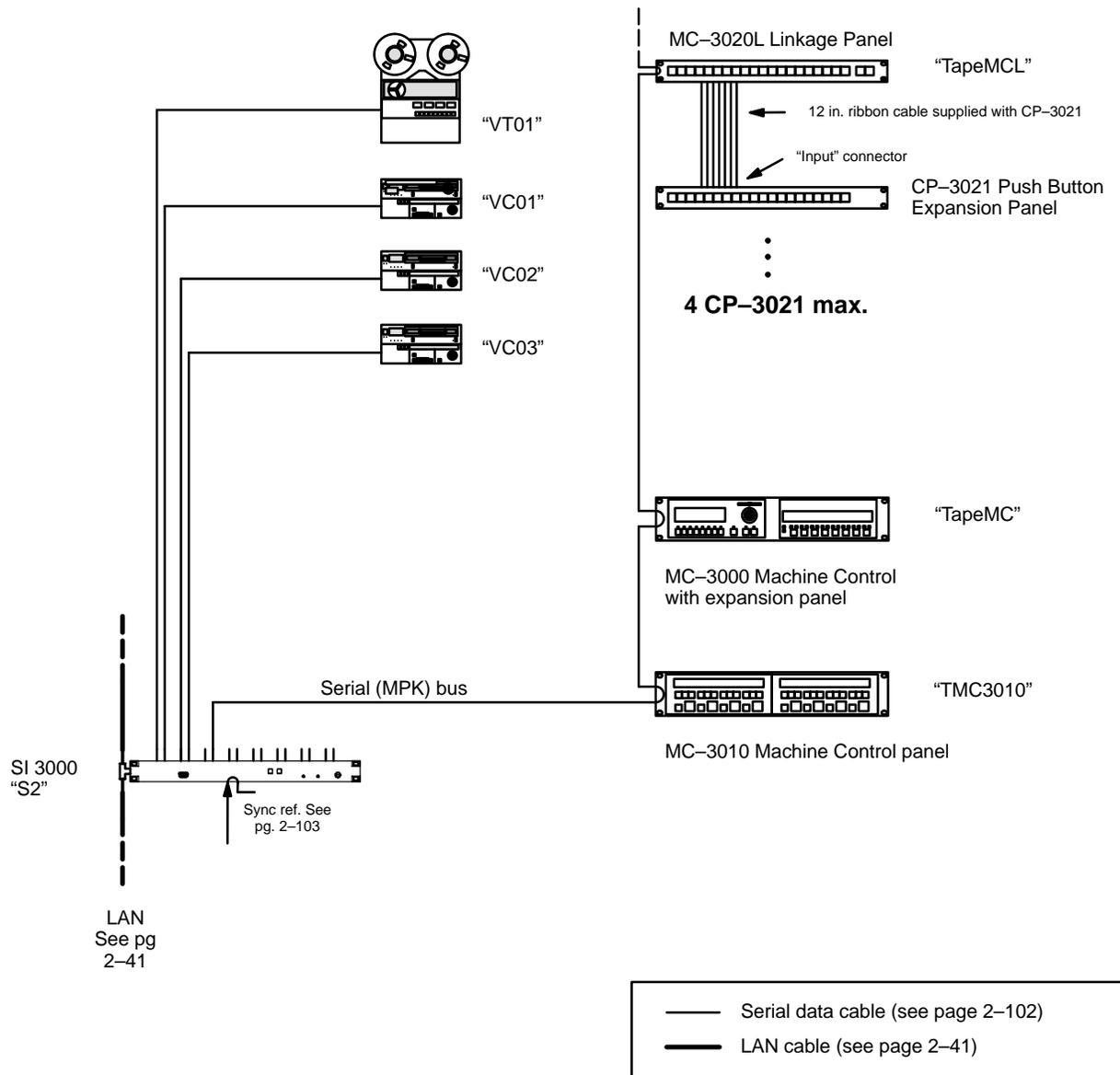
Figure 2-80. MC-3020L Linkage Panel installation..
