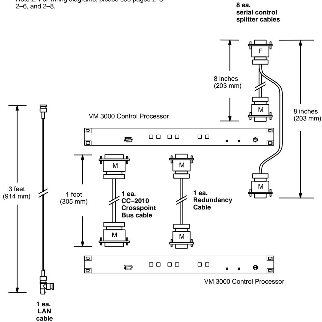
Figure 2-6. VM 3000 redundancy kit cables. Kit part no. 44-045838-001.
