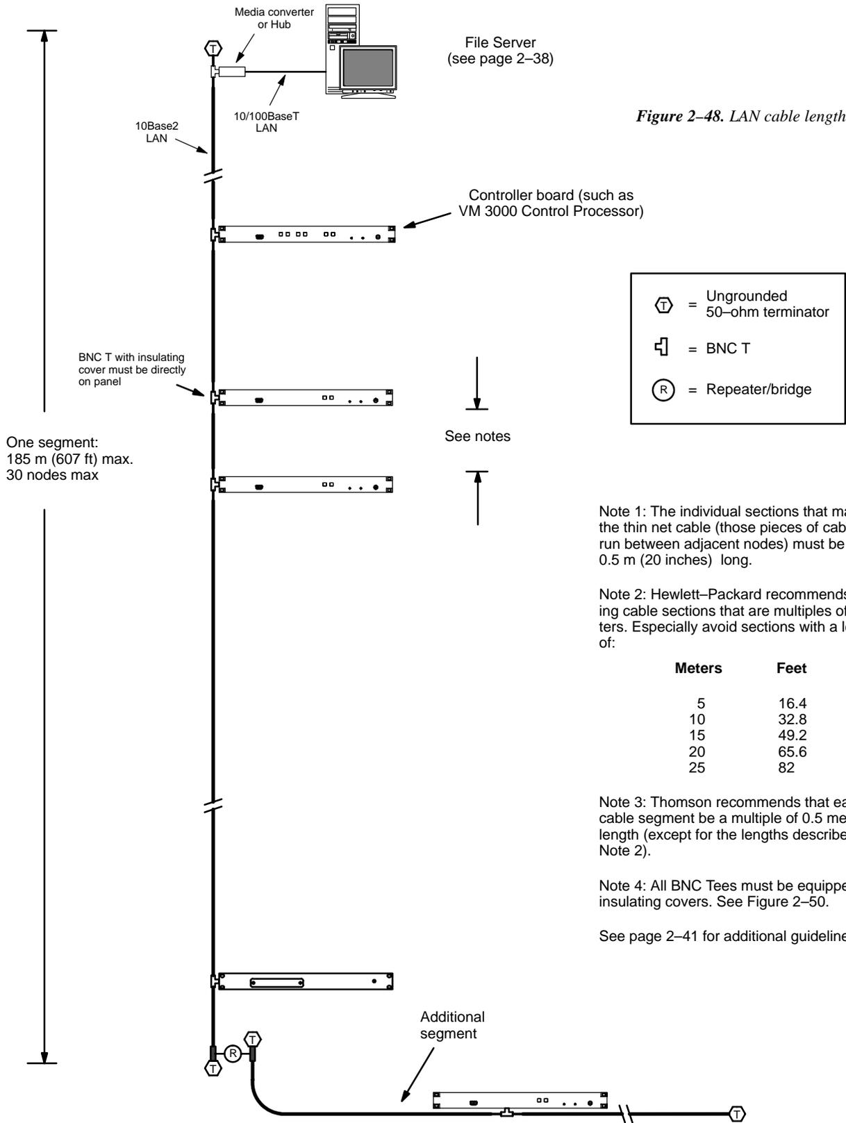
Figure 2-48. LAN cable lengths
