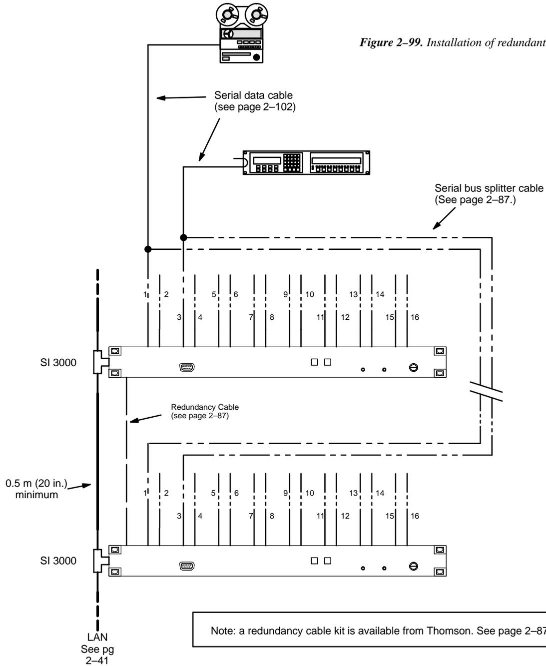
Figure 2-99. Installation of redundant SI 3000s.
