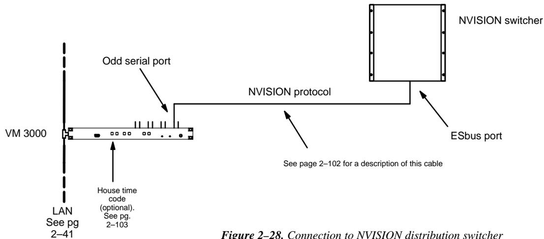
Figure 2-28. Connection to NVISION distribution switcher
