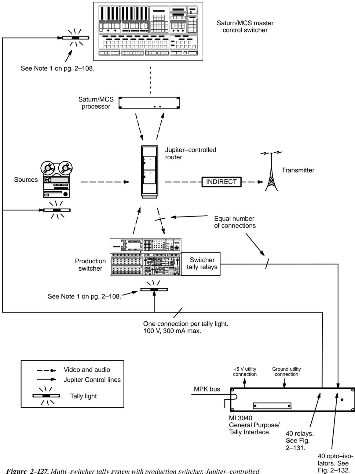
**Figure 2-127.** Multi-switcher tally system with production switcher, Jupiter-controlled router, Saturn/MCS master control, and indirect feed to transmitter.
