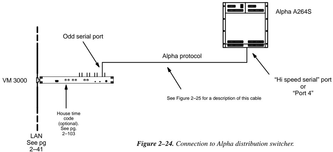
Figure 2-24. Connection to Alpha distribution switcher.
