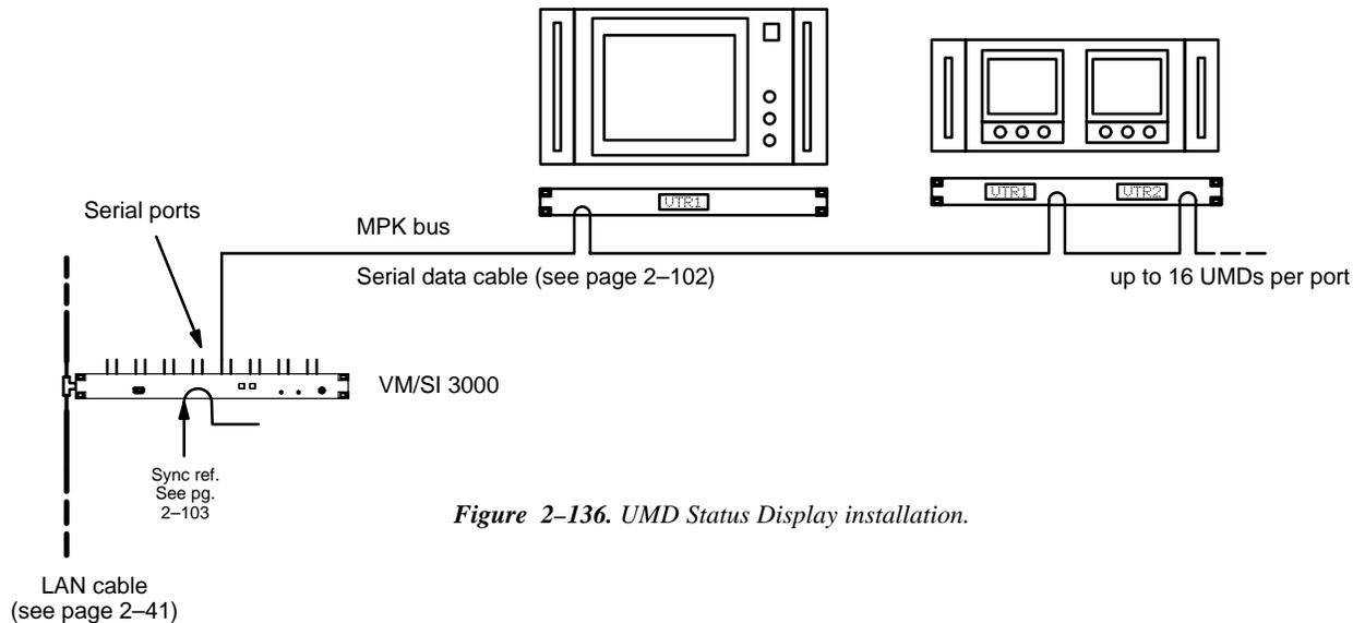
Figure 2-136. UMD Status Display installation.
