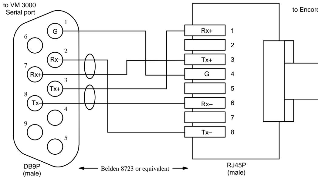
**Figure 2-20.** Cable for connecting VM 4000 to Encore.
