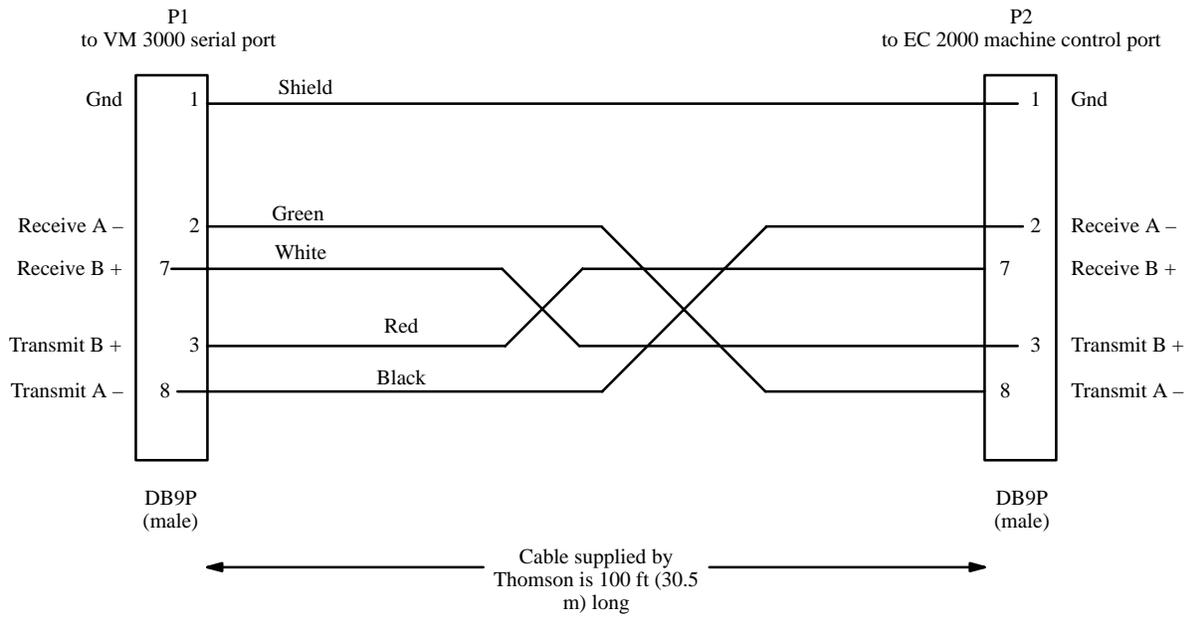
Figure 2-121. Assembly, MCS 2000 automation cable. Ref: Thomson drawing no. 01-036373-001.
