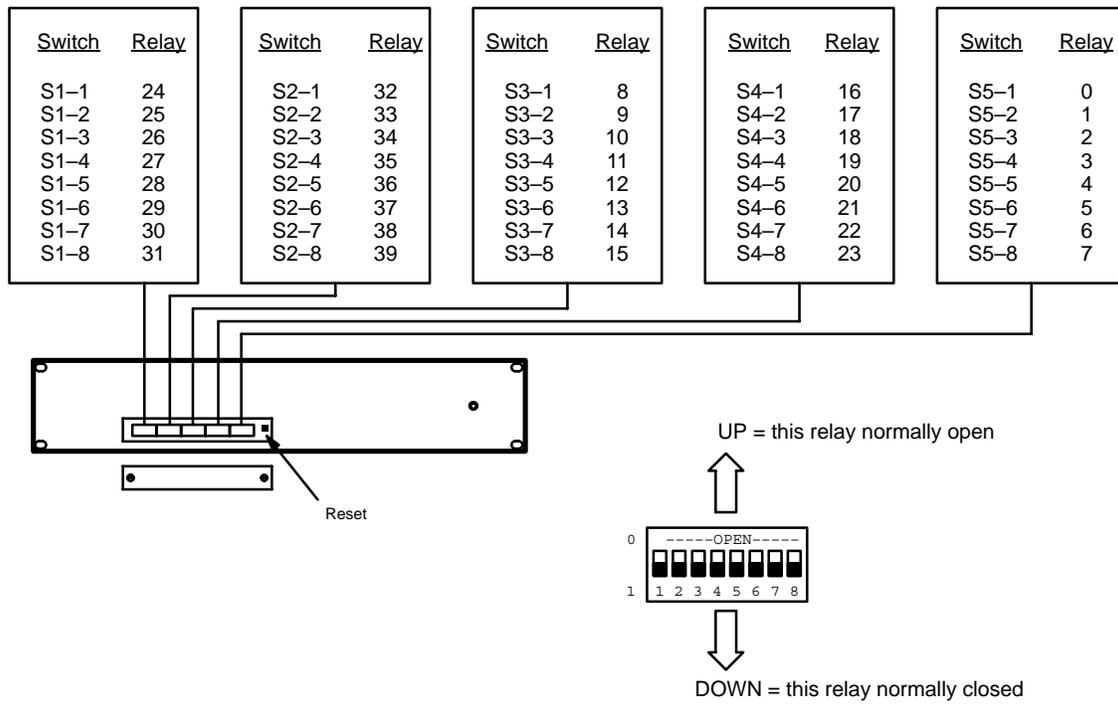
Figure 2-133. MI/MC 3040 normally open/closed relay DIP switches.
