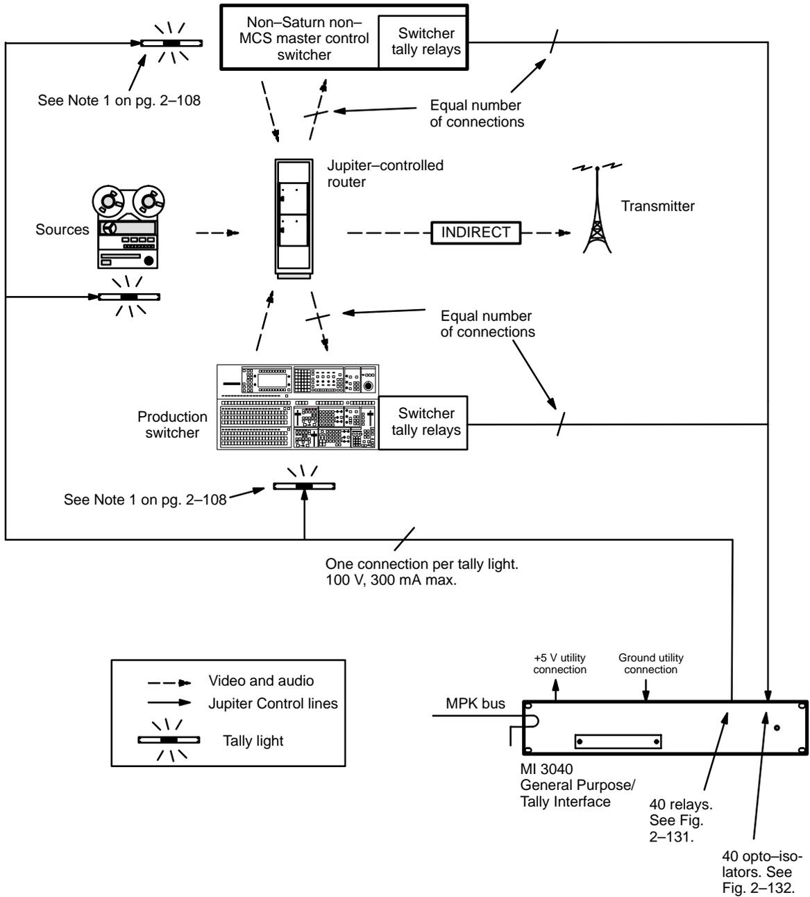
**Figure 2-129.** Multi-switcher tally system with production switcher, Jupiter-controlled router, non-Saturn non-MCS master control, and indirect feed to transmitter.
