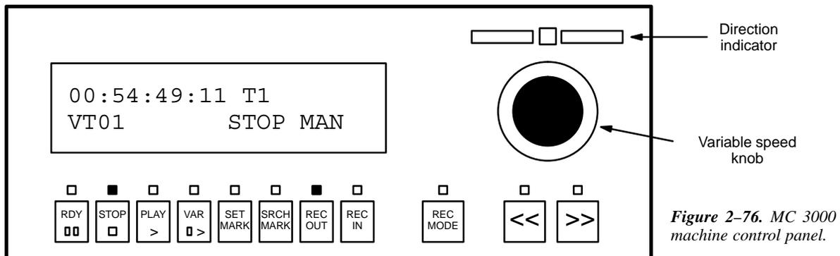
Figure 2-76. MC 3000 machine control panel.
