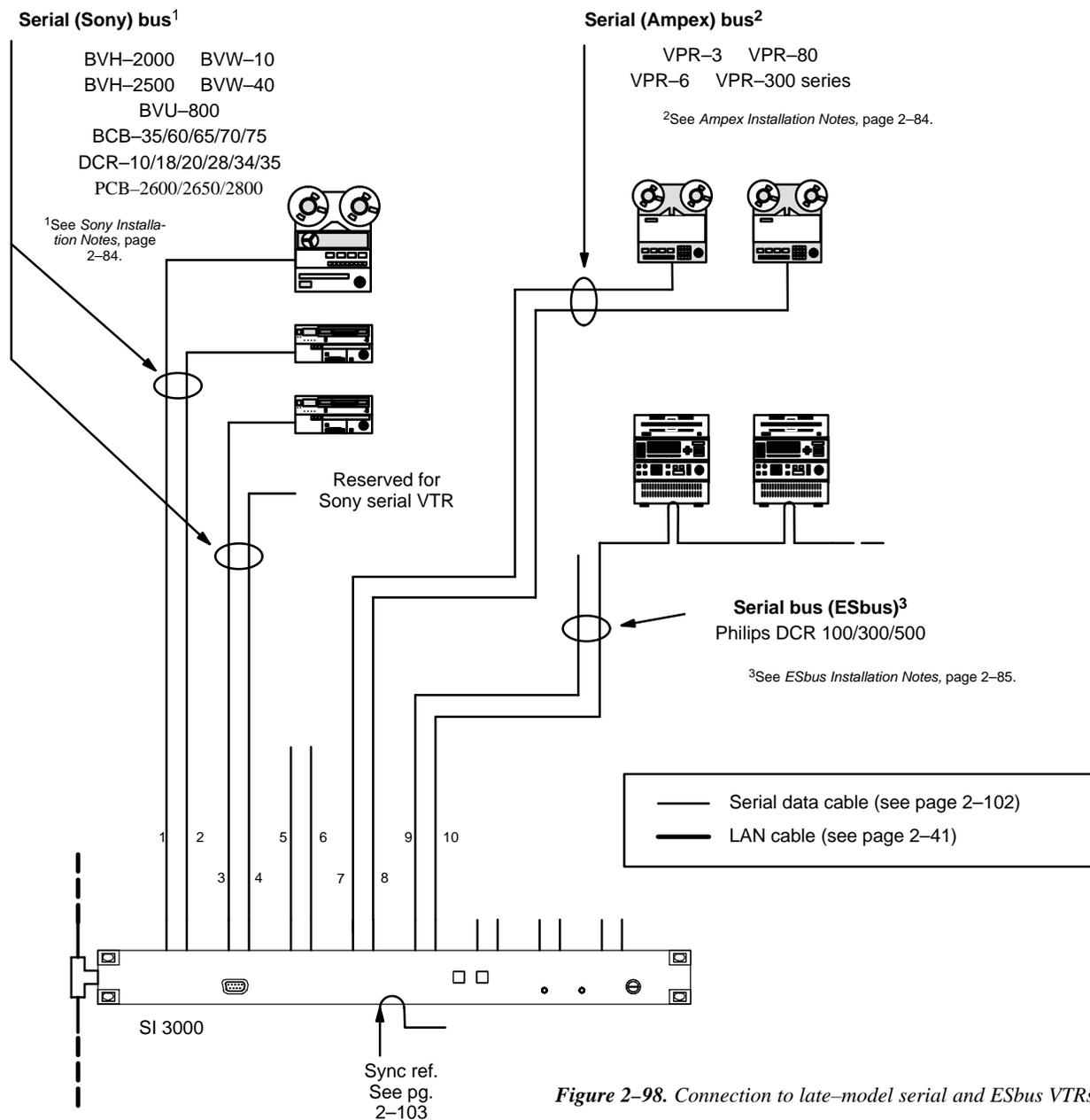
Figure 2-98. Connection to late-model serial and ESBUS VTRs.
