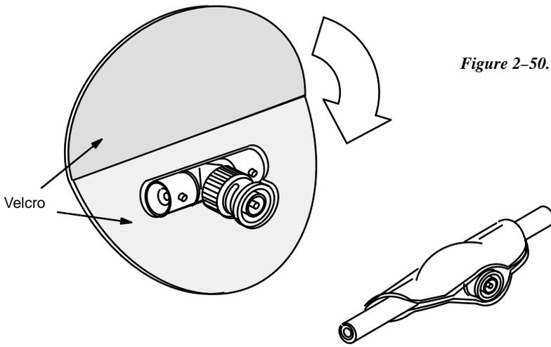
Figure 2-50. ThinLAN insulating cover for tee connector.
