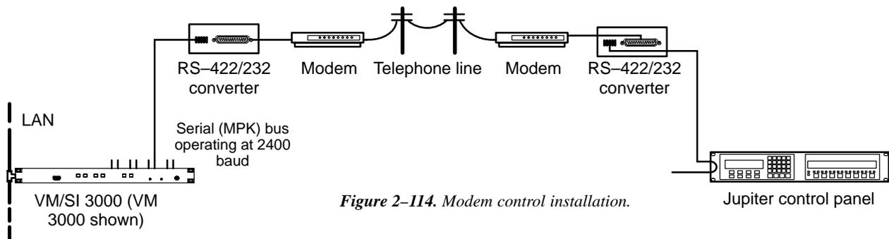
Figure 2-114. Modem control installation.
