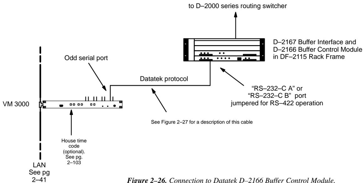
Figure 2-26. Connection to Datatek D-2166 Buffer Control Module.
