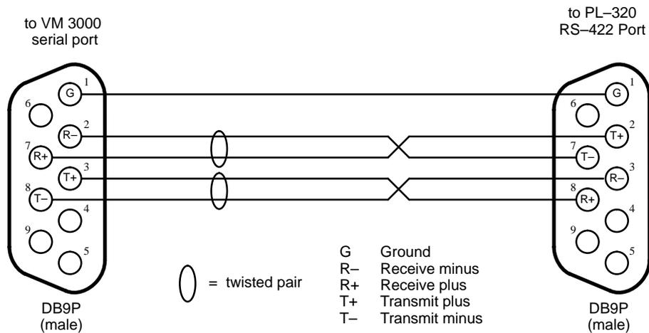
Figure 2-34. Cable for connecting VM 3000 to PL-320.
