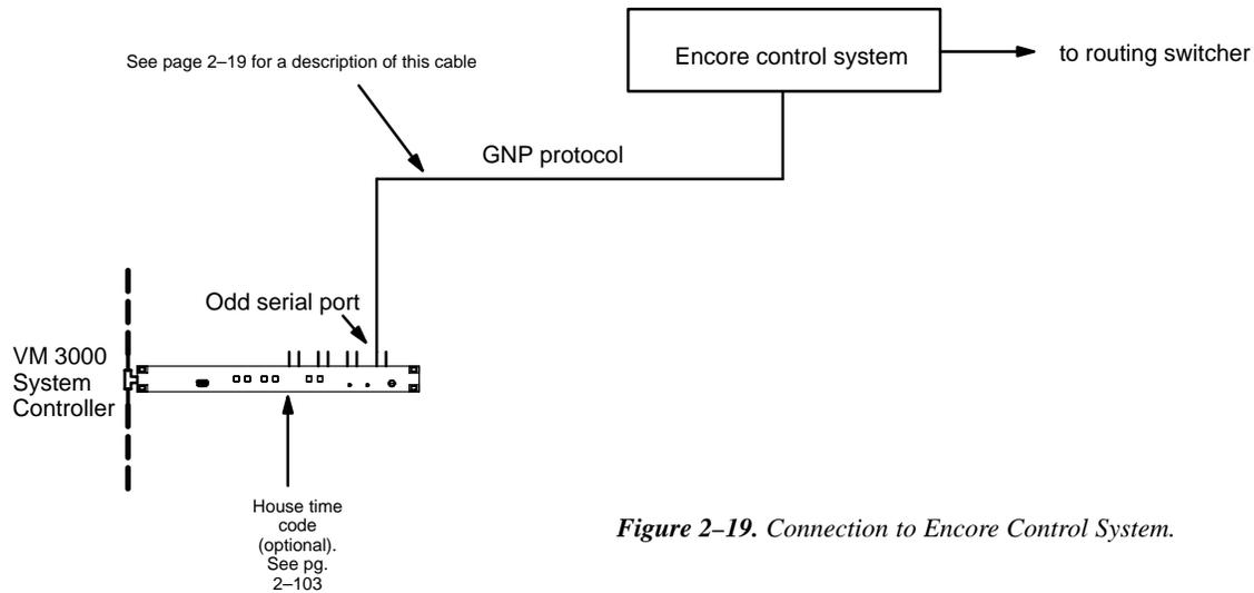
**Figure 2–19.** Connection to Encore Control System.
