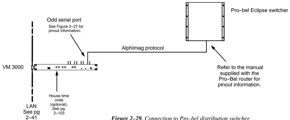
Figure 2-29. Connection to Pro-bel distribution switcher.
