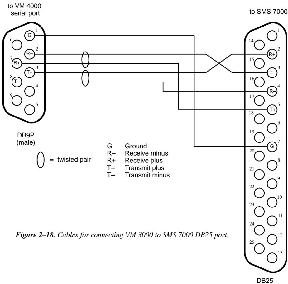
Figure 2-18. Cables for connecting VM 3000 to SMS 7000 DB25 port.
