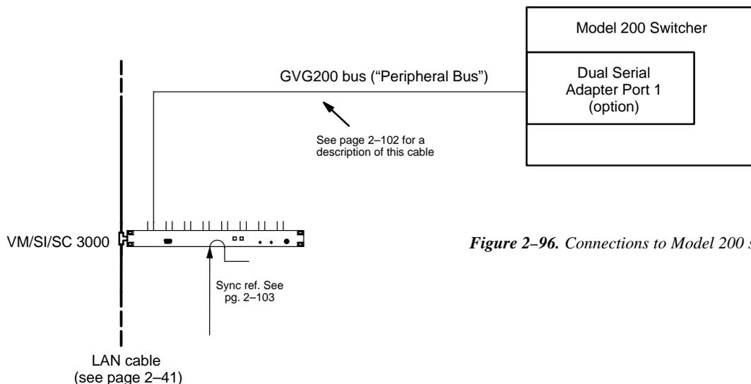
Figure 2-96. Connections to Model 200 switcher.
