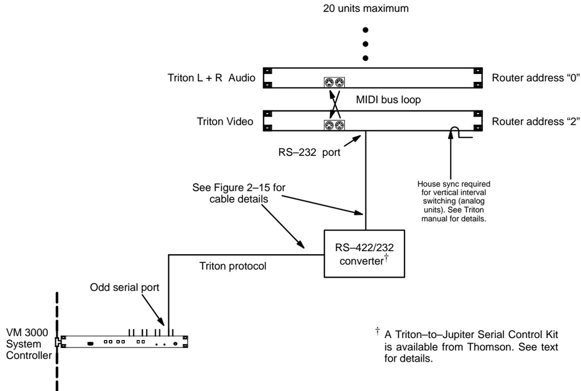
Figure 2-14. Example of connection to Triton distribution switchers.
