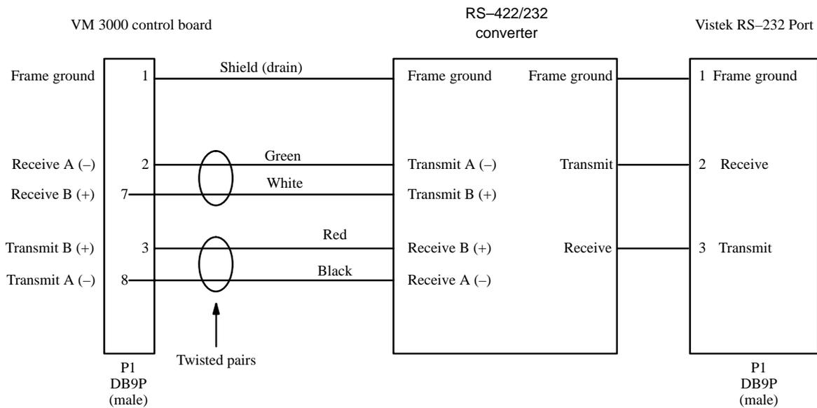
Figure 2-37. Cables for connecting VM 3000 to Vistek RS-232 port.
