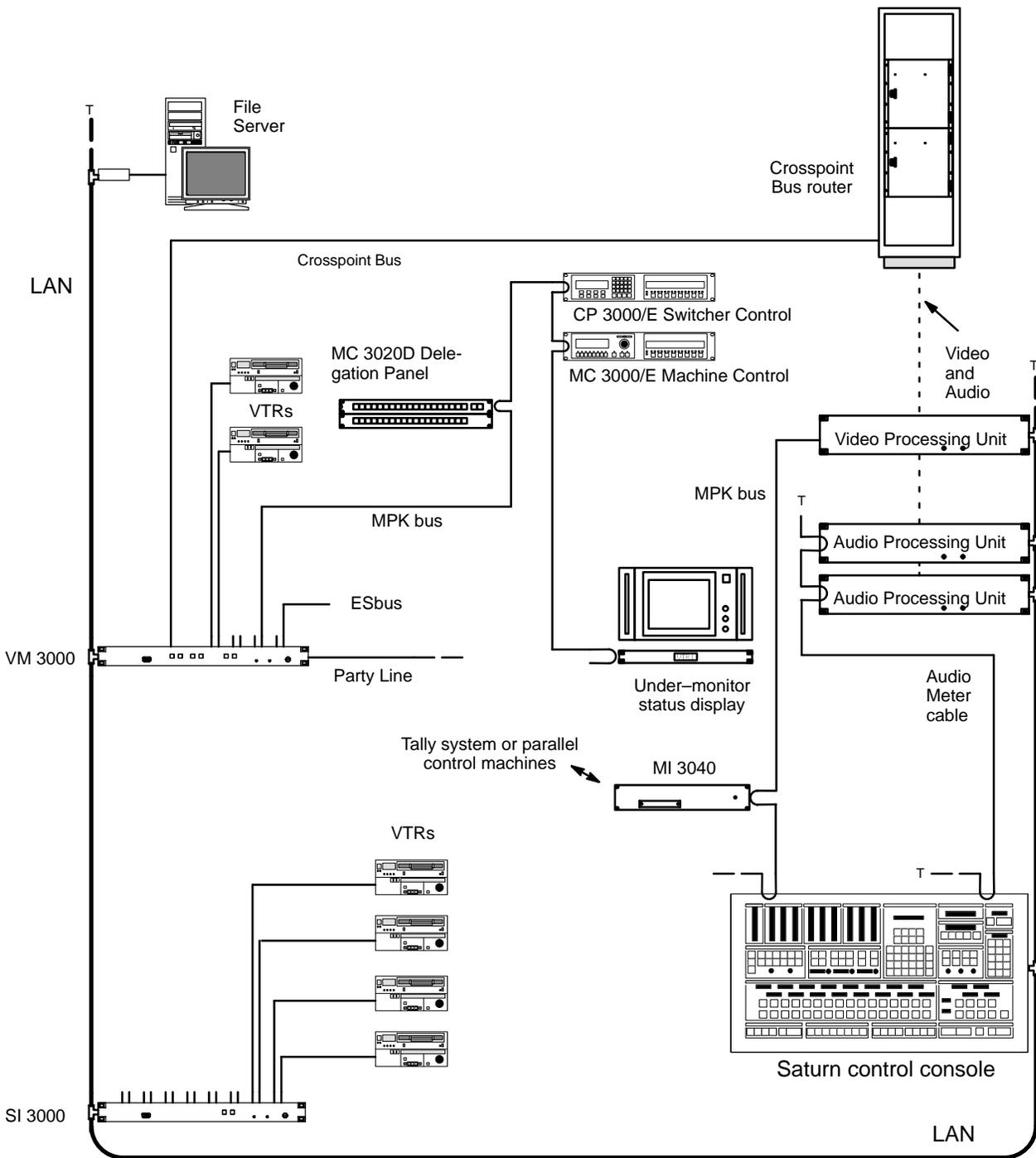
**Figure 2-119.** Example of Saturn MCS with Crosspoint Bus router and Jupiter control system. For Saturn instructions, see Saturn Master Control Switcher Installation and Operating Manual.
