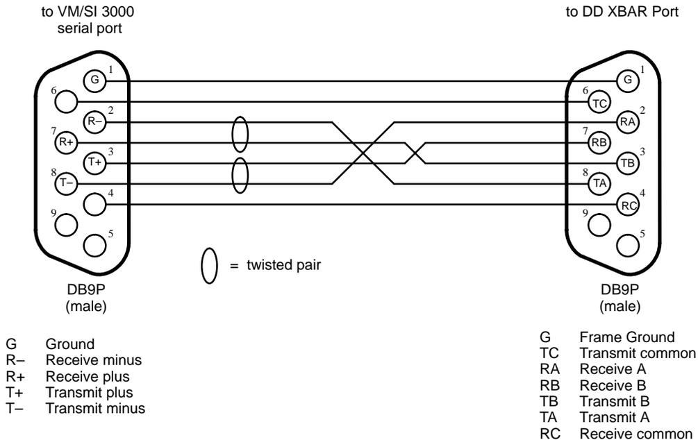
Figure 2-89. Cable for connecting VM/SI 3000 to Thomson DD XBAR Port.
