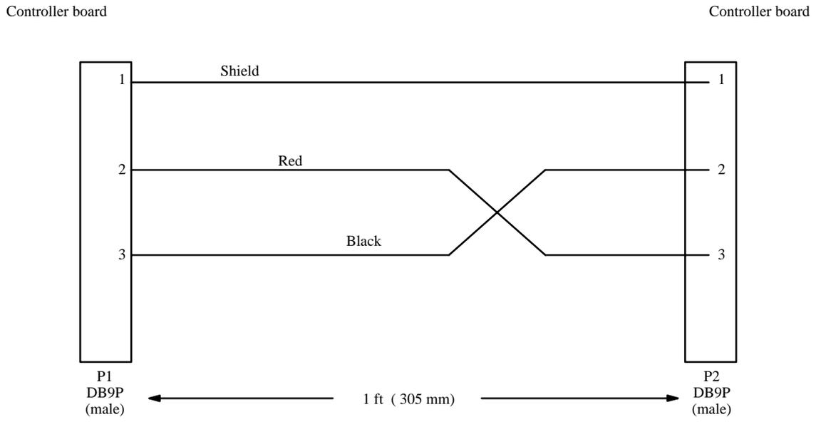
**Figure 2-7.** Assembly, BCS-3000 Redundancy Cable. Ref: Thomson drawing no. 01-041340-001.
