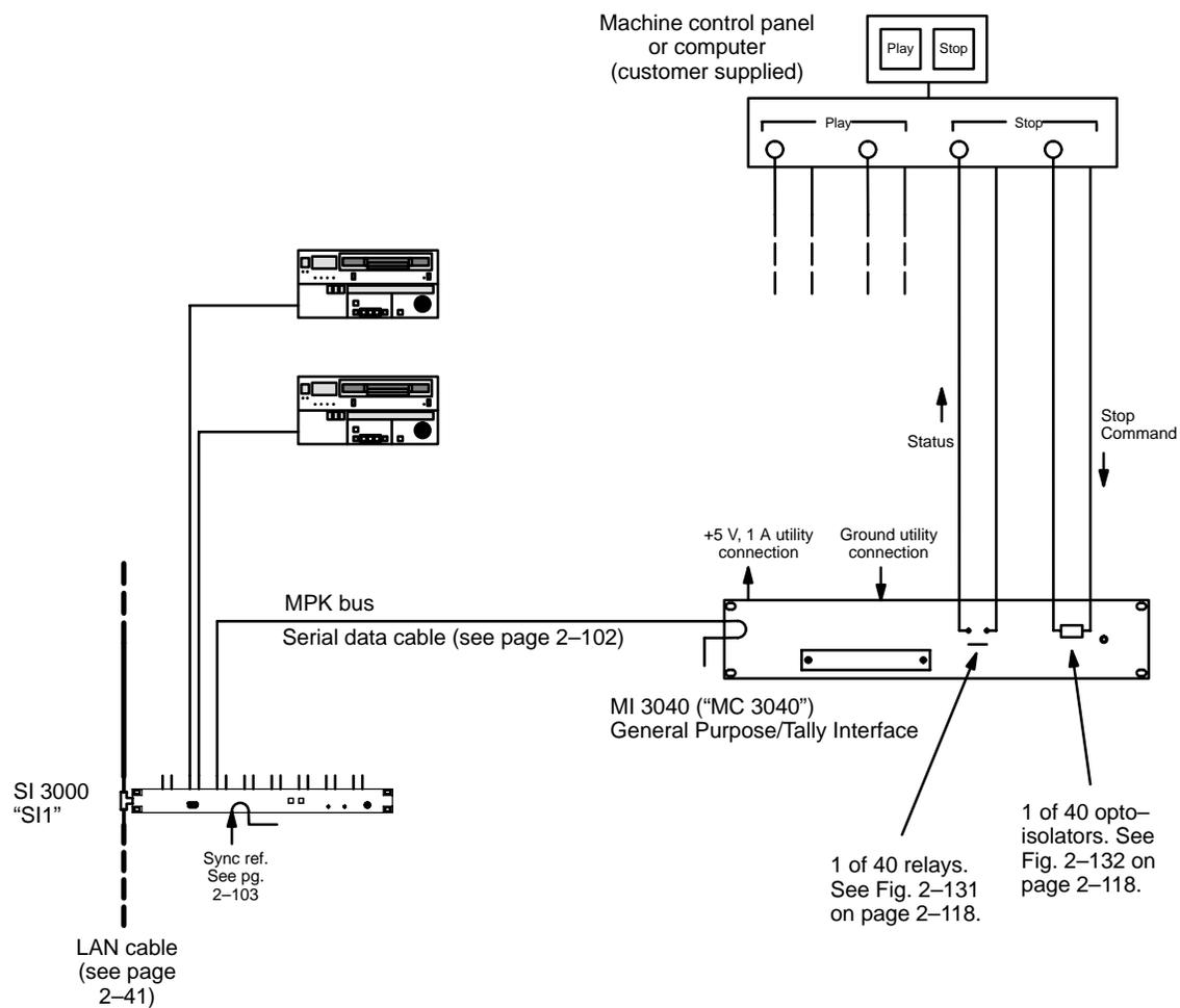
Figure 2-110. External machine control using MI 3040 (“MC 3040”).
