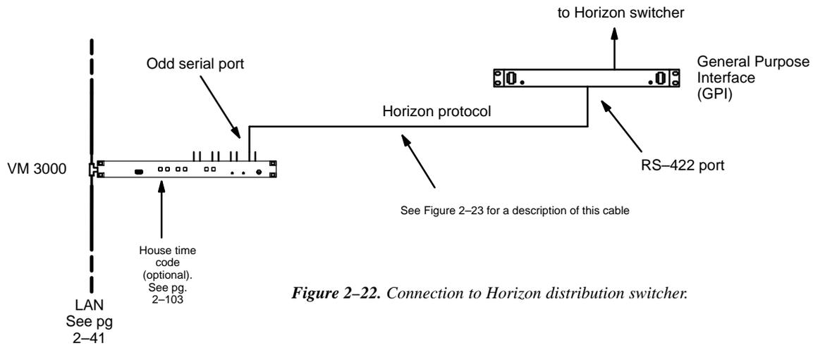
Figure 2-22. Connection to Horizon distribution switcher.
