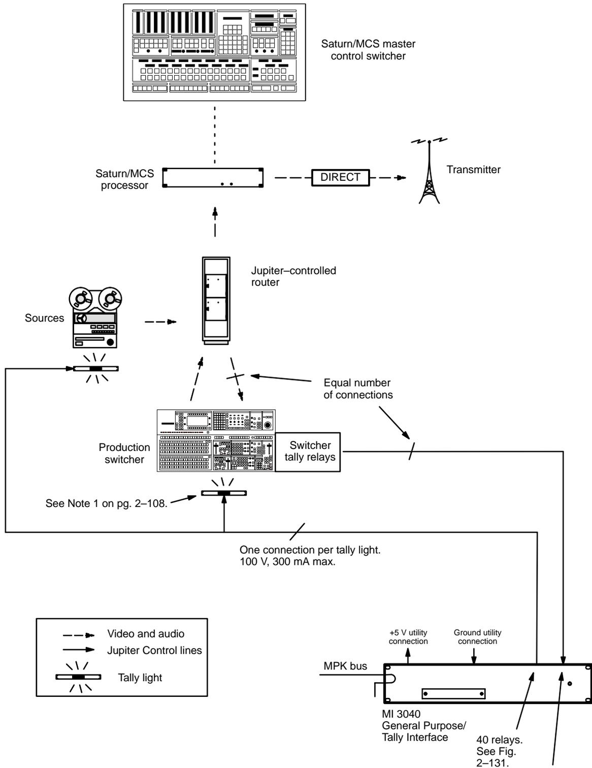
Figure 2-126. Multi-switcher tally system with production switcher, Jupiter-controlled router, Saturn/MCS master control, and direct feed to transmitter.
