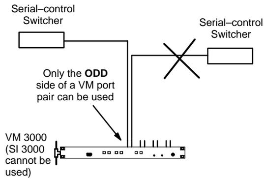
Figure 2-13. Serial-control switcher restrictions.
