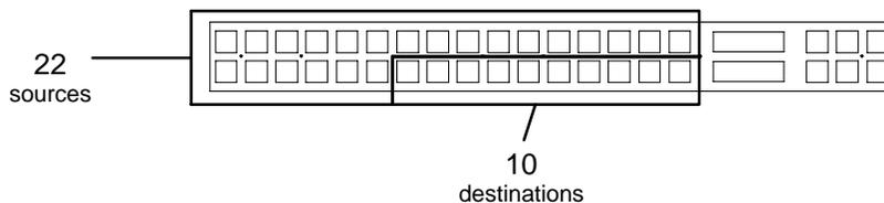
*Figure 2-69. Example of “unbalanced split” configuration (22 x 10).*
