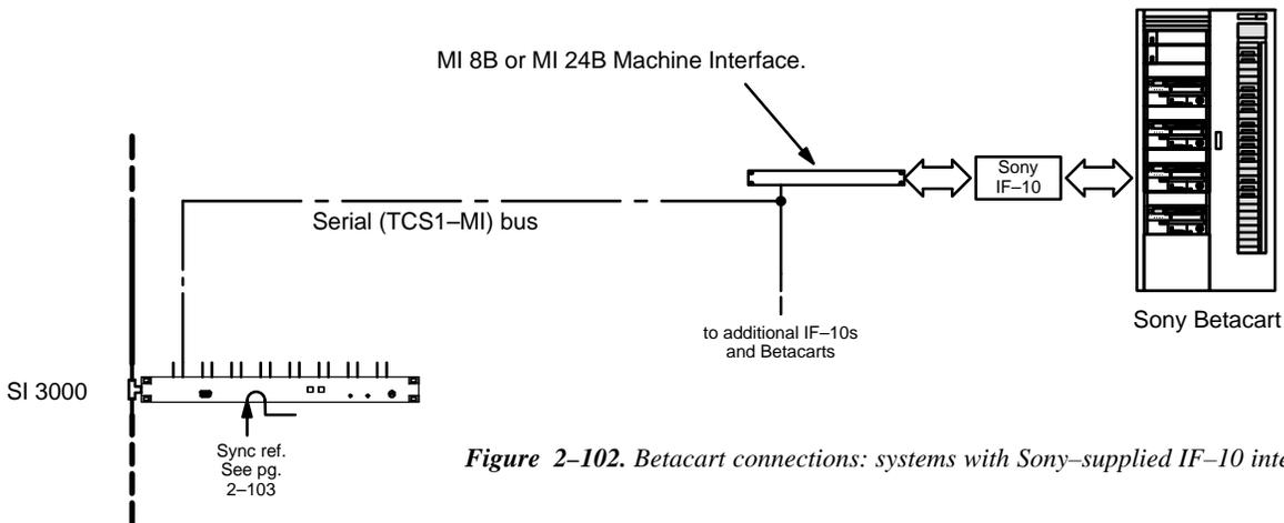
Figure 2-102. Betacart connections: systems with Sony-supplied IF-10 interface.
