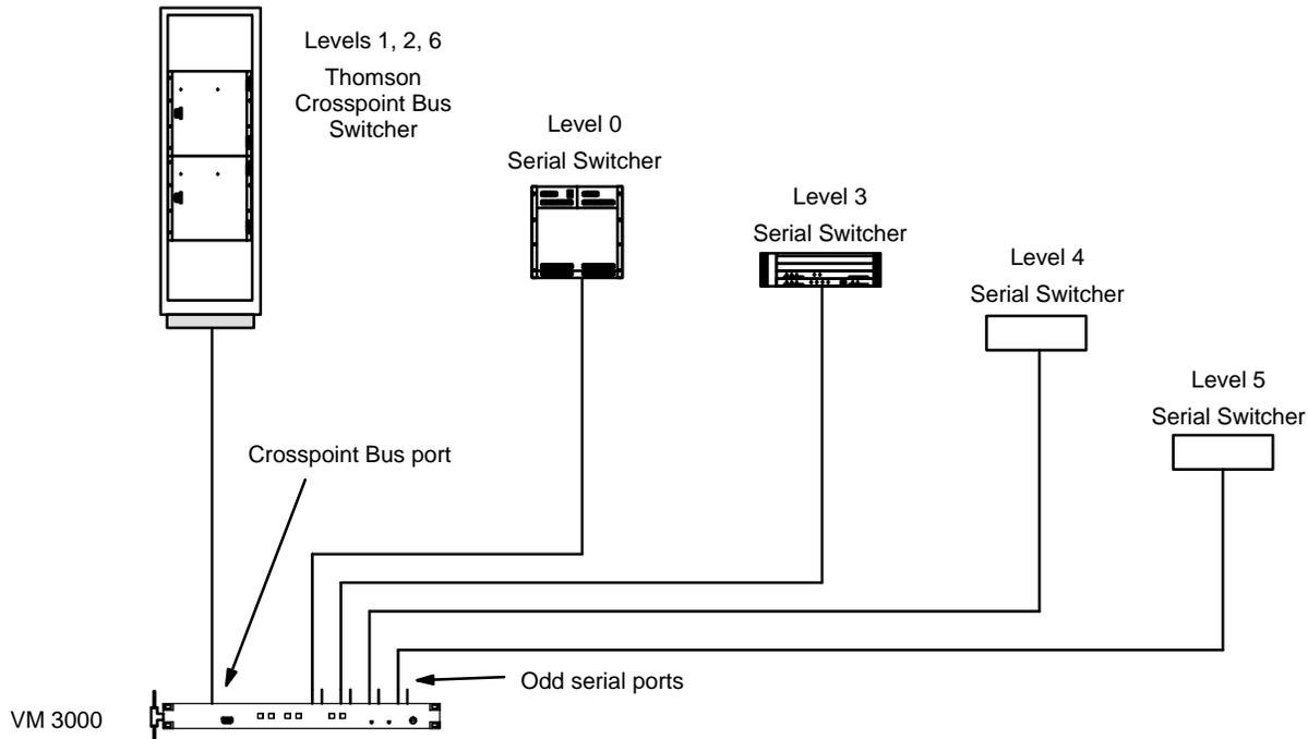
**Figure 2-12.** Connection to serial control routers (example).
