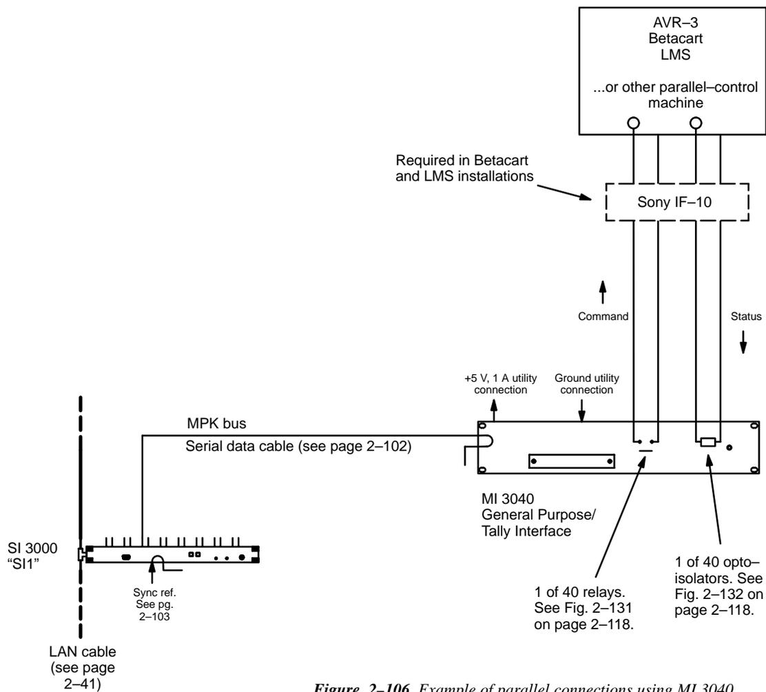
Figure 2-106. Example of parallel connections using MI 3040.
