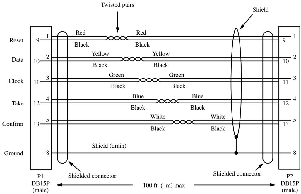
Figure 2-9. CC 2010 wiring. Reference: "Assembly, XPT Bus Cable Shield," Thomson drawing no. 01-048592-TAB.
