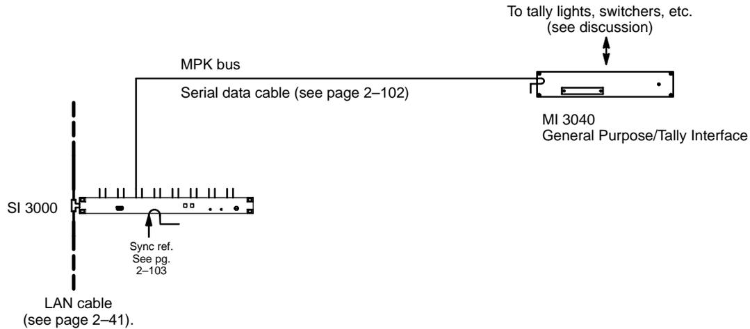
Figure 2-122. MPK connections to MI 3040.
