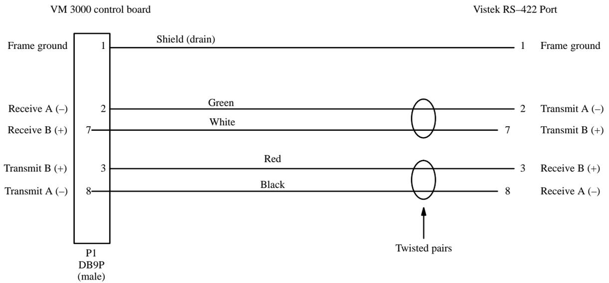
Figure 2-36. Cable for connecting VM 3000 to Vistek RS-422 port.
