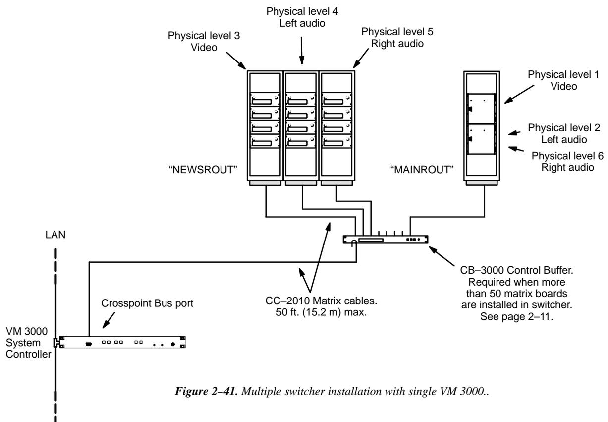
Figure 2-41. Multiple switcher installation with single VM 3000..
