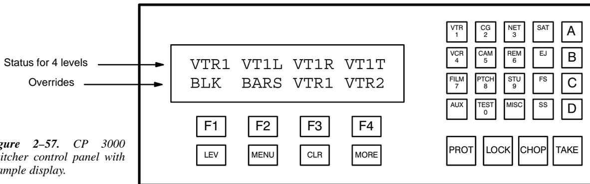
Figure 2-57. CP 3000 Switcher control panel with example display.
