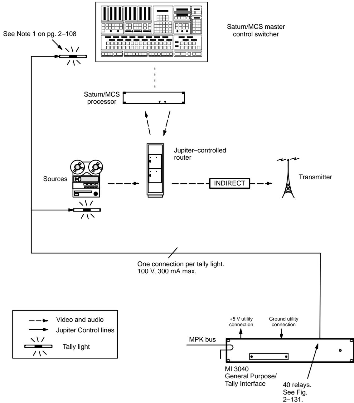
**Figure 2-125.** Tally system with Thomson/MCS master control, Jupiter-controlled router, and indirect feed to transmitter.
