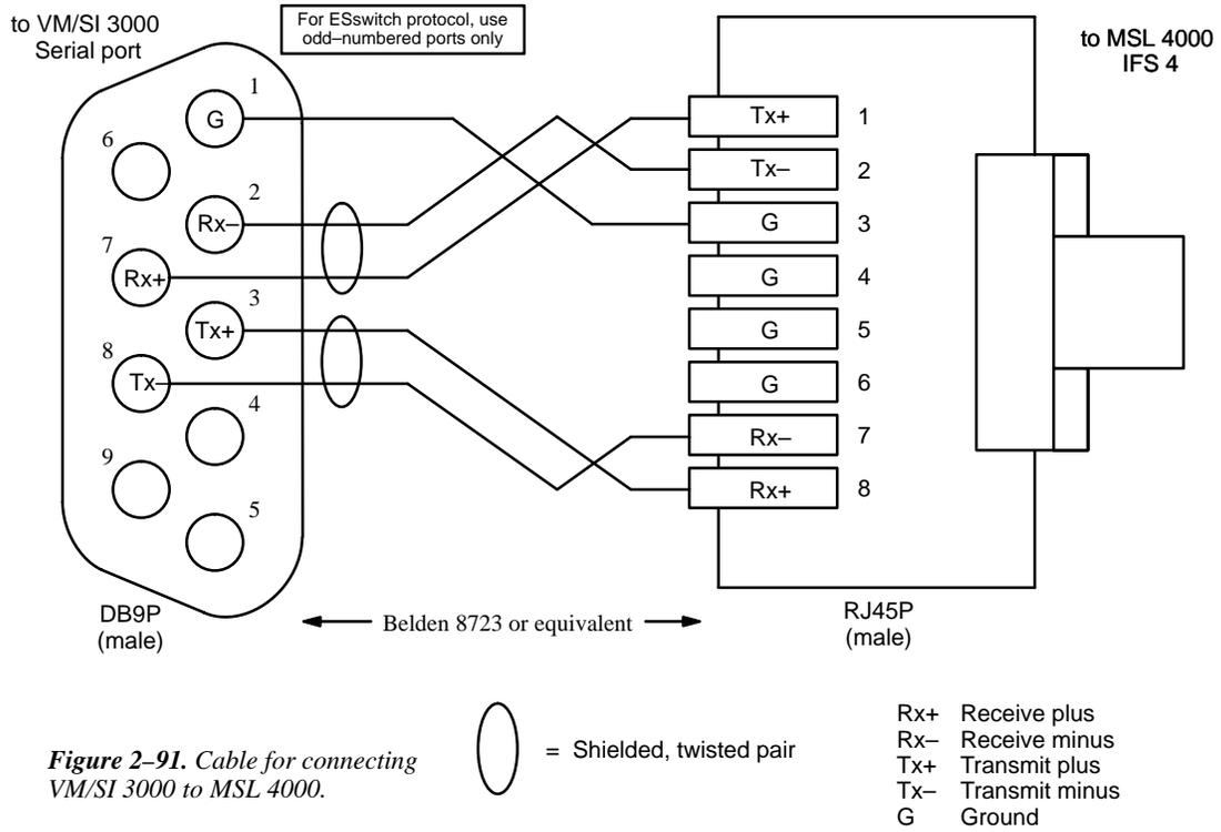
**Figure 2-91.** Cable for connecting VM/SI 3000 to MSL 4000.
