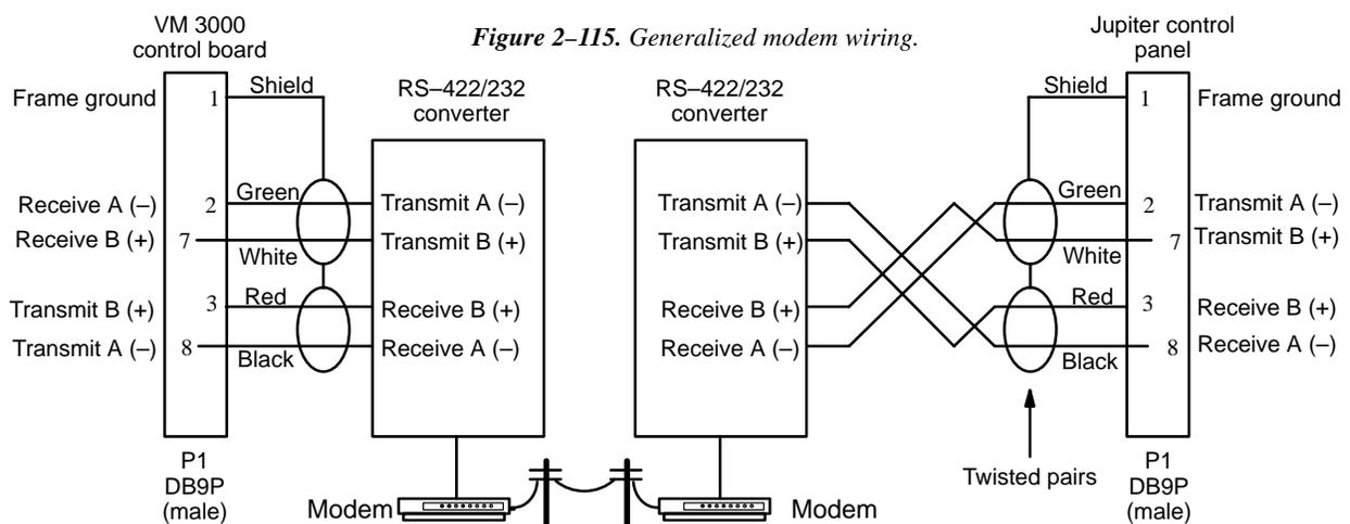
Figure 2-115. Generalized modem wiring.
