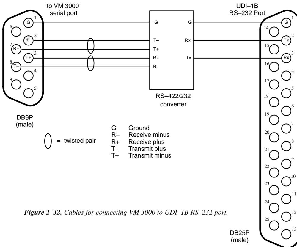
Figure 2-32. Cables for connecting VM 3000 to UDI-1B RS-232 port.
