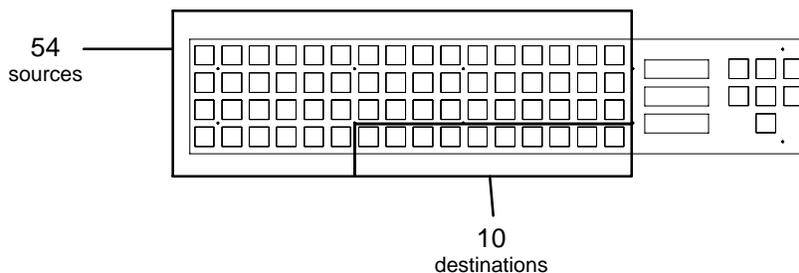
*Figure 2-73. Example of “unbalanced split” configuration (54 x 10).*
