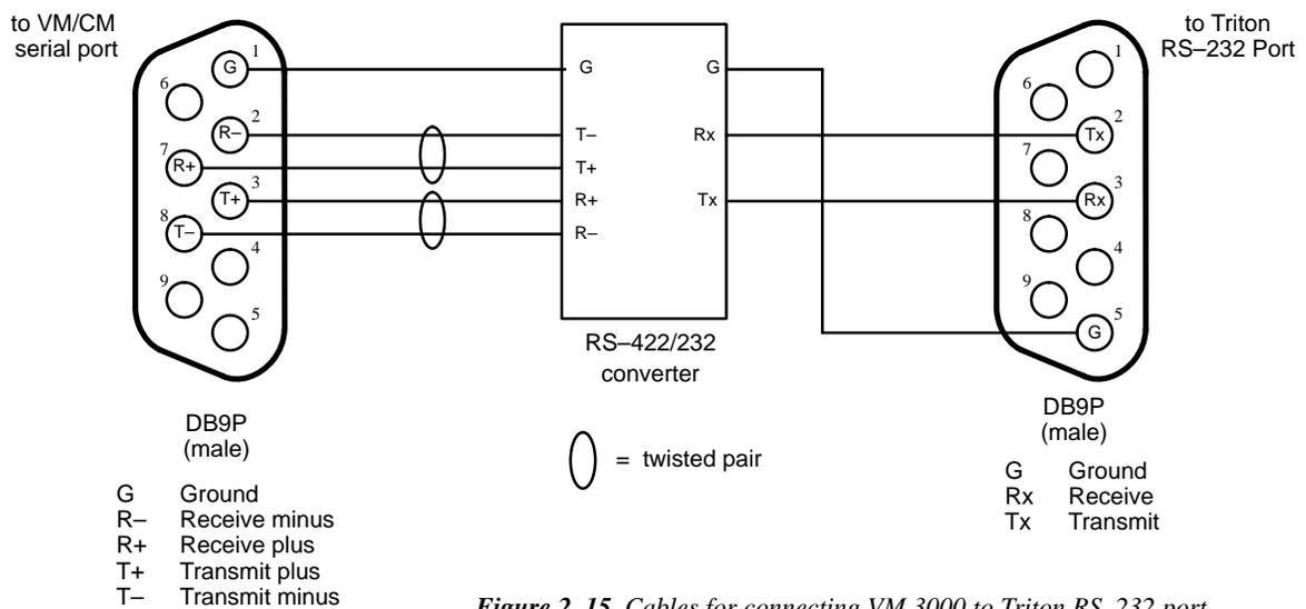
Figure 2-15. Cables for connecting VM 3000 to Triton RS-232 port.
