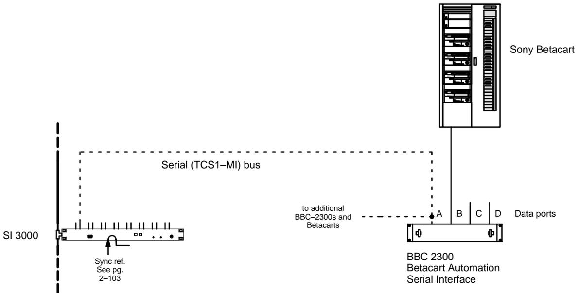
Figure 2-103. Betacart connections: systems with Thomson BBC 2300 interface.
