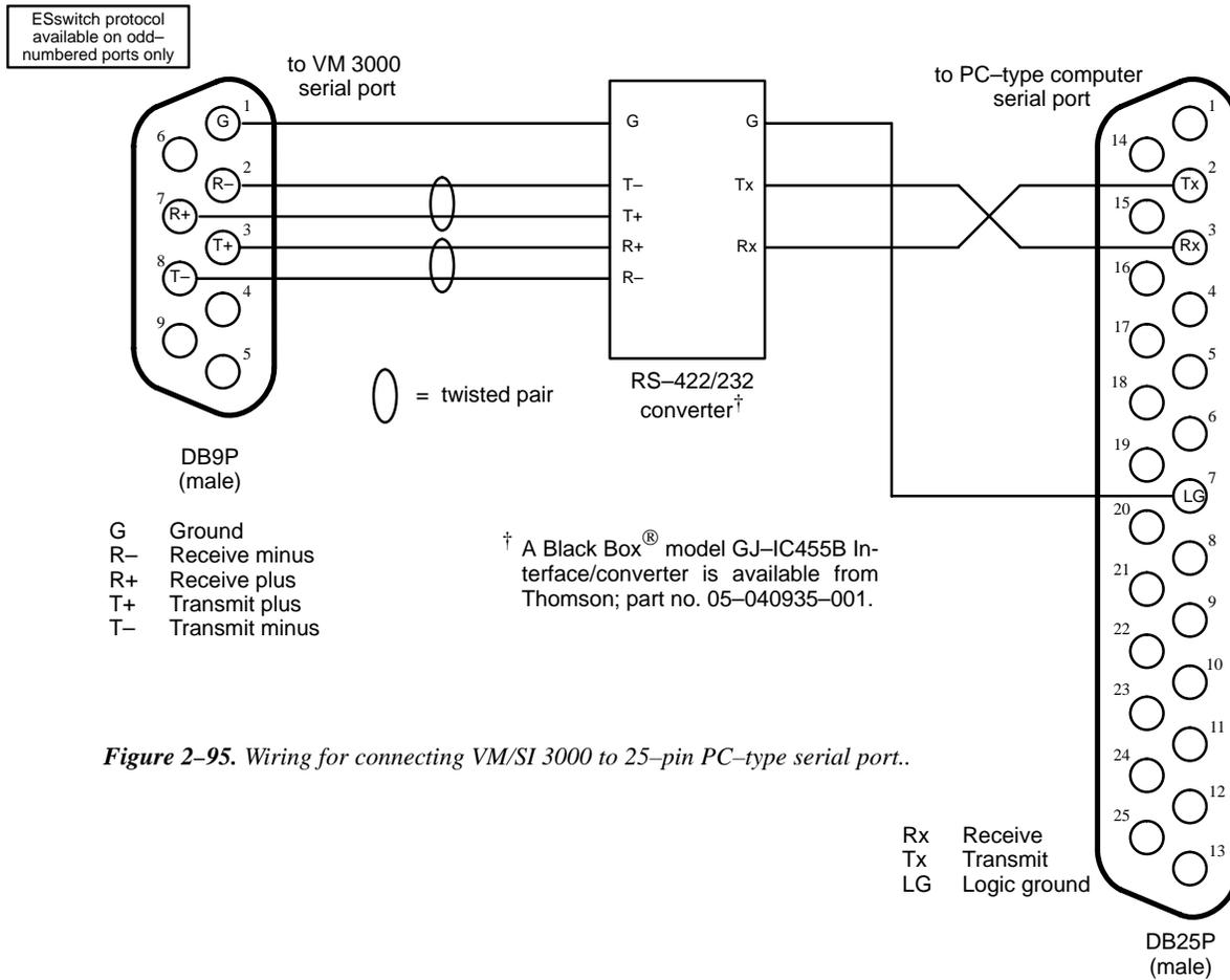
Figure 2-95. Wiring for connecting VM/SI 3000 to 25-pin PC-type serial port.
