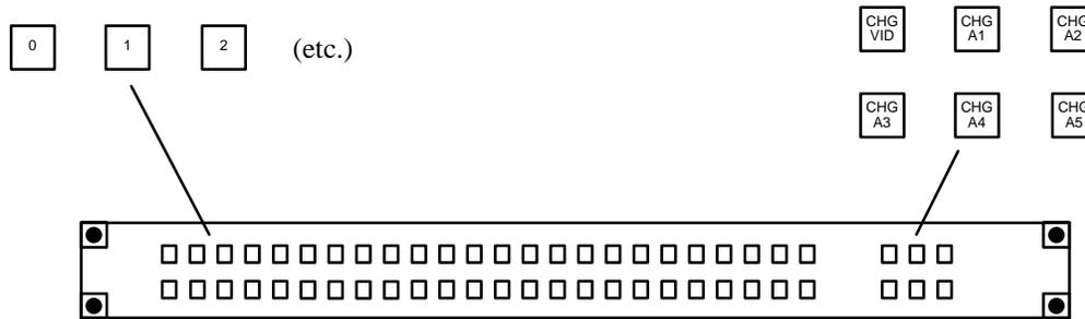
Figure 2-55. CP-330 Control Panel (as supplied).
