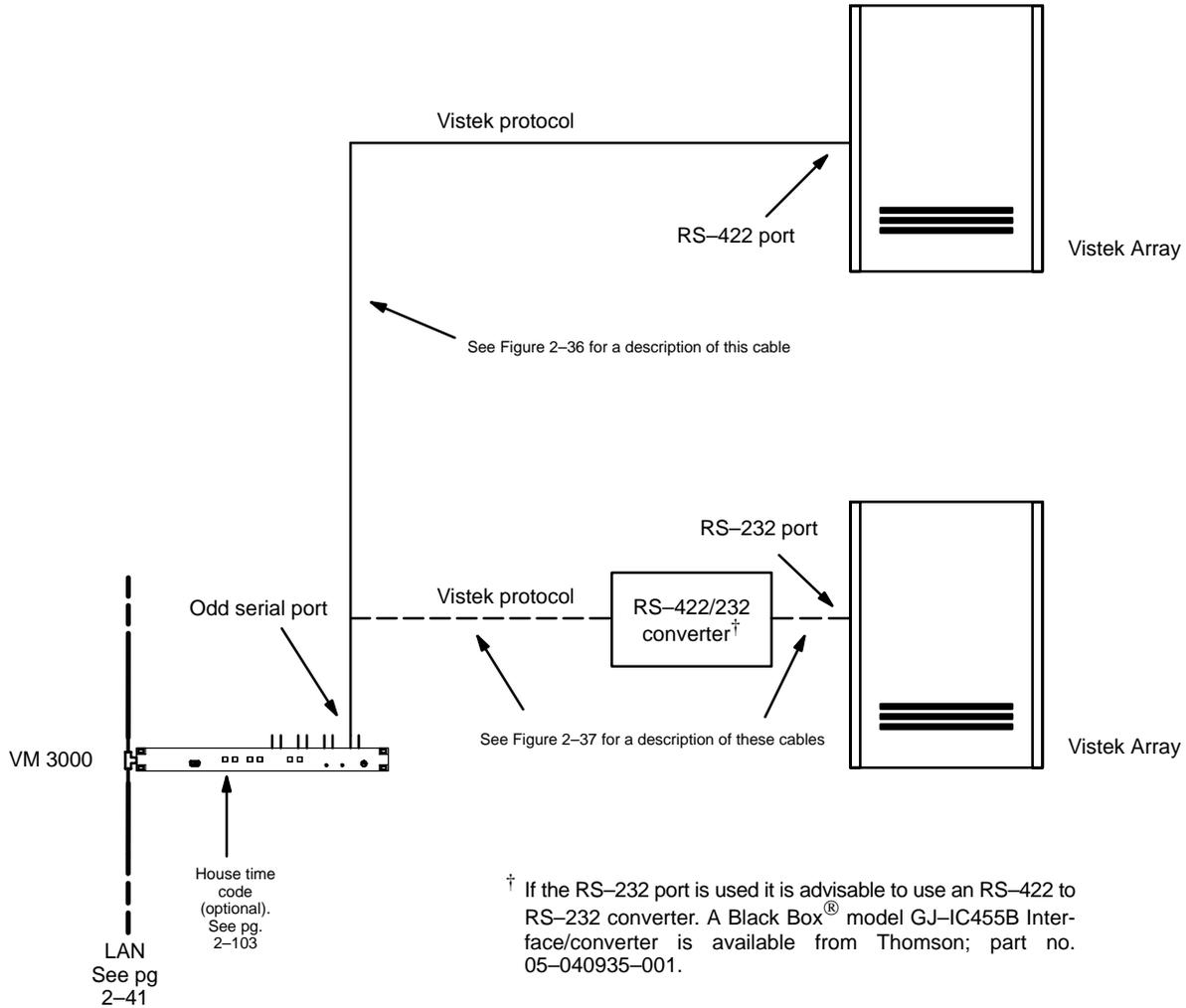
Figure 2-35. Alternate methods for connection to Vistek Array distribution switcher.
