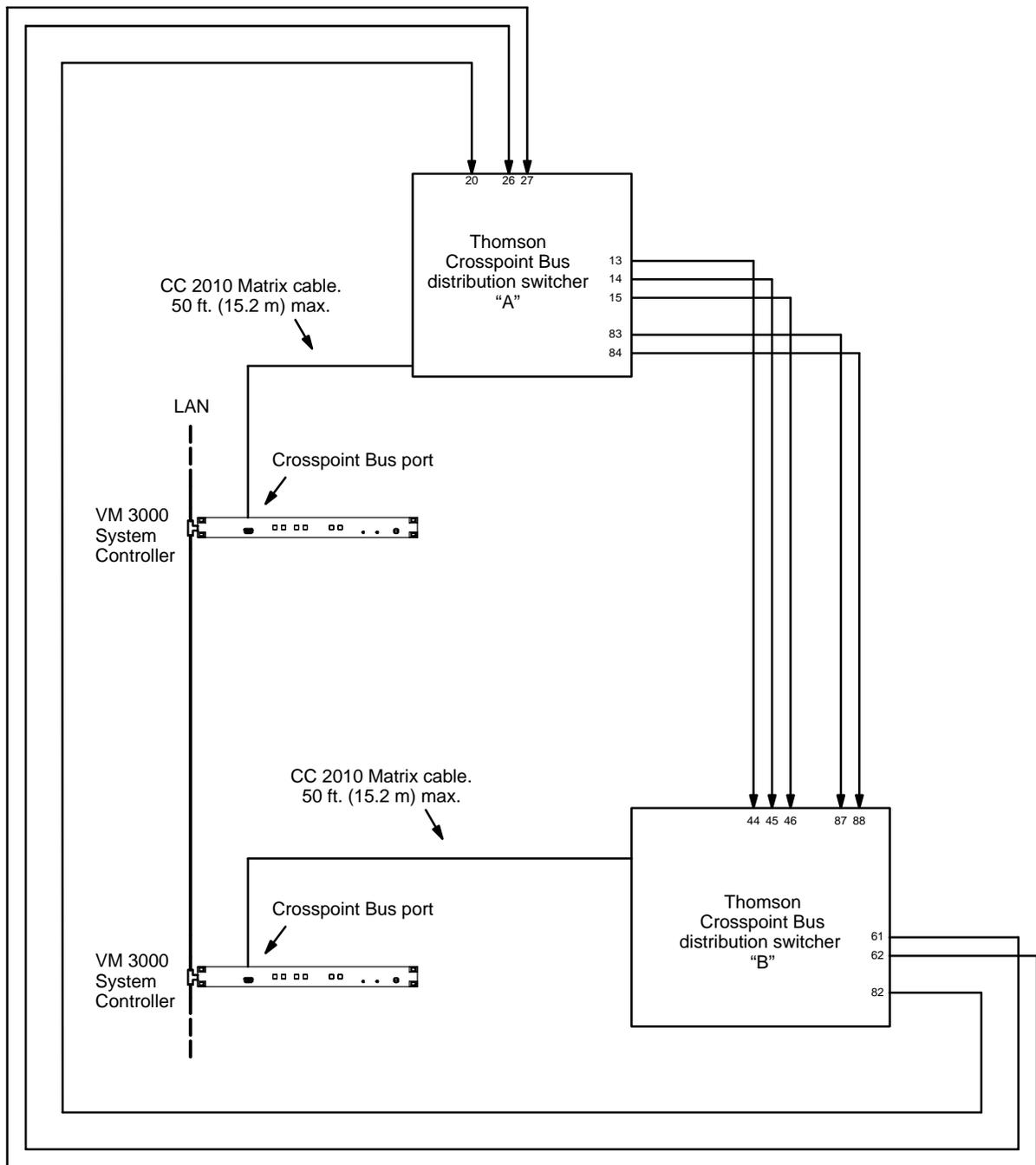
Figure 2-44. Non-sequential path finding connections (example).
