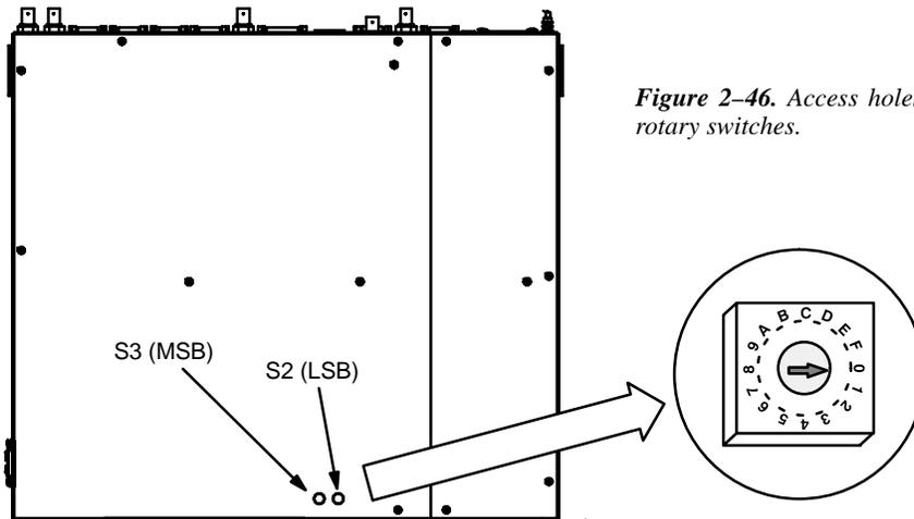
Figure 2-46. Access holes for VM/SI 3000 “Device” rotary switches.
