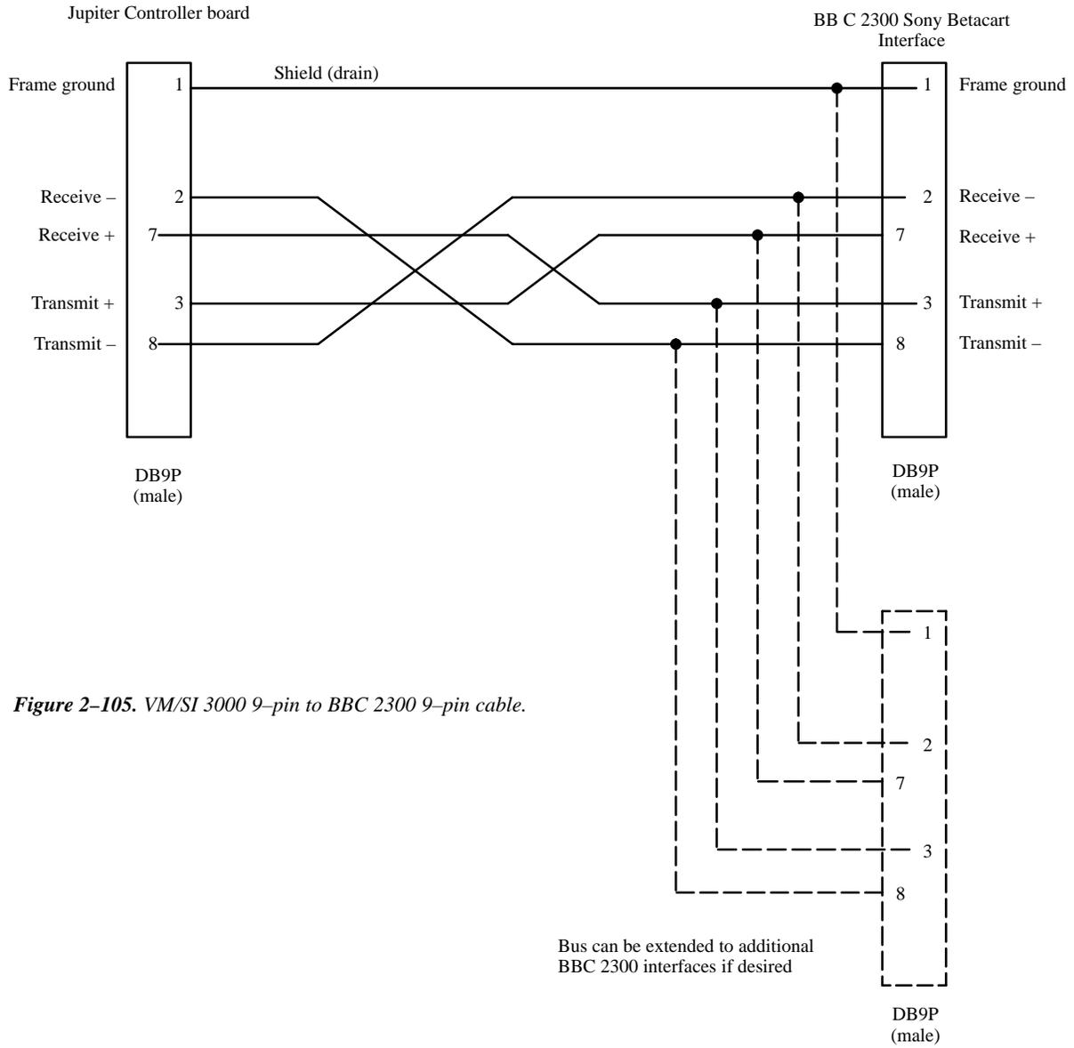
Figure 2-105. VM/SI 3000 9-pin to BBC 2300 9-pin cable.
