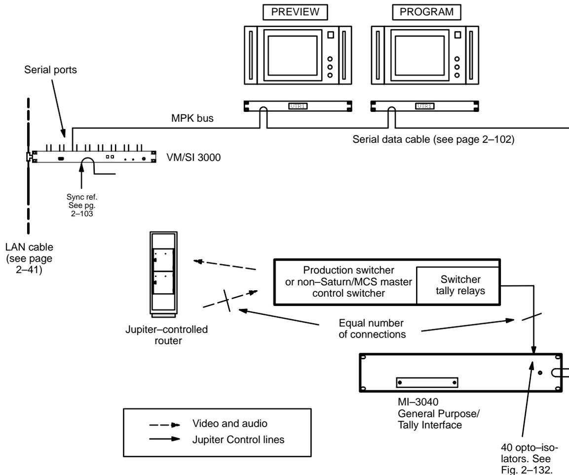
Figure 2-138. Use of MI-3040 with production switcher / non-Saturn non-MCS master control switcher.
