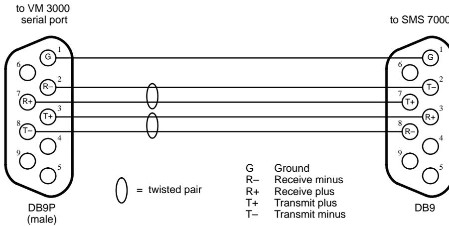
Figure 2-17. Cable for connecting VM 3000 to SMS 7000 DB9 port.
