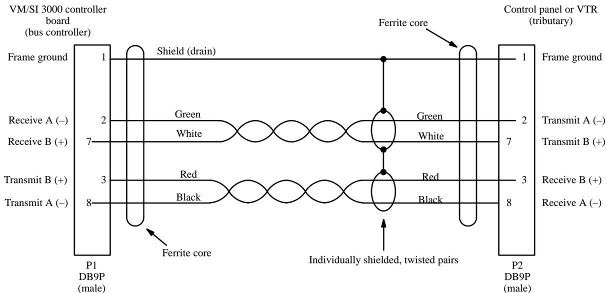
**Figure 2-116.** Serial data cable wiring. Reference: “Assembly, BCS-3000 Serial Data Cable,” Thomson drawing no. 01-041600-TAB.
