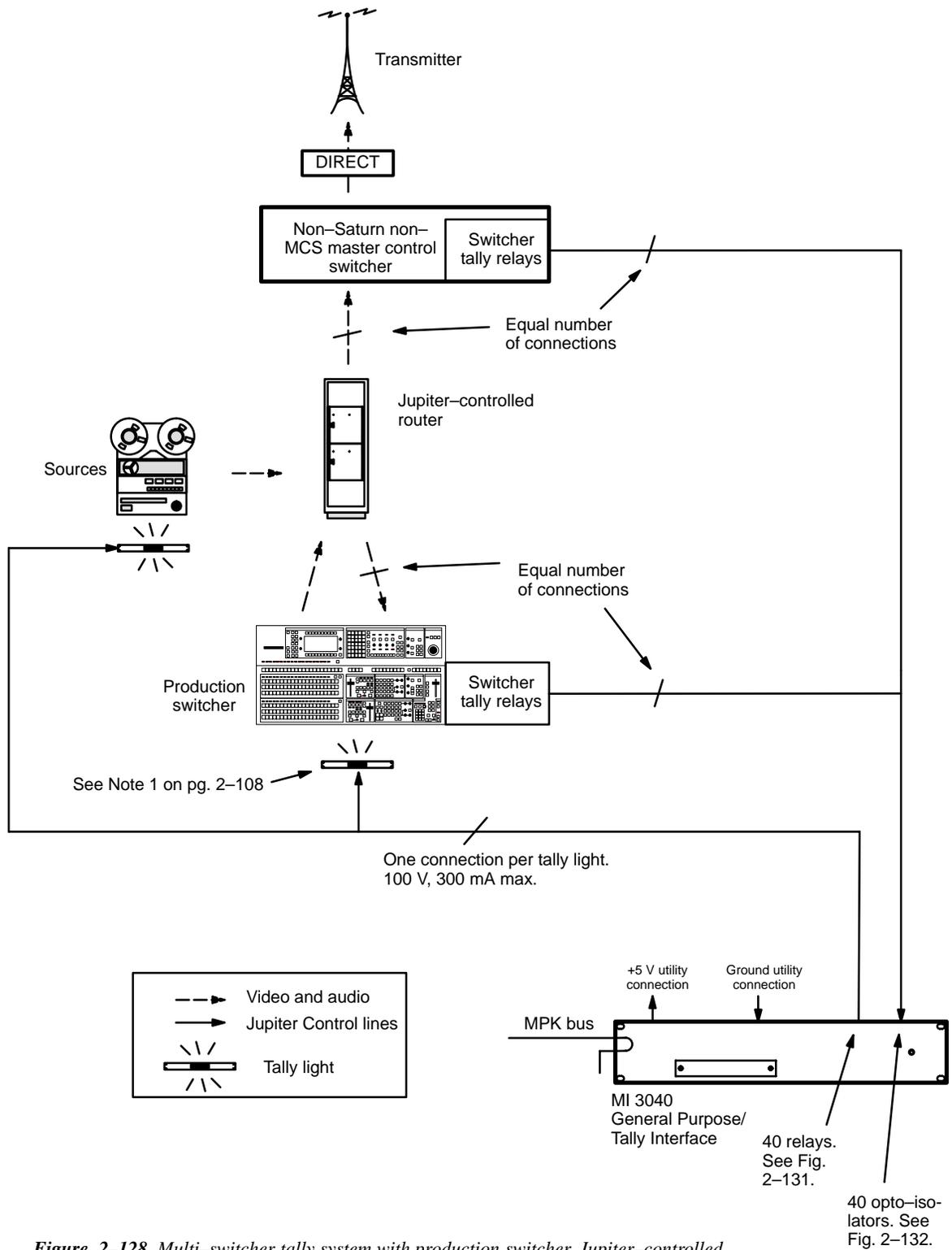
**Figure 2-128.** Multi-switcher tally system with production switcher, Jupiter-controlled router, non-Saturn/MCS master control, and direct feed to transmitter.
