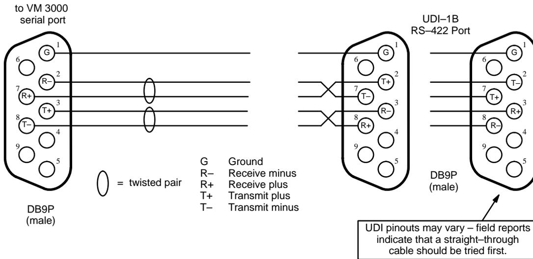
Figure 2-31. Cable for connecting VM 3000 to UDI-1B RS-422 port.
