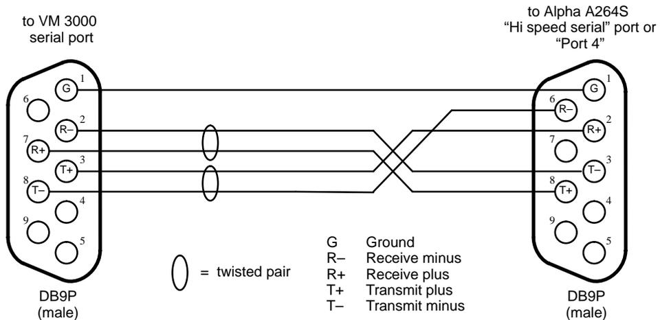
Figure 2-25. Cable for connecting VM 3000 to Alpha Image A264S switcher.
