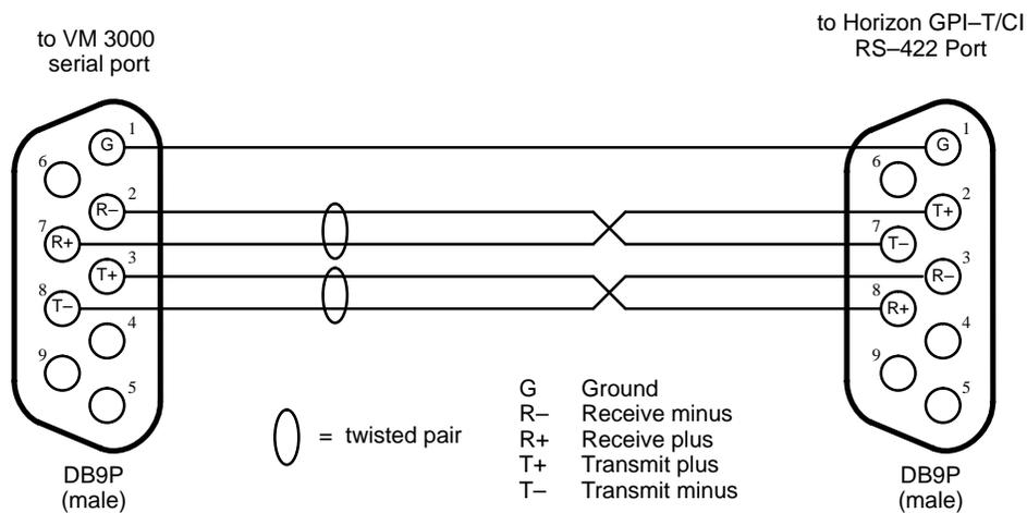
Figure 2-23. Cable for connecting VM 3000 to Horizon switcher.
