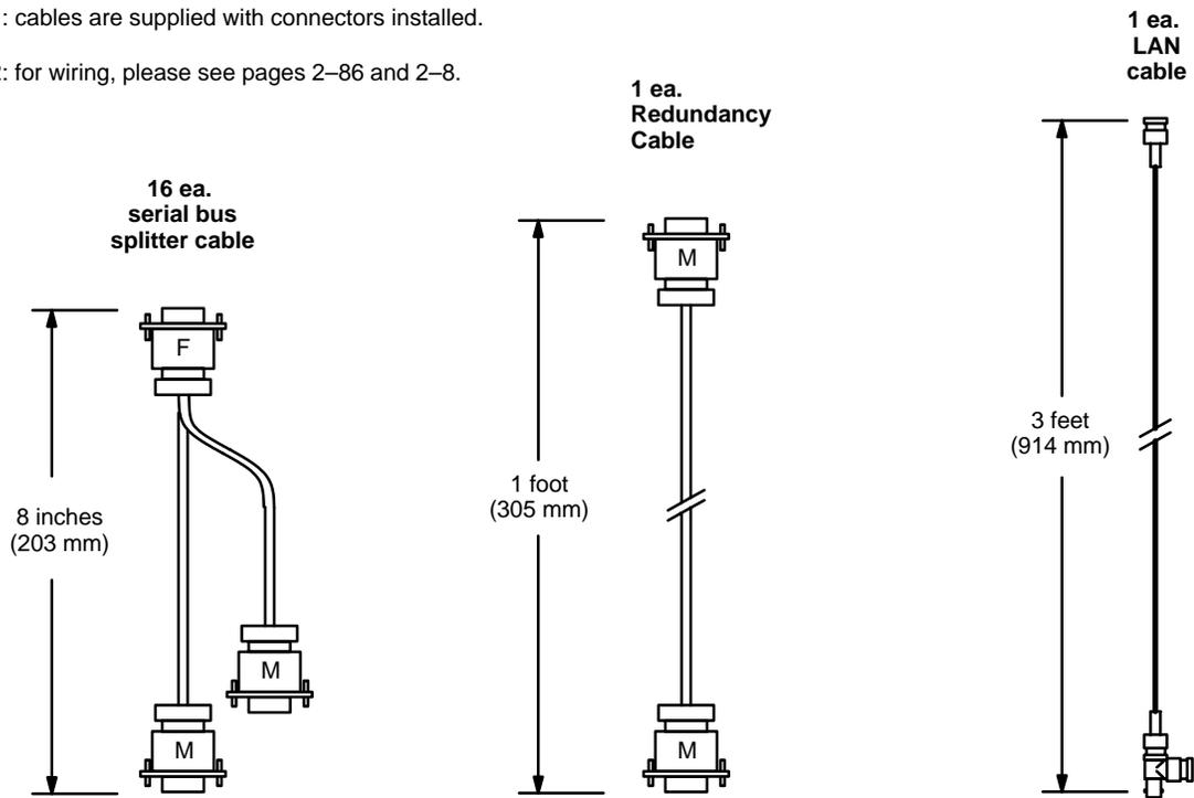
*Figure 2-100. SI 3000 redundancy kit cables. Kit part no. 44-045839-001.*
