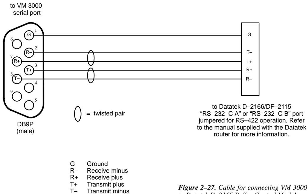
Figure 2-27. Cable for connecting VM 3000 to Datatek D-2166 Buffer Control Module.
