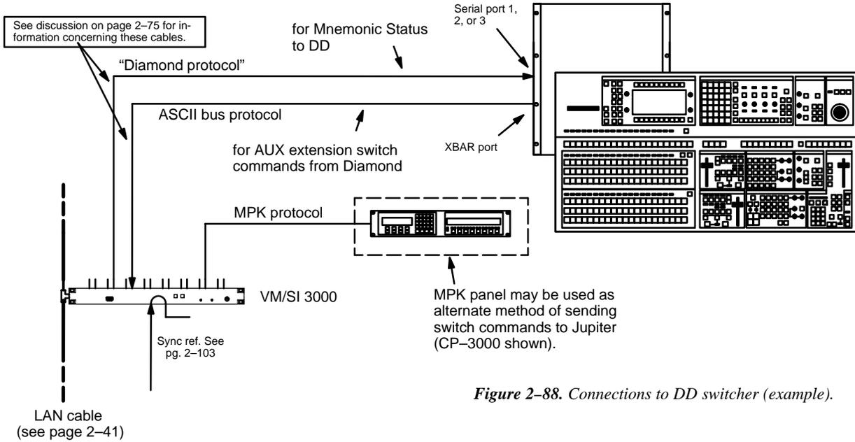
Figure 2-88. Connections to DD switcher (example).
