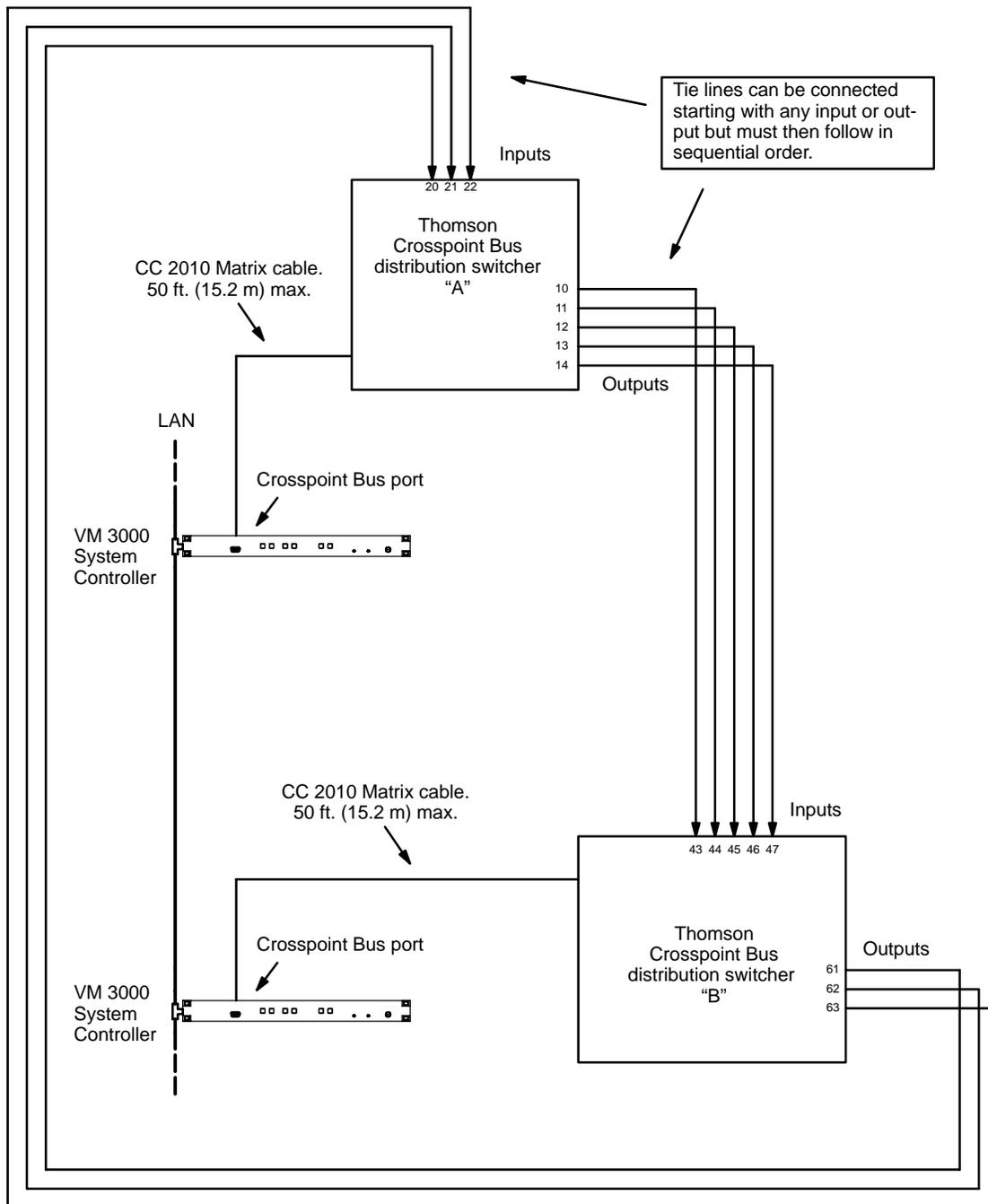
Figure 2-43. Sequential path finding connections (example).
