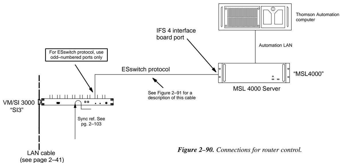
Figure 2-90. Connections for router control.
