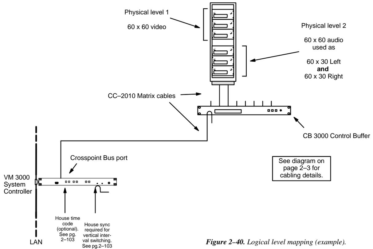
Figure 2–40. Logical level mapping (example).
