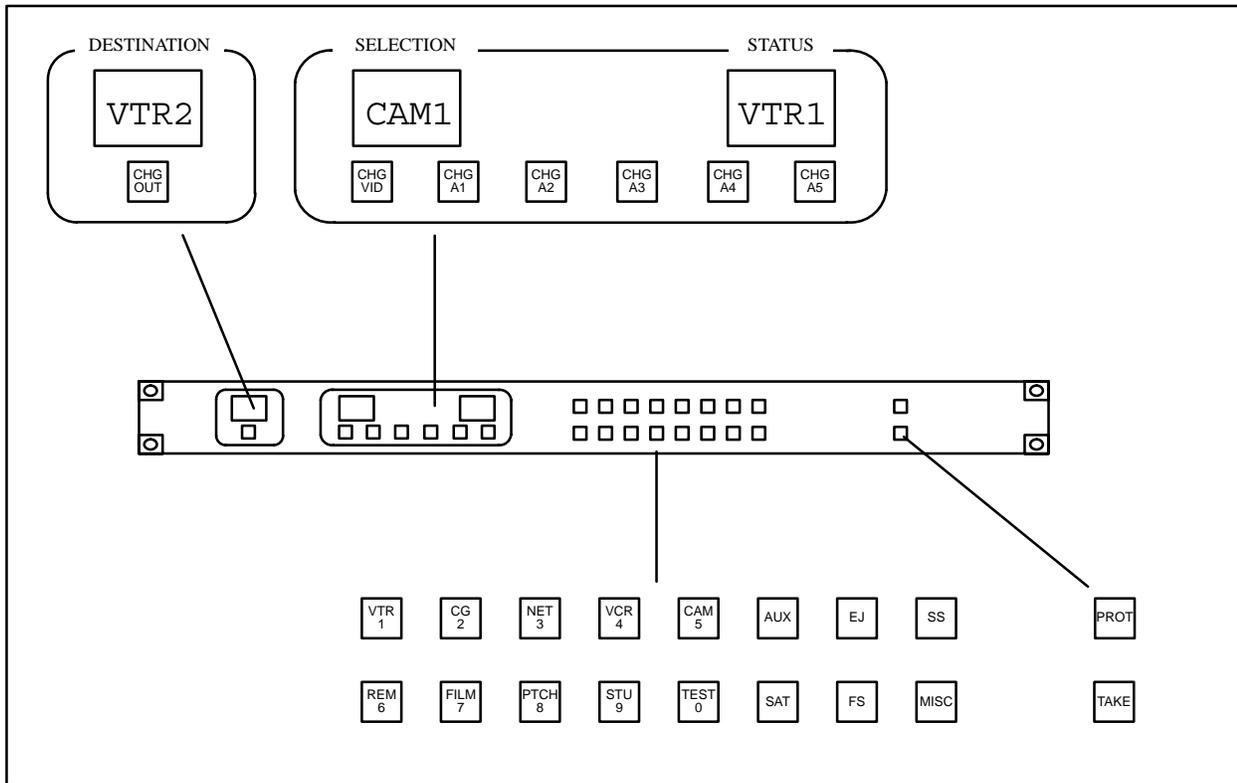
Figure 2–54. CP 320 Push Button Control Panel (as supplied).
