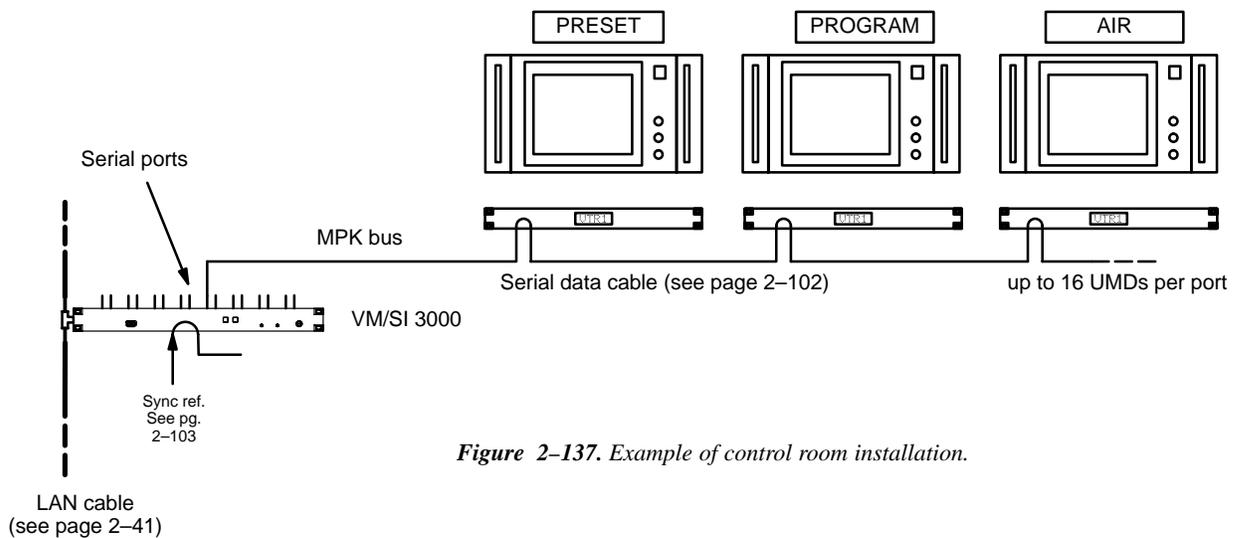
Figure 2-137. Example of control room installation.
