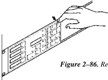
Figure 2–86. Removing CP 3800 series keycaps.
