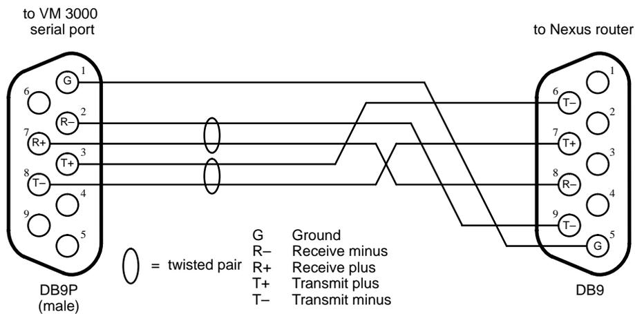
Figure 2-39. Cable for connecting VM 3000 to Nexus audio router.
