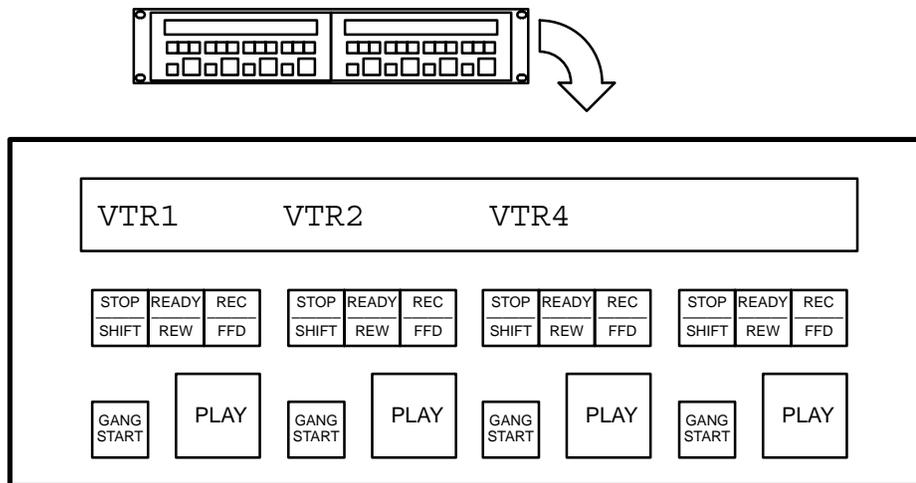
**Figure 2-78.** MC 3010/2 Dual 4-Machine Control Panel.
