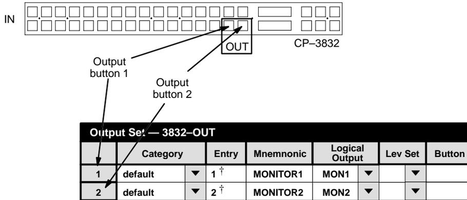
Figure 5-72. Entries for CP 3832 configured as 30 x 2 “unbalanced split” panel.
