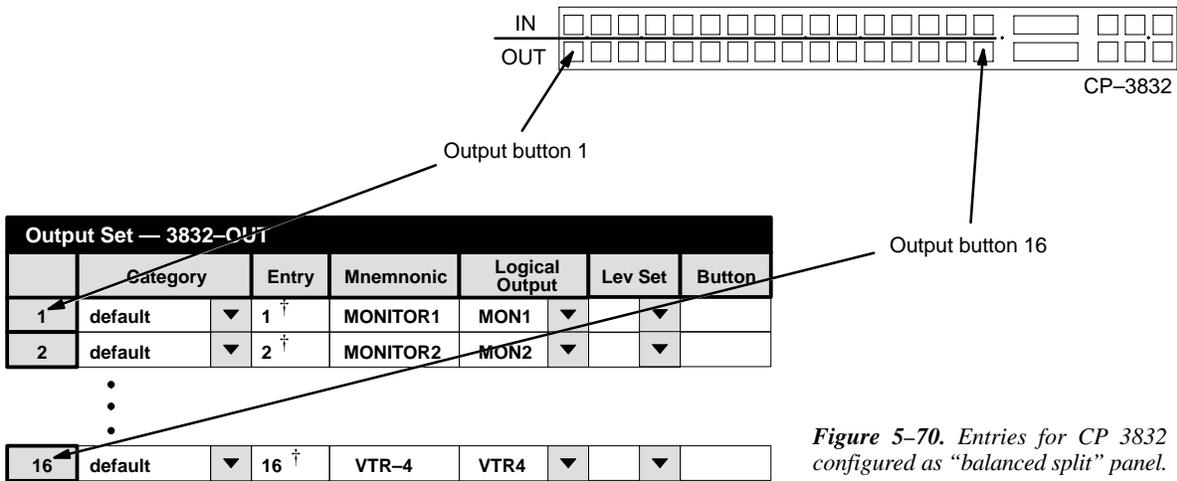
Figure 5–70. Entries for CP 3832 configured as “balanced split” panel.
