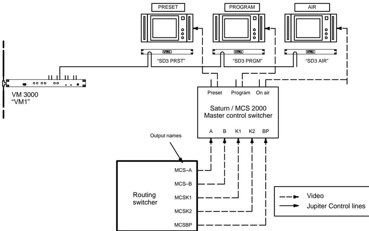
**Figure 5-100.** Example of status display system with Saturn/MCS master control switcher. Equipment shown here corresponds to tables on page 5-123.
