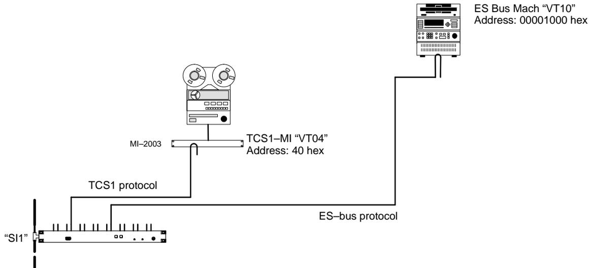
Figure 5-130. Machine control devices listed in table on page 5-129.
