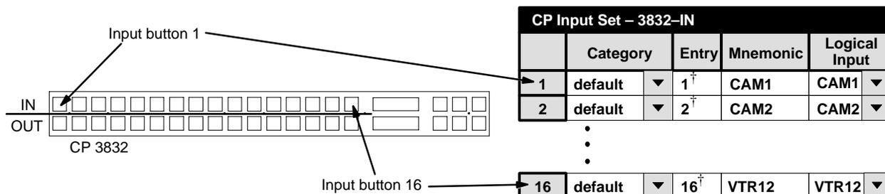
Figure 5–52. Entries for CP 3832 configured as “balanced split” panel. Balanced number of input/output buttons is determined by output assignments made on the CP Output Set. For details, see page 5–92.
