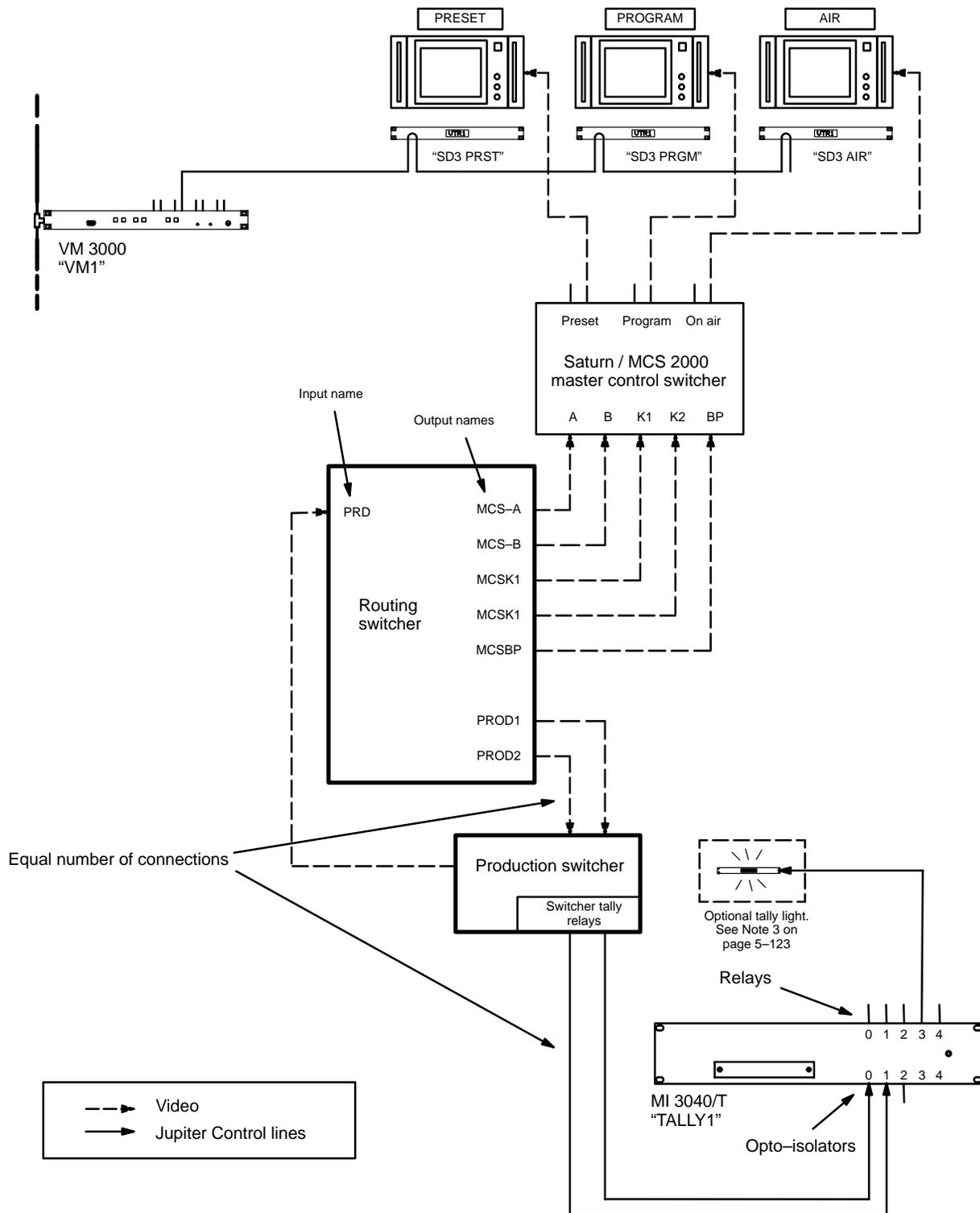
**Figure 5-102.** Example of status display system with Saturn / MCS 2000 master control switcher and production switcher. Equipment shown here corresponds to tables on page 5-127.
