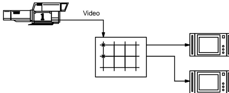
In a data switcher, it may be desirable to restrict operation to “point-to-point” switching. For example, this would insure that the transmit data from an editor could be switched to only one VCR at a time, as shown in Figure 5–24.
