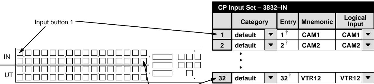
Figure 5-55. Entries for CP 3864 configured as 32 x 32 “balanced split” panel. Balanced number of input/output buttons is determined by output assignments made on the CP Output Set. For details, see page 5-92.
