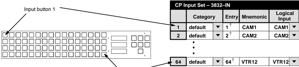
Figure 5-54. Entries for CP 3864 operated as single-bus panel.
