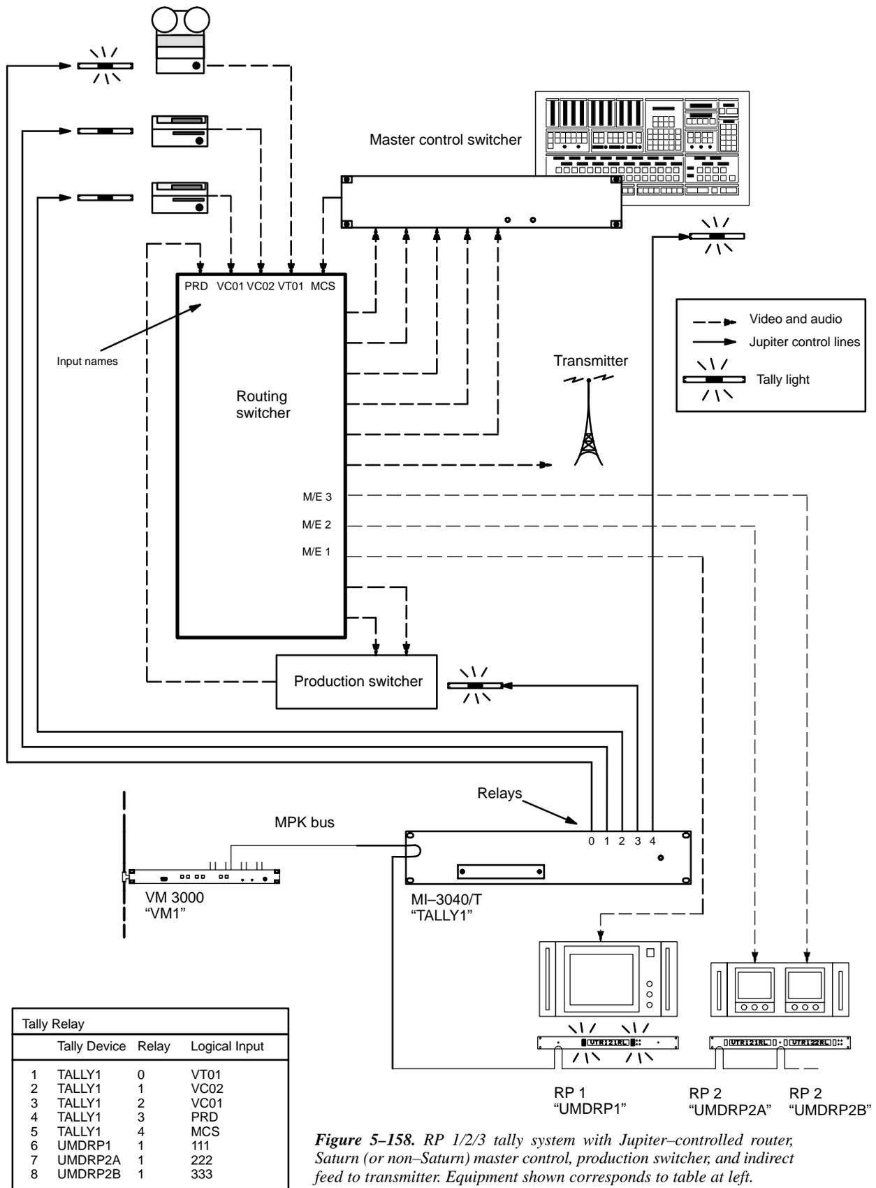
Figure 5-158. RP 1/2/3 tally system with Jupiter-controlled router, Saturn (or non-Saturn) master control, production switcher, and indirect feed to transmitter. Equipment shown corresponds to table at left.
