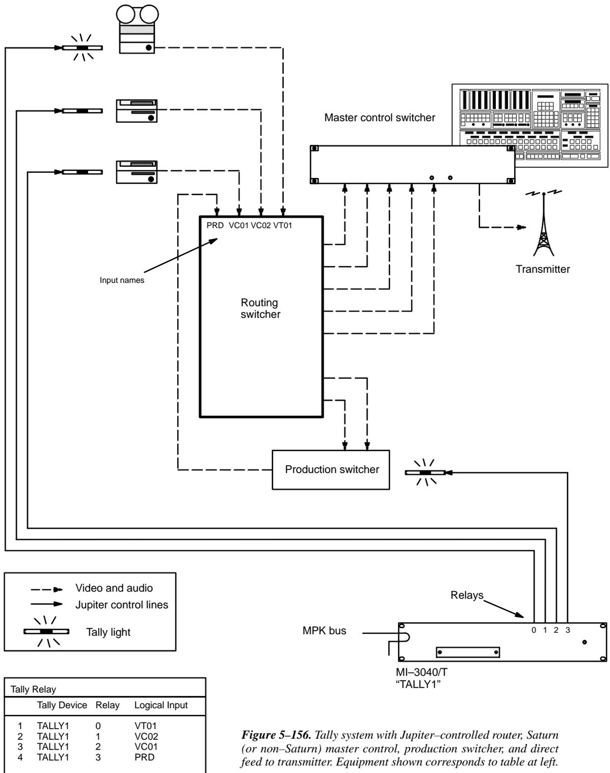
Figure 5-156. Tally system with Jupiter-controlled router, Saturn (or non-Saturn) master control, production switcher, and direct feed to transmitter. Equipment shown corresponds to table at left.
