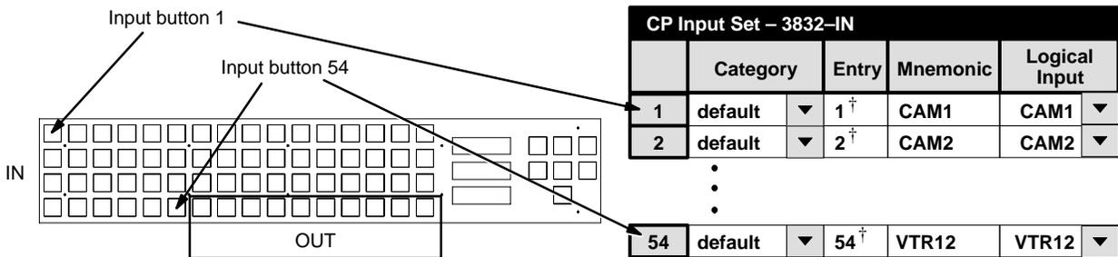
Figure 5-56. Entries for CP 3864 configured as 54 x 10 “unbalanced split” panel. Total number of input buttons vs. total number of output buttons is determined by number of output assignments made on the CP Output Set. For details, see page 5-92.
