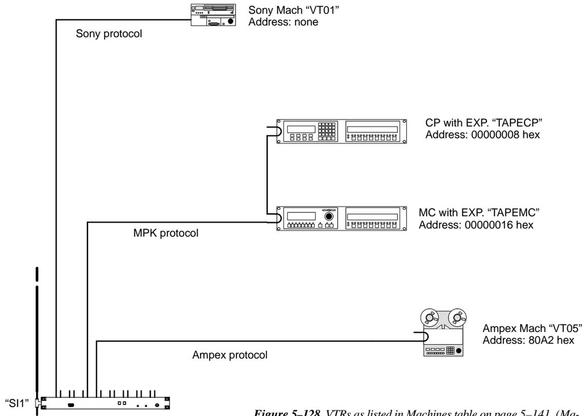
**Figure 5-128.** VTRs as listed in Machines table on page 5-141. (Machine control panels are listed in MPK table on page 5-108.)
