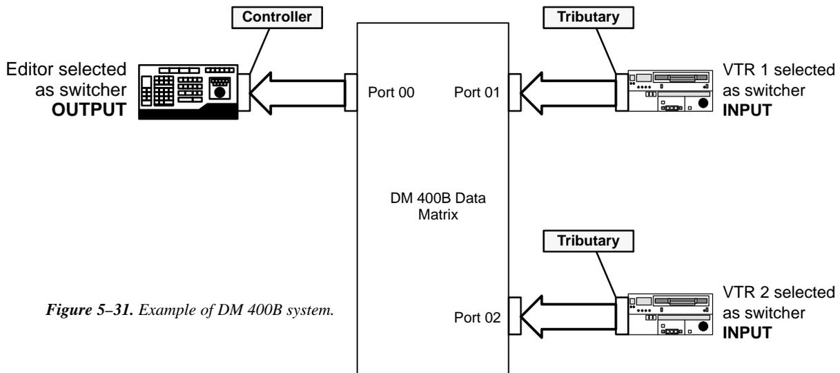
Figure 5–31. Example of DM 400B system.
