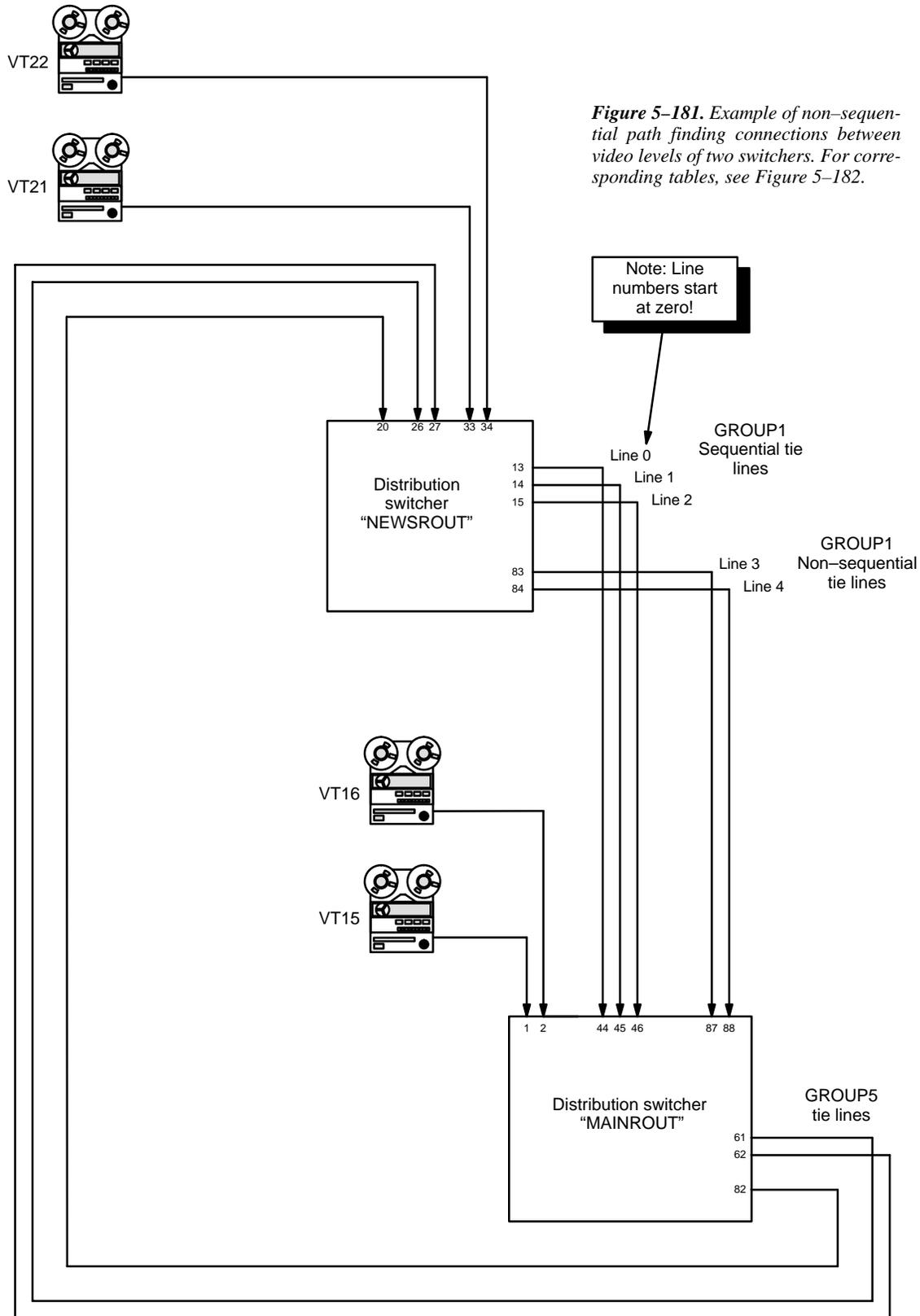
**Figure 5-181.** Example of non-sequential path finding connections between video levels of two switchers. For corresponding tables, see Figure 5-182.
