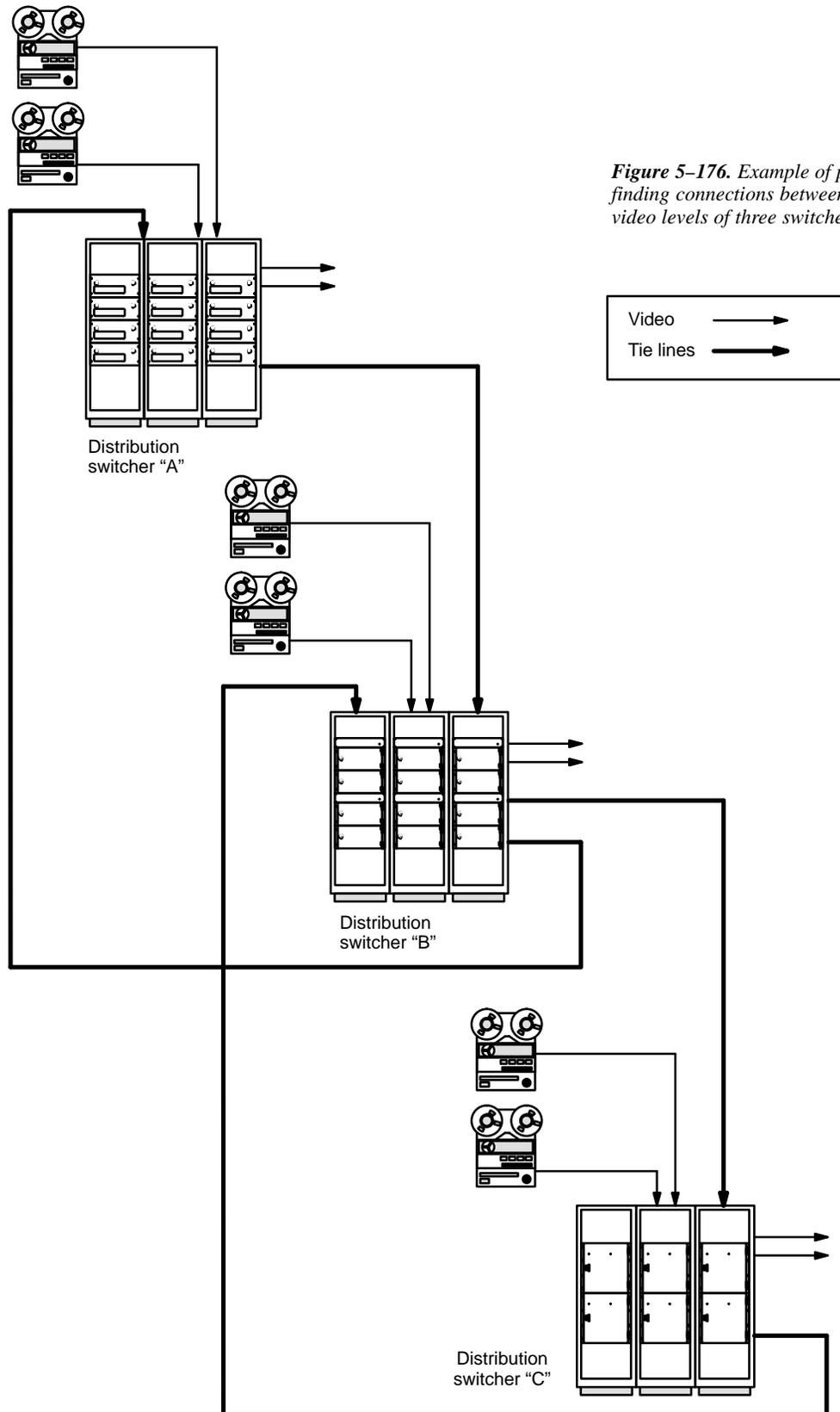
Figure 5-176. Example of path finding connections between video levels of three switches.
