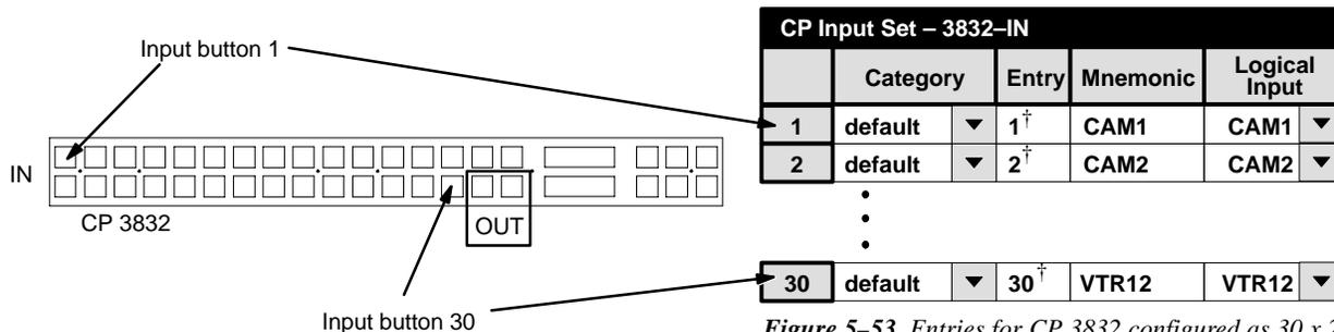
Figure 5–53. Entries for CP 3832 configured as 30 x 2 “unbalanced split” panel. Total number of input buttons vs. total number of output buttons is determined by number of output assignments made on the CP Output Set. For details, see page 5–92.
