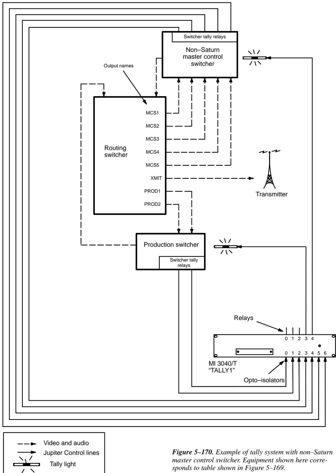
**Figure 5-170.** Example of tally system with non-Saturn master control switcher. Equipment shown here corresponds to table shown in Figure 5-169.
