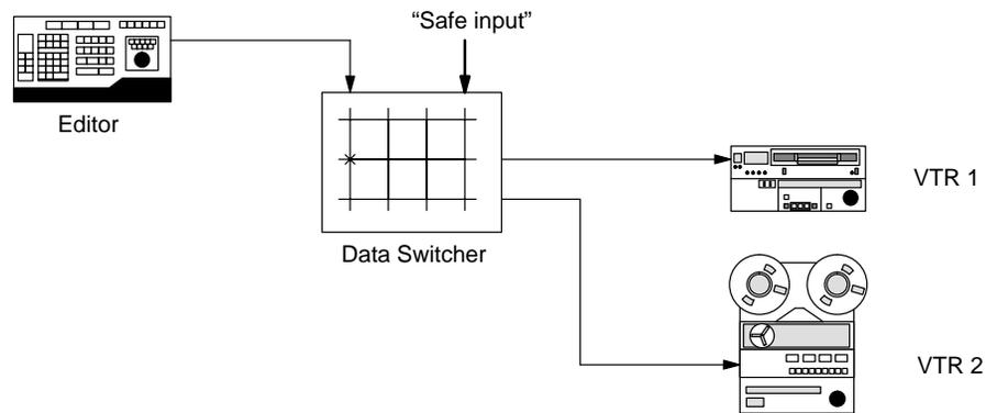
To avoid this problem, the data switcher can be set to switch to a Safe input, wait for a specified minimum number of frames, and then switch to the new device. This will cause the editing system to send a request to the new VTR to identify itself and get the correct ballistics.
