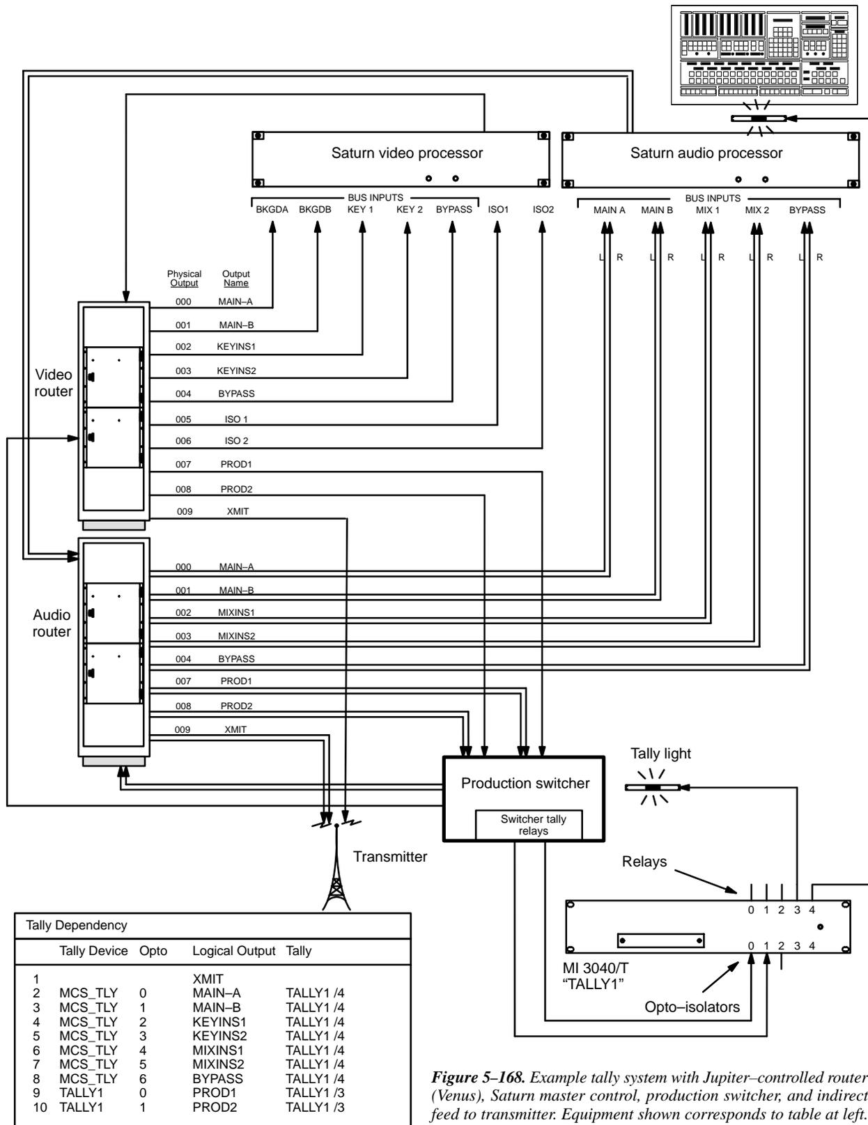
Figure 5-168. Example tally system with Jupiter-controlled router (Venus), Saturn master control, production switcher, and indirect feed to transmitter. Equipment shown corresponds to table at left.
