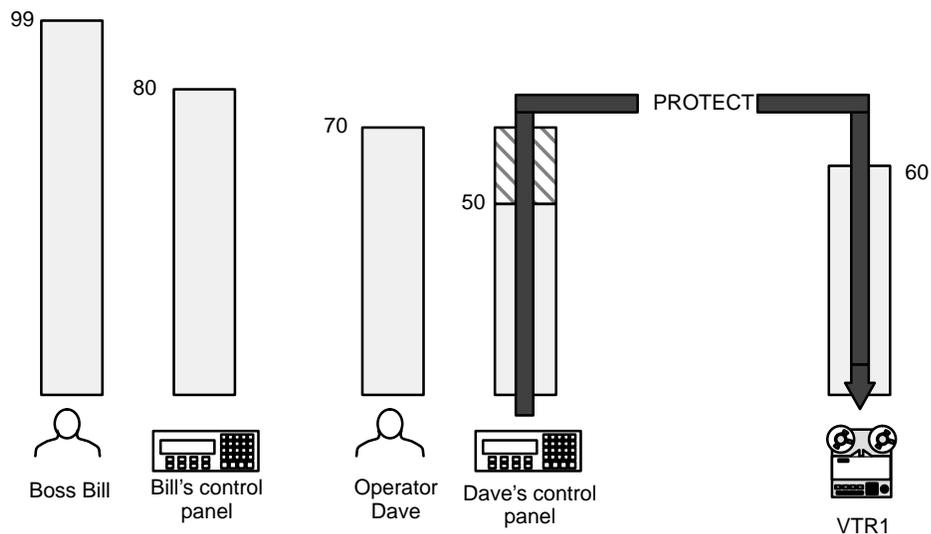
A more rigorous form of protection is *lock*, where the output must be deliberately *unlocked* before changing the source for a particular destination (Figure 5-14). Only the panel used to lock the output could unlock the output. †
