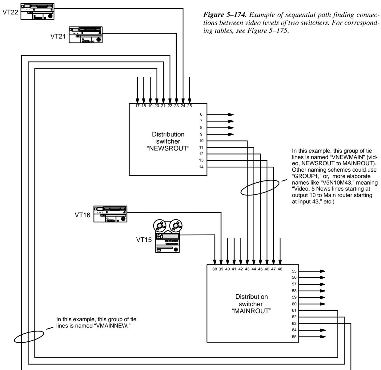
Figure 5-174. Example of sequential path finding connections between video levels of two switchers. For corresponding tables, see Figure 5-175.
