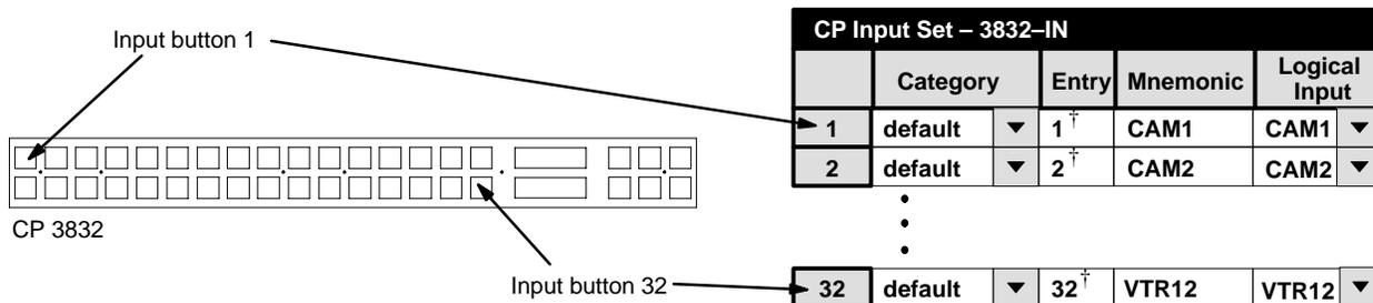
Figure 5–51. Entries for CP 3832 configured as single-bus panel.
