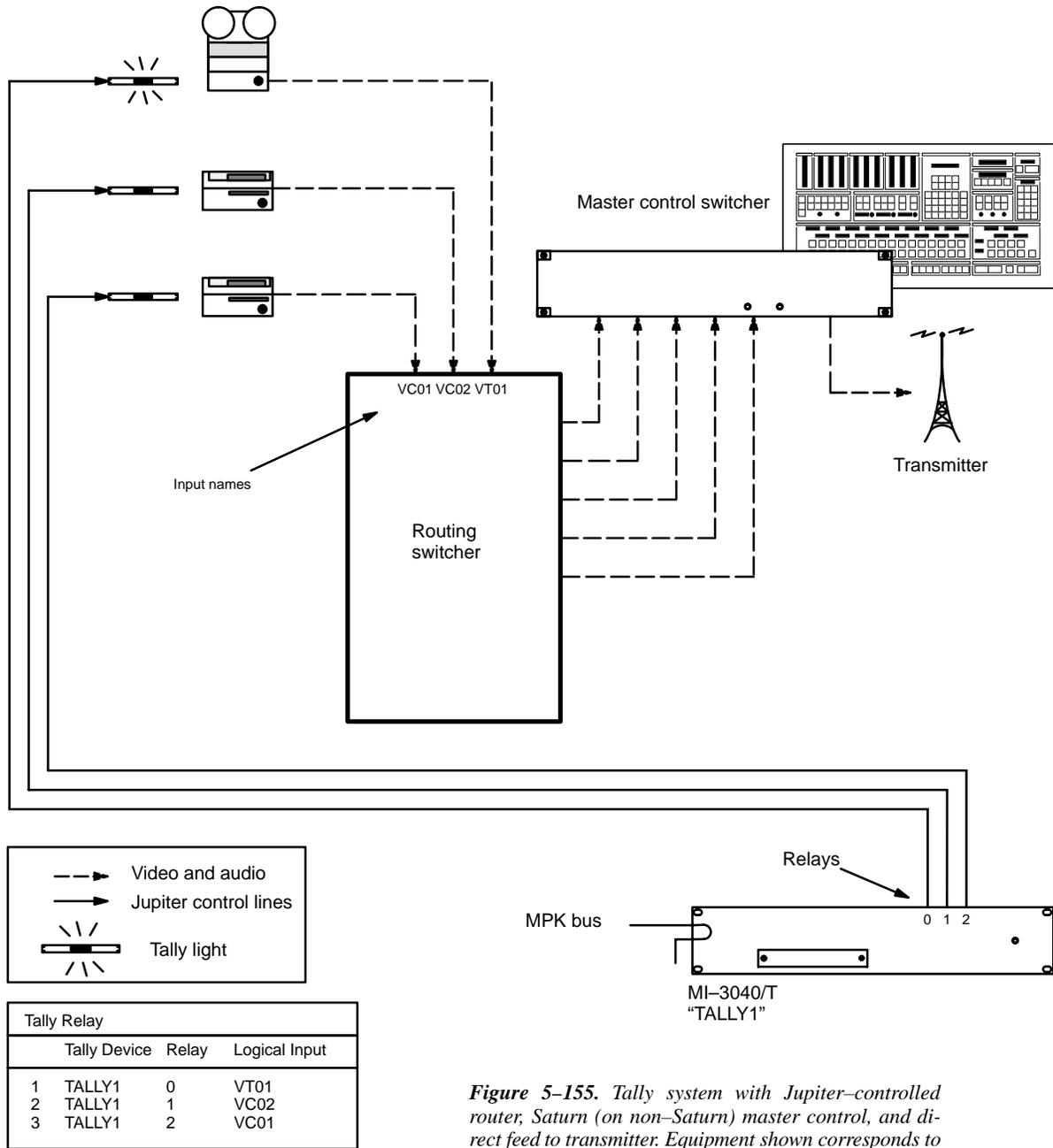
**Figure 5-155.** Tally system with Jupiter-controlled router, Saturn (on non-Saturn) master control, and direct feed to transmitter. Equipment shown corresponds to table at left.
