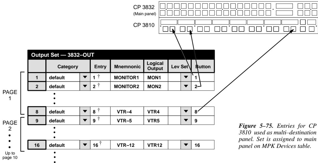
Figure 5-75. Entries for CP 3810 used as multi-destination panel. Set is assigned to main panel on MPK Devices table.
