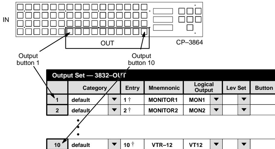
Figure 5-73. Entries for CP 3864 configured as 54 x 10 “unbalanced split” panel.
