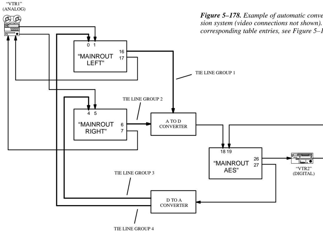
**Figure 5-178.** Example of automatic conversion system (video connections not shown). For corresponding table entries, see Figure 5-179.
