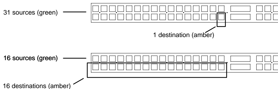
Figure 6-150. Examples of CP 3832L split configurations.
