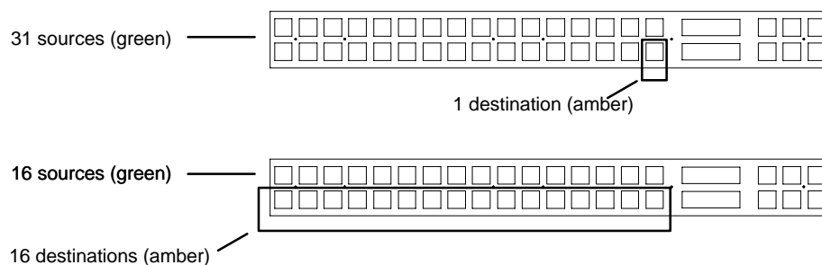
Figure 6-134. Examples of CP 3832 split configurations.
