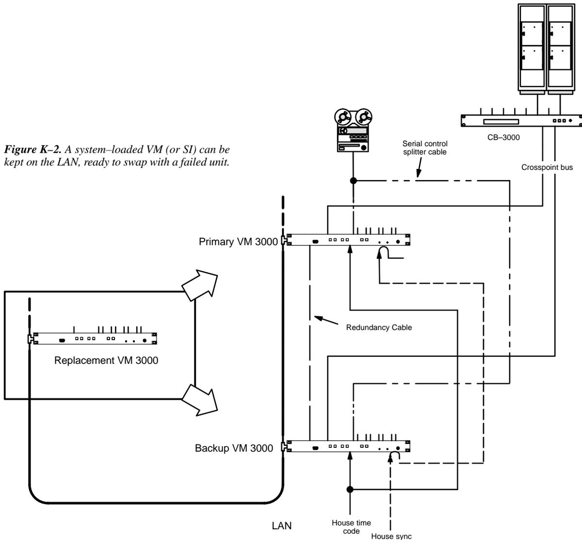
**Figure K-2.** A system-loaded VM (or SI) can be kept on the LAN, ready to swap with a failed unit.
