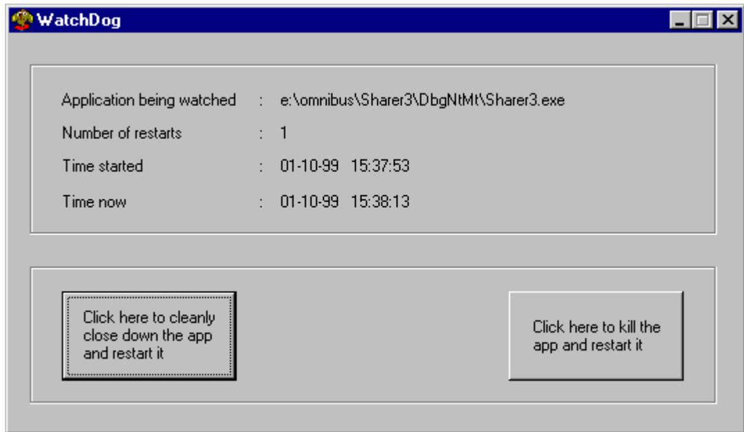
The Watchdog application is designed to minimise problems due to crashes. It is a simple application that runs up the Sharer and watches it. If the application terminates for any reason, the watchdog restarts it. It can be used on any application, but has one Sharer specific feature.
