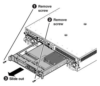
2. When replacing the carrier module, the screw attachment sequence is critical, as illustrated.
