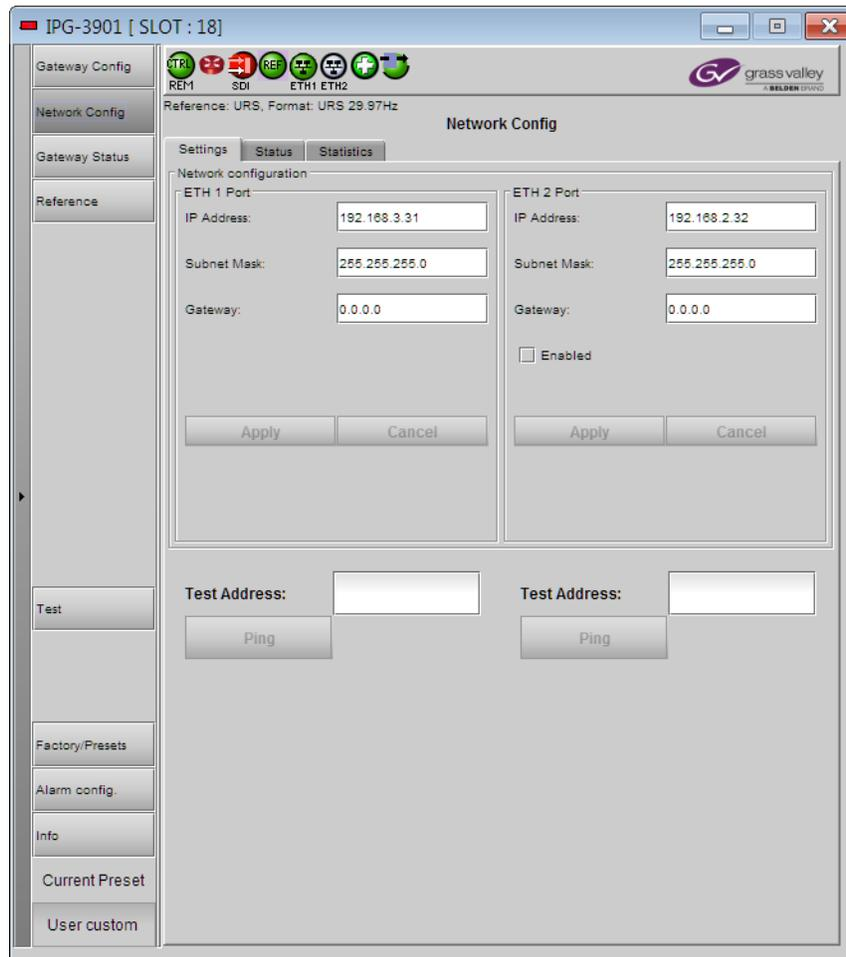
**Note:** These settings apply to the rear-panel Ethernet port of the KMX-3901-IN-IP input/output cards; *not* to the Ethernet ports at the back of the CPU-ETH3 frame controller card.
