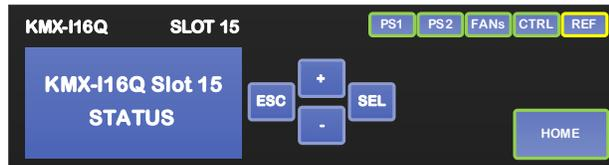
The panel is assigned to operate any card in the frame by pressing the icon representing the appropriate card on the Densité 3+ FR1 frame's local control panel touch display. Alternatively, pressing the status button on the front edge of a card will also bring up the menu. The Status LED on the selected card becomes flashing orange.
