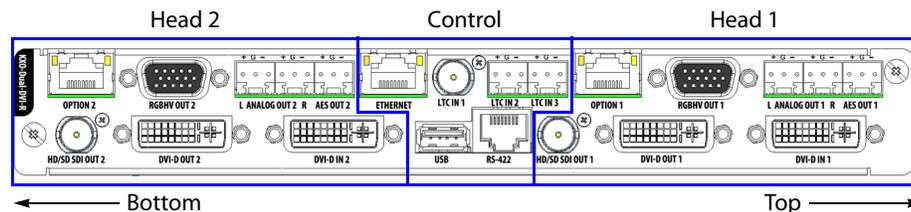
When the rear panel is horizontal and you can read the connector labels normally, the connectors located at the right-hand side are the *Head 1* connectors and the connectors located at the left-hand side are the *Head 2* connectors
