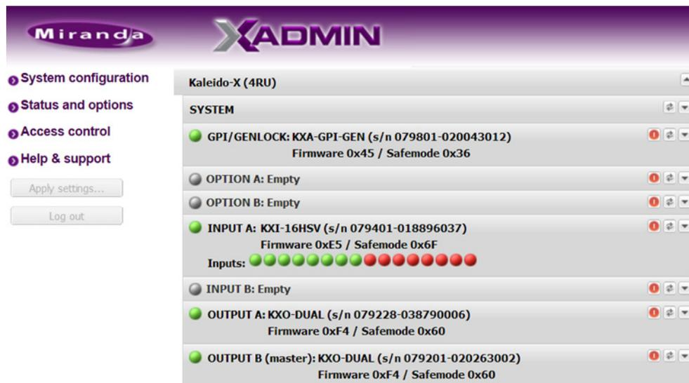
Cards are presented in the order they appear, from left to right when looking at the front of the chassis. The card heading shows the card type, serial number, firmware and safemode versions, and a summary view of the input signals for each input card.
