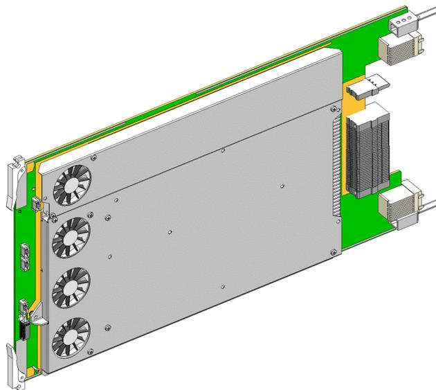
The KXO-EXP card must be installed in the slot labelled OUTPUT D / EXP (color-coded yellow) in the Kaleido-X frame.
