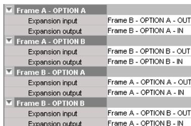
All sources can now be routed to any internal router destination via the router expansion cables.
