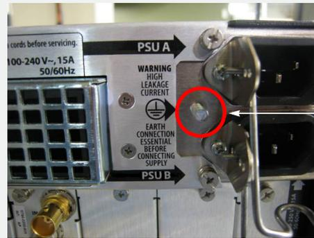
Connect a ground cable between this stud and the rack
