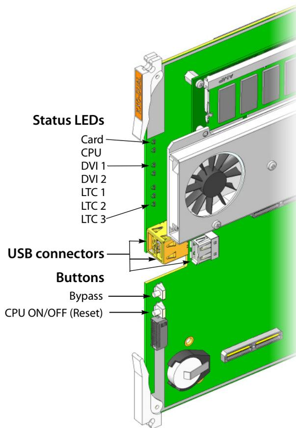
The front card-edge connectors are not accessible in normal use, as they are covered by the front door of the frame. They are provided for maintenance purposes, or for special circumstances. One exception is the recessed USB connector, which can hold a USB key that can be left in place during operation with the door closed.
