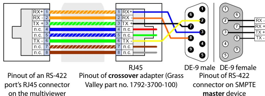
*Standard wiring between multiviewer and devices wired to SMPTE "master" specification (e.g. Philips Jupiter router control system, Grass Valley Presmaster PCS)*
