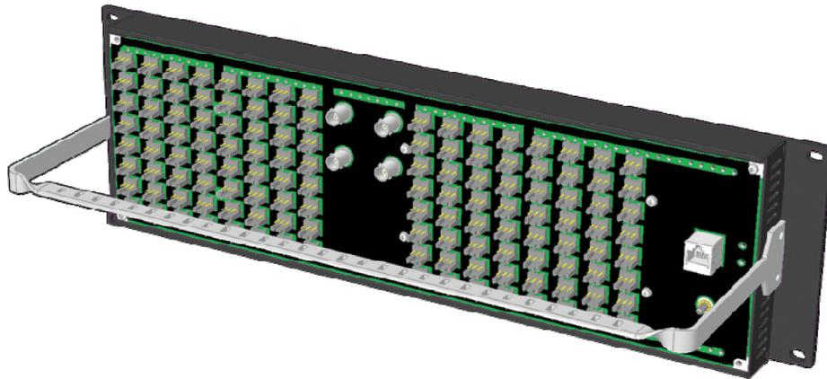
Note: The ABT is powered through the RJ-45 Ethernet connector. There is no power ON/OFF button, so the device is ON whenever a powered Ethernet cable (PoE) is connected.
