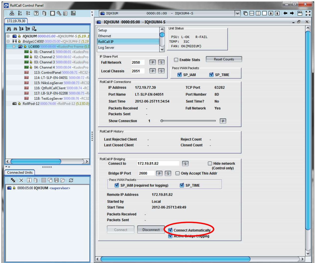
Figure 6: RollCall IP Bridging Connected
