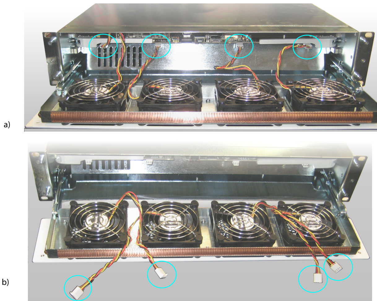
Fig. 6-8: Door-Fan Supply Wires: a) Fan Wires Connected to MV-821 Main Module. b) Fan Wires Disconnected.
