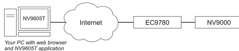
Figure 1-1. Network Connections for the NV9605T
