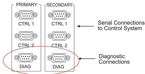
Figure 2-9. Permanent Diagnostic Connections (Rear View)
