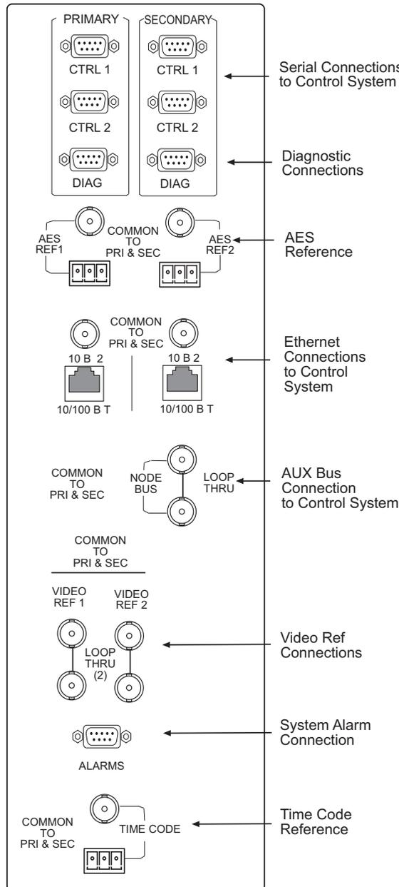
Figure 2-5. System Connections
