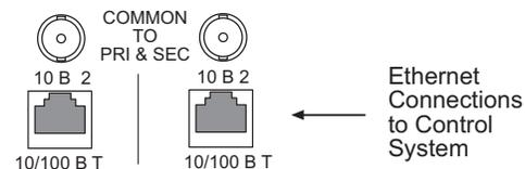
Figure 2-7. Ethernet Control Connections (Rear View)
