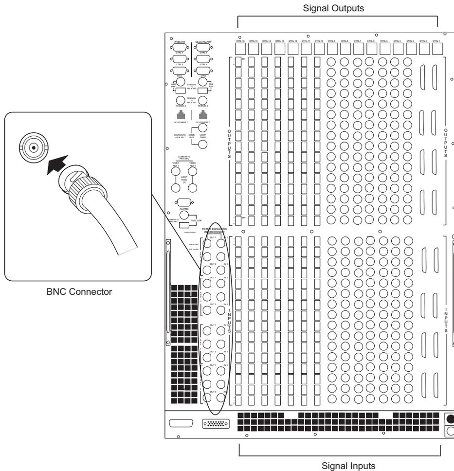
Figure 3-17. Example of Frame Expansion Connections on NV7256Plus (Rear View)
