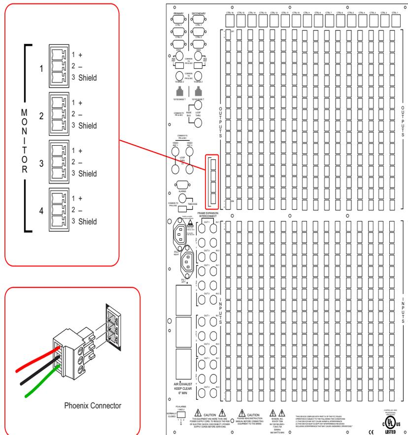
Figure 3-28. Example of Monitor Connections and Phoenix Connectors on NV7256 (Rear View)
