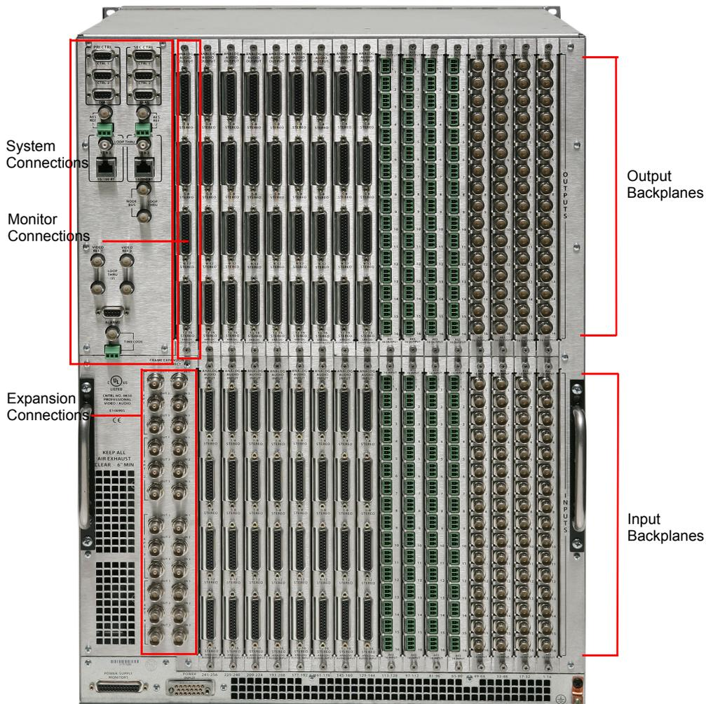
Figure 2-3. NV7256Plus Router (Rear View)
