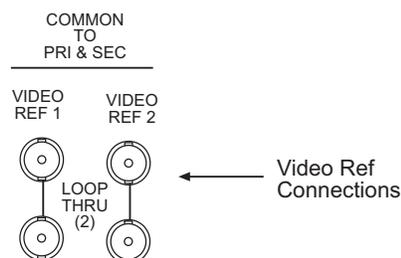
Figure 2-11. Connections to Video References (Rear View)
