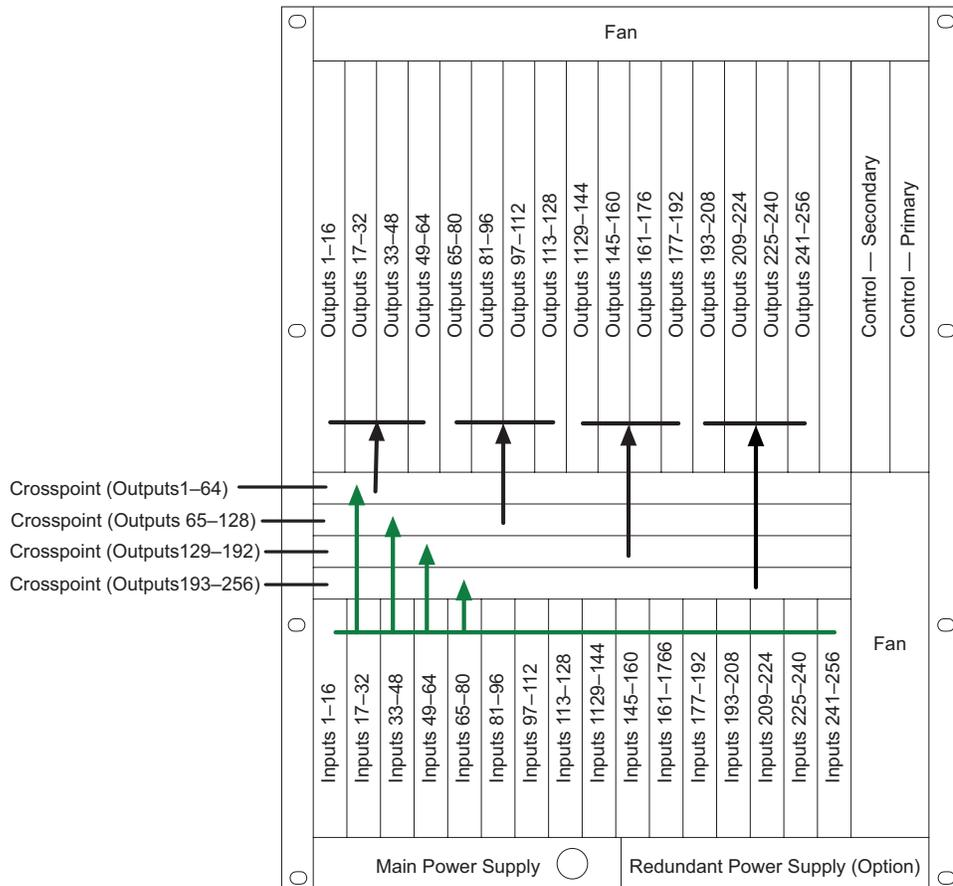
Figure 2-14. NV7256 Signal Flow (Front View)
