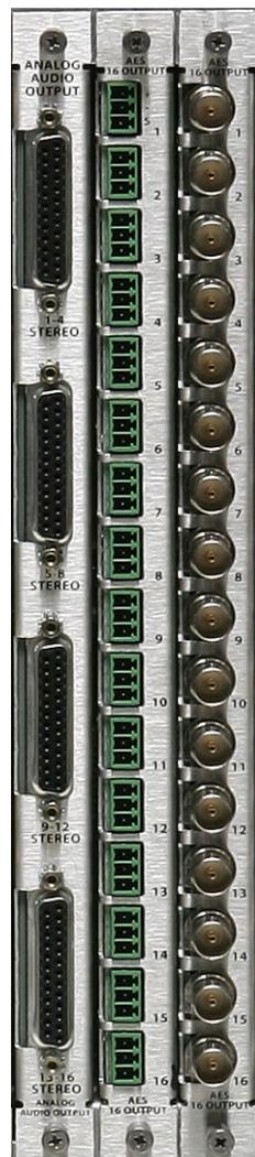
Figure 2-4. Backplanes: DB25, Phoenix and BNC Connectors
