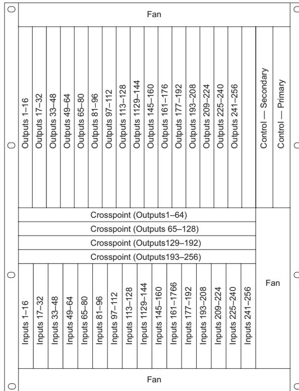
Figure 3-10. Location of Fan Trays for NV7256Plus
