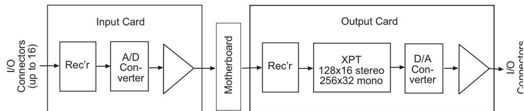
Figure 2-18. Simplified Analog Audio Signal Flow
