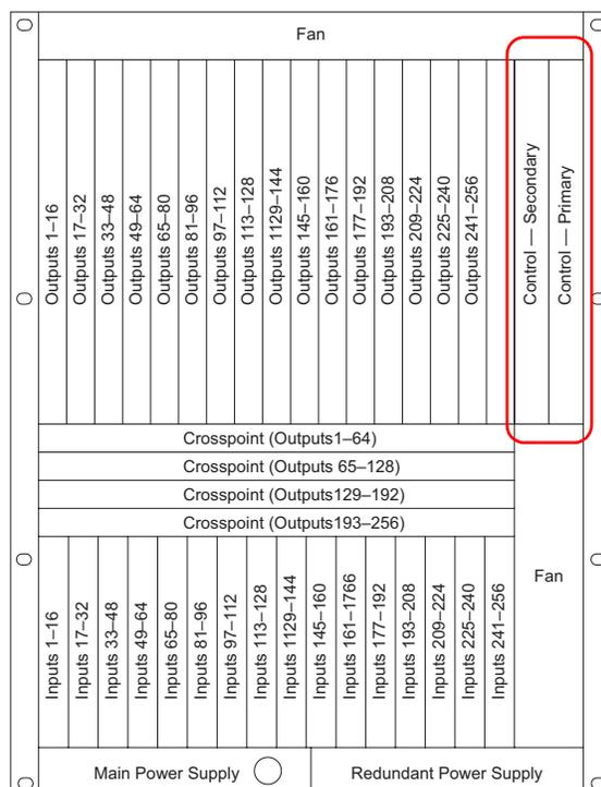
Figure 4-1. NV7256Plus Control Module Location (Front View)
