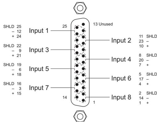
Figure 3-16. DB25 Pin Connections for Mono Signals
