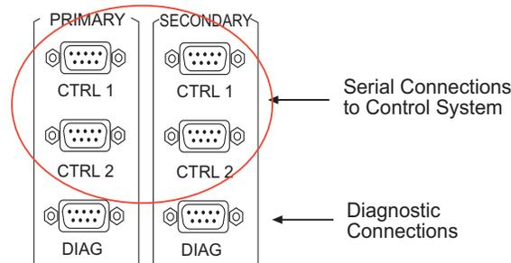
Figure 2-6. Serial Control Connections (Rear View)
