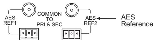
Figure 2-10. Connections to AES References (Rear View)
