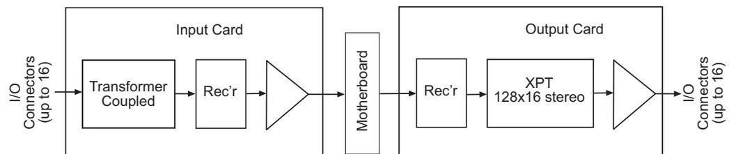
Figure 2-17. Asynchronous AES Signal Flow (Balanced or Unbalanced)
