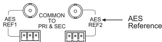
Figure 3-25. AES Reference Connections (Rear View)
