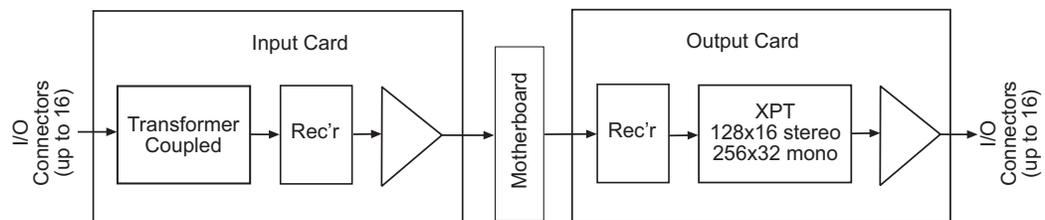
Figure 2-16. Synchronous AES Signal Flow (Balanced or Unbalanced)
