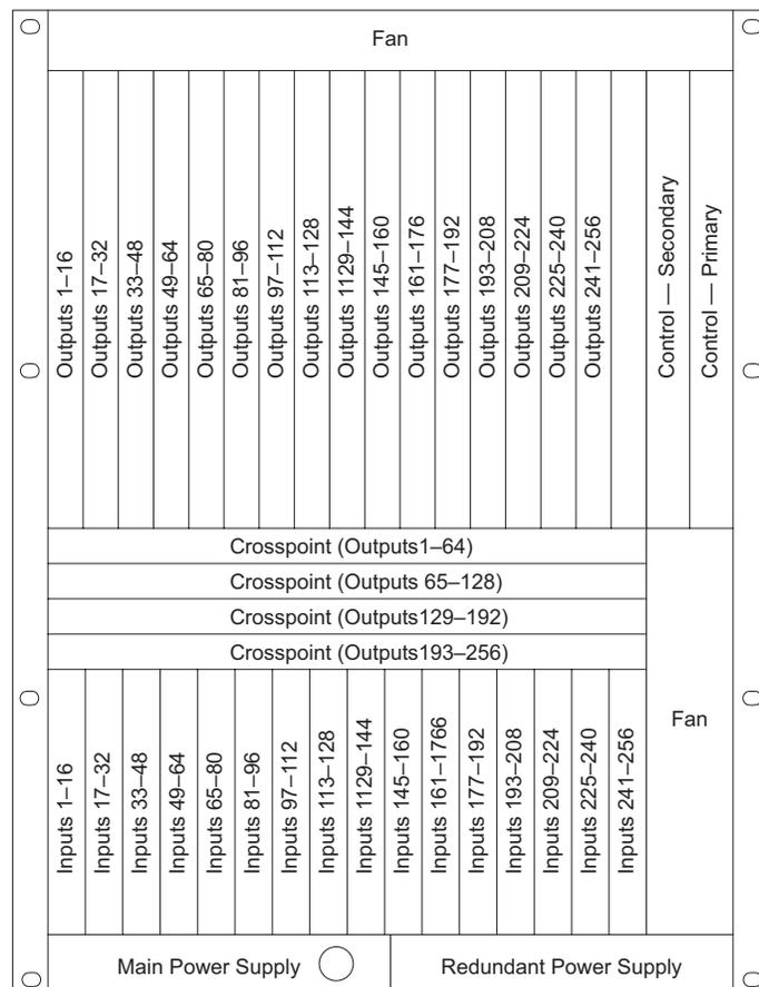
Figure 2-15. NV7256 Slots and Corresponding Signal Numbers (Front View)
