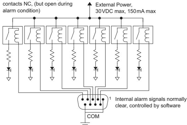
Figure 3-30. Alarm Connections and On/Off Switches
