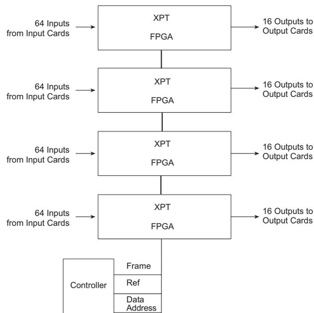
Figure 2-21. TDM Crosspoint Simplified Block Diagram
