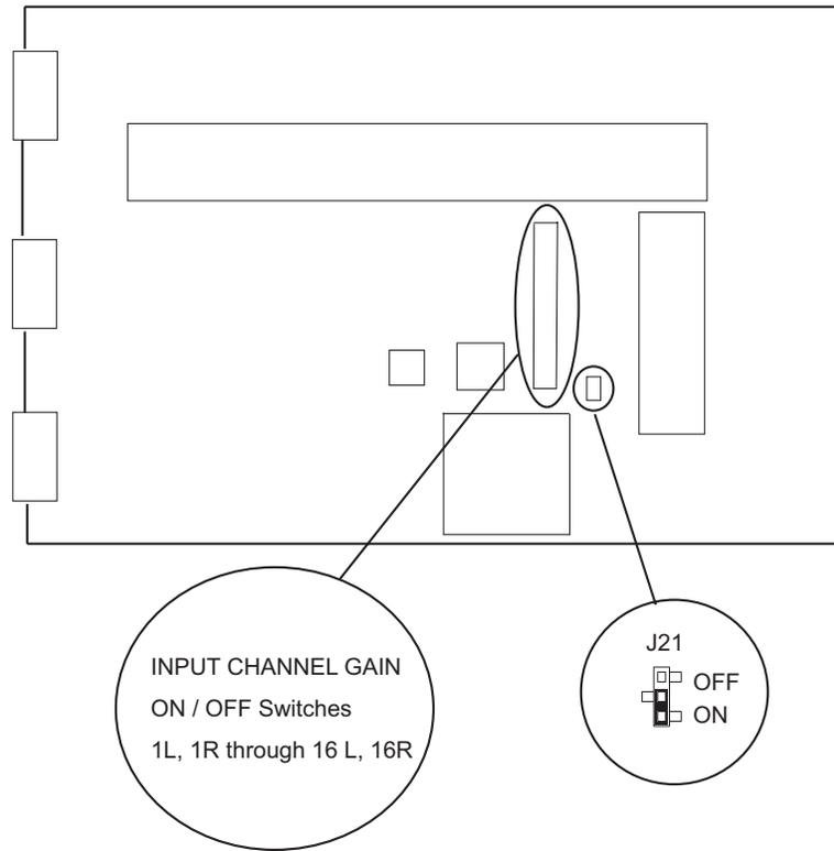
Figure 4-2. Analog Audio Input Module Switch and Jumper Locations
