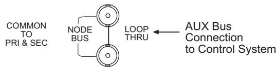
Figure 2-8. GSC Node Bus Control Connections (Rear View)
