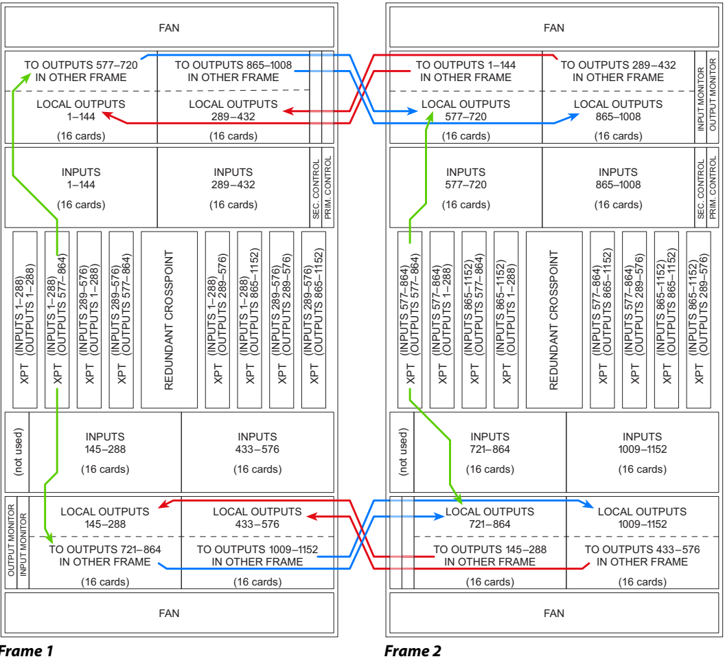
Fig. 6-5: Physical Signal Regions of the NV8576-Plus (Front View)
