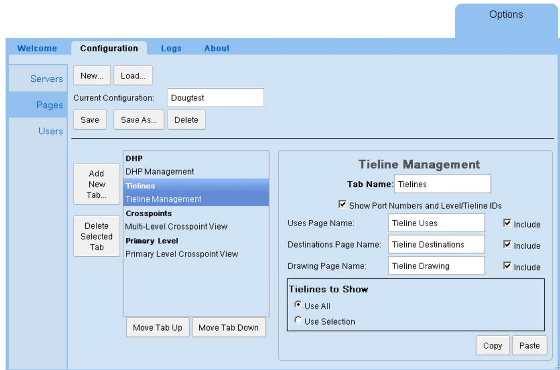
Use the check boxes to enable or disable the display of any of the three tieline subtabs.
