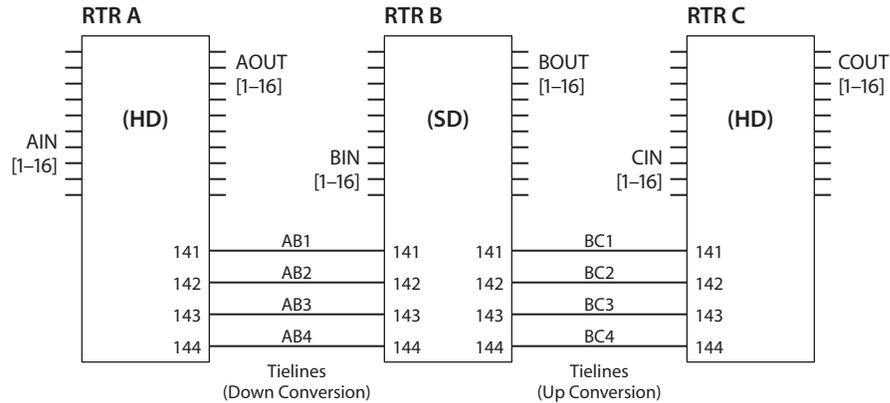
The routers are identical in size, each having 16 general inputs and outputs, except that router B routes SD, not HD. Tielines that perform up- and down-conversion are required between A and B and between B and C.
