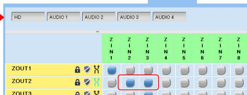
When you display only level AUDIO1, the display shows that it is from ZIN3 (for ZOUT2):
