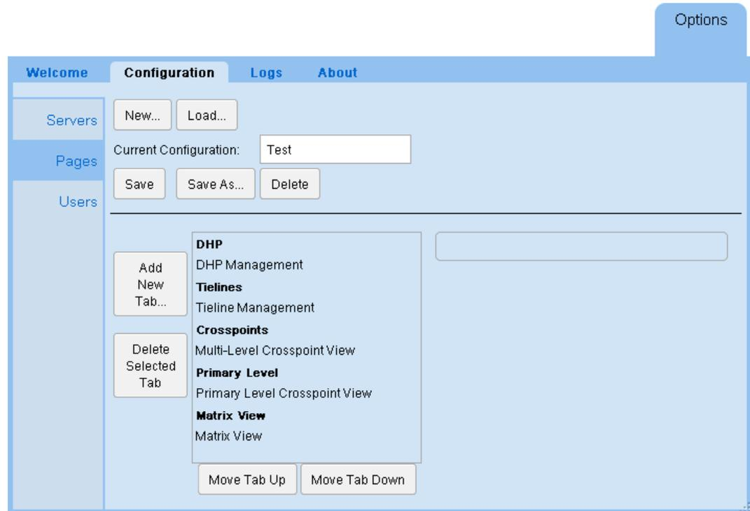
The 5 bold headings identify the 5 different page configurations in the default configuration. When you click one of the headings, the configuration options for tab that appear in the page.
