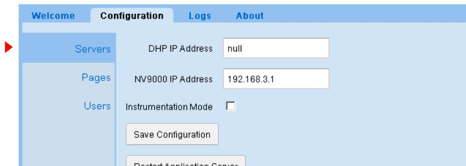
Type the IP address of the system controller or the virtual IP address of a redundant pair of system controllers in the 'NV9000 IP Address' field. (Whether your system controller is an NV960 or an NV920, its IP address goes here.)
