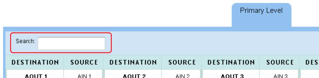
You can place text in the 'Search' field to limit the number of destination/source pairs that are displayed. Only those pairs in which the search text appears — in either the destination or the source — are displayed.
