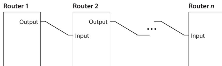
A tieline route is one taken from a source on an upstream router to a destination on a downstream router.
