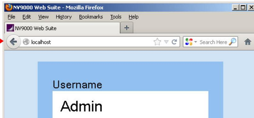
You can also type the IP address of your PC or the IP address of another PC on which the Web Suite has been installed. The term "localhost" is a synonym for the IP address of your own PC. In any case, specify the IP address of the PC on which the Web Suite is running.
