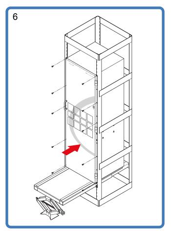
6. Attach door. Slide router into position. Attach to rack with screws.
