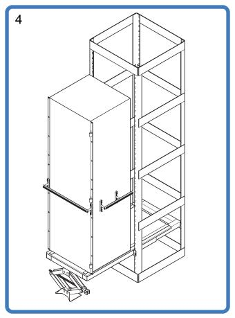
4. Load router on shelf using handles as needed.
