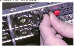
3 Pull the power supply out of the frame:
