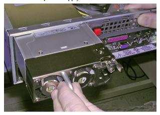
Push the power supply in until the connectors firmly lock in place.
