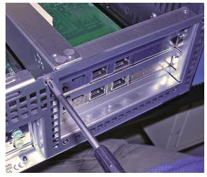
3 Loosen the T-bar (only), so that the NIC assembly bracket can slide in its track:
