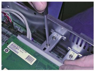
12 Insert and tighten the flathead screws for the T-bars.
