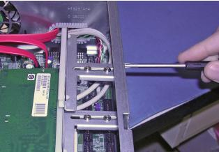
4 Then remove the 3 T-bars' hardware and brackets:
