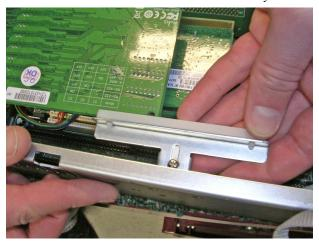
13 Insure that all T-brackets flathead screws are tightened.
