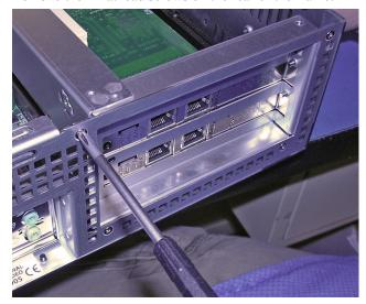
3 Remove the screw from the inside standoff as shown.
