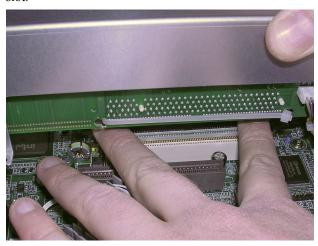
8 Insert and tighten the NIC assembly on the rear of the unit.
