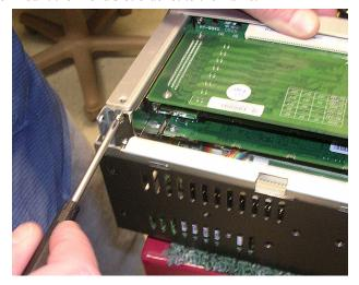
7 Ensure that the main ribbon cable is plugged into the slot
