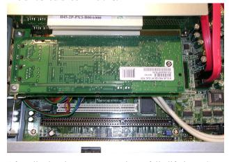
5 After all T-brackets are removed, carefully lift the NIC assembly without disengaging the main ribbon and remove the top blank slot cover. Install the new Moxa assembly card in the top slot.
