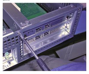
9 Re-attach the screw to the inside standoff as shown.
