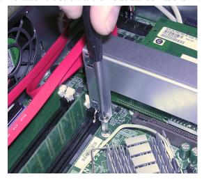
Push back the white tab on the SIMMs connector to align and tighten the screw.
