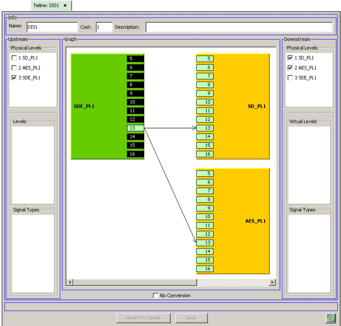
Here, the small black rectangles and light green rectangles are router ports. The black rectangles indicate that no connection is possible at that port. Connections are possible only at the ports represented by light green rectangles.
