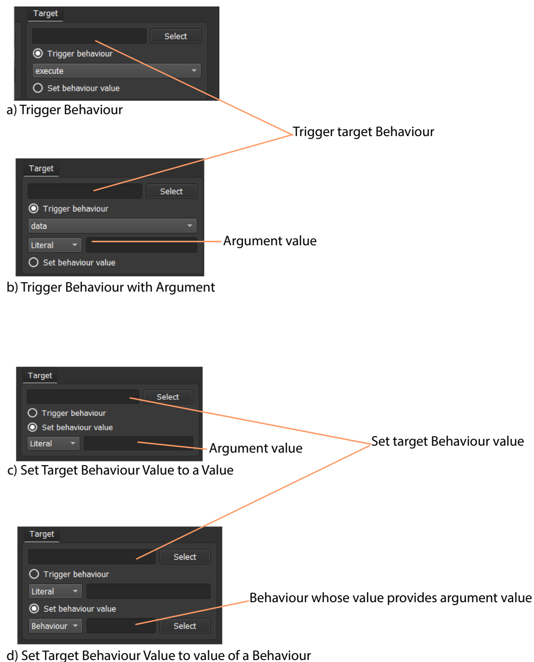
Fig. 5-5: Event Binding Settings - Target
