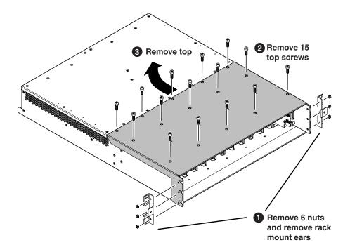
Use a #2 Phillips screw driver to remove the top screws.
