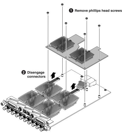
Use a #1 Phillips screwdriver to remove the screws.
