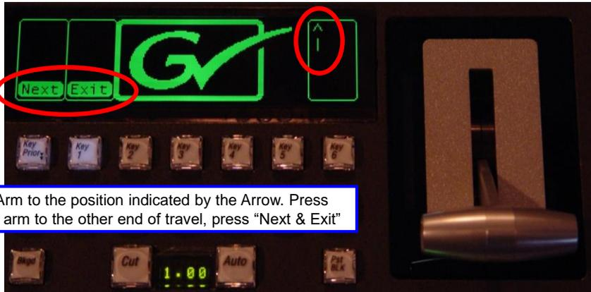
Move the Lever Arm to the position indicated by the Arrow. Press "Next". Move the arm to the other end of travel, press "Next & Exit"
