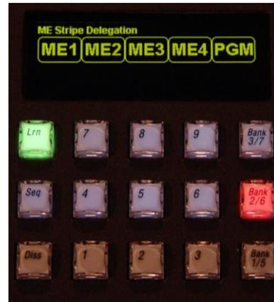
Top Rows show Low Talley representing a two Stripe (2 M/E) Panel. The 3<sup>rd</sup> row of buttons would be illuminated also for a 3 M/E Panel.
