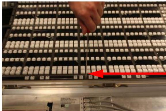
2. The right System Bar will disengage from its socket as it is unscrewed. Once it is completely unthreaded it can be lifted out of the tray. You may need to tilt it to a flat, horizontal position to allow clearance for removal.
