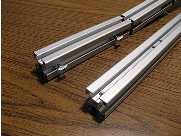
10. Attach the top plastic end cap and rear round ended reinforcing bracket. Tie wraps are not used on the middle support beam.
