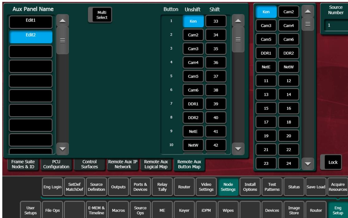
The Remote Aux Button Map Menu is used to configure sources to the Remote Aux Panel source select buttons.
