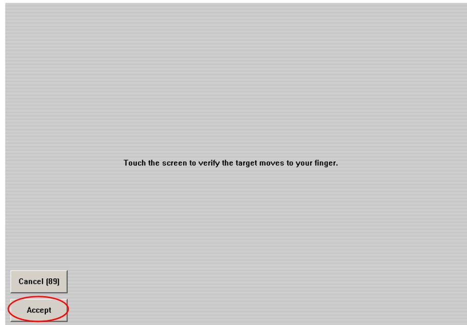
9. Touch the screen to verify the calibration. A calibration circle will appear and follow your finger touch across the screen. If satisfied, touch the **Accept** button at the bottom of the screen to save the calibration.
