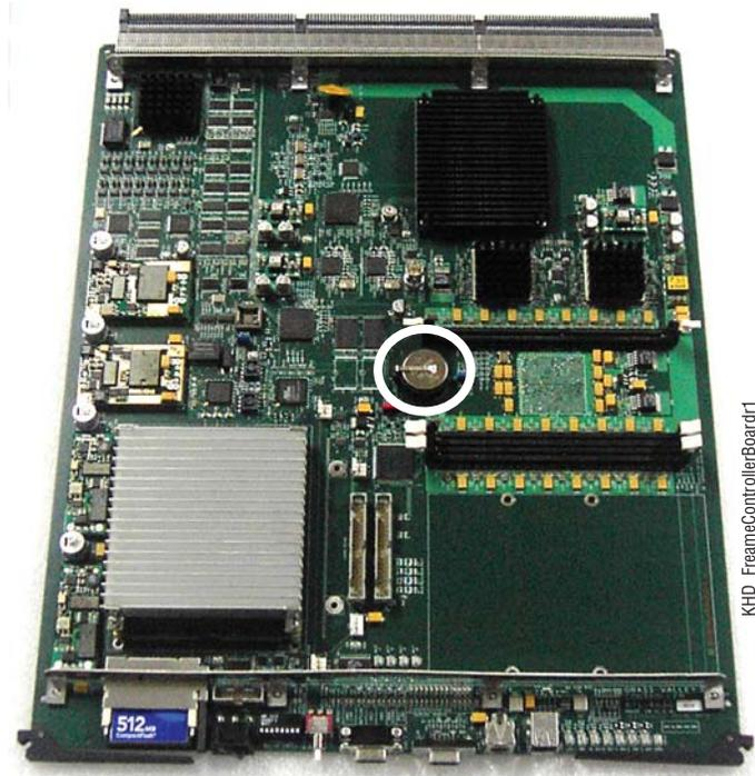
Figure 212. Video Processor Frame Controller Board Battery
