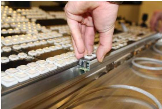
2. On larger Control Panels, connect the flat ribbon cable to the Extended System Bar, align it horizontally and screw it into place as above.
