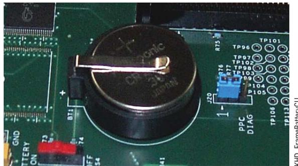
3. Remove the old battery by lifting the clip holding it in place.
