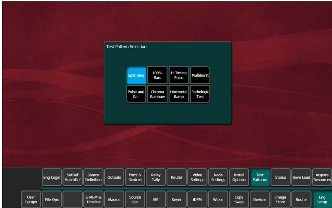
The Test Patterns menu allows the selection of different video test patterns. The chosen test pattern will be displayed when the Test source is selected.
