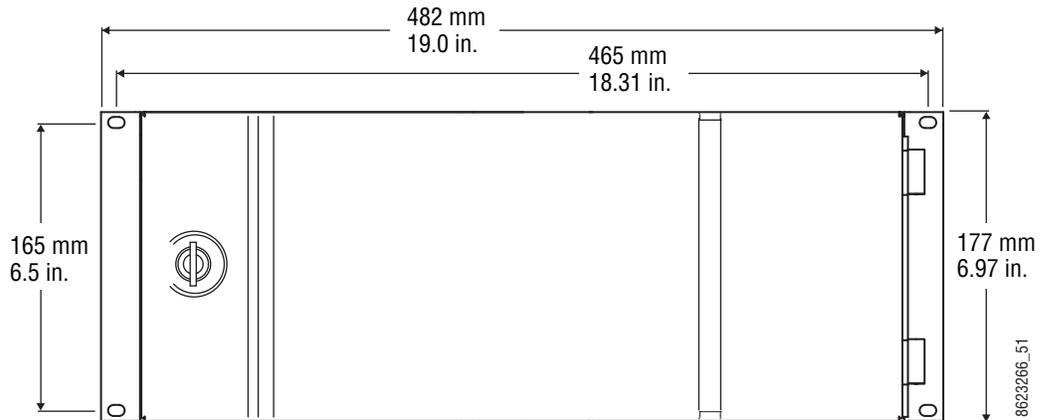
The top view dimensions of the Kayenne 4-RU Frame are the same as the 8-RU Frame, except there are only two AC line cord retainers (see [Figure 70](#) on page 99).
