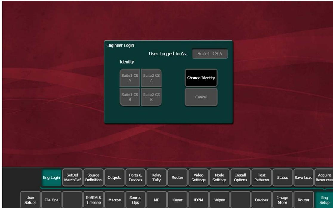
A Kayenne system can be configured as two suites, with each suite having up to two control surfaces. The Eng Login menu is used to choose which suite and control surface the Kayenne Menu will interact with and control.
