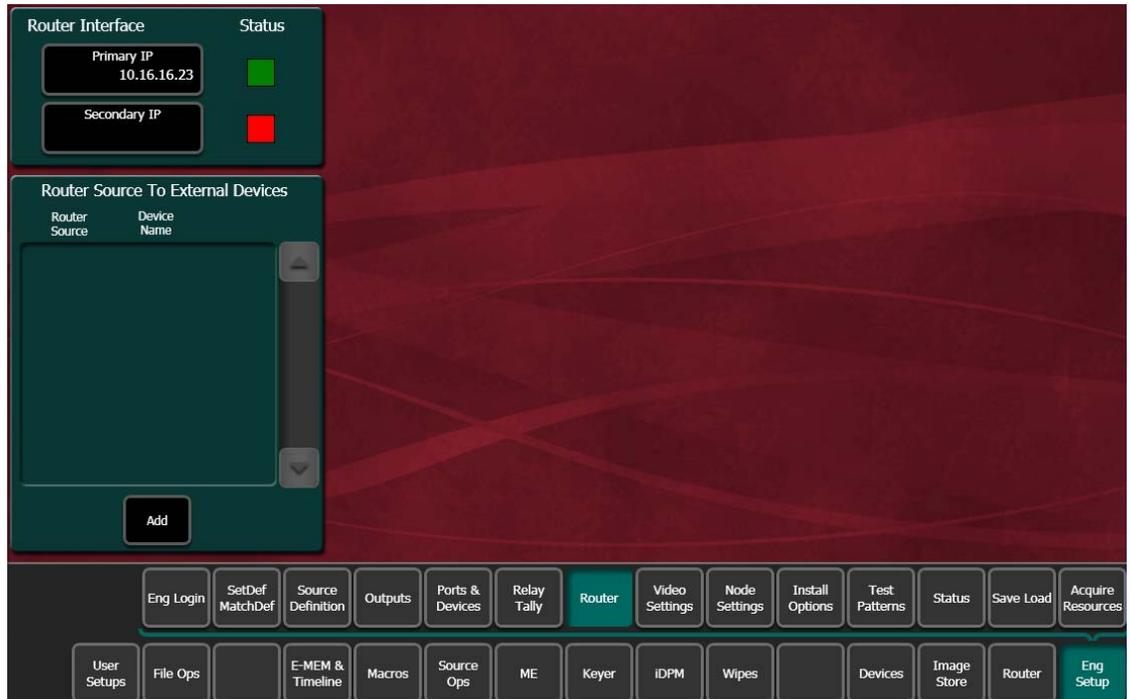
The Router Menu is used to establish communications with a facility video router, and to map router sources to external devices.
