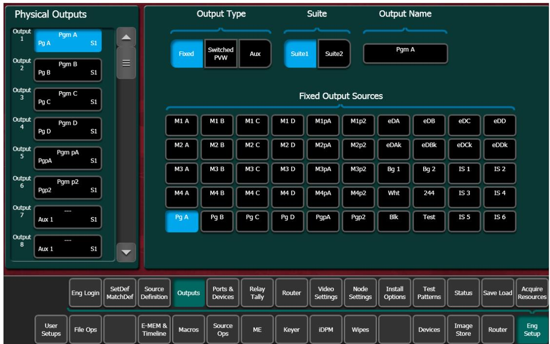
The Outputs menu is used to change the Kayenne system output assignments. See *Output Assignments* on [page 161](#) for detailed information.
