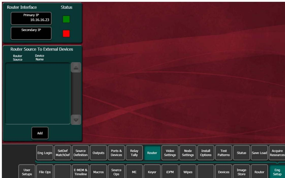
The **Status** indicator is red when communication is not detected, and goes green when communication is established.
