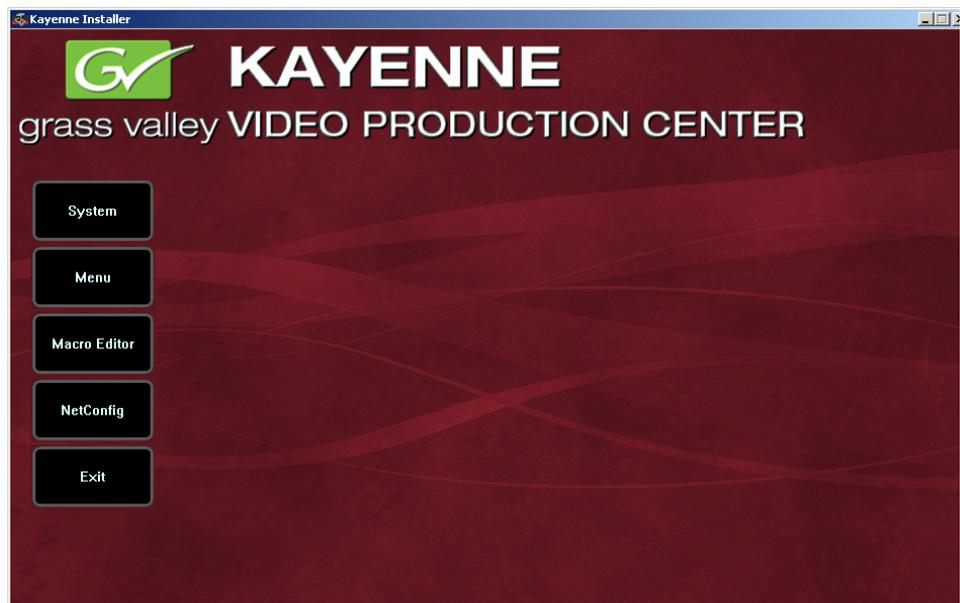
3. Click on the **System** button on the left to open a hierarchy display of Kayenne systems. Each Kayenne system consists of a Video Processor Frame and associated Control Panel(s). Use the mouse to navigate to the desired component (Figure 103).
