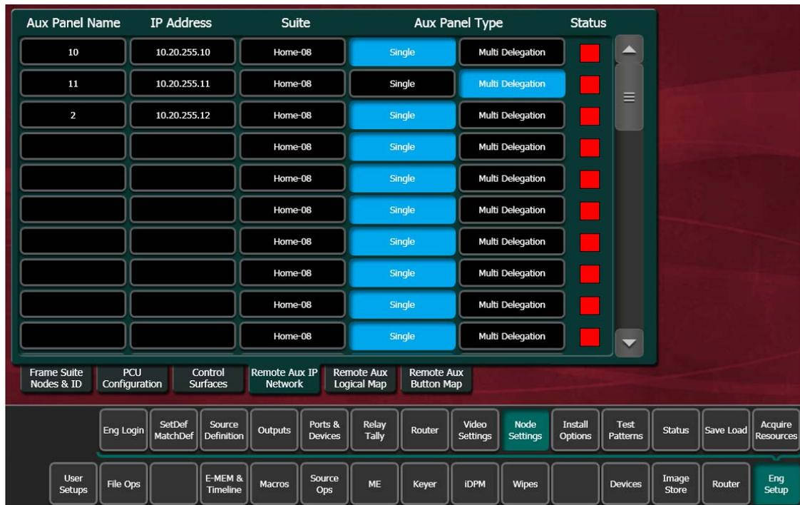
The Remote Aux IP Network Menu is used to register Remote Aux Panels for communication with the Kayenne Video Processor Frame, and identify their type and suite assignment. See *Remote Aux Panel Registration on page 154* for more information).
