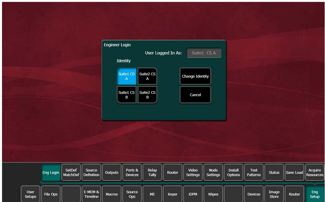
2. Touch **Eng Setup, Acquire Resources**, select **Yes** to the warning message, and release resources not needed in suite 1 that you wish to make available to suite 2. This can be done individually using the scrolling list on the left (Figure 142) for each type of resource. Alternatively, you can use the category tabs on the right to release all the resources in each category, and then reacquire only what is needed by suite 1.
