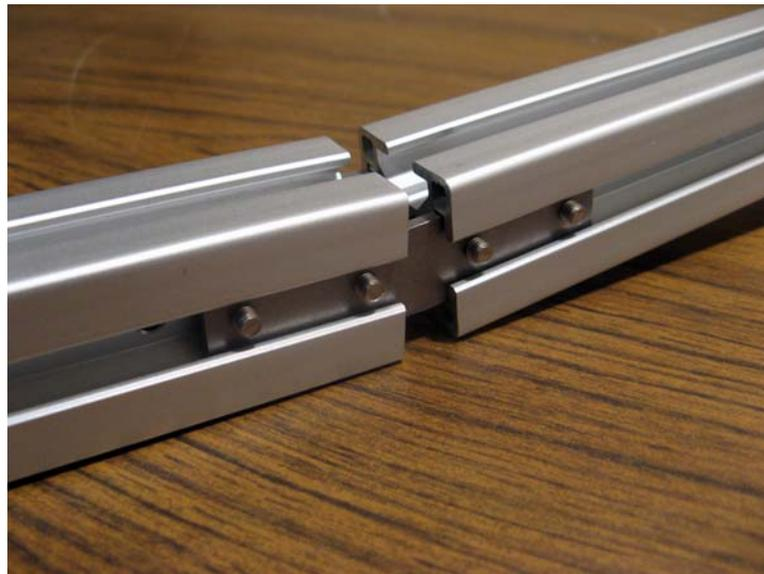
9. Connect the long middle curved support beam to a shorter straight beam. This is a mirror image of the left support beam. The middle straight beam is attached the RIGHT side of the middle curved support beam (Figure 24).
