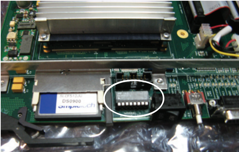
Figure 235. Kayenne Control Processor Board - S2 Boot Mode Dipswitch Location
