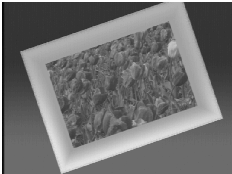
Figure 27. Incorrect Key With White Halo
