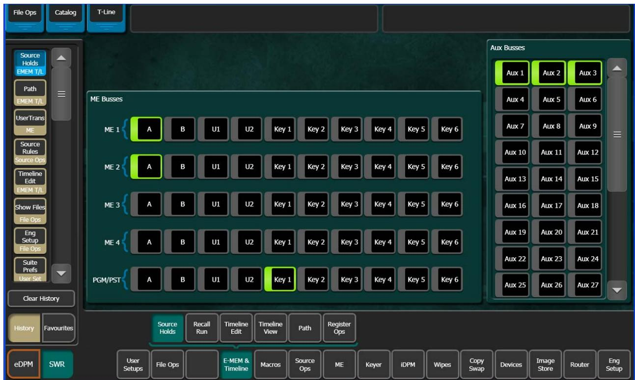
3. Press **LRN** on the Kayenne Control Panel (Master or Local E-MEM Module), then press a bank and register number to create a new effect with a Source Hold in its one keyframe.
