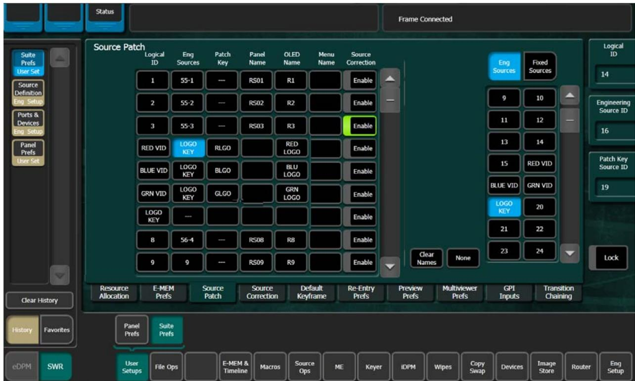
2. Touch the data entry pad in the Patch Key column for the Logical ID you wish to patch a key from a different source.
