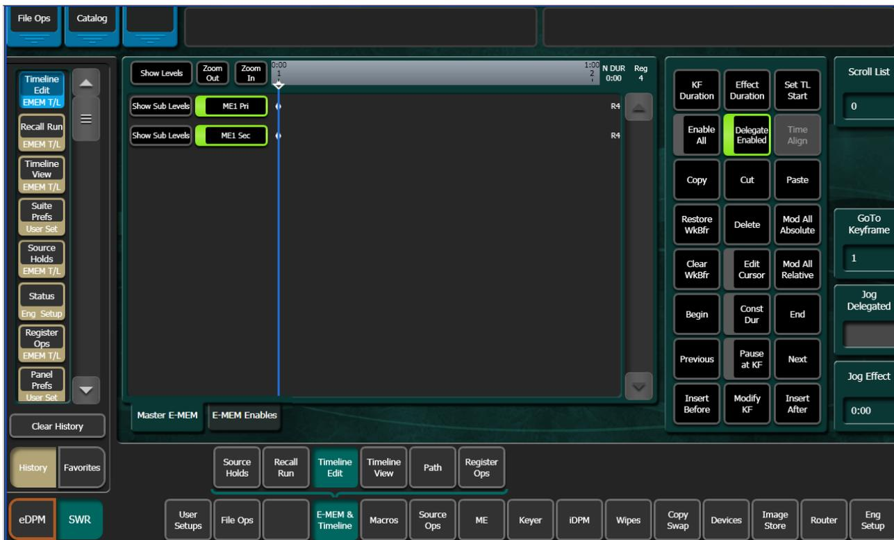
3. Touch the Enable button of any sub-level to disable that sub-level from being included in the current E-MEM register.
