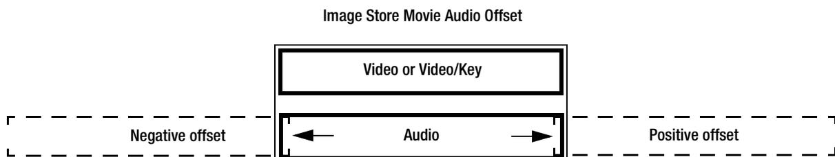
3. Enter the offset value in the Offset data pad (a negative (-) value means the audio is set to begin before the video):
