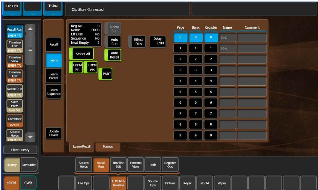
In the Control Panel, the eDPM Primary and Secondary partitions are available via the **eDPM Pri**/**eDPM Sec** buttons in the Master E-MEM area.
