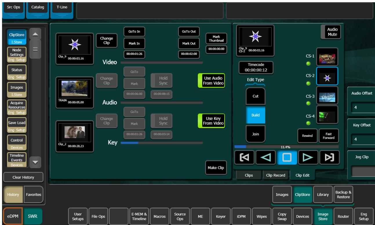
The clip created with the Make Clip operation will be a sub-clip that has its head to tail length defined by the mark-in and mark-out points of the Video track (if there are no marks, the sub-clip created will be the same length as the original). Both Audio and Key tracks of the new clip will only exist between the Video track's marks.
