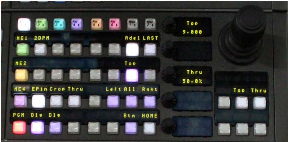
8. Press the **All**, **Top**, **Right**, **Left**, or **Bottom** button and use the soft knobs to pin the edges to the cropped box; this allows very precise edge adjustment.
