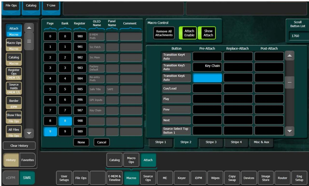
2. Select the button you wish to attach a macro to. You can either touch the physical panel button while **Show Attach** mode is active, which will scroll to and blink that button on the Macros Attach menu, or you can use the menu to select the panel section and then scroll the Macro Attachments list to display the desired button.
