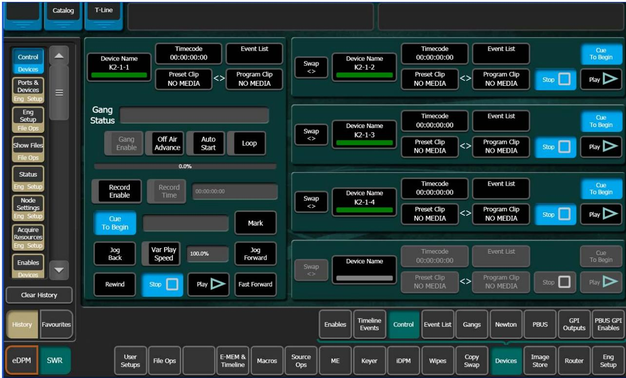
Standard **Cue To Begin**, **Stop** and **Play** controls are available for all devices configured for control. The **Swap** buttons transfer the control of devices between panes.
