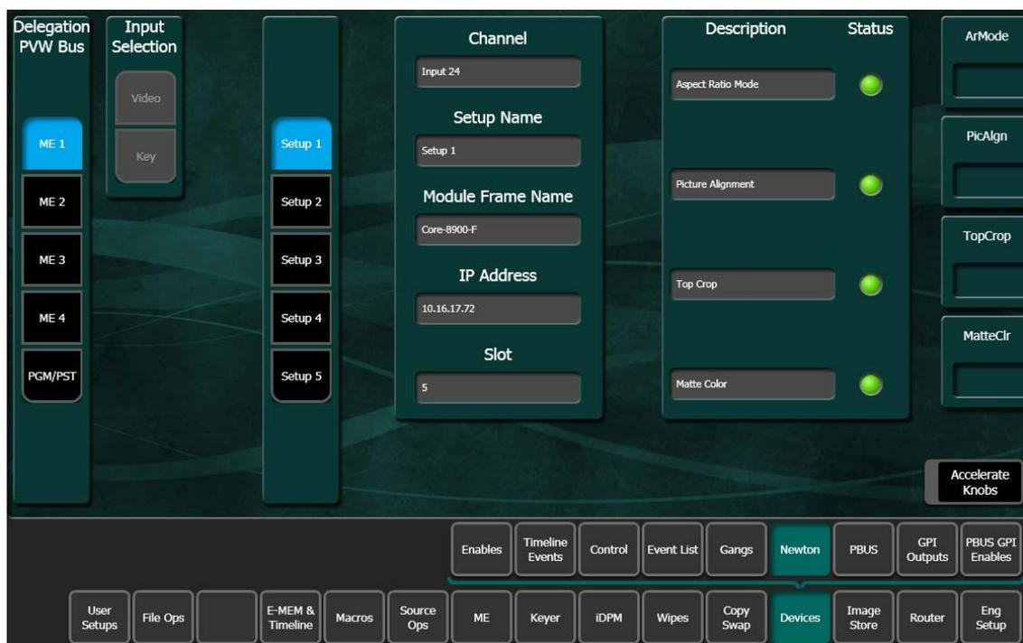
Selection of a module parameter to control is mediated through the GV Switcher source selection mechanism. By selecting a source on the currently delegated Preview bus of the GV Switcher's Control Panel, the source's physical input, and that input's associated Newton channel controls are activated on the GV Switcher's Device menu.
