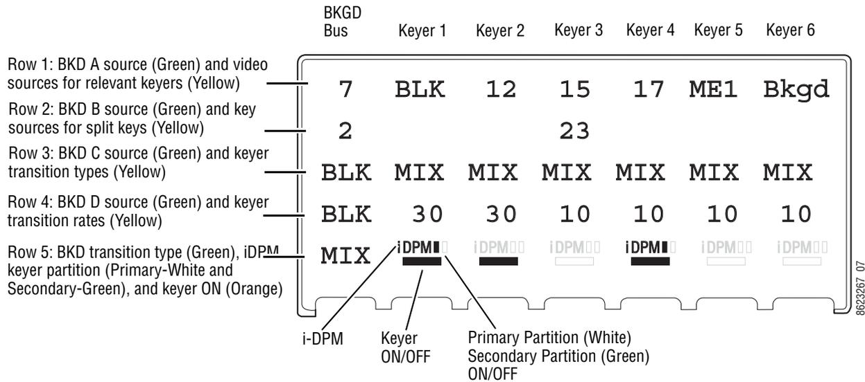
Additionally, when the **Key Prior** button (Keyer Priority) is pressed on the Transition Module, Row 4 changes from displaying transition rates to Keyer Priority for Keyers 1, 2, 3, etc. and shows the differences between the current and next priority stacks.
