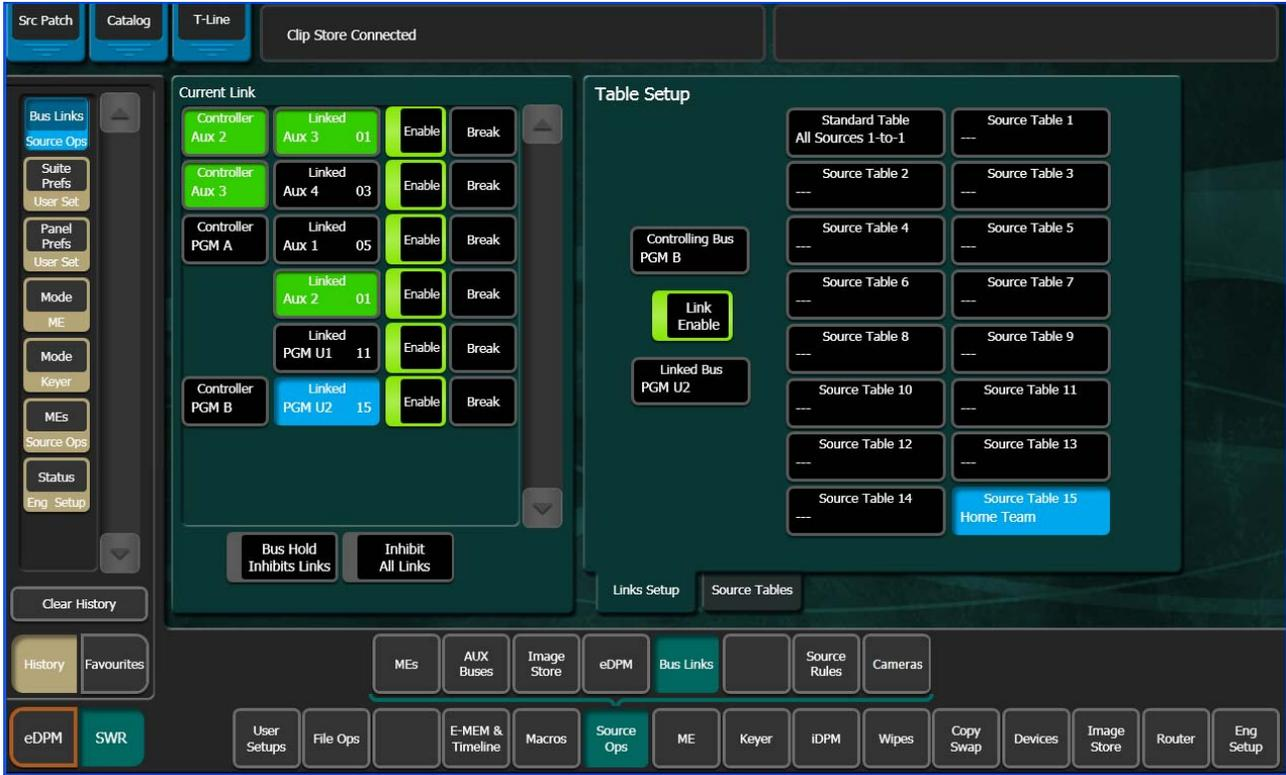
Selected **Controller** bus and **Linked** bus buttons turn blue when selected in the Current Link pane. In the example in [Figure 76](#), the Linked bus button **PGM U2** is the selected button.
