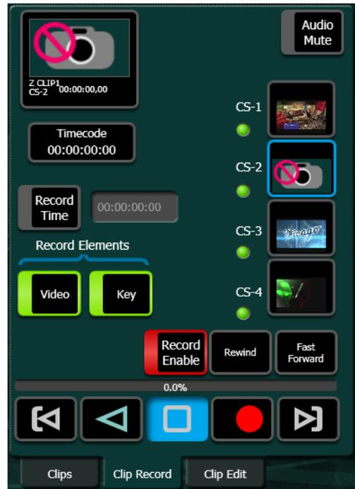
When the **Record Enable** button is touched, ClipStore ejects the clip from the selected channel, places the ClipStore channels in E/E mode, and displays a pop-up keyboard. Type in the name of the new clip. Once the name is typed, **Enter** is pressed, and the keyboard closes, the **Record Enable** button is highlighted red and the menu has changed to display recording controls and parameters in readiness for recording. The **Play** device control button is replaced by a **Record** button.
