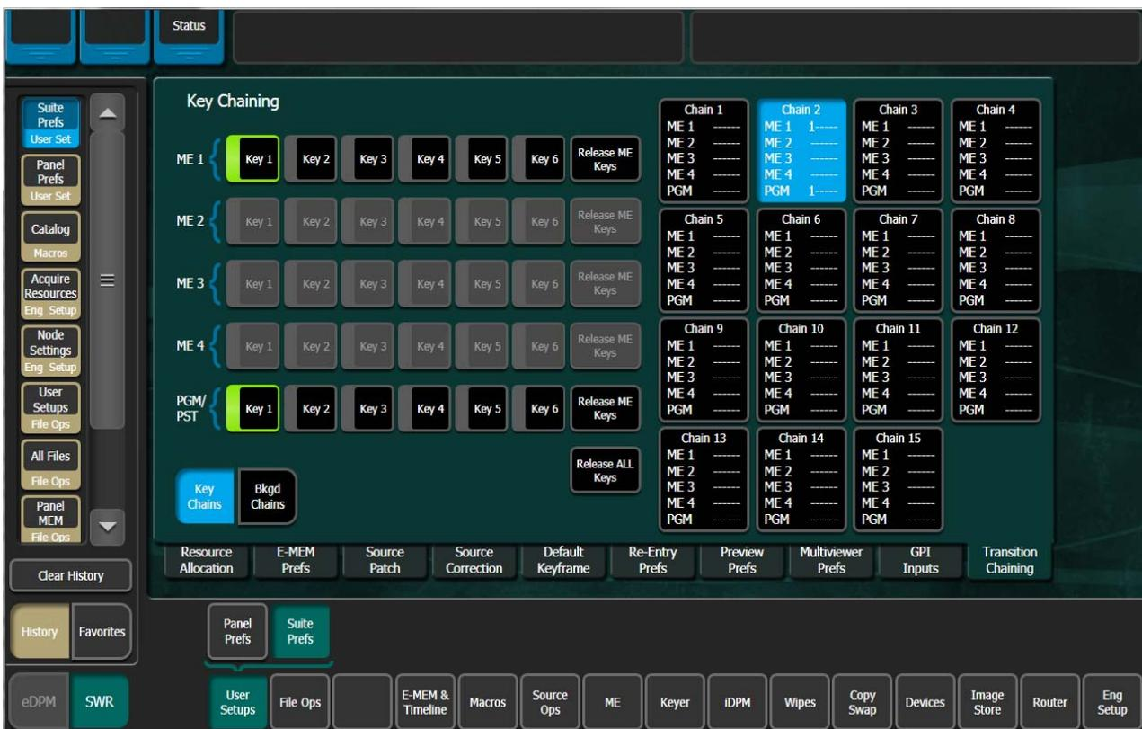
Selecting a keyer in the Next-Transition section of the Control Panel will make that keyer the initiator. On the MEs with keyers in the chain, their next-transition selections will be erased and the keyers in the chain selected. These keyers will flash to indicate that they are in the chain. The key which is not flashing is the initiator.
