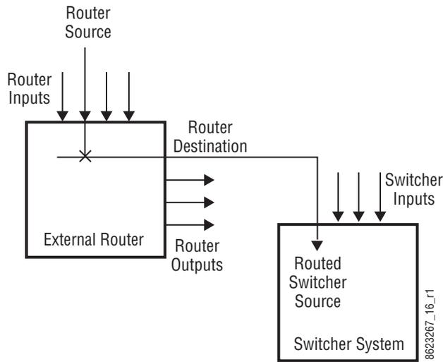
Router signal switching is non-deterministic, as compared to source selections performed on a production switcher. For this reason, it is better to choose the desired router source in advance, then switch it on-air using switcher controls, rather than select a different router source while it is on-air.
