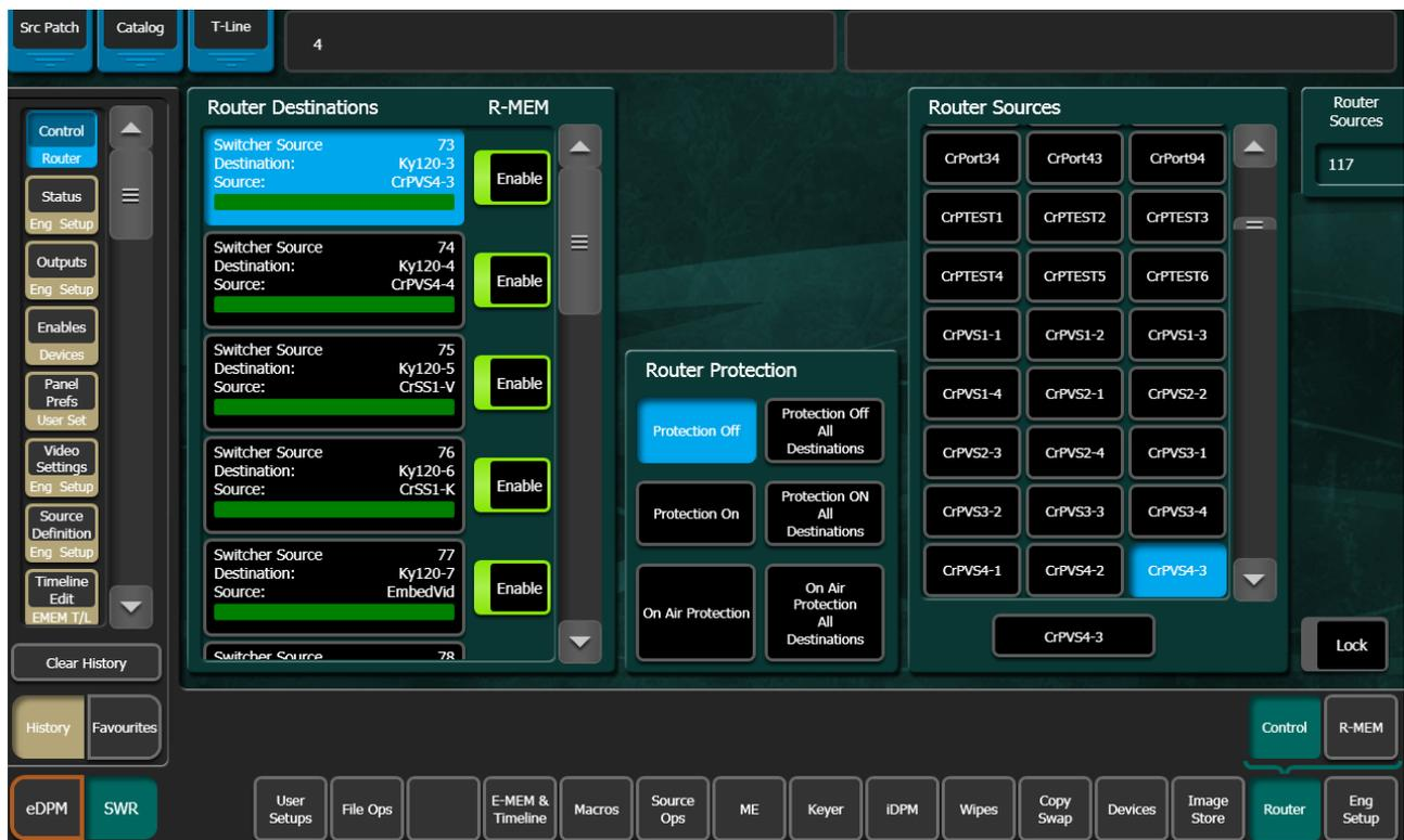
The Router Destination pane on the left is a scrolling list of switcher sources (only sources configured as routed GV Switcher sources appear). Each button displays the Switcher Source ID number, Destination, and Source. The currently selected switcher source on the list is colored light blue.
