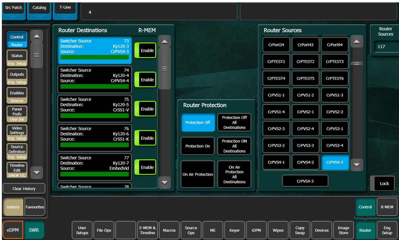
3. Press the **LRN** button in the Control Panel Master E-MEM Module, then press the Page, Bank, and Register keypad number of the desired register. This will save the current R-MEM setting in the menu to the header area of that E-MEM effect register and the first keyframe of the new effect will be created. The corresponding R-MEM register in the menu will also be updated.
