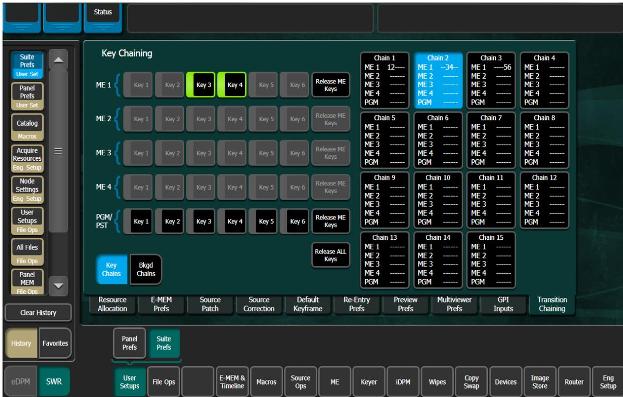
Result: Once a keyer is enabled as part of a chain, the button is grayed out as each key can only be part of one chain.
