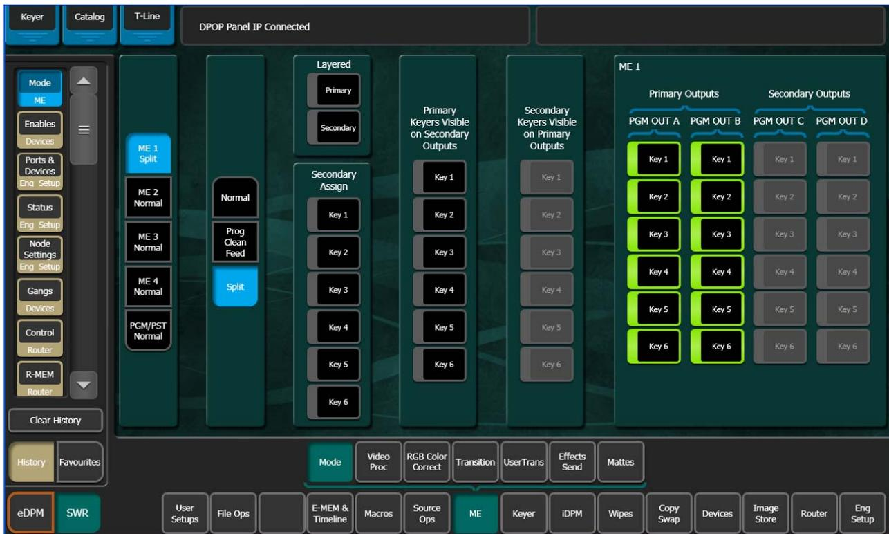
In **Split** operating mode, the ME is divided into Primary and Secondary partitions. The Primary partition has the Pgm A and Pgm B outputs that use the Background A and B buses, and the Secondary output has the Pgm C and D outputs that use the Utility buses. The Pgm Out columns on the menu are re-arranged when Split mode is selected to show the A and B Primary outputs on the left and the C and D Secondary outputs on the right.
