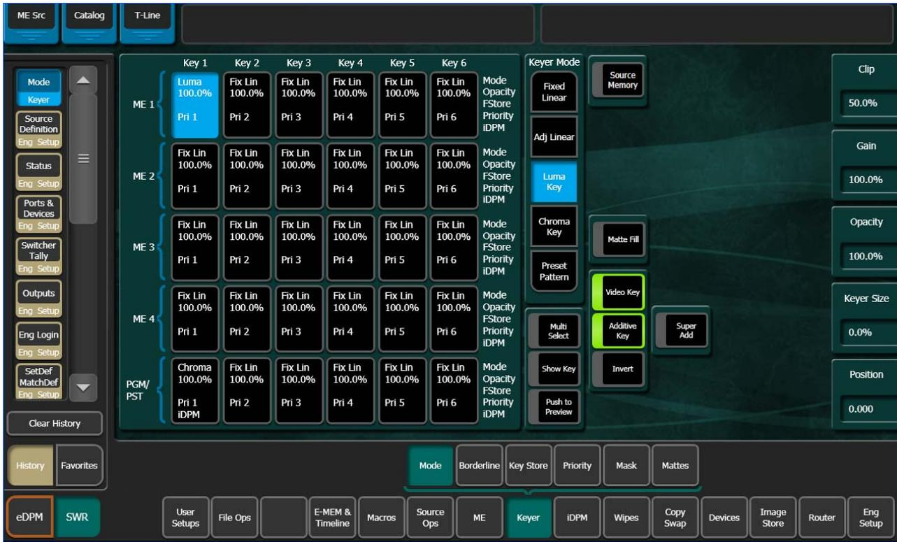
**Note** Selecting or re-selecting any Keyer Mode button (**Fixed Linear**, **Adj Linear**, or **Luma Key**) will reset the shape type to “Auto”, i.e. as defined in the Source Definition menu.
