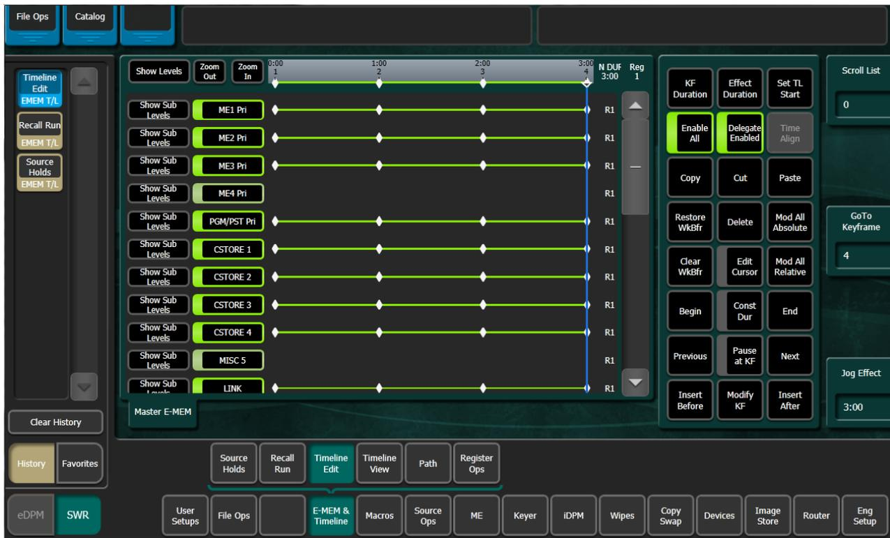
3. Touch the **Effect Duration** button to open a keypad (located in pane, just right of the Timeline view). Type a new duration in Seconds • Frames • Fields format and touch **Enter**.
