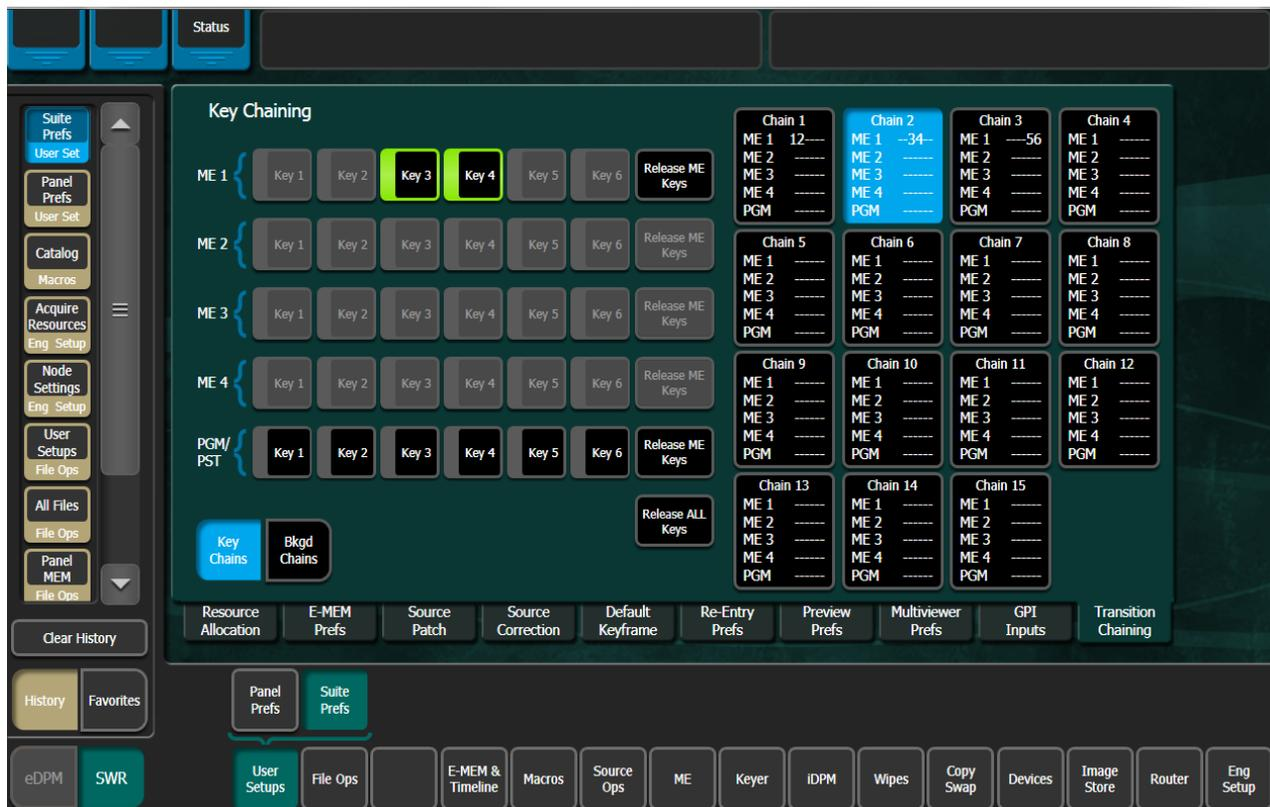
Selecting keyers in the Next-Transition section of the Control Panel will make those keyers initiators for the transition. Key Chaining causes the chained (controlled) keyers to be selected as well. These chained keyers will flash to indicate they are in the chain. The keys which do not flash are the initiators. When the Lever Arm is moved, or the **Auto** button is pressed, the keys transition together.
