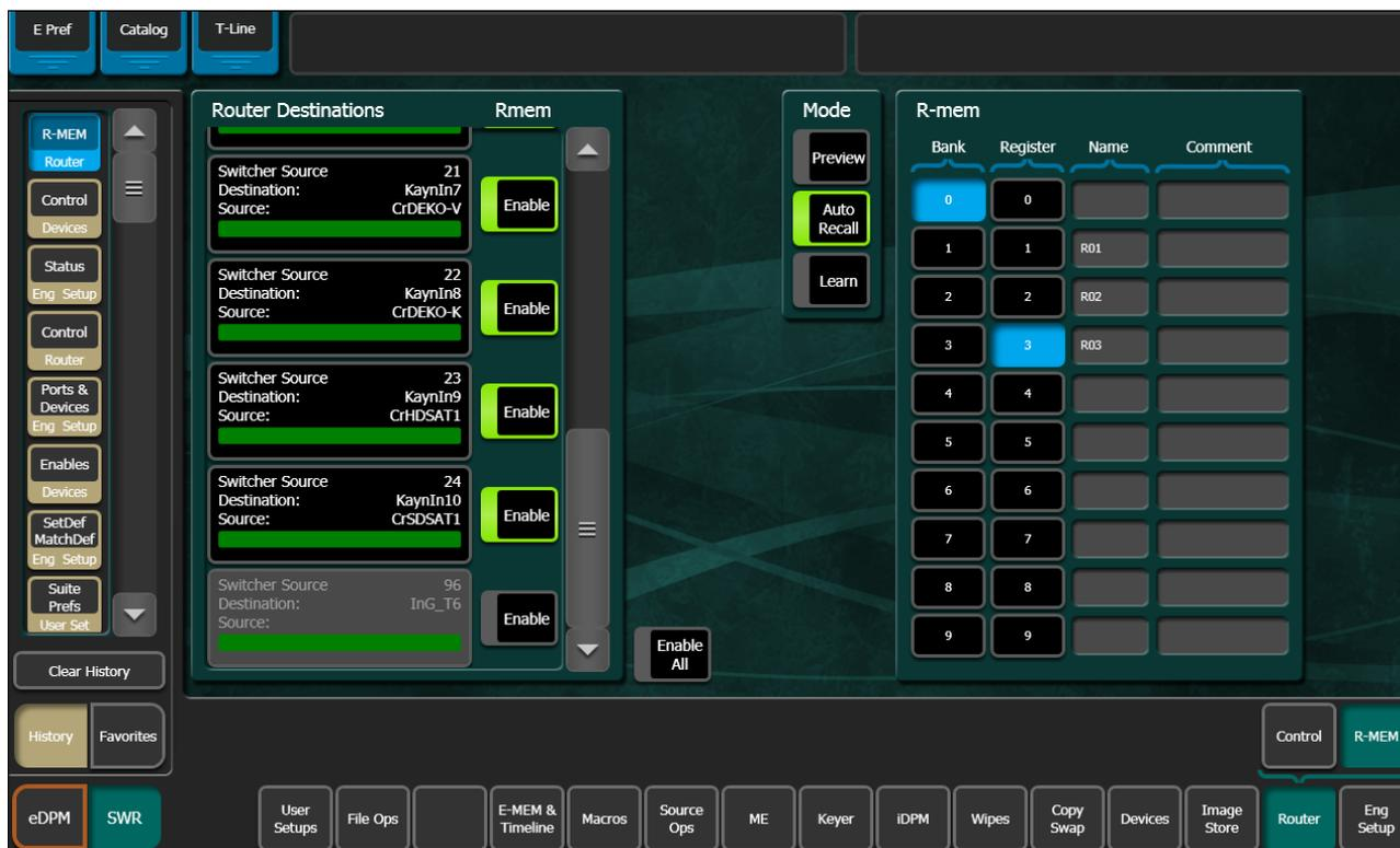
The R-MEM menu has a Router Destinations pane on the left showing the switcher sources, router sources and destinations, and protection status. Switcher sources configured as routed sources also appear in the left pane. There is a Mode pane in the center and an R-MEM pane on the right listing the R-MEM registers available (the full register number is displayed on each register button).
