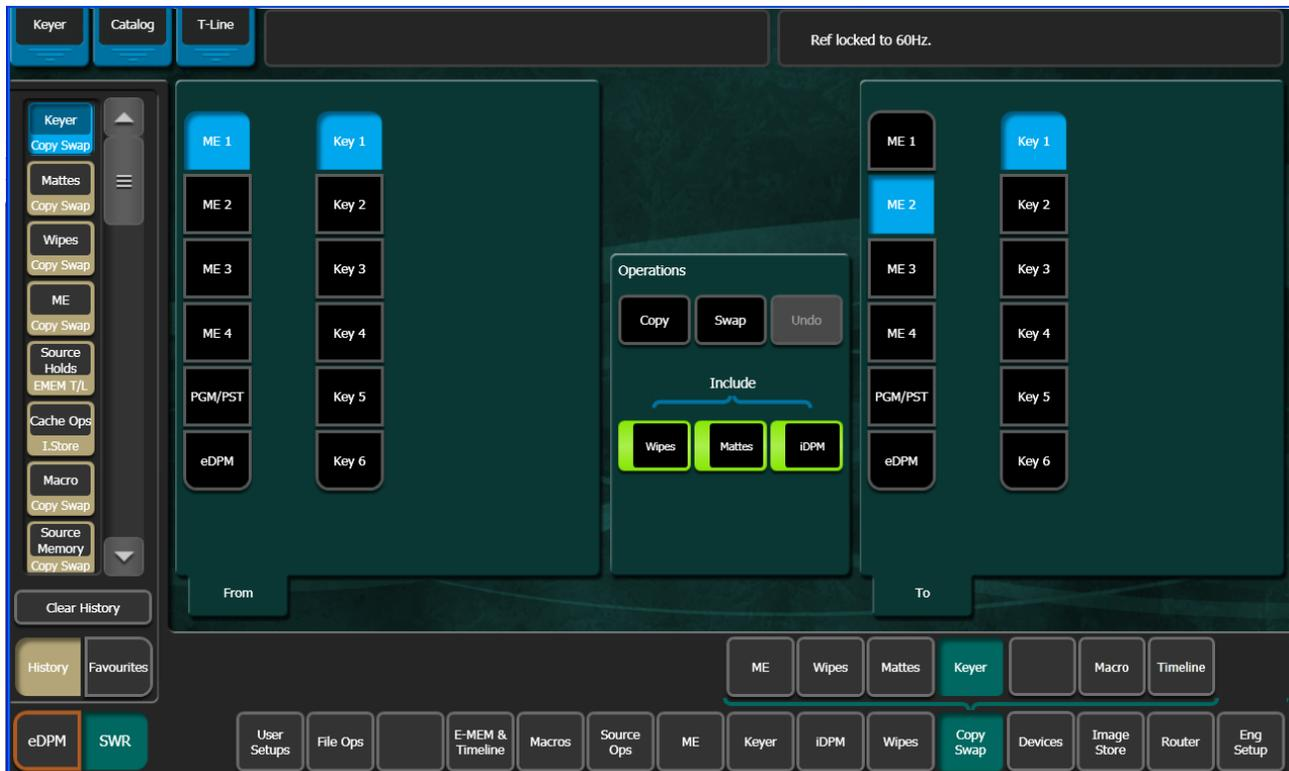
The menu enables the copying and swapping of entire keyers, including the mapping of key cutter and key fill sources. It is a direct copy of what is currently in the chosen From keyer, including key type, key split condition, and all parameters describing the key's behavior.
