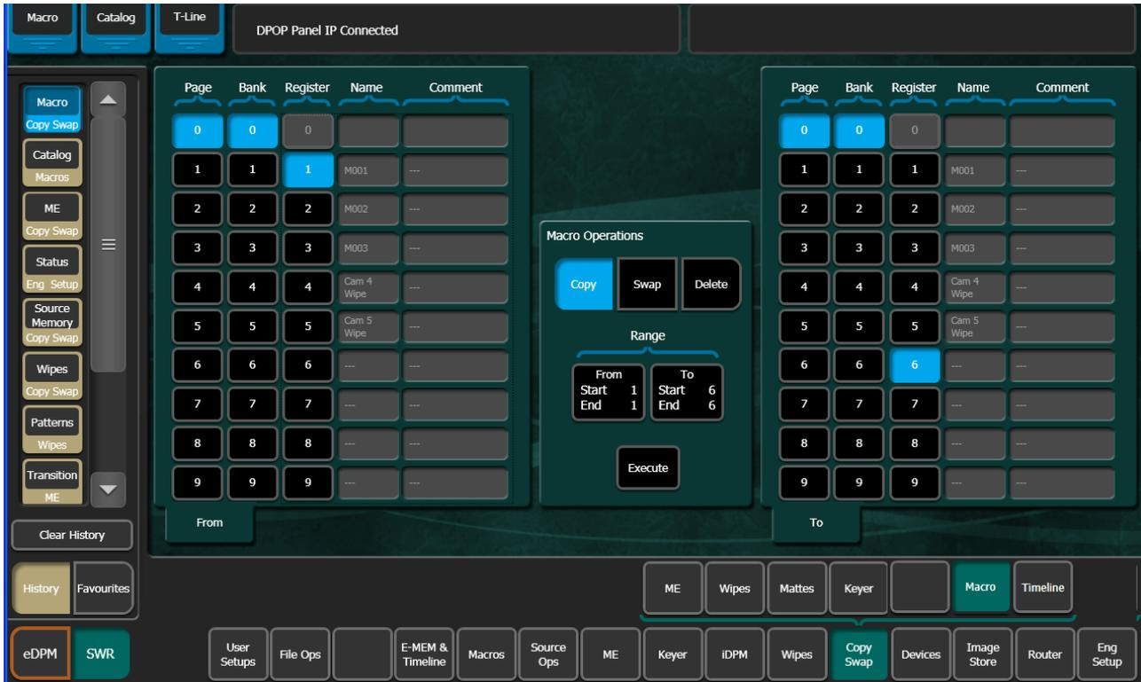
Macro register information can be moved from one register to another with this menu by selecting the registers in the From and To scrolling panes, then touching the **Copy** or **Swap** buttons in the Macro Operations pane. The soft knobs and data pads on the upper right can be used to quickly select specific register numbers in each pane.
