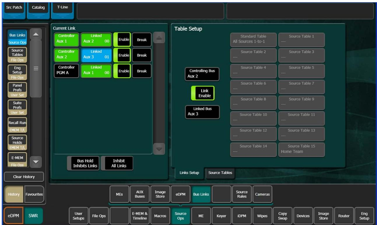
1. Touch the **Controlling Bus** data pad in the Table Setup pane; the Controlling Bus selection menu is displayed.
