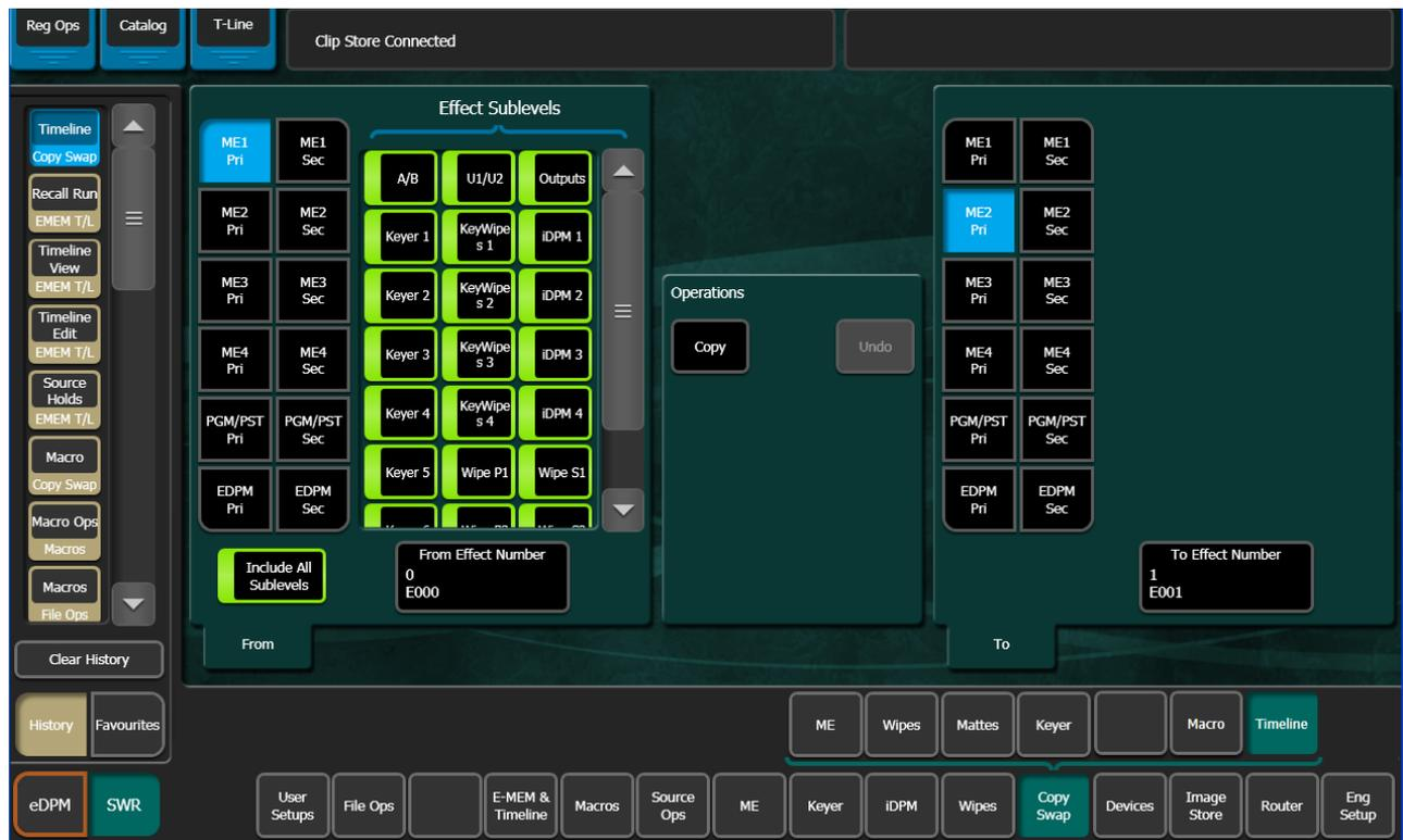
Complete E-MEM timelines containing multiple keyframes can be copied from one ME to another ME or the eDPM and vice versa. All sub-level information can be included using the **Include All Sublevels** button or with this button off, sub-levels can be excluded from being copied by touching the sub-level's enable button.
