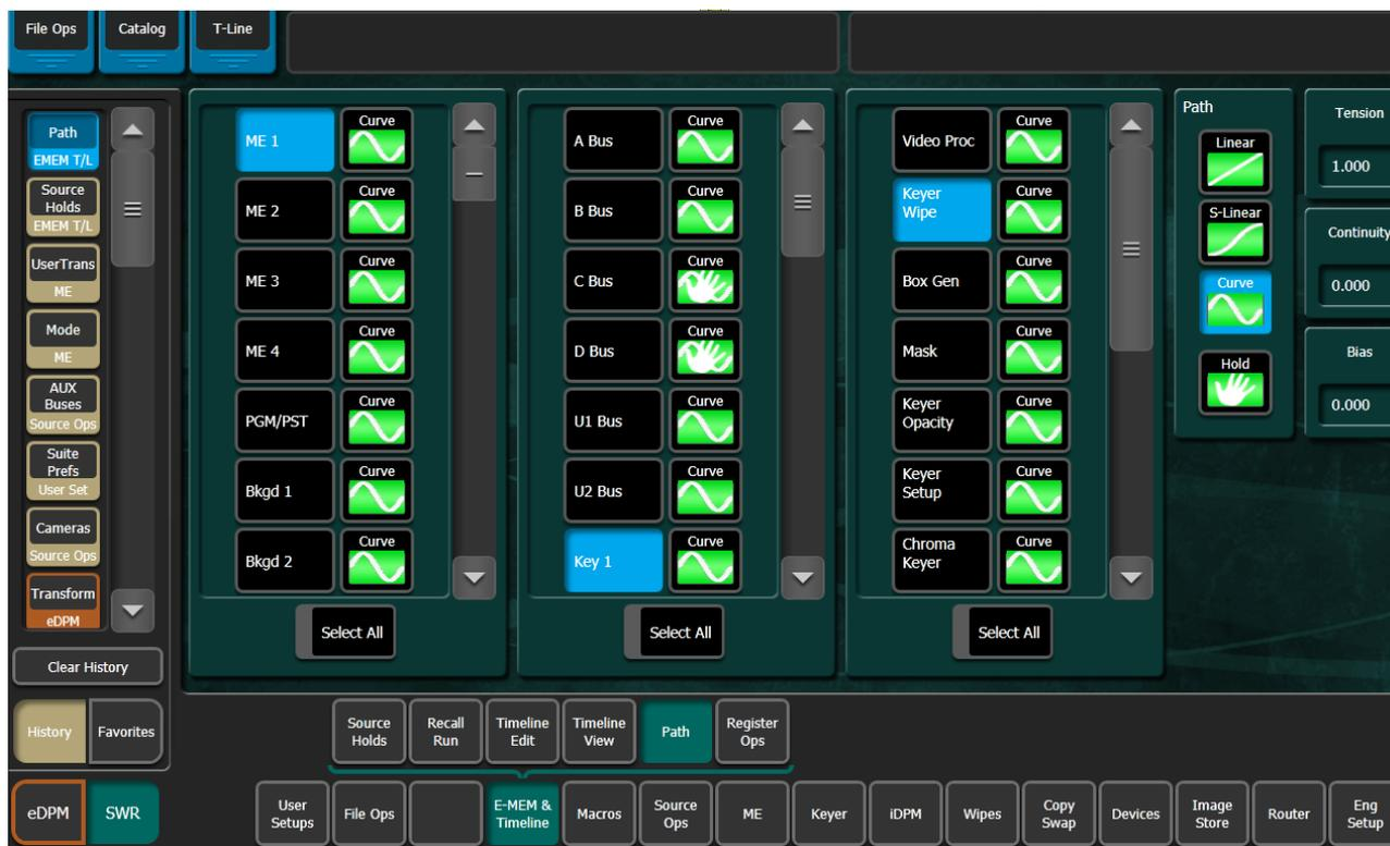
3. Choose the desired Path type (**S-Linear, Linear, or Curve**). If **Curve** is selected, you can use the soft knobs or data pads to change the values for **Tension, Continuity, and Bias**.
