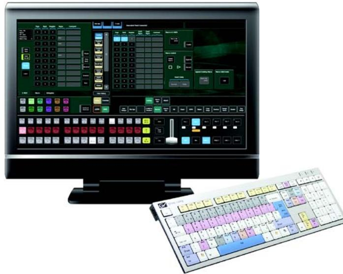
The KSP is an optional 1-ME Soft Panel GUI which provides direct control of switching crosspoints, recalling effects and macros together with an integrated version of the Menu application. A customized PC keyboard is included with the option for users who like quick cut and mix action from a hard-button interface. The KSP can be used as an adjunct to a main panel, providing a second seat (second control surface) in a Suite, or as the only control surface for a second Suite.
