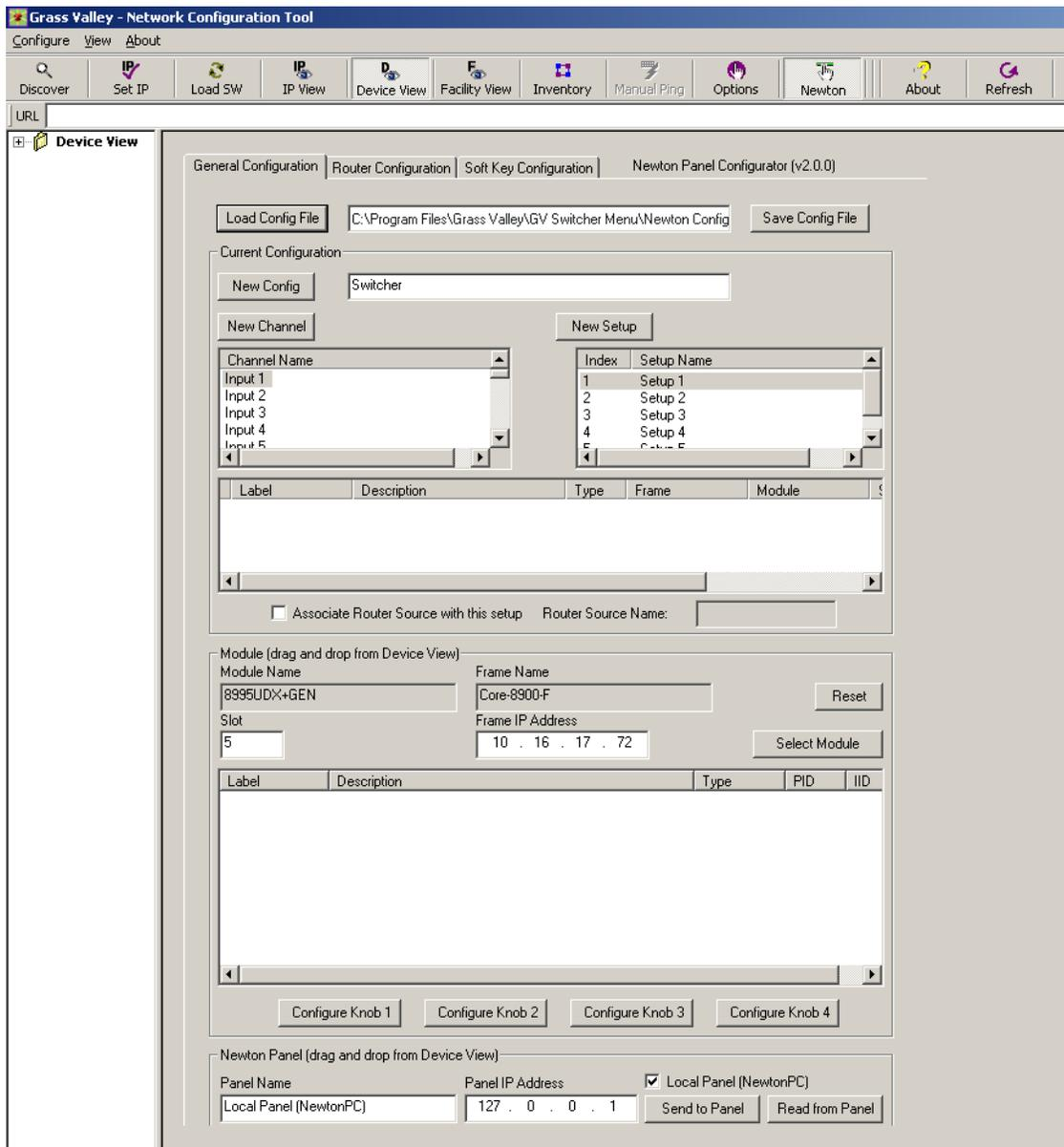
The Configurator tool is used to define the functionality of Newton controls by creating a Newton configuration file. The Newton configuration
