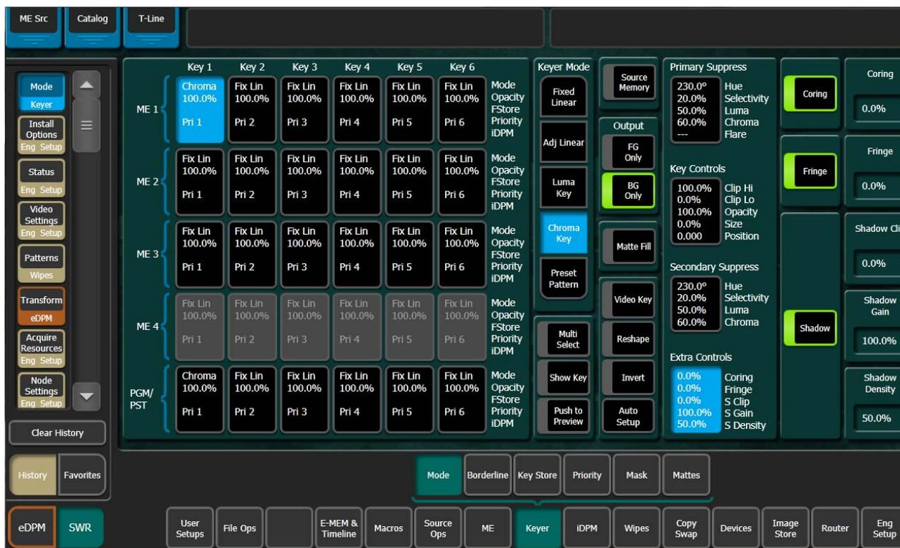
**Coring** replaces any pixels in the luminance signal after primary suppression that are below the adjustable threshold with black. This eliminates noise resulting from incomplete suppression. While coring can improve some keys, it can easily be over done. Coring thresholds much above black will affect dark grays that are actually part of the foreground subject, making the chroma key composite look unnatural.
