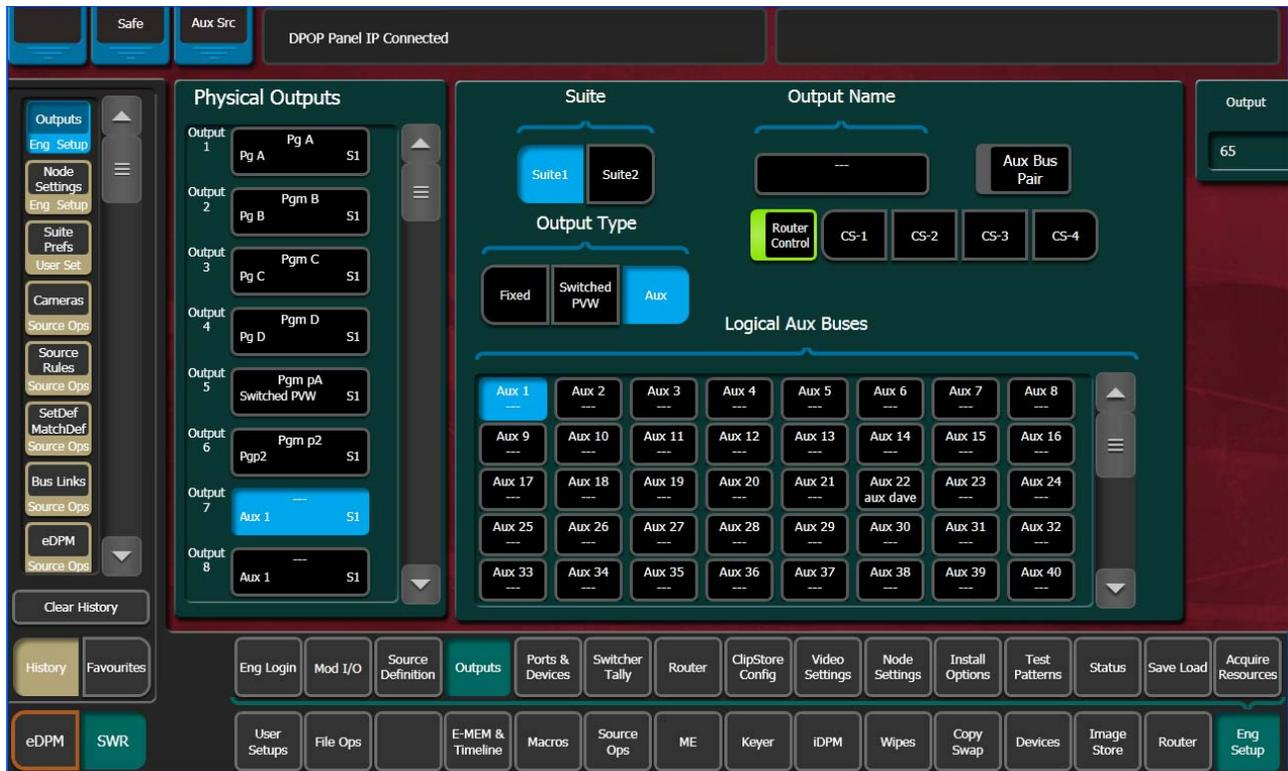
Enable the Aux Buses for router control:
