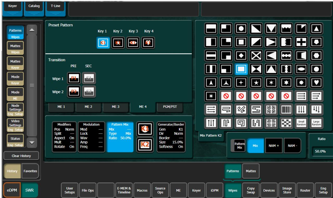
3. Select the **Pattern Mix** data pad, this switches the Pattern tab on the right to the other generator; in this case P2 (to select the base wipe pattern again, touch the Wipe Pattern button as in Step 2).
