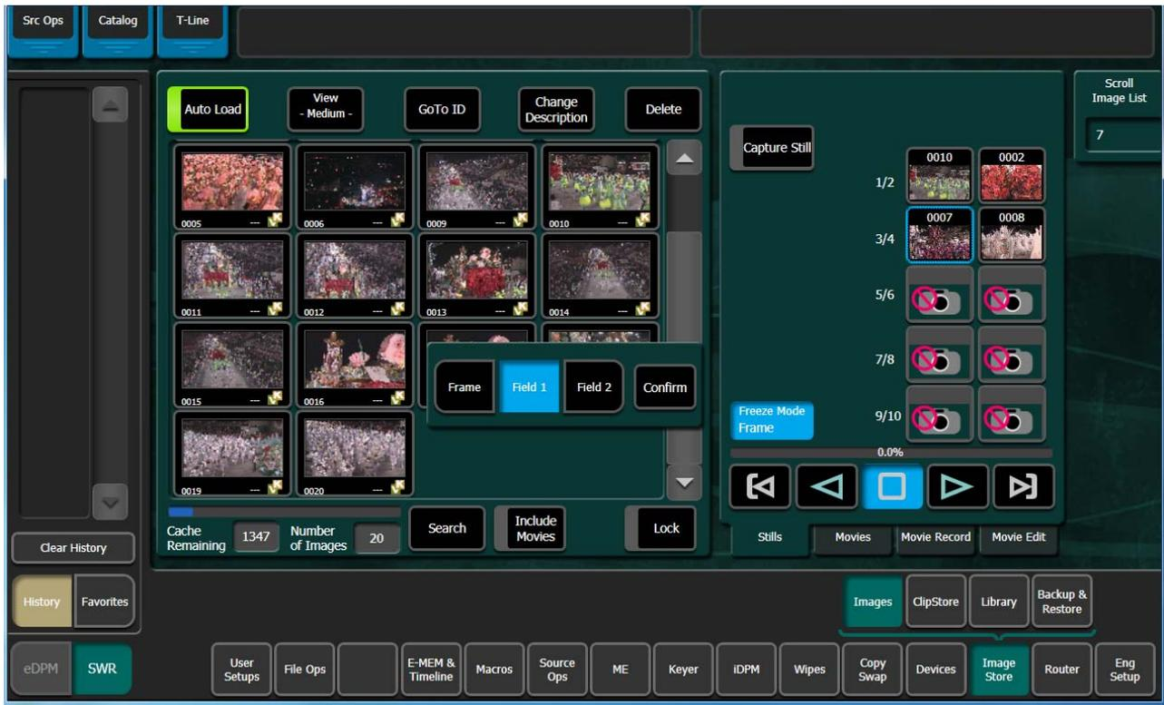
3. Viewing the still on a monitor, touch the **Frame / Field 1 / Field 2** buttons to change the mode for the best result.
