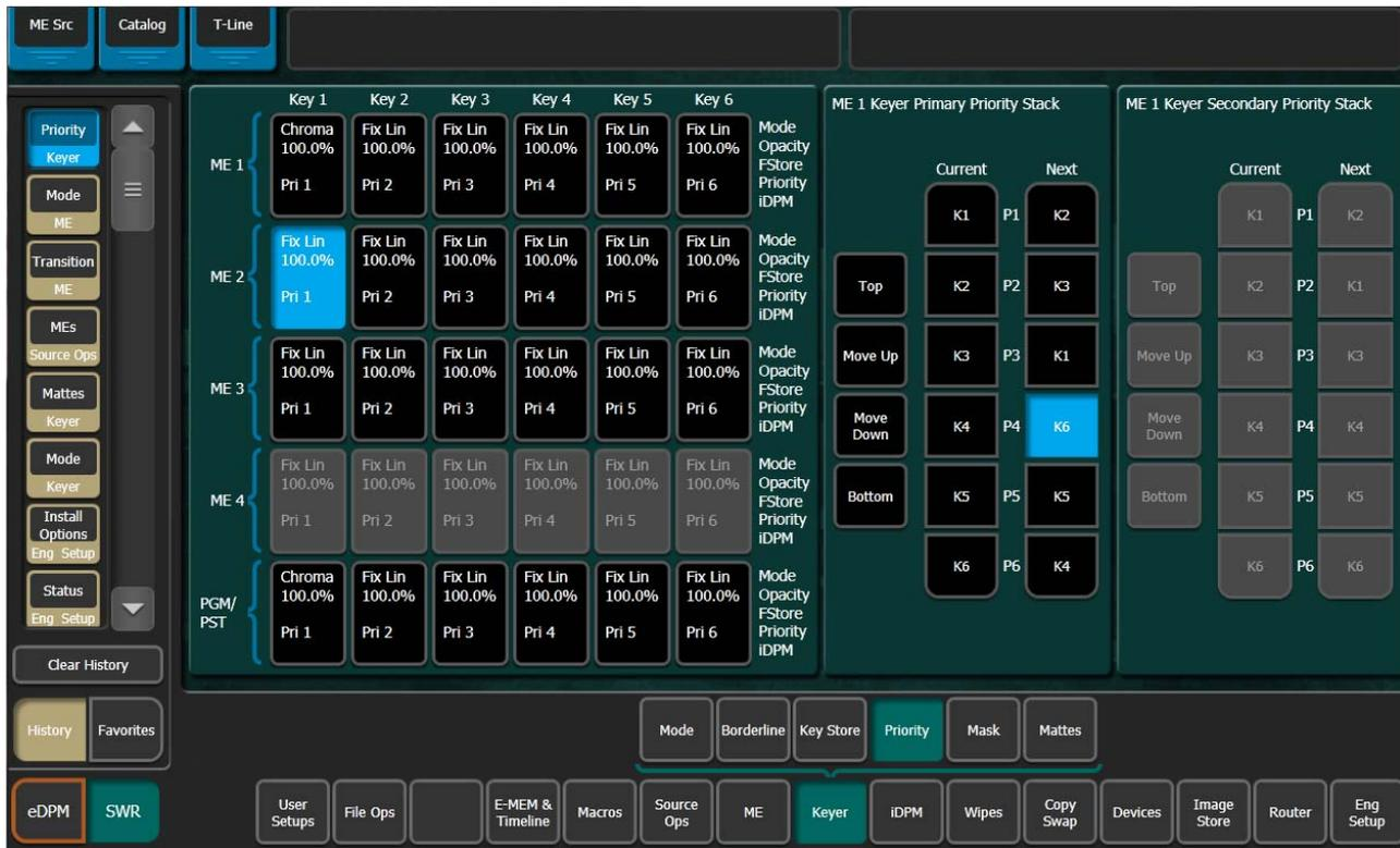
2. If not already set up, turn on the desired keys and arrange them so they overlap, observing the Program monitor. This will make the changes in key priority visible. For demonstration purposes, you can use four preset pattern keys.
