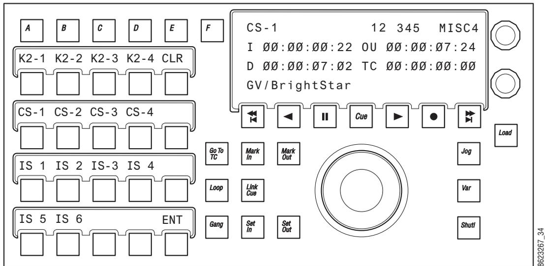
Hold down a lettered button (**A - F**) and press the **Link Cue** button (high tallies blue), the Cue Device Selection menu is displayed (Figure 89). Press the device buttons to add (or remove) devices as part of the cue then press the **ENT** (or **Link Cue**) button. All device buttons added to the cue will tally blue.
