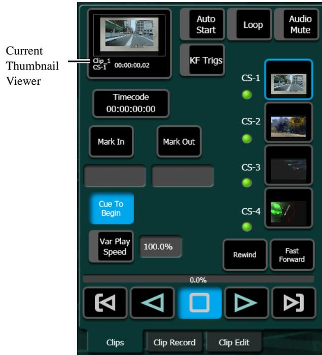
**Note** When a ClipStore channel is selected and a clip is loaded, that clip will be highlighted in *blue* in the scrolling clip list and the list will automatically scroll to display the selected clip.
