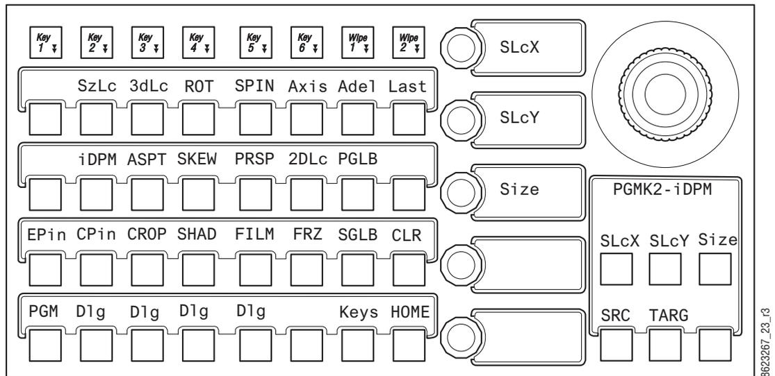
Corner Pinning and Crop controls are located in the CPin MFM Module menu. Press the CPin button to enable/disable Corner Pinning, press the D1g button directly below to turn on Corner pinning and adjust the Corner Pinning parameters using the soft knobs.
