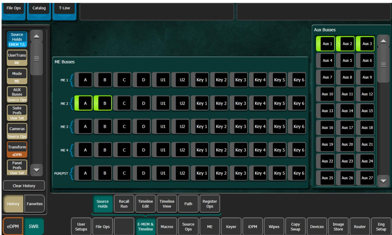
3. Press **Lrn** on the GV Switcher Control Panel (Master or Local E-MEM Module), then press a bank and register number to create a new effect with a Source Hold in its one keyframe.
