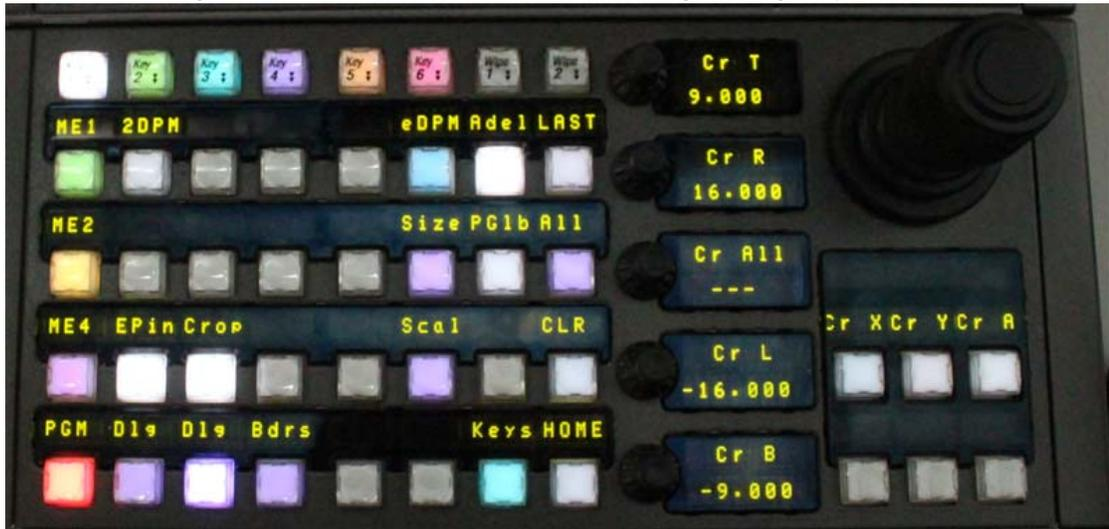
4. Adjust the crop edges using the soft knobs to include the portion of the video you want in the box (key); the shot clock in this example.
