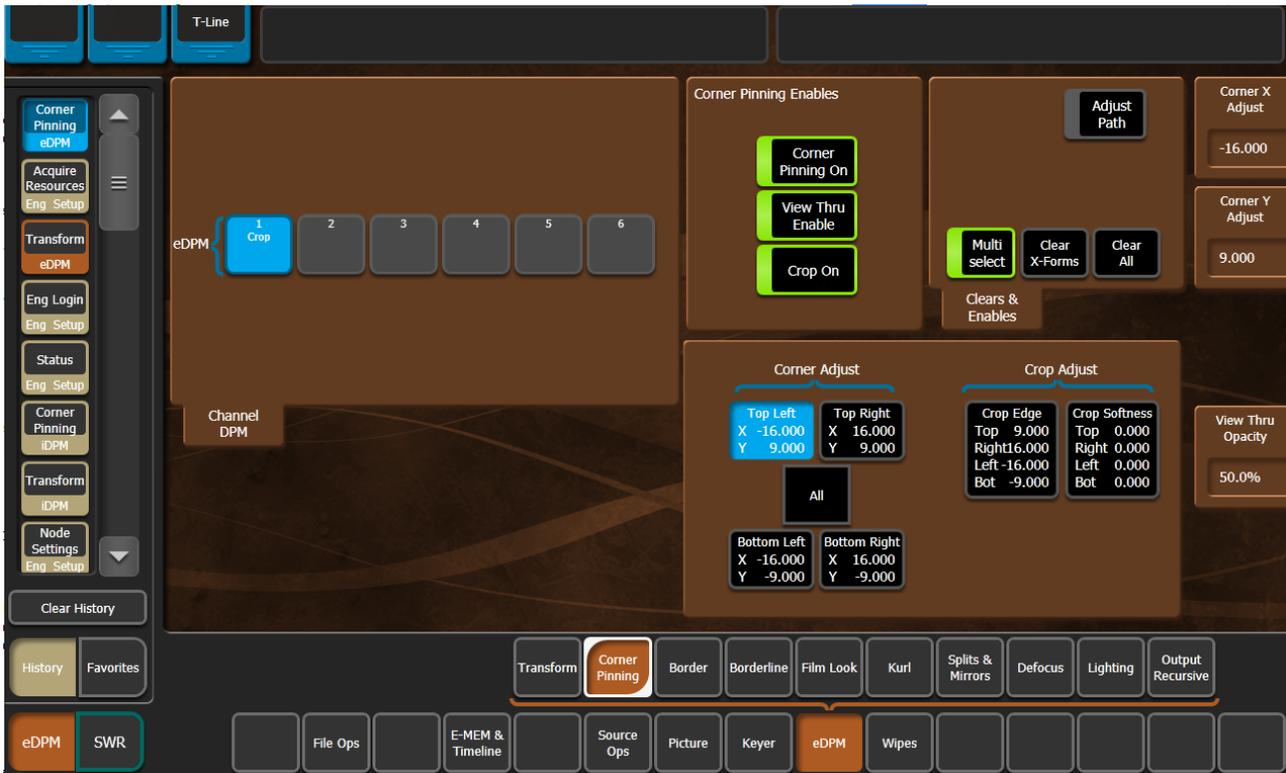
Corner Pinning example: during a sporting event, a camera points at a shot clock. The DPM uses Corner Pinning to build a box to contain the clock and crop adjustments place the clock exactly in the box but the camera is accidentally moved and the content of the box no longer shows the entire shot clock. Using Pan and Scan, you can move the camera content to be shown correctly without moving the edges of the box.
