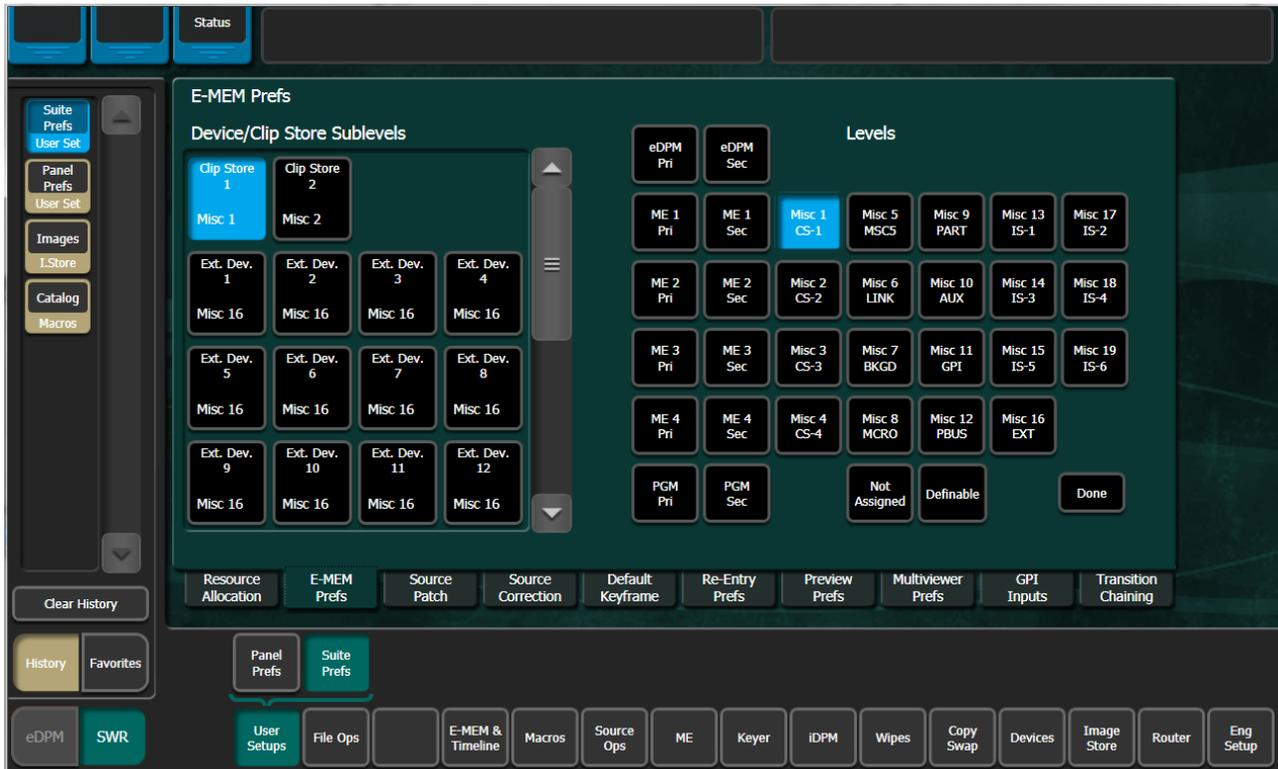
The sub-level is now definable and can be defined to a level. The definable sub-levels are not yet attached to a level.
