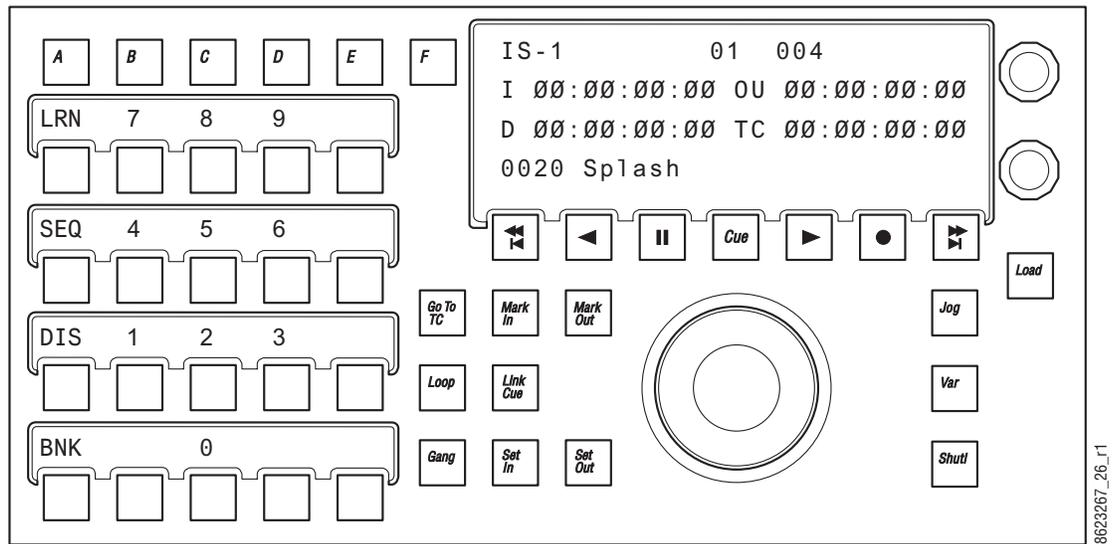
1. Use the soft knob in the upper right of the DCM to scroll through the devices until the desired Image Store channel is seen in the display.
