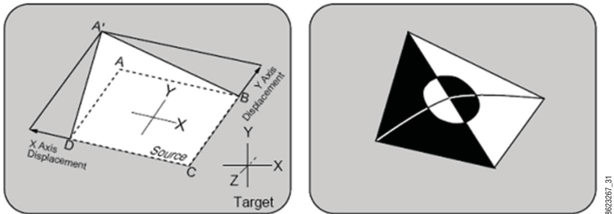
**Corner Adjust Limits**—Corner Pinning works for convex quadrilaterals but not for concave quadrilaterals. A convex quadrilateral is defined as a four-sided shape with all angles less than 180 degrees, all vertices point outwards and all diagonals lie entirely inside the quadrilateral.
