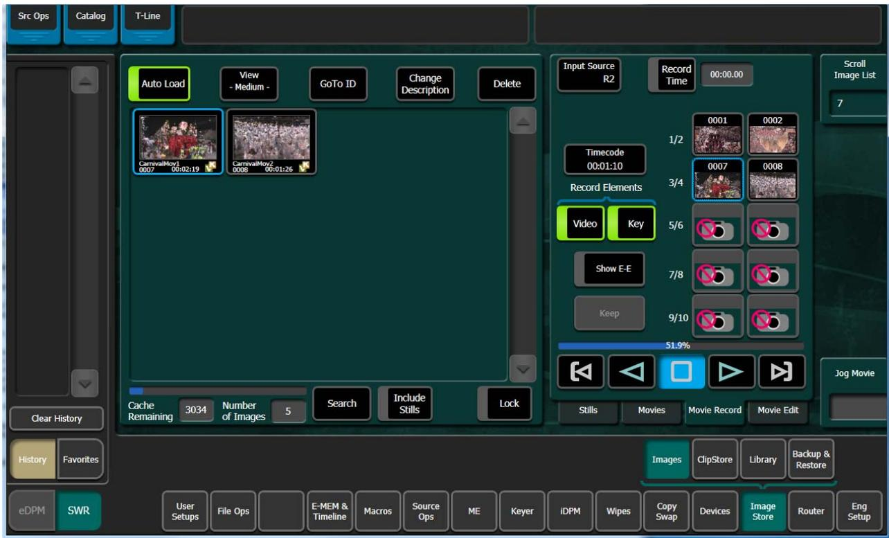
3. Touch the **Show E-E** button. The current movie or clip on that Image Store channel, if loaded, will be unloaded in preparation for recording. The incoming video will be displayed on the output of that Image Store channel. The **Show E-E** button legend also changes to **Record**.
