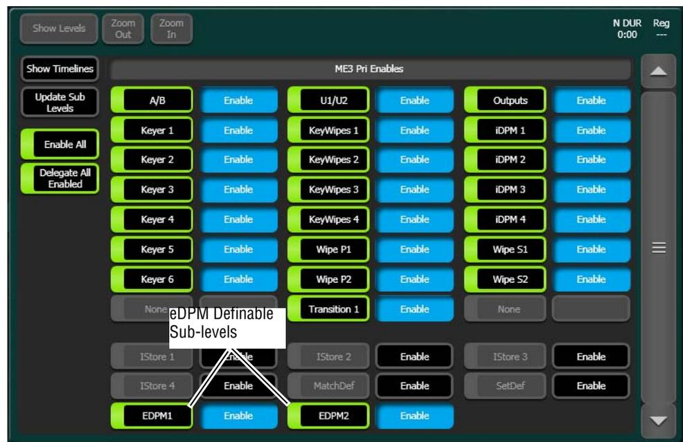
Using definable sub-levels allows for the recall of eDPM effects from Local E-MEM. For example, effects created for ME 1 can have the eDPM definable sub-levels and will then run eDPM effects.
