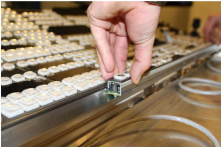
*Aligning the System Bar for Replacement*
