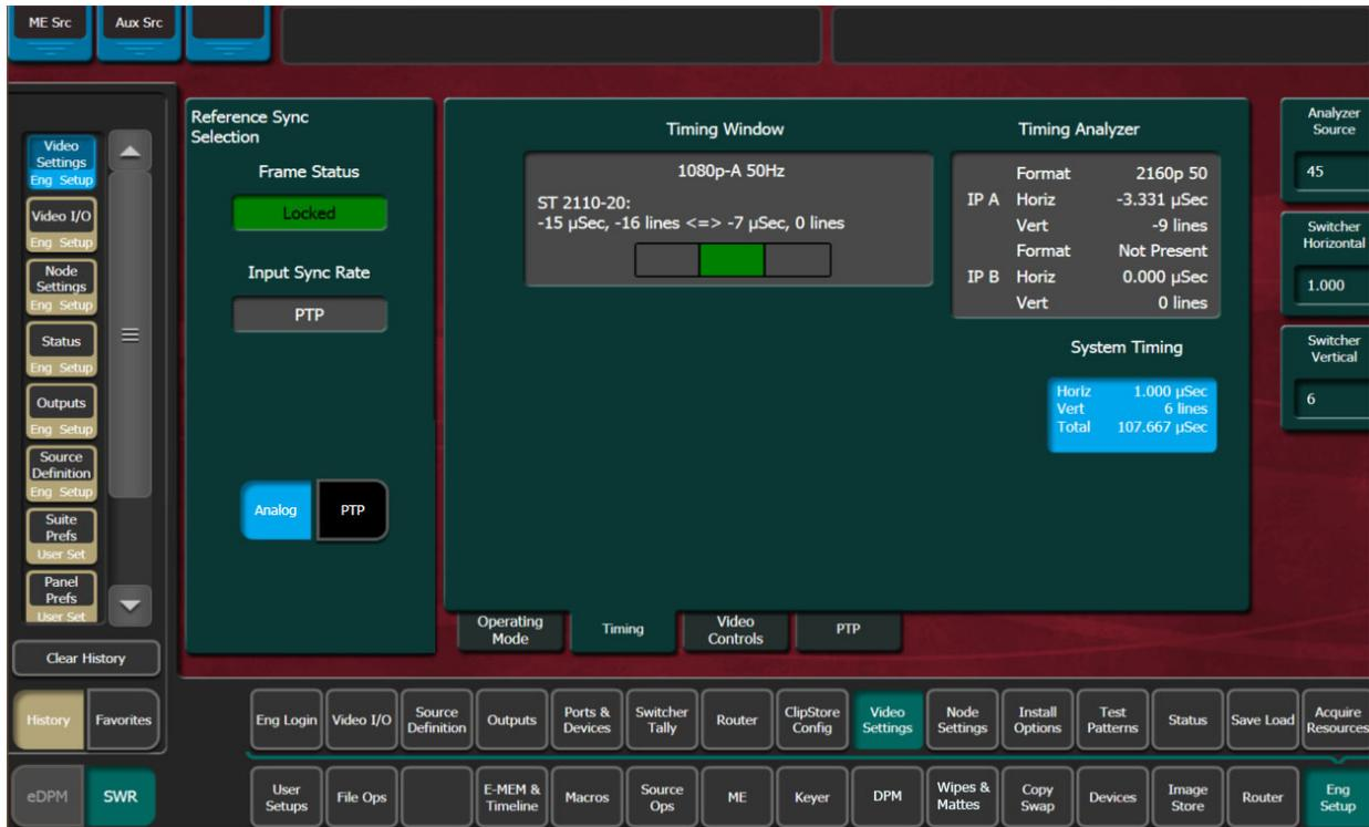
This analyzer reports the timing position of a selected source relative to the internal sync generator. The source is selected with the upper right Analyzer Source soft knob and data pad. The relative position of that source is reported in lines and  $\mu\text{s}$ . Positive values indicate the source is later in time than the internal sync generator, and negative values indicate the source is earlier.
