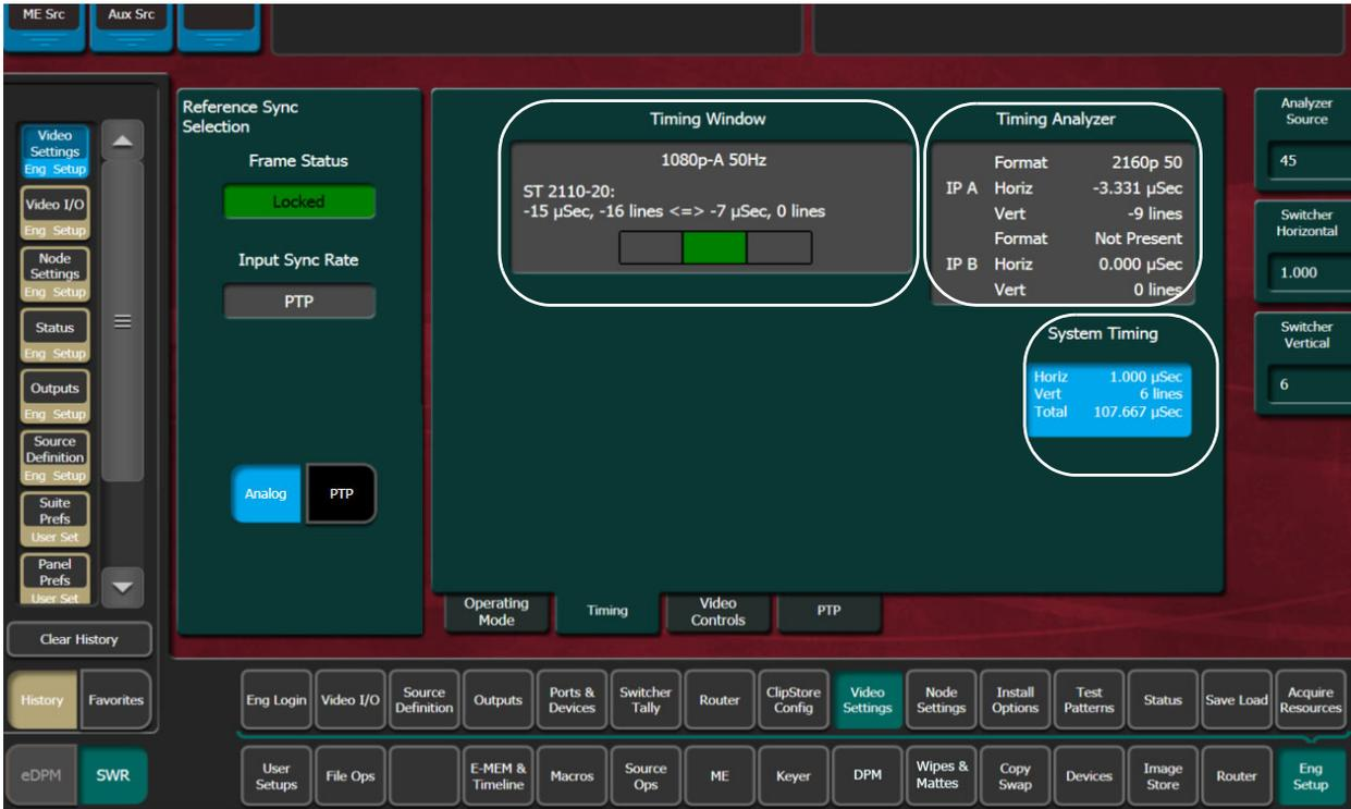
For IP, the *Timing Window* displays the Frame Operating Mode, source type, and the timing window (range) that the source must be within to receive the video. Sources outside the timing window will most likely not pass through the switcher.
