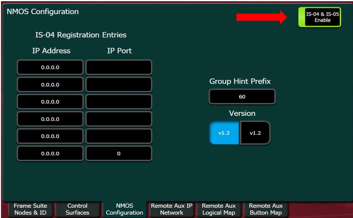
Simple check in the Menu that the Enable button is highlighted green (Eng Setup->Node Settings->NMOS Configuration).
