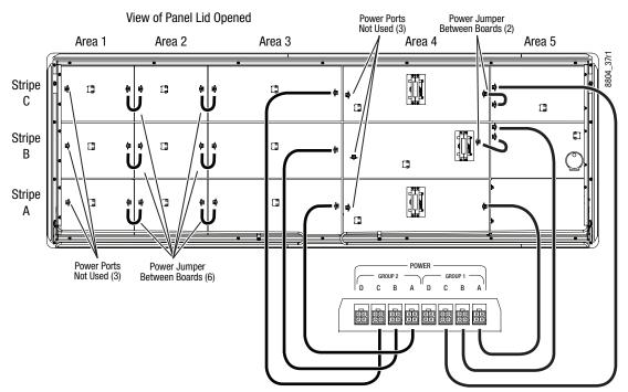
Power Cable Internal Connections, 3-ME Panel
