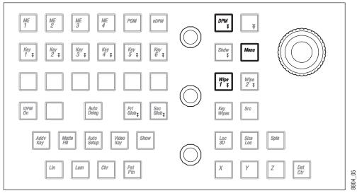
Joystick Calibration Indicator Buttons, Modifier Area
