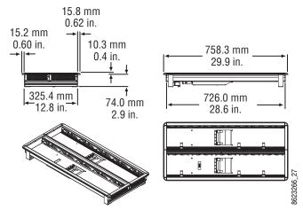
1-M/E 15 Control Panel Dimensions, Flat Installation
