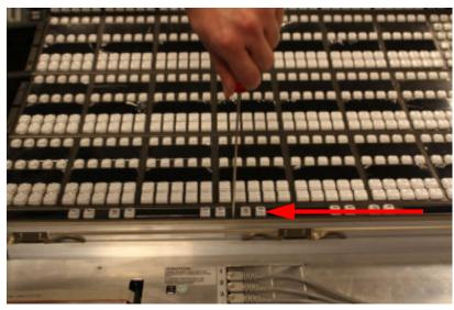
Unscrewing the System Bar
