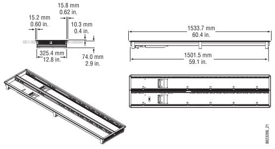
2-M/E 35 Control Panel Dimensions, Flat Installation
