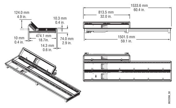
2-M/E 35 Control Panel Dimensions, Flat Installation
