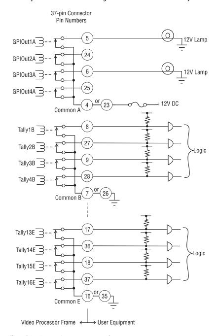
Relay Tally and GPI Output Connection Example
