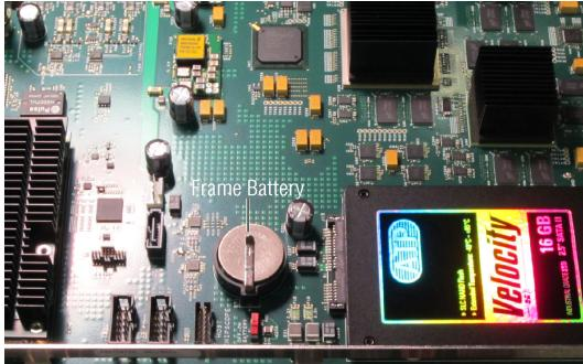
Video Processor Frame Controller Board with Battery Indicated
