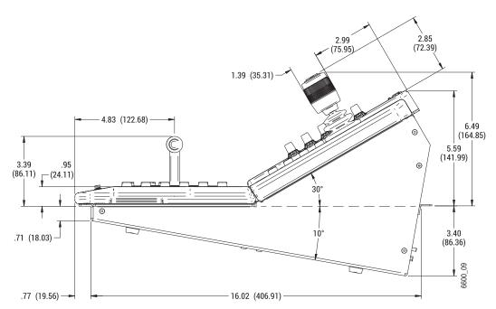
1-M/E GV Korona Control Panel Mounting Dimensions
