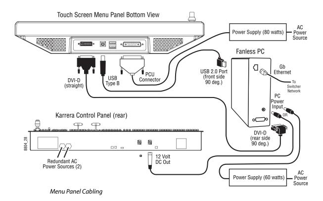
CAUTION: Connect the USB port on the front of the Fanless PC (next to the firewire 1394 port) to the Menu Panel. The default PC settings enable knob control by mapping Com 3 to that front USB port.
