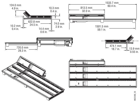
3-M/E 35 Control Panel Dimensions, Flat Installation
