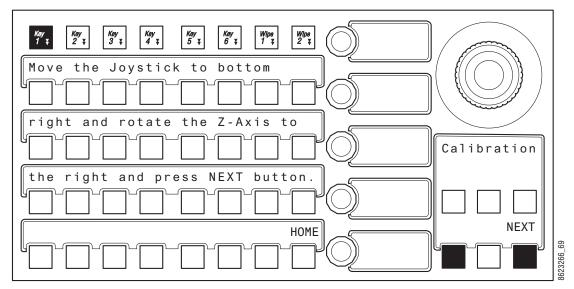
Button Hold Down for Joystick Calibration
