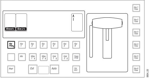
Karrera Lever Arm Calibration Procedure, Transition Area
