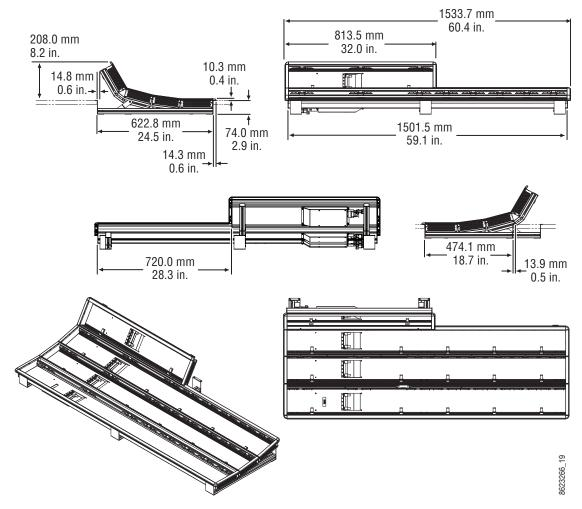
3-M/E 35 Control Panel Dimensions, Curved Installation
