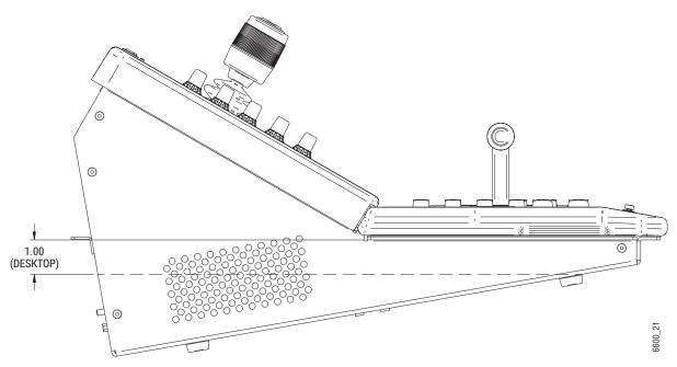
1-M/E GV Korona Control Panel Left Side Mount to Vent Dimension
