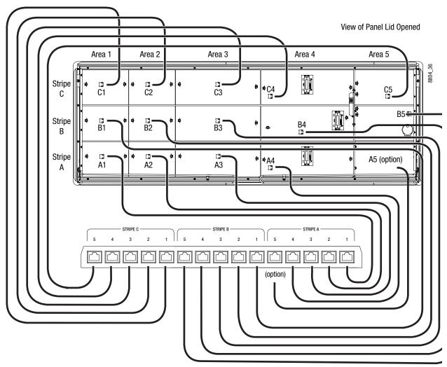
Data Cable Internal Connections, 3-ME Panel
