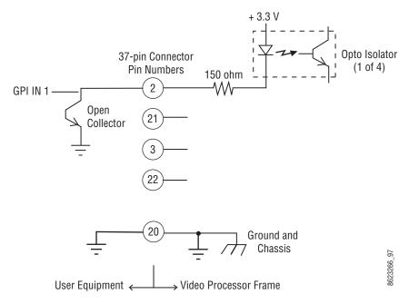
GPI Input Connections (Typical 1 of 4 Connections)
