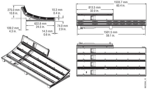
4-M/E 35 Control Panel Dimensions, Curved Installation
