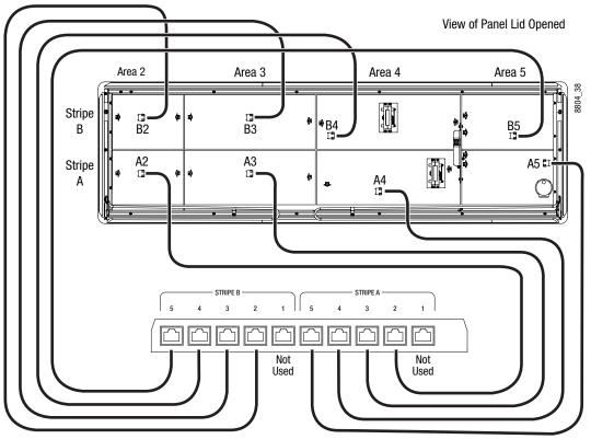
Data Cable Internal Connections, 2-ME Panel
