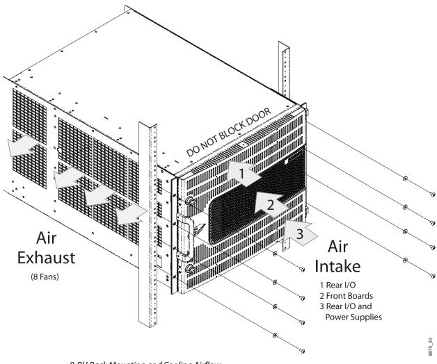
8-RU Rack Mounting and Cooling Airflow
