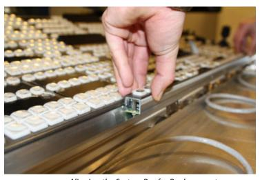
Aligning the System Bar for Replacement
