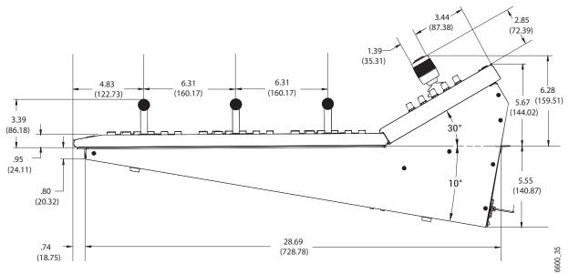
3-M/E GV Korona Control Panel Mounting Dimensions
