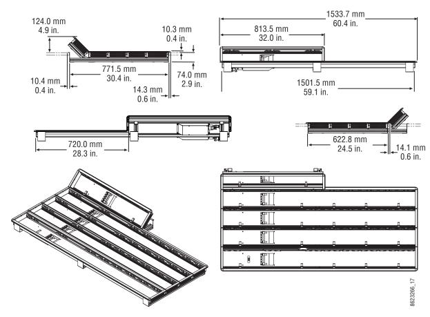
4-M/E 35 Control Panel Dimensions, Flat Installation
