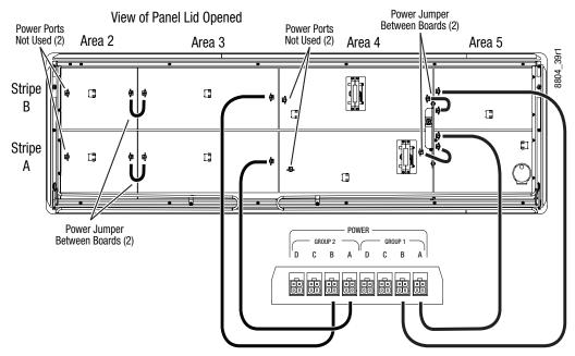
Power Cable Internal Connections, 2-ME Panel
