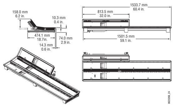
2-M/E 35 Control Panel Dimensions, Curved Installation
