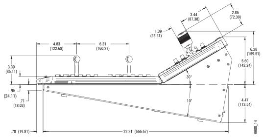
2-M/E GV Korona Control Panel Mounting Dimensions
