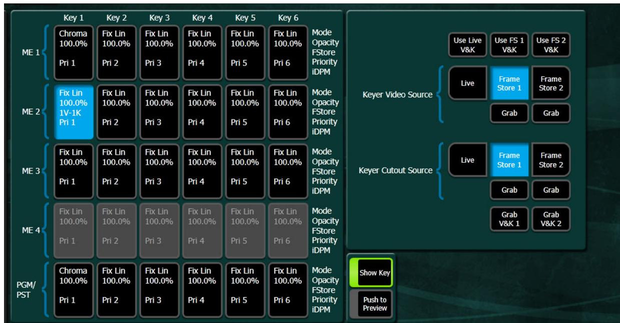
The fill and cut from Live, Frame Store 1, and Frame Store 2 pages can be used in any combination, for example you can use the fill from Keyer Video Source, Frame Store 1 with the cut from Keyer Cutout Source, Frame Store 2. You can even use the Live video from the Keyer Video Source and the cut from Keyer Cutout Source, Frame Store 1.
