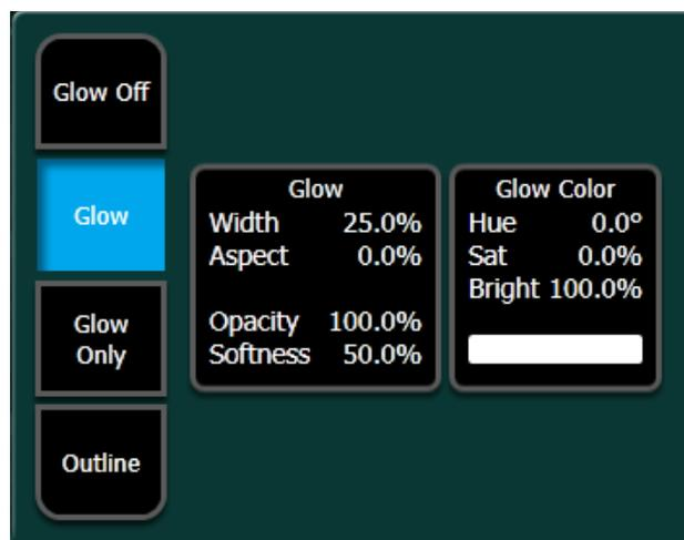
Glow adds a soft edged variable opacity border around keys, leaving the original keyed image unmodified, and is a standard feature available on all GV Switcher systems.
