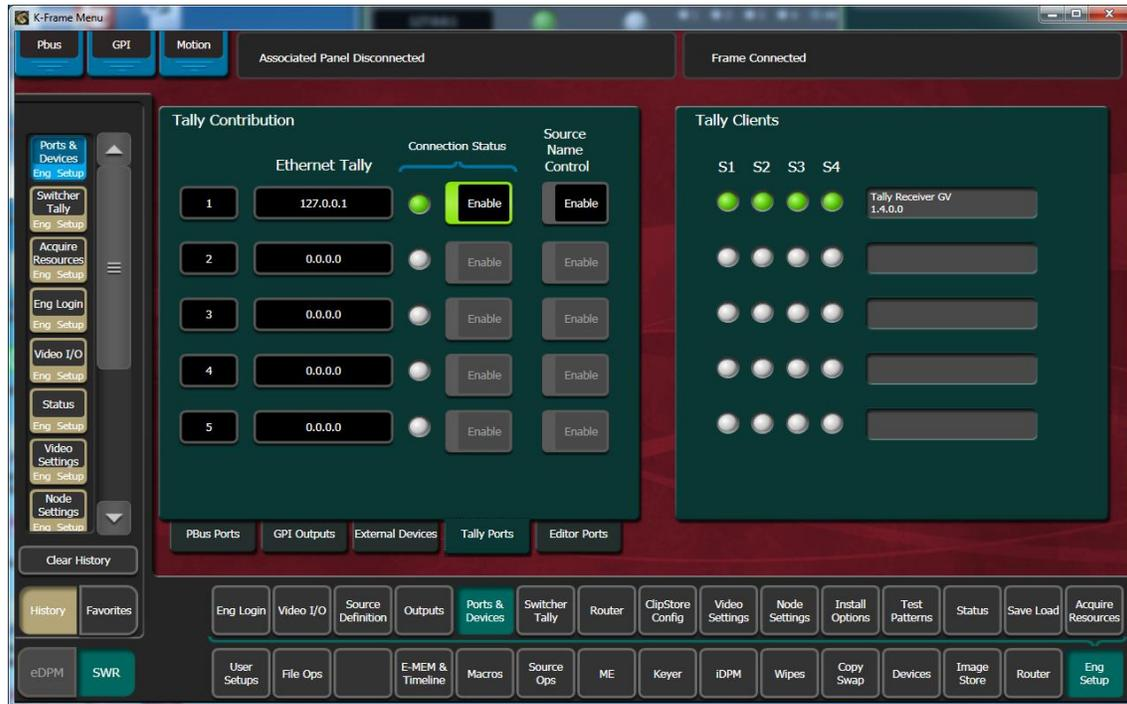
Once Source Name Control is enabled for your connection, Engineering source names may be modified by simply selecting the name field of the engineering source you would like to modify, typing in the new name, and pressing <enter>. This will send a packet to the K-Frame instructing it to change the name of that source. The packet will only be sent when <enter> is pressed. Selecting another source, or pressing <esc> will abort entry and revert the value to its original state.
