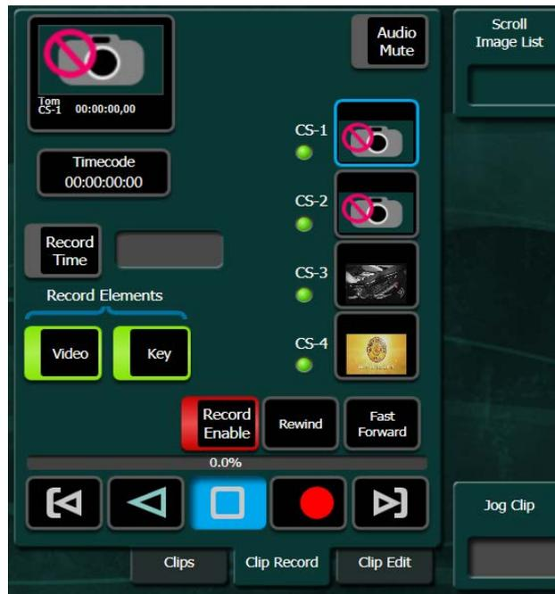
If K-Frame has been configured to use outputs from the frame to feed sources to inputs of ClipStore, in the Source Ops/ImageStore menu incoming feeds can be selected. These input selectors can also be mapped to the local aux panel.
