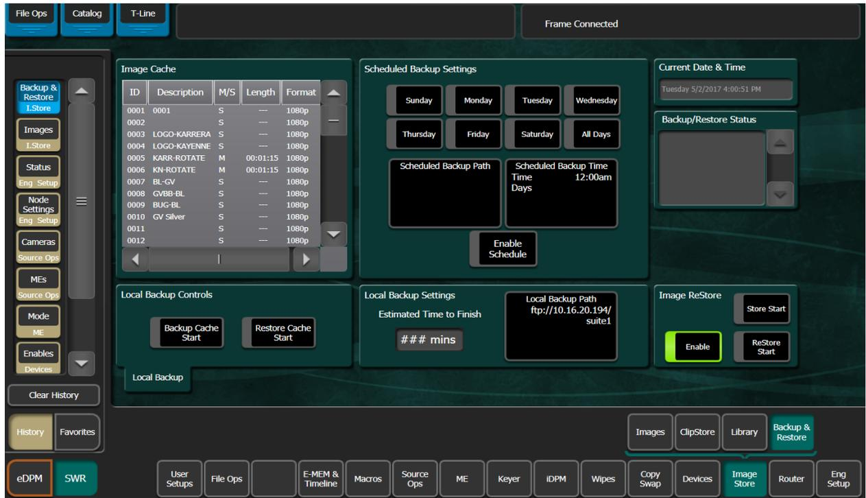
A manual backup can be initiated at any time by designating the backup location in the Local Backup Settings panel and then selecting the Backup Cache Start button in the Local Backup Controls panel. These backed up files can be restored at any time by selecting the Restore Cache Start button in the Local Backup Controls.
