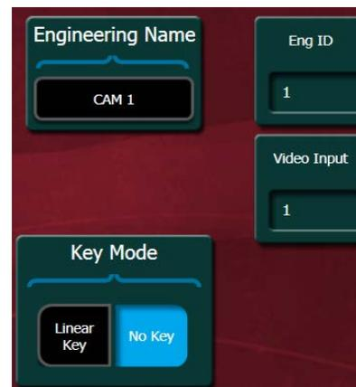
If a source does have a key signal connected to an input connector on the frame, set the “Key Mode” to Linear Key. This adds additional set up dialogue to the menu. Key Input is the BNC connector on the frame where the key signal is connected. Clip High is the maximum value of the matte signal for key (fully opaque portion of key) and Clip Low is the minimum value of the matte signal for key (fully transparent portion of key)
