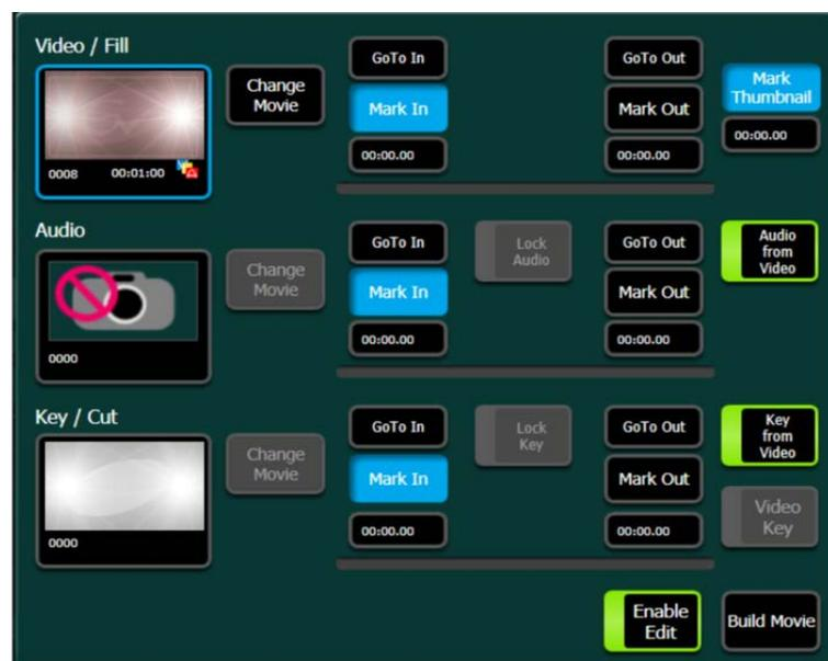
In Cut edit mode selected movies can be trimmed for length or split to make two separate clips. To load the movie to be edited select Change Movie. This will open the cache window to allow for clip selection. To shorten a clip by removing frames from the beginning or end, set a Mark in at the frames where the clip begins and a Mark Out after the last frame of the desired clip. Once marked selecting Trim Movie will remove the unwanted frames.
