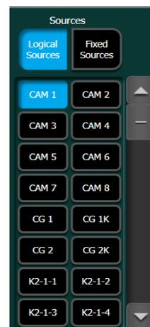
The panel on the right of the menu is the map-able sources. Logical Sources are sources defined in Eng Setup/Source Definitions. Sources such as cameras, clip servers, graphics, etc.
