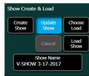
When updating a show, select the show file in the storage area of the menu and on the right side of menu enable the portions of the show file you wish to update. In register based files such as EMEM and Macro's, enter the register numbers of the elements you wish to add to the show in the field next to the enable buttons.
