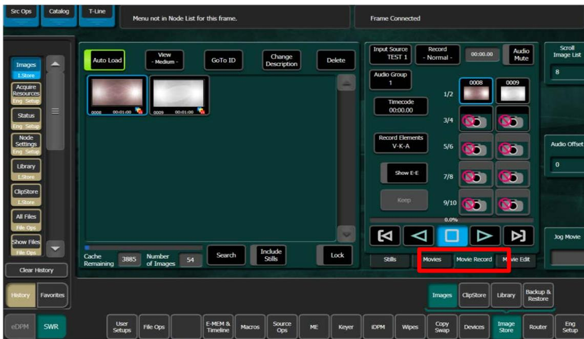
The Movie Record works in a similar manner as the Still Capture controls. Selecting the Input Source box will present the source select table.
