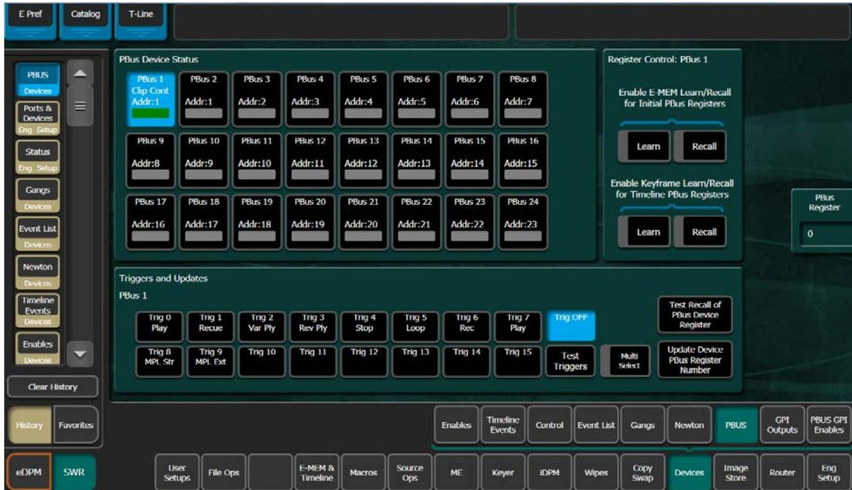
The upper left portion of the menu is delegation for selecting which PBus device is to be controlled by either E-MEM or Macro commands. The green bar in the delegation box indicates that a device has been programmed. From the Eng Setup menu the device can also be named to indicate which device has been programmed for that position.
