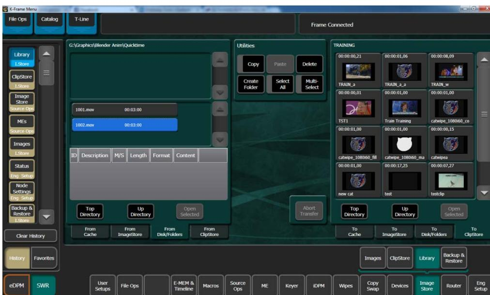
Files that are not ClipStore native format will be converted if supported by K2. MXF, AVI and MOV files with the following elemental formats can be converted on import.
