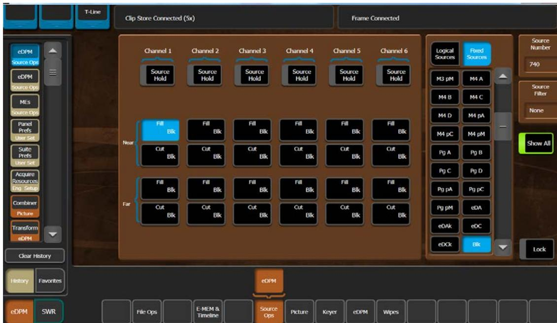
When a source is selected for the input to a channel of eDPM both the video (fill) and key (cut) are input to the channel. Because DPM channels don't have their own key signal, the one being fed from the source is used.
