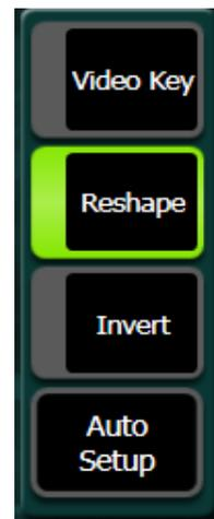
Data box selections with controls that have adjustable numeric values, selection will assign those controls to the adjustable soft knobs on the right edge of the menu panel.
