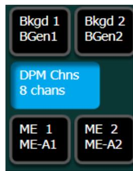
Any or all available channels can be assigned where needed by selecting the left pointing arrow. Each mouse click of the arrow will assign another available channel.
