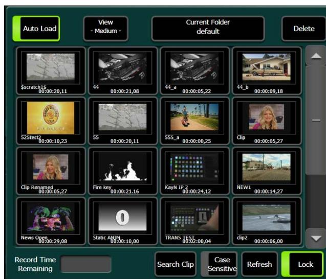
Because ClipStore can have several different directories/folder for storing clips, to change the clips displayed in the left panel, select the box labeled Current Folder and a menu
