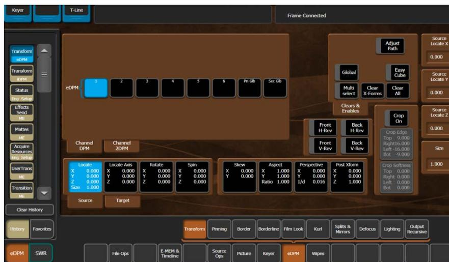
Available channels can be assigned where needed by a double left mouse click (or double-tap with finger) on the source delegation box of the desired channel or keyer, in the upper left quadrant of this menu. For iDPM channels you can also assign channels by going to the ME/Effects Send menu, selecting the desired keyer and enabling the “Effect Send Active” button.
