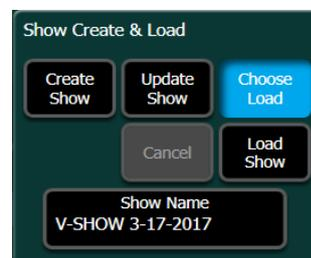
When using the Choose Load command you can select what you want to load into the system by enabling the specific items on the right. In the case of register based files (EMEM, Macro, etc.) and you can enter the register number in the corresponding fields.
