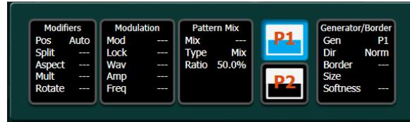
The controls selected above are wipe pattern select. On each ME the transitional wipe generators are labeled P1 and P2 for primary 1 & 2 and S1 and S2 for secondary 1 & 2. As indicated by the menu transition wipe 1 (the button on transition panel) has been assigned primary wipe 1 and the pattern select for P1 is displayed on the menu screen.
