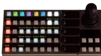
Note: When using the Joystick on Kayenne and Karrera, the Locate 3D button controls the X, Y and Z parameters of Locate. The Size Locate button controls X, Y and Size. On Korona the Joystick will control the selected item in the iDPM menu. Where there are more than 3 parameters, the ones highlighted in blue will be affected. To toggle the blue highlighted items in the menu, press the softknob associated with the parameter you wish to control with the joystick.
