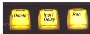
***Macros do not record any adjustments made with the knobs, lever arm or joystick.***
