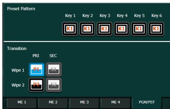
The panel below wipe delegation is selection for each of the different sets of controls. Each box in this panel indicates which set of controls by the text title at the top of the box. Each box also indicates the current settings of the controls accessed by that box.
