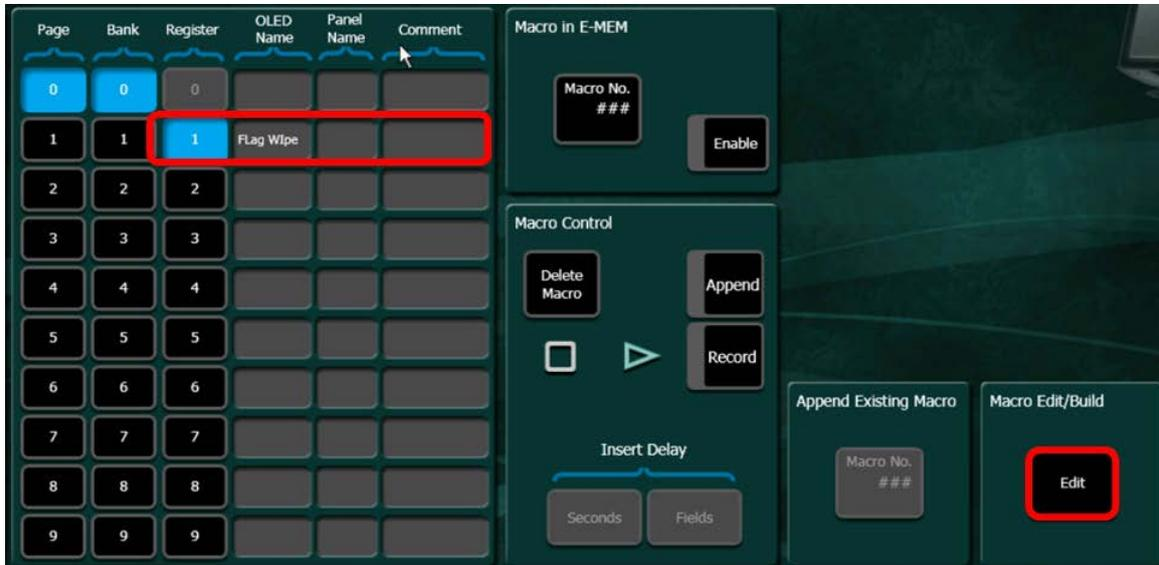
The edit screen will open with a list view of each of the commands recorded. The macro below is similar to the one in the example on the previous page. One of the issues in the macro below is that the Key Cut key stroke is a toggle. This means that if the macro is in the on state when the macro is run the first key cut will turn the key off and the second will turn the key on. This command can be changed by selecting the line to edit and then selecting the Edit Line button on the right.
