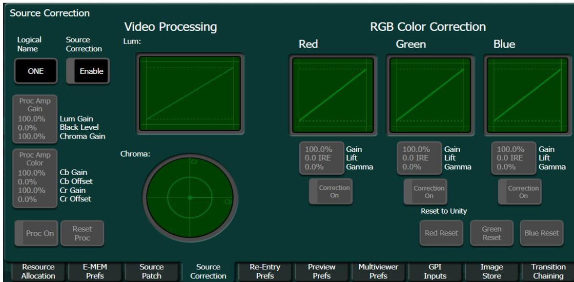
YUV video processor has settings for gain control of luminance, black levels and chroma levels. There are also controls for gain and offset of Cb and Cr components.
