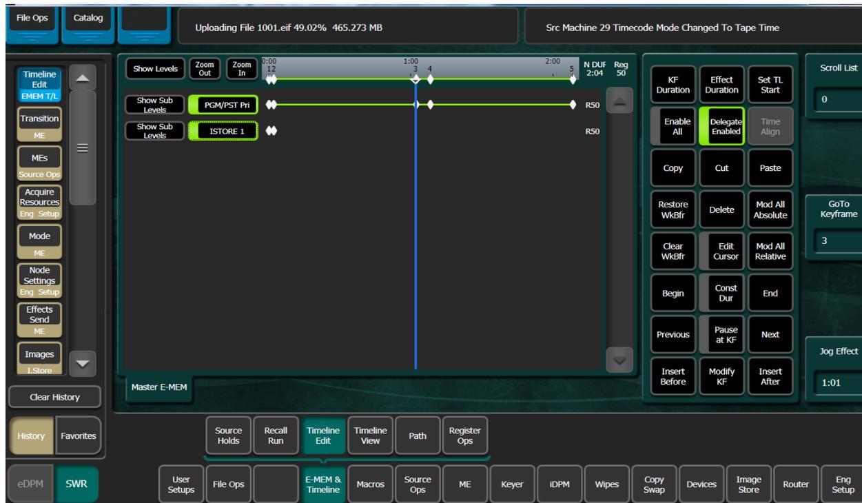
From the E-MEM & Timeline primary menu select the Timeline Edit sub-menu. On the right side of this sub-menu are a series of buttons used to create and modify timelines in the Master E-MEM registers.
