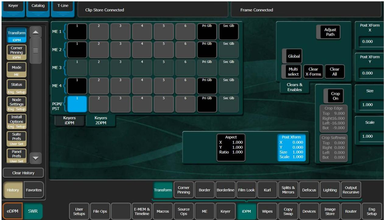
Post Xform in 2dDPM differs from iDPM in that it has both a Size and Scale control
