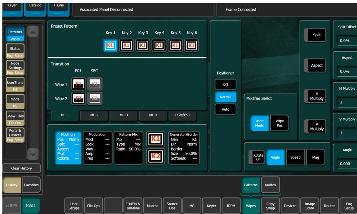
Each ME has two transitional wipes for primary and two for secondary partitions (on systems with Double-Take). There are also two wipe generators for each key. Keyer wipes are used for masks and pattern keys. Keyer wipes are not used for transition.
