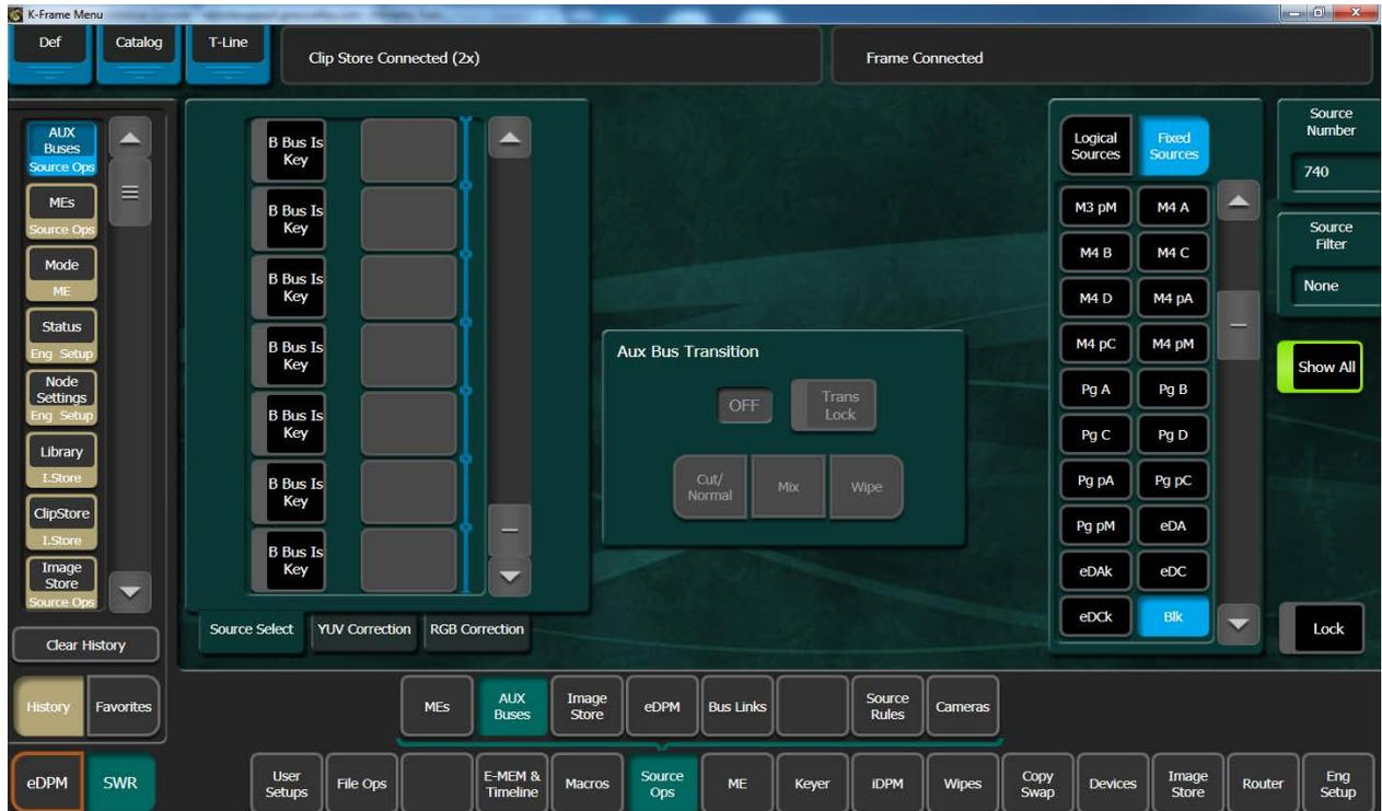
If an ME transition partition has been allocated in the User Setup menu, Aux Bus transitions can be set up from the Aux Bus menu. From the Aux Bus Transition panel in the menu Mix or Wipe transitions can be enabled for the selected Aux Bus. If a transition is selected the next source change on the selected Aux Bus will be placed to that output using the selected transition.
