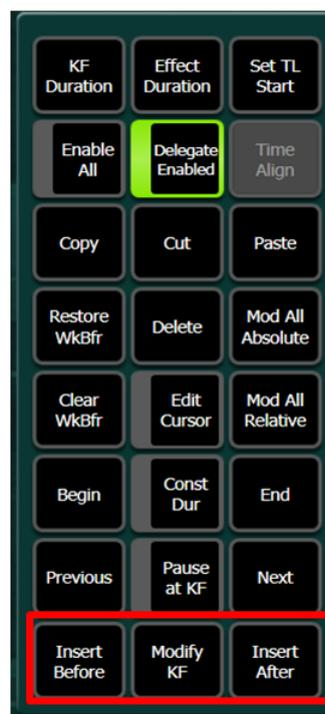
Existing key-frames can be updated with new values using the modify buttons. Place the timeline cursor on the key-frame to be updated, make the necessary changes and then use one of the following selections:
