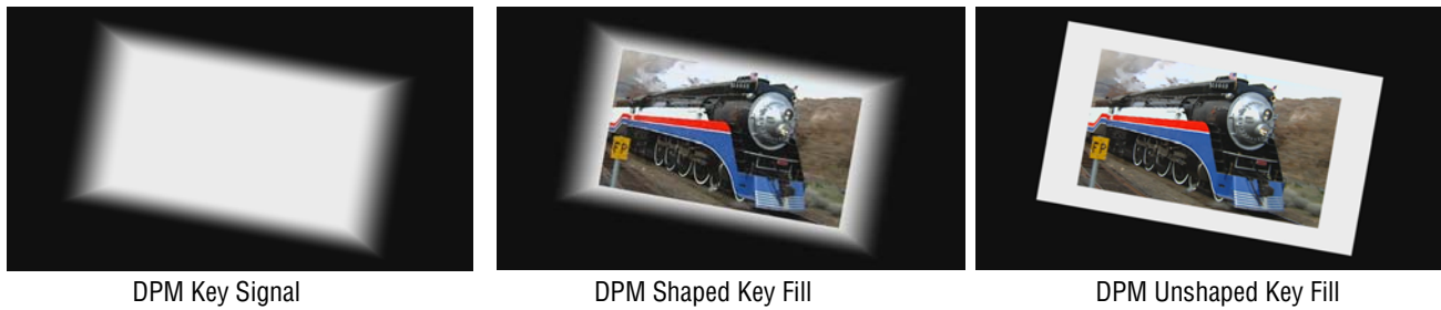
Figure 15. Video and Key Signals from DPM
