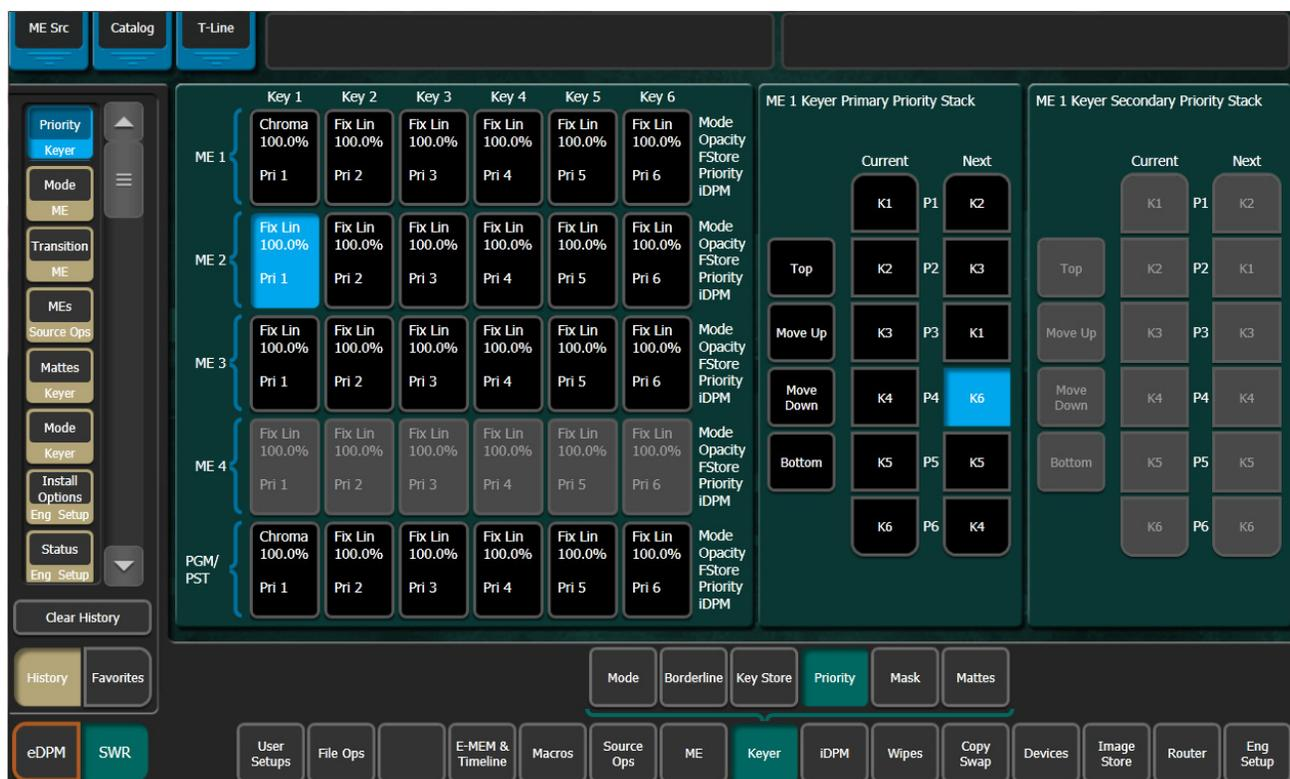
7. Select the type of transition, using the **Mix**, **Wipe 1**, or **Wipe 2** transition buttons on the Control Panel. If you selected a wipe, go to the Wipes menu by double pressing one of the **Wipe** buttons, and then select the pattern and any modifiers to be used with the wipe.
