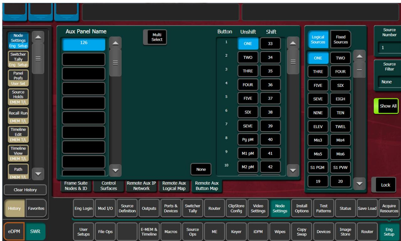
2. Select an individual Remote Aux Panel by selecting its button in the left pane or select the **Multi Select** button for group selection of the Node Settings menu.
