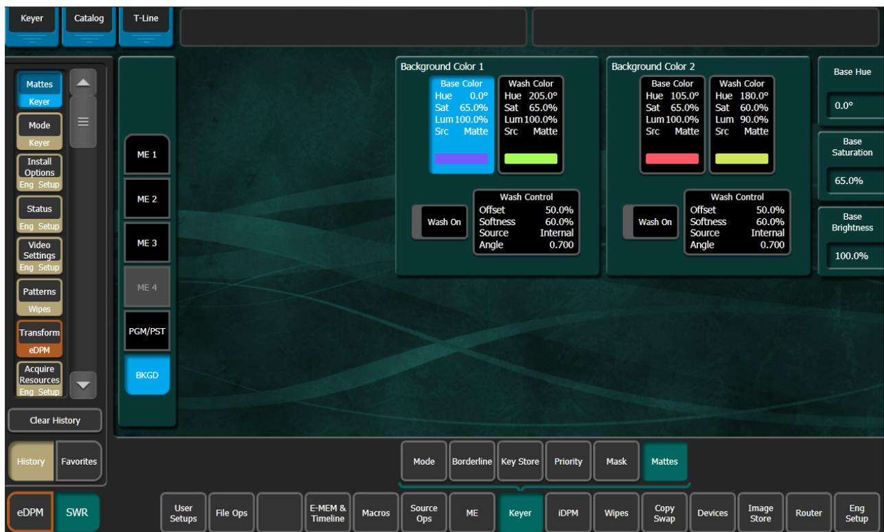
4. Select the **Wash On** button at the bottom so its indicator illuminates to create a wash matte.
