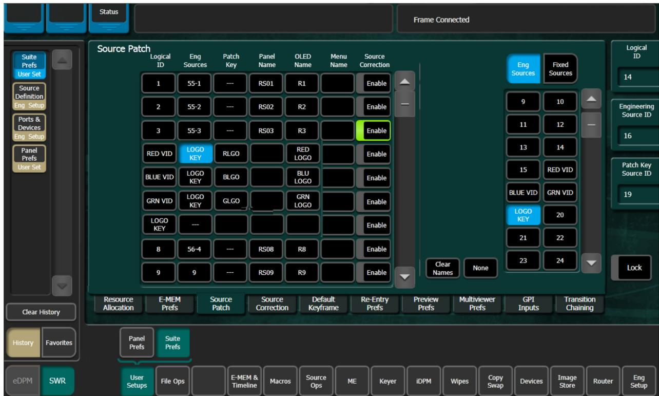
2. Select the data entry pad in the Patch Key column for the Logical ID you wish to patch a key from a different source.
