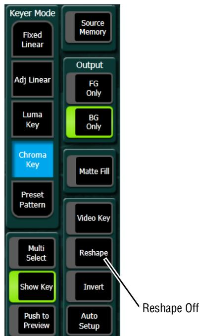
6. Press the **Auto Setup** button on the Control Panel or select it in the menu. Preview for that ME will now display the chroma key source with a superimposed cursor. The cursor actually represents a box of 16 x 16 pixels.
