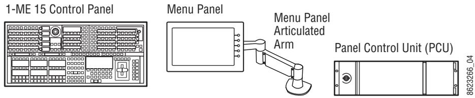
The modular design and use of a separate PCU supports the hot-replacement of individual Control Panel components, if necessary, while the rest of the system remains operational.
