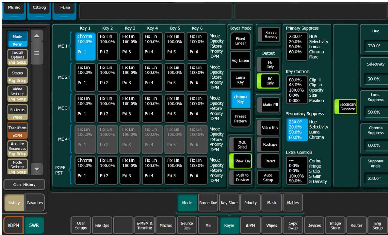
2. Adjust secondary suppression **Hue** and **Selectivity** so that the translucent area is affected, but opaque areas of the foreground are not. The final hue will lie somewhere between the backing color (primary suppression hue) and the uncorrupted foreground color.
