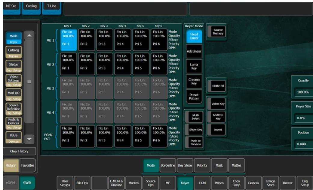
The Grass Valley menu is “always on top” but can be minimized to a pull-down in the upper left corner. Minimizing the KSP minimizes the entire GUI.
