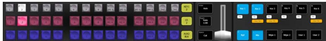
The Transition Area in the Operations window is used to select the transition components (Bgd, Key 1-Key 6) and the transition type (Mix, Wipe 1 and Wipe 2, and User 1 and User 2). These selections are keyboard and/or mouse controlled with each button as an on/off toggle for the transition components and a “radio button” group for the transition type.
