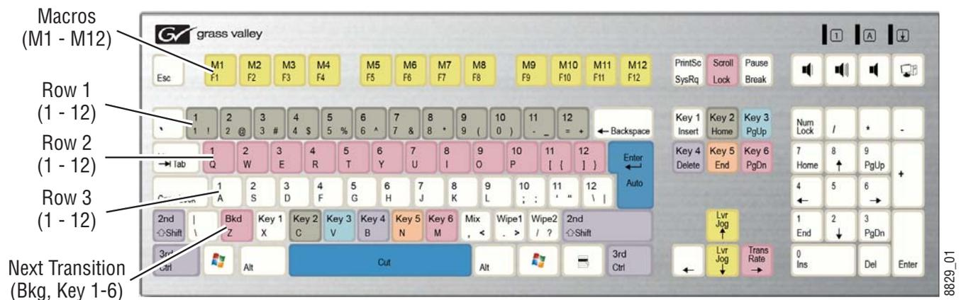
Dedicated buttons are also provided on the keyboard for each of the ME's six keyers, along with twelve Macro Attachment buttons. The numeric keypad provides E-MEM control. Also available are Cut, Auto transition, and lever jog control at the touch of a button.
