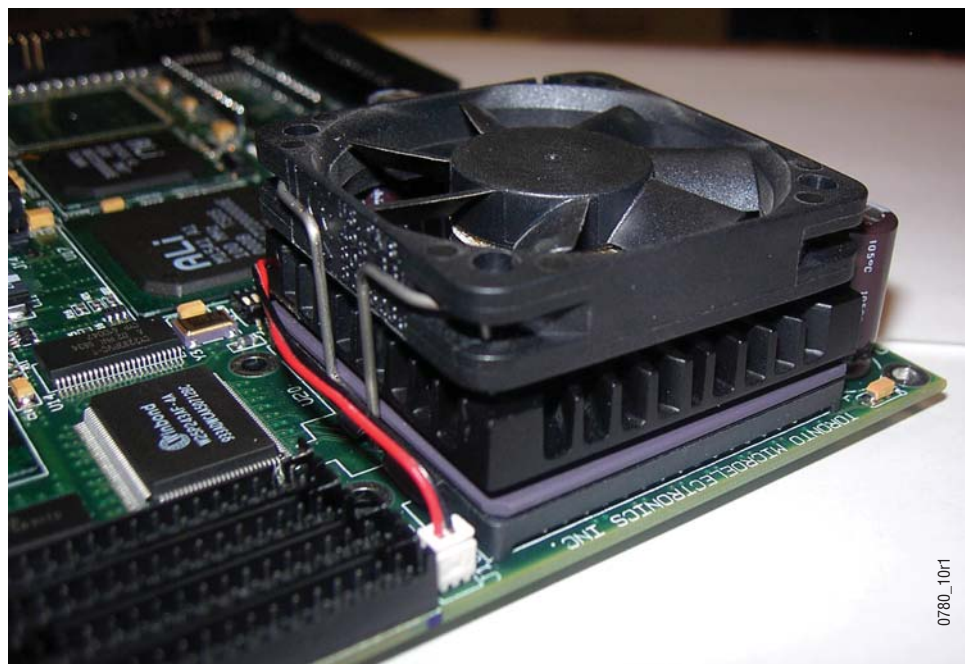
Figure 10. New fan installed on heat sink with label side down, clips secure, and power connected
