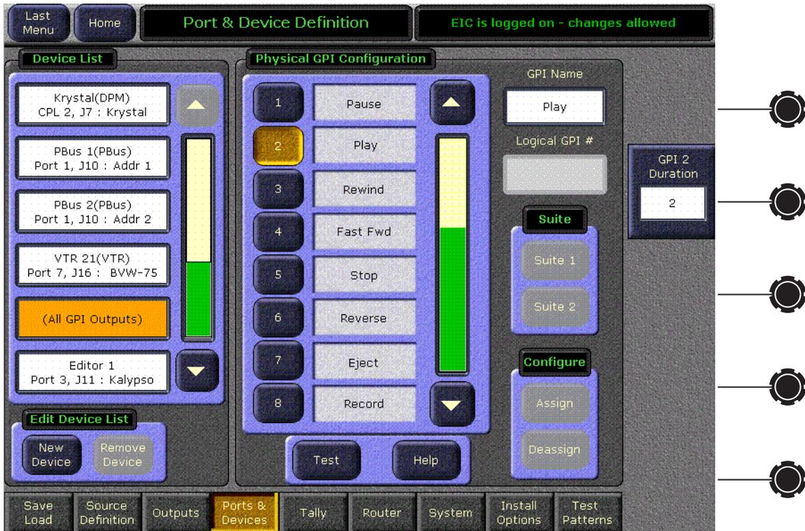
The buttons in the scrolling list represent the 16 physical GPI output relays available on the Kalypso system (1-16). The functions performed by these relays depend on how they have been connected to the device being controlled.
