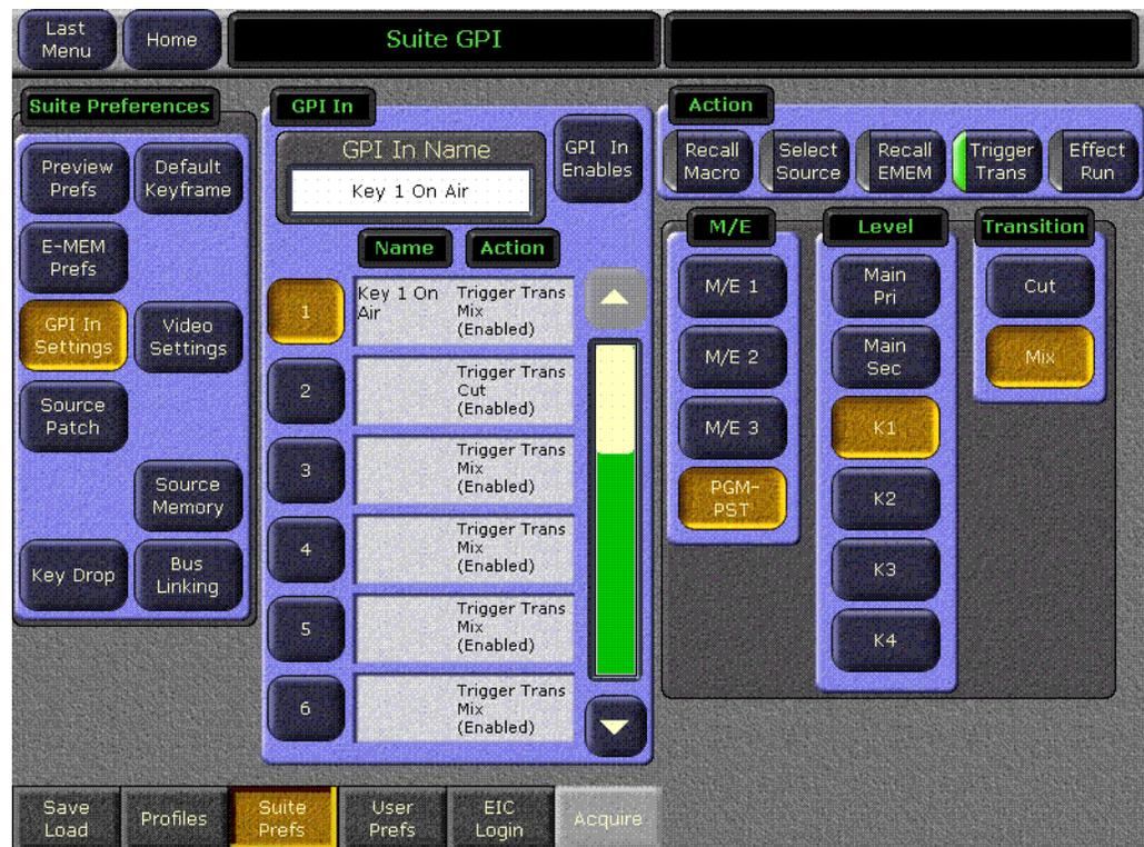
To program a GPI, select the GPI input to program from the scrolling list in the central pane. Then select the action and appropriate qualifiers on the remainder of the menu. In the example above, GPI 1 has been programmed to transition Key 1 on the PGM PST A bus. See the *Kalypso User Manual* for more information.
