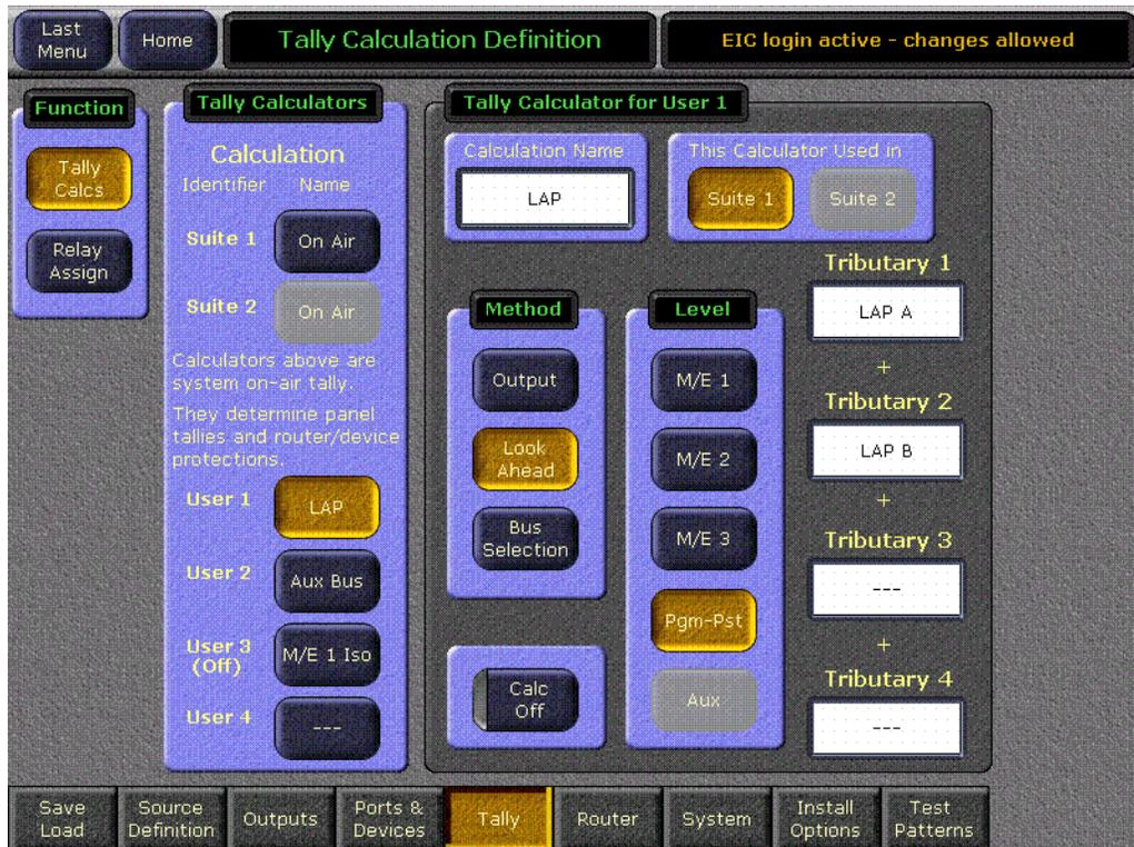
The Method pane has three button choices so you can select between **Output**, **Look Ahead**, and **Bus Selection**. **Calc Off** is a toggling button with a red LED. If **Calc Off** is activated, the tally calculator is shut off, and (Off), is printed
