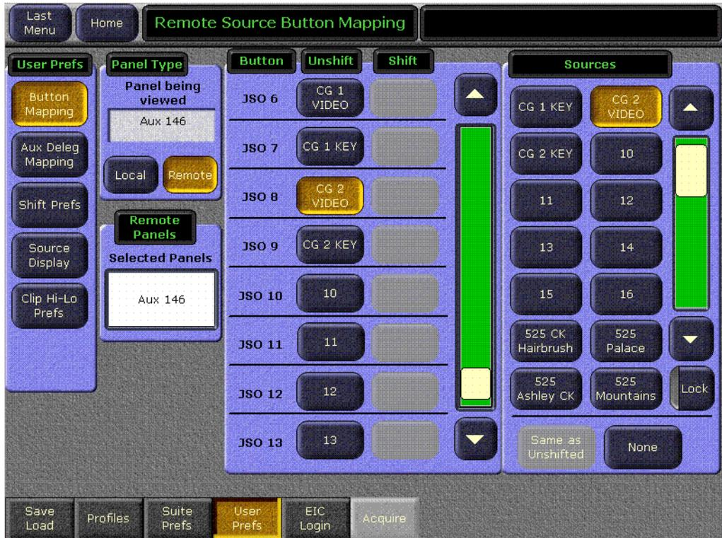
1. Select the Remote Aux panel to be programmed by touching the lower right **Remote Panel** button, touching the yellow data pad, and selecting the remote Aux panel from the list. After selection you are returned to the previous menu.
