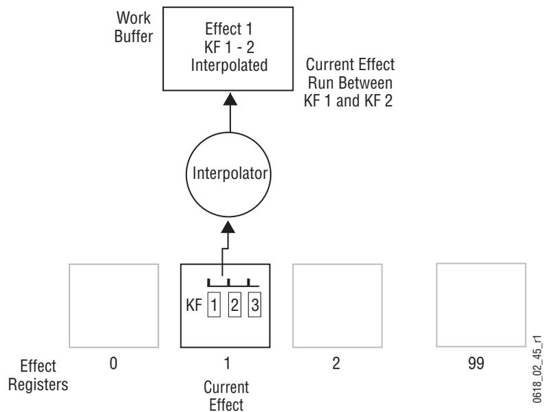
The interpolated work buffer values created during the effect run do not exist in the effect register. Instead, *path* information saved in the effect
