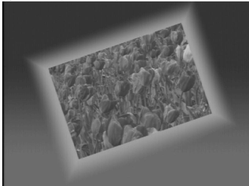
When the DPM provides a shaped video output but the key is processed as though it were unshaped, the shaped video does not completely fill the key hole in the background so a dark halo appears around the key (Figure 66).
