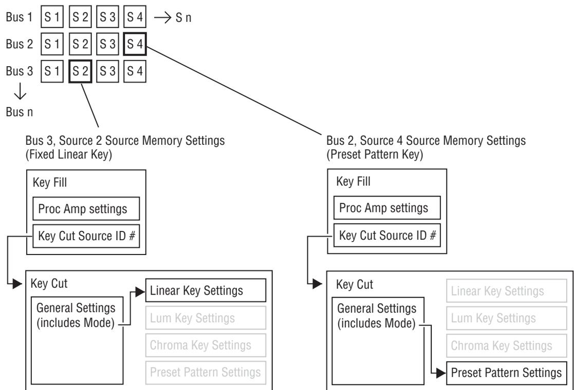
Because a Kalypso source may have two signals (key cut and key fill), different groups of source memory parameters are associated with each signal. The Kalypso system key buses always have key cut and key fill signals. The background A and B buses that do not have key cut signals do not use the key cut group of source memory parameters.
