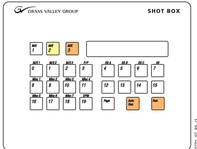
The Shot Box can be powered from the Main panel through the cables provided. If located more than 3 m (10 ft) from the Main panel, an optional Satellite Panel extension kit is available that includes a brick type power supply.
