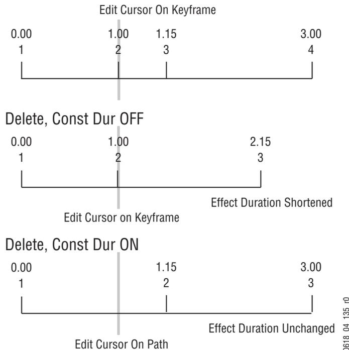
Note that after a **Delete** with Constant Duration ON the cursor is located on the path, not on a keyframe. You will need to move the cursor to a keyframe before you can use **Delete** again.
