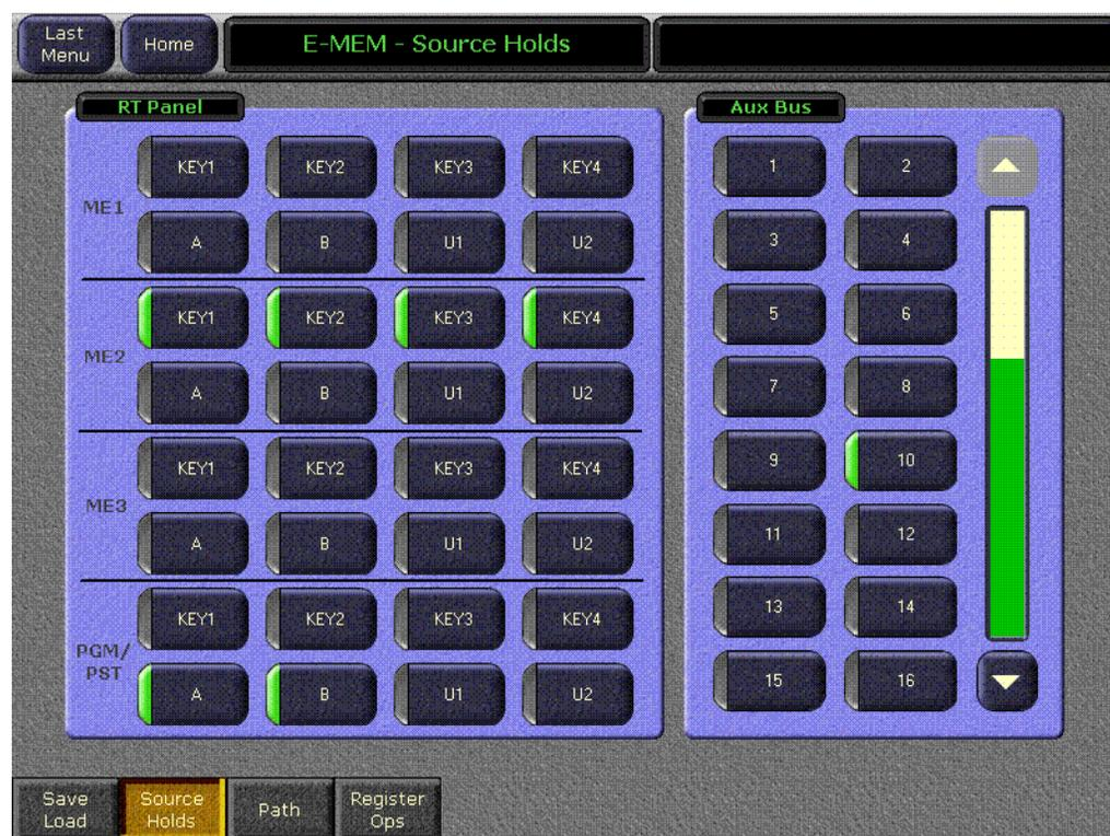
3. Press **Learn** on the Kalypso Main panel E-MEM subpanel, then press a bank and register number to create a new effect with a Source Hold in its one keyframe.
