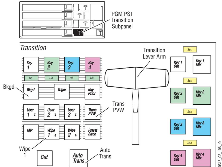
4. Observing the program monitor, move the PGM PST transition lever arm from one limit to the other. A wipe pattern is now used for the transition.
