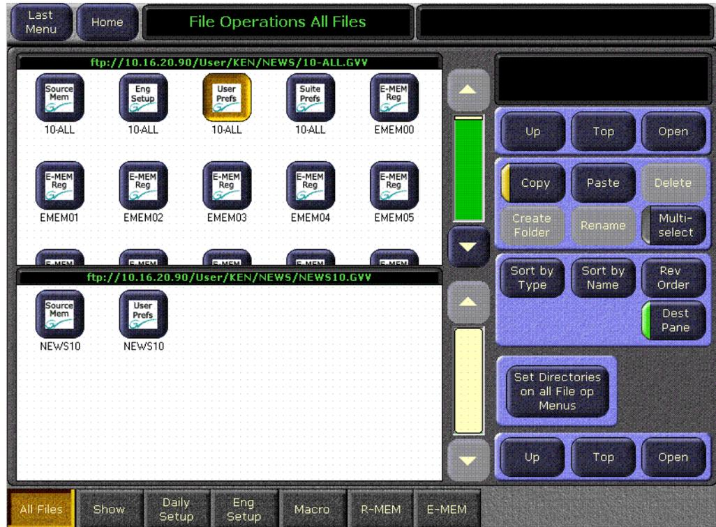
4. Navigate the lower pane to the desired directory, using its navigation buttons.
