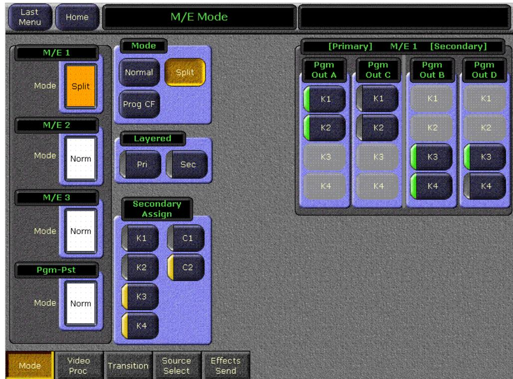
In **Split** operating mode, the M/E is divided into Primary and Secondary partitions. The Primary partition has the Pgm A and Pgm C outputs that use the Background A and B buses, and the Secondary output has the Pgm B and D outputs that use the Utility buses. The Pgm Out columns on the menu are re-arranged when Split mode is selected to show the A and C Primary outputs on the left and the B and D Secondary outputs on the right.
