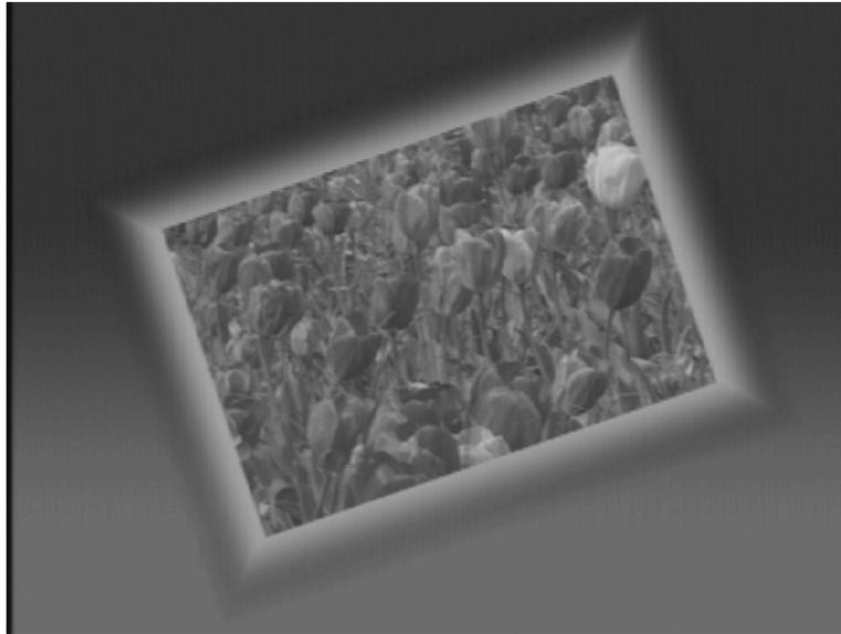
In this case the shaped input is incorrectly shaped again, sometimes called a double-multiply (Figure 67).
