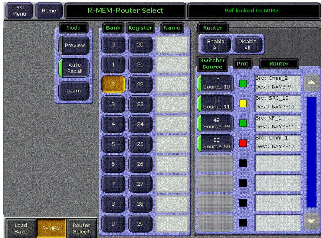
The R-MEM menu has a mode pane on the upper left, a pane in the center listing the R-MEM registers available (the full register number is displayed on each register button), and a Router pane on the right showing the switcher sources, router sources and destinations, and protection status. Switcher sources configured as routed Kalypso sources appear in the right pane.
