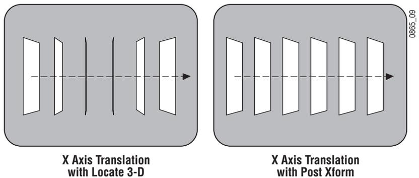
All post transform functions are made relative to the monitor screen frame of reference. For example, a positive X post transform always moves to the right side of the screen.
