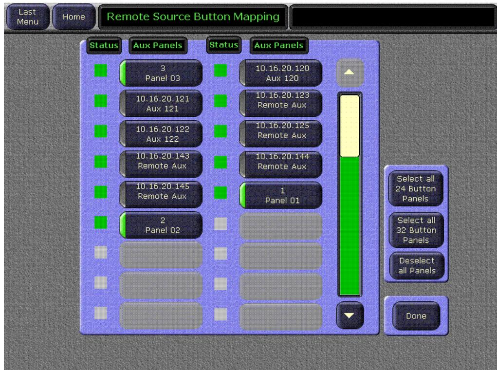
3. Individual Remote Aux panels are selected by touching the buttons in the large pane. Buttons on the right allow selection of a group of Remote Aux panels, by type. Only the same type of Remote Aux panel can be selected with the Select All buttons or individually. An attempt to select both a 24 button and a 32 button panel will be rejected with a message posted indicating the panels are not the same type.
