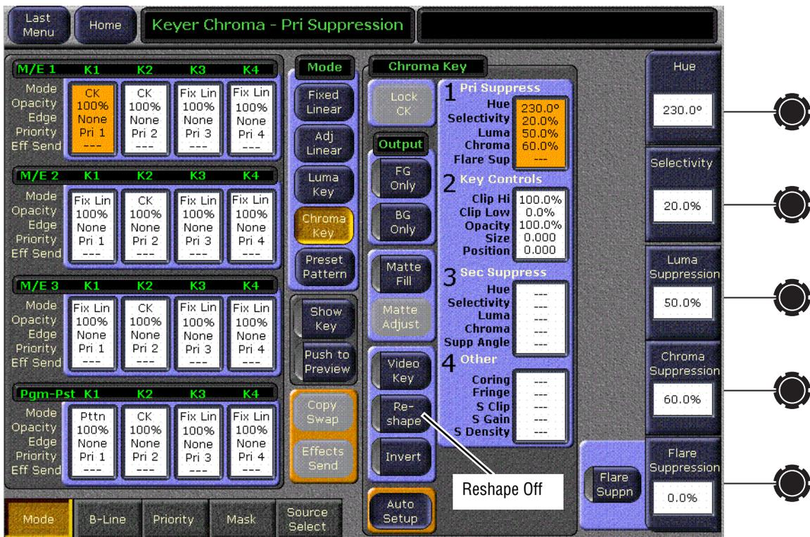
6. Press the **Auto Setup** button on the Main panel. Preview for that M/E will now display the chroma key source with a superimposed cursor. The cursor actually represents a box of 16 x 16 pixels.
