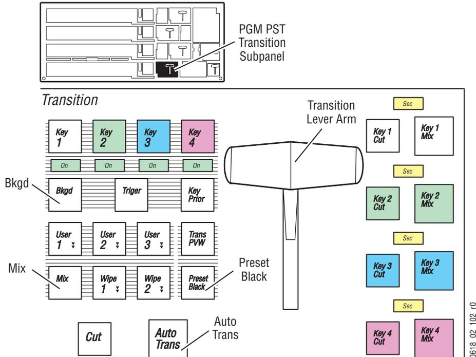
4. Move the PGM PST lever arm slowly from one limit to the other, observing the Program monitor. The picture will mix from <Src 1> to <Src 2>, and at the end of the transition the bus will flip flop.
