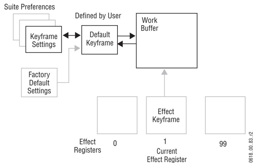
The operator can define exactly what these default settings should be (Suite Preference), and these settings can be stored and reused to meet varying requirements. A separate set of factory default settings also exist that cannot be changed, but may be loaded to the Default Keyframe and then to the work buffer, typically for system test and initial system installation.
