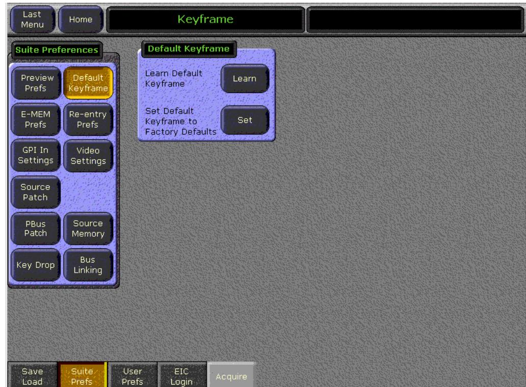
2. Touch the **Set** button. This applies factory settings to the current Default Keyframe. Existing settings will be lost (unless previously saved to disk). The factory default settings will later be applied to the Kalypso system's operating state using the **Clear WkBfr** button.
