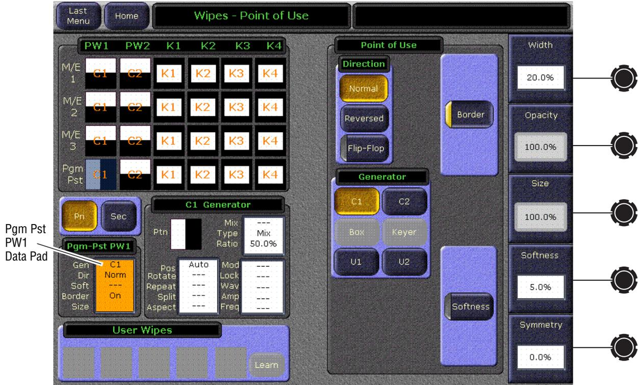
10. Touch the **Softness** button on the lower right, and then touch the Softness data pad just above it to the right. Enter a value of **5** on the pop up keypad and then touch **Enter**. This softens the wipe edge to exactly that amount.
