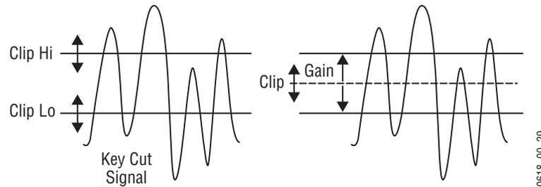
In this mode, Gain changes when either control is adjusted. The difference between the upper and lower keying thresholds is equivalent to gain:
