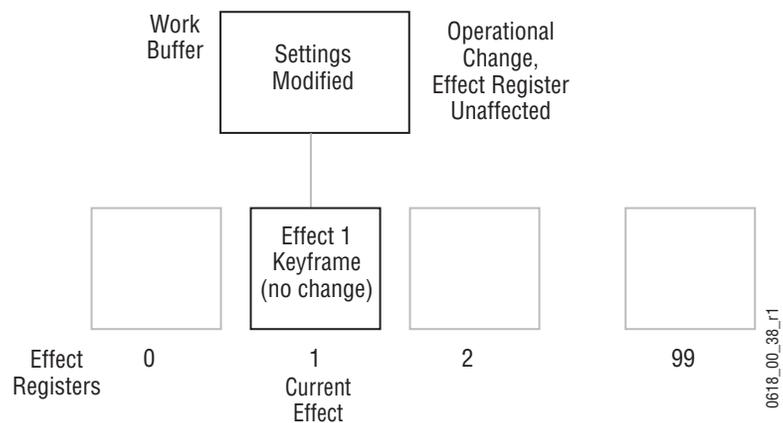
When an effect is learned, the current operational settings in the work buffer are loaded into the specified effect register, overwriting any information that was in that register. If a register different from the current effect is learned, the information is loaded into it and that register becomes the current effect. In this case the original effect register will not be altered, and can be instantly recalled to return the system to its earlier state (Figure 72).
