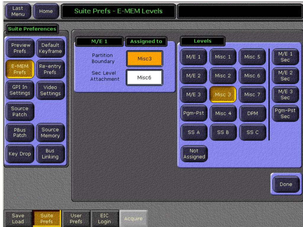
Touching the Partition Boundary or Sec Level Attachment data pad and then touching one of the Level buttons assigns that element to that level.
