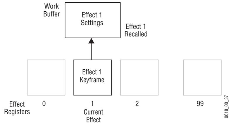
The work buffer actually holds a copy of some of the effect register information. When an operator changes a control setting manually, the work buffer settings change but the effect register data itself remains unaltered (Figure 71).
