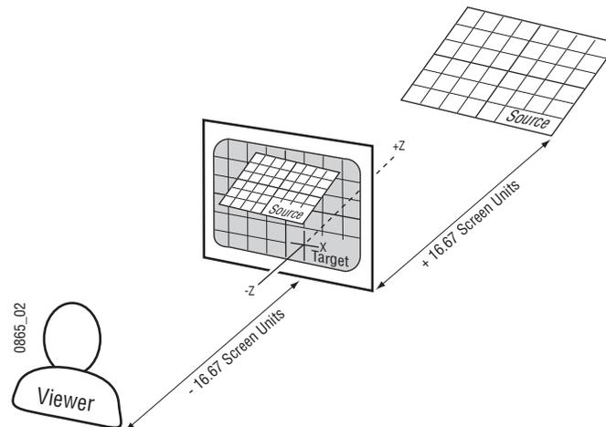
For perspective calculations the factory default viewpoint places the viewer -16.67 screen units from the monitor screen surface (4 x 3 aspect ratio). In this case, moving a full screen image 16.67 screen units back behind the screen makes the picture appear half its normal size to the viewer.
