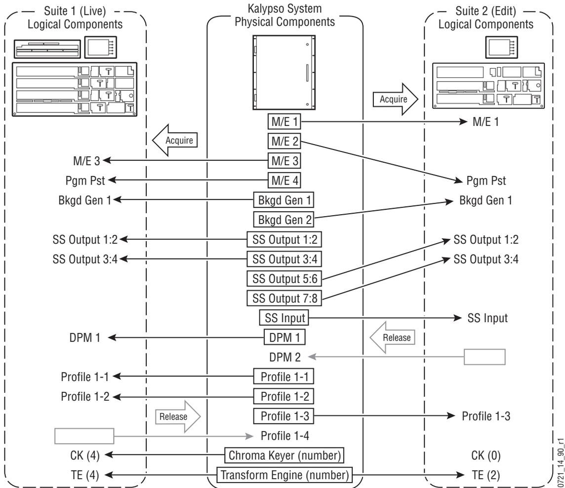
When a suite acquires a physical resource (like an M/E) it uses that resource logically. For example, the M/E 2 physical resource can be used as a logical PGM PST bank. Each of the two switchers created can therefore
