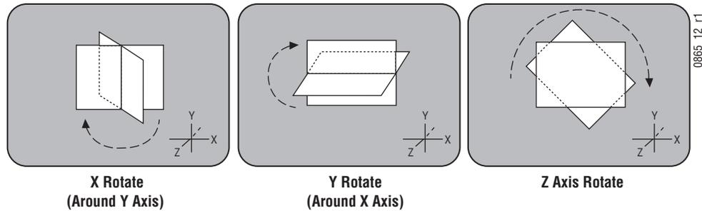
**Spin** — Supports multiple rotations about the reference axis in the X, Y, and Z directions. Spin supports fractional values, and is similar to Rotate when the move is less than  $\pm$ . one half revolution. Spin uses Euler math to calculate the move, which is not quite as precise as Quaternion, but permits multiple rotations. Spin applies transform values in Z, X, Y order, so editing effects in this axis order provides the best control of the effect.
