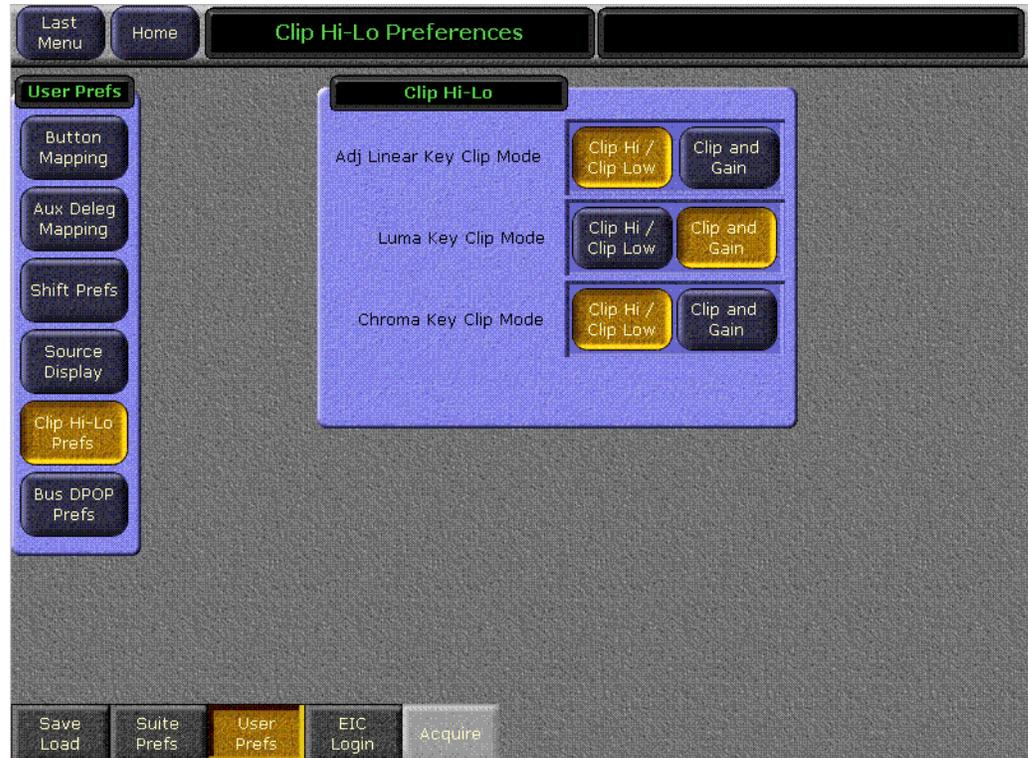
6. Set the **Adj Linear Key** and **Chroma Key** clip modes to Clip Hi/Clip Low, and set the Luma Key clip mode to Clip and Gain, as shown in the figure.
