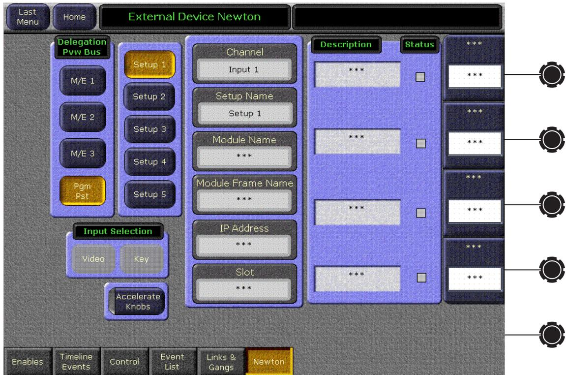
Selection of a module parameter to control is mediated through the Kalypso source selection mechanism. By selecting a source on the currently delegated Preview bus of the Kalypso's Main panel, the source's physical input, and that input's associated Newton channel controls are activated on the Kalypso's External Device menu.
