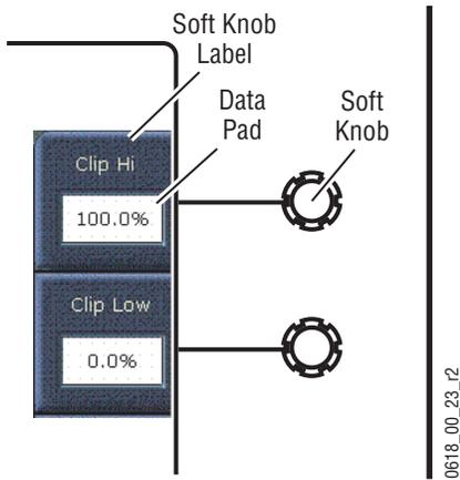
Knobs along the right side of the Menu panel can be used to dial in parameter values for functions displayed on the touch screen. When a knob is active, the touch screen displays the parameter name and its current value on a data pad (Figure 111). The parameter can be adjusted by turning the knob, or the data pad can be touched to bring up a numeric keypad.
