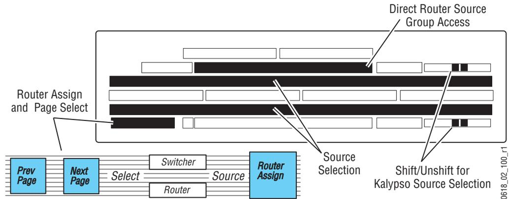
The **Router Assign** button on the Local Aux panel places that panel in Router Assign mode. All Aux Bus selection capabilities are disabled, replaced with router interface functions, and the button flashes to indicate this state. The Router light pipe also illuminates to show the current mode. Pressing **Router Assign** a second time exits Router Assign mode.
