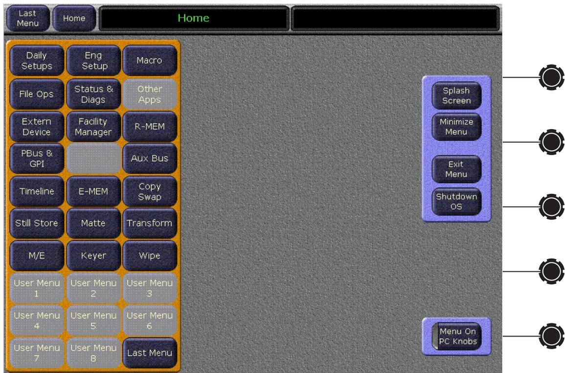
The original Menu panel also has hard buttons on the left side that correspond to the soft buttons on the Home menu. The hard button for the currently displayed menu will be high tally.
