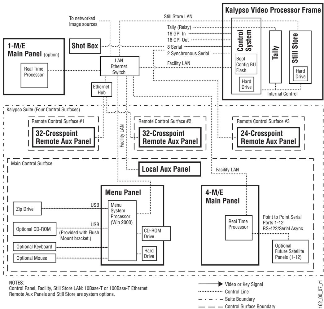
Late model 2-M/E Kalypso system control is the same as the 4-M/E Kalypso system, except the Local Aux panel is built into the 2-M/E Main panel (Figure 43).
