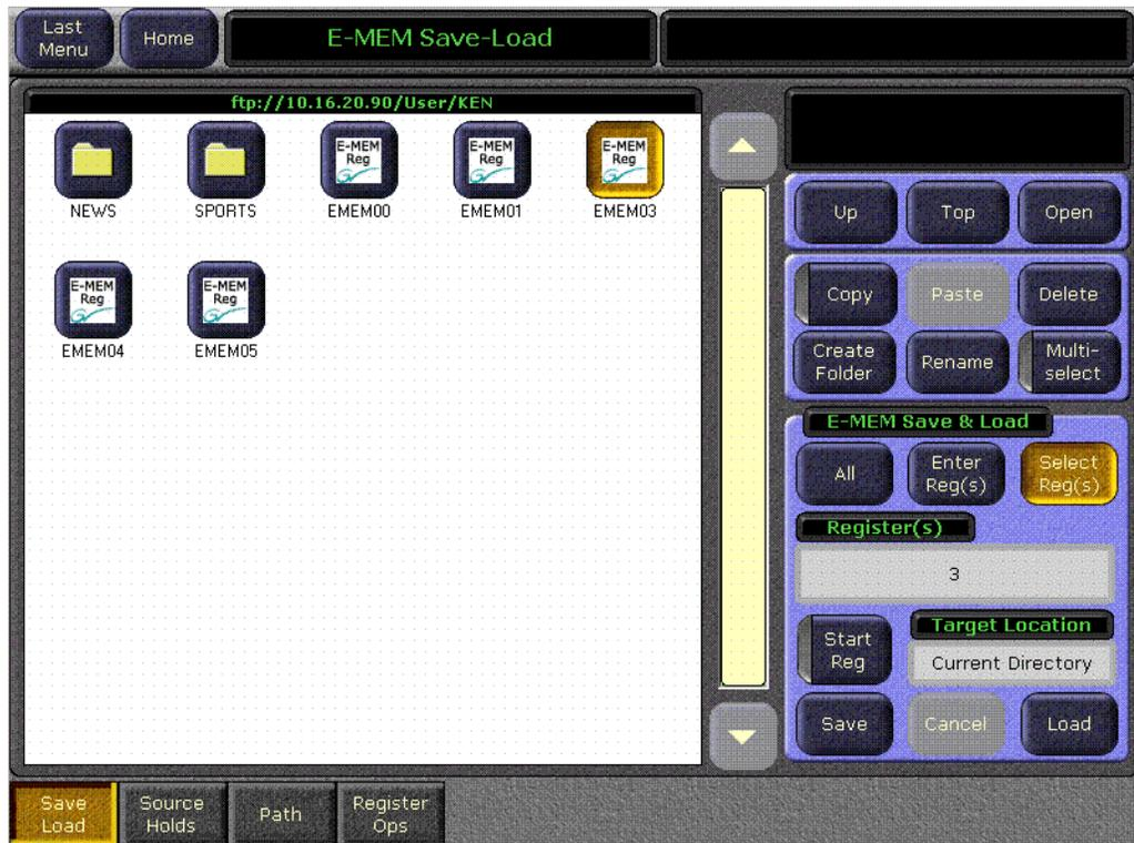
Saving and loading E-MEMs is similar to the file operations described above, except you can choose to save or load all the current E-MEMs, a range of E-MEMs, or a single E-MEM file.
