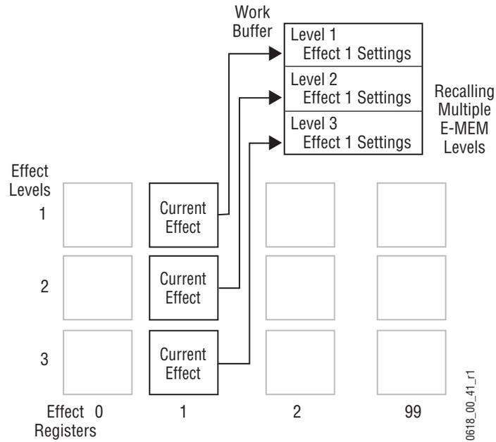
If only one effect level is selected for a recall, the resulting change is only applied to its level in the work buffer. The other levels of the work buffer remain unaltered. Note that this makes it possible to have current effects from different registers, also called a *skewed effect* (Figure 78).
