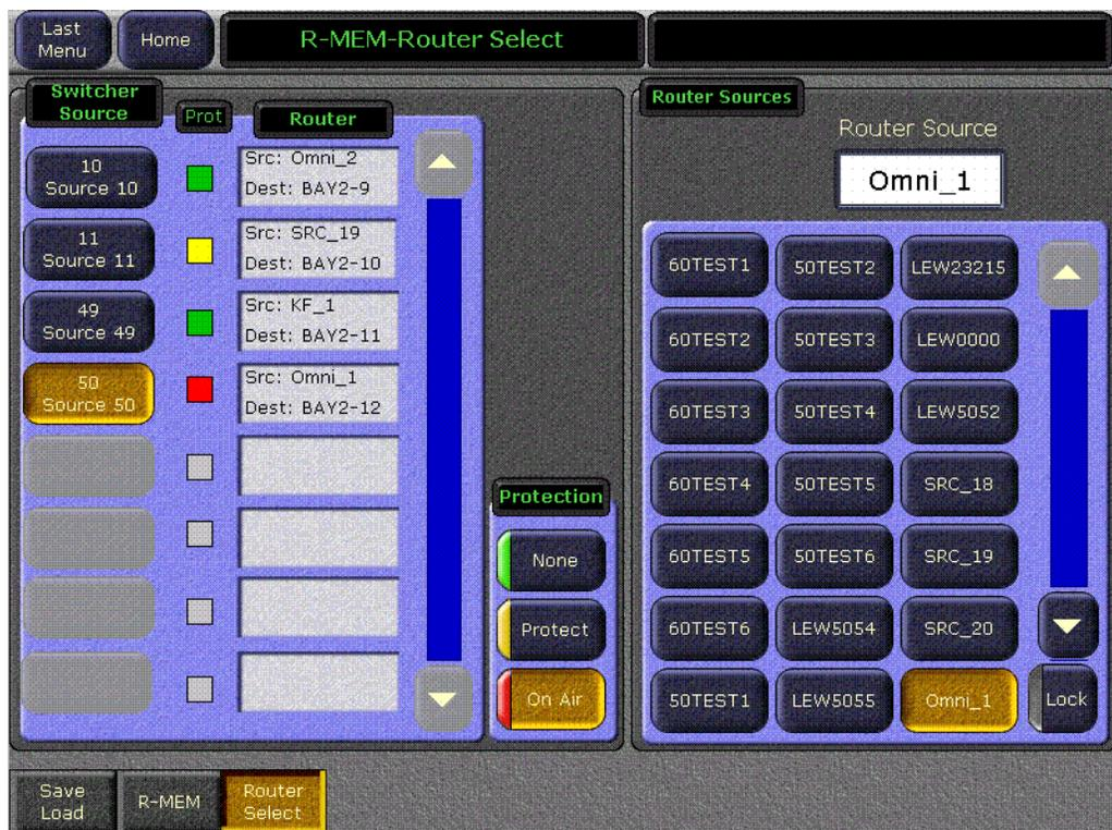
The Switcher Source pane on the left is a scrolling list of switcher sources (only sources configured as routed Kalypso sources appear). Each button displays the Switcher Source ID number and source name.
