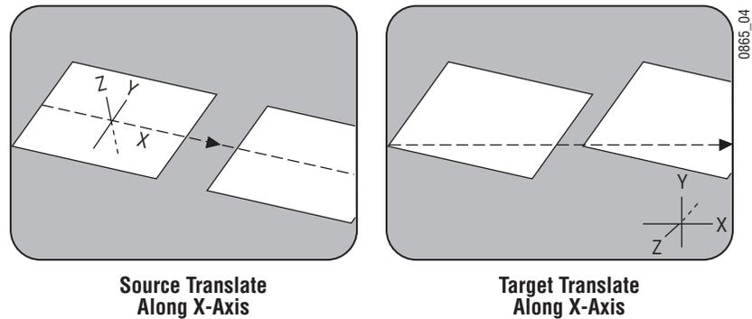
If the channel is controlled by a global channel, and the global channel itself has been rotated, an X axis translation will depend on whether the channel itself or the global channel is being manipulated, and whether source or target space is being used (Figure 91 and Figure 92). Note that the target translate of the channel is the same as a source translate of the global channel.
