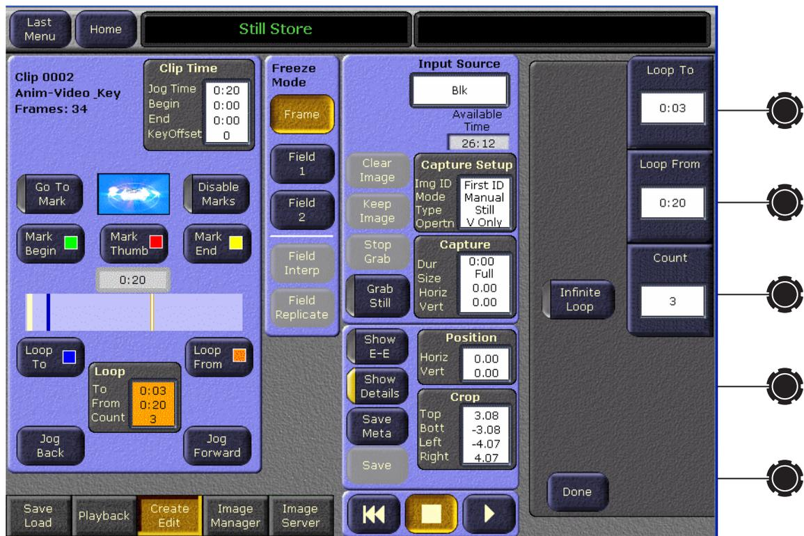
2. Using the **Jog Time** soft knob or the **Jog Forward** and **Jog Back** buttons, go to the first frame to be looped and press **Loop To**.
