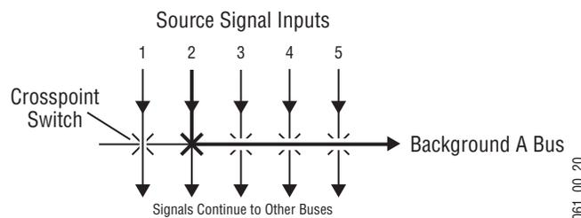
Buttons on a control panel can be used to control the switching of crosspoints. The buttons are usually arranged horizontally, making it easy to imagine the available signals coming in from the top, and the single bus output signal going out the right side.
