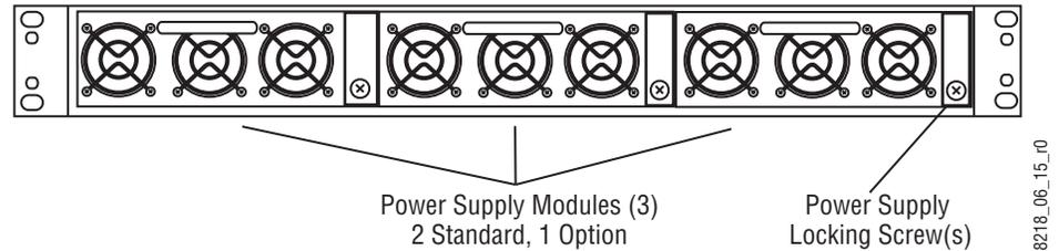
Power connectors are located on the rear of the Video Processor Power Supply (Figure 38), including a special connector for feeding power to the Video Processor. Each module has its own power connection. Though not required, we recommend each module be plugged into a separate AC circuit.
