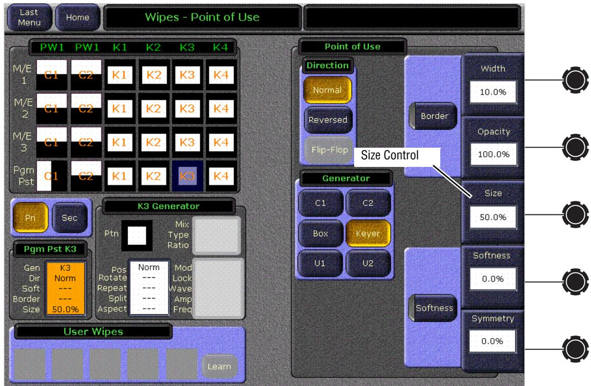
9. Touch the **Size** soft knob data pad (Figure 266) and enter 25% in the pop up keypad. Alternatively, you can use the soft knob to adjust the size of the preset pattern. Make it relatively small, suitable for over the shoulder use.
