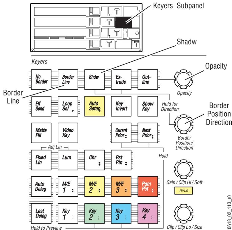
5. Turn the **Border/Position/Direction** knob in the Keyers subpanel to change the size of the border. Key borders have a limited size. Make the border as large as possible.
