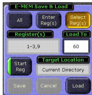
5. The **Load To** data pad. A Register range keypad appears ([Figure 142](#)).
