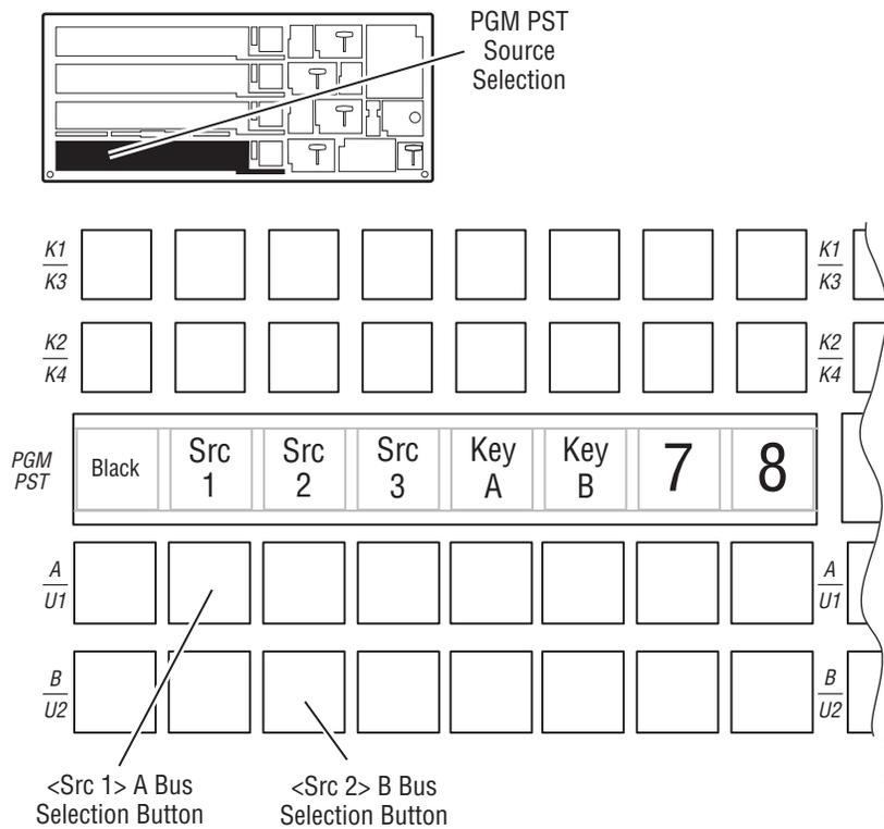
When the source select button is pressed, that source instantly appears on the program monitor, and its source button goes high tally, indi-
