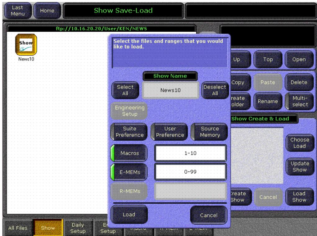
The controls in this pane operate the same as the Create Show, except the **Load** button replaces the Create button.
