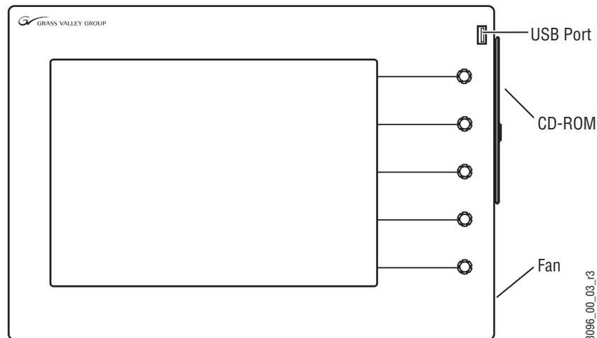
Ports located on the rear of the Menu panel (Figure 9) provide connections to the Main panel, Video Processor frame, an external Zip drive, a PS/2 mouse and keyboard, and other devices.
