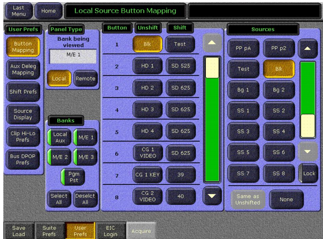
The **Panel Type** delegation buttons are used to select the device to be mapped.
