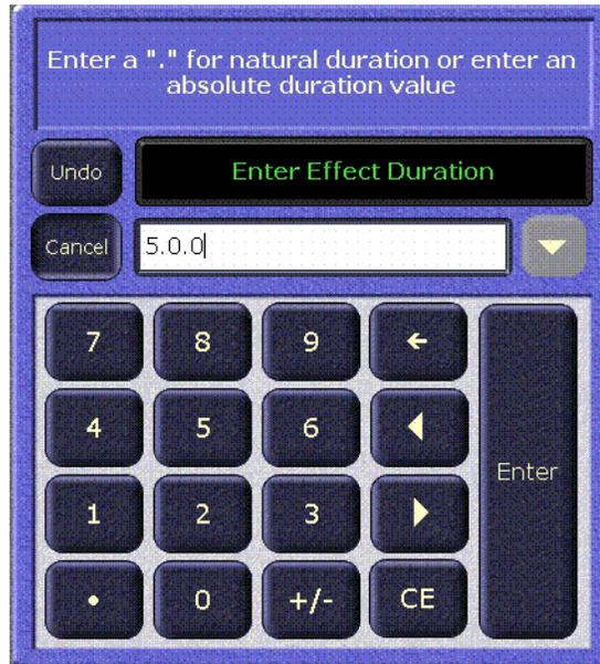
4. Type a new duration in Seconds • Frames • Field format and touch **Enter**.
