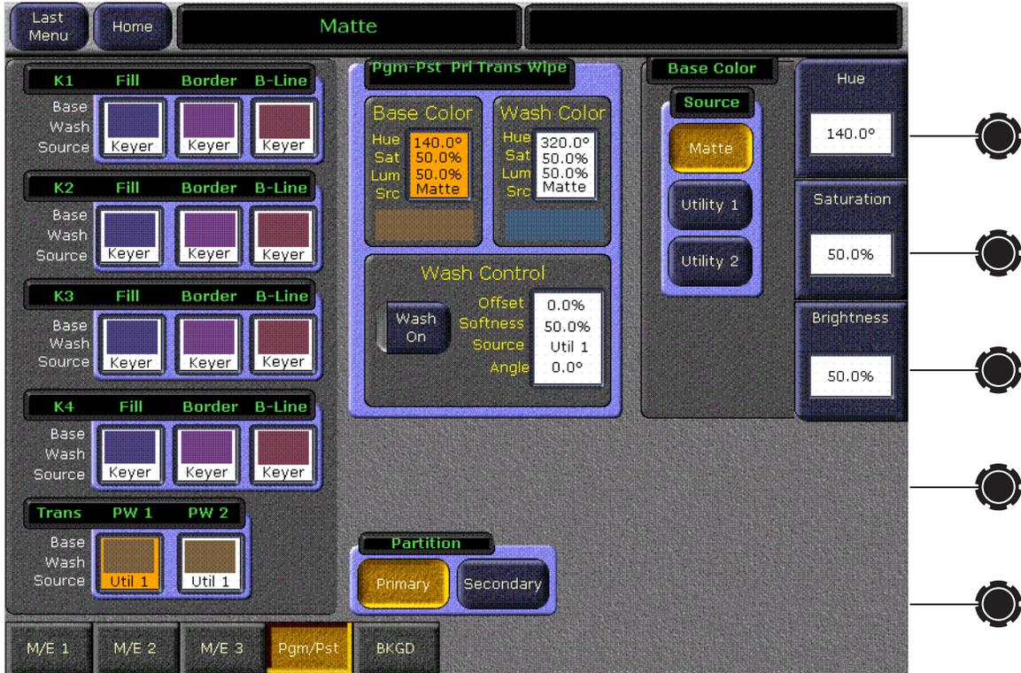
14. Move the transition lever arm in the same direction as before to complete the Transition Preview (the Trans PVW button will go off). Now press the **Auto Trans** button to see the transition with the matte border.
