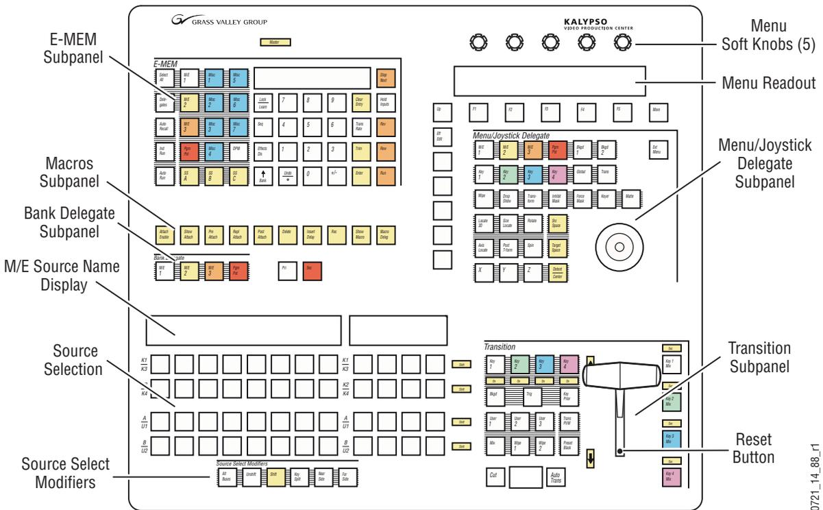
The 1-M/E Main panel's top lid is held closed with screws and is not designed to be opened by the operator. No user controls or field serviceable parts reside in the unit.
