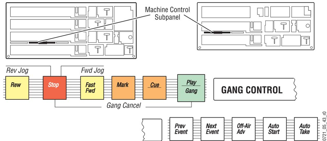
Once a group of devices has been selected, the Machine Control subpanel controls (Figure 182) apply to the entire group. The display reports GANG CONTROL to indicate this special operating mode. The basic transport controls (Stop, Play, Rew, Fast Fwd, Forward Jog, Reverse Jog, Mark, and Cue) are operational in Gang Roll mode.
