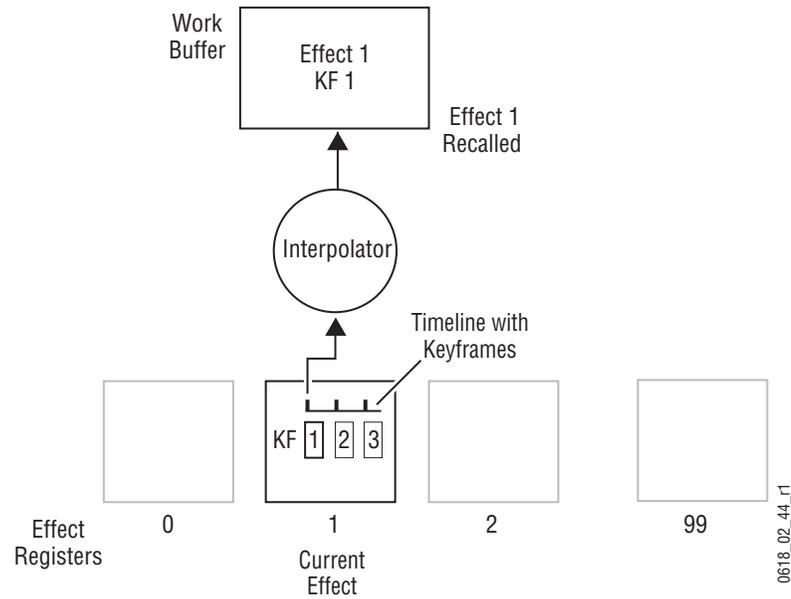
The only difference between a single and multiple keyframe effect is a multiple keyframe effect can be run after it has been recalled. Running an effect changes the state of the system from keyframe to keyframe. During the effect run the values between the keyframes are usually interpolated (Figure 74).
