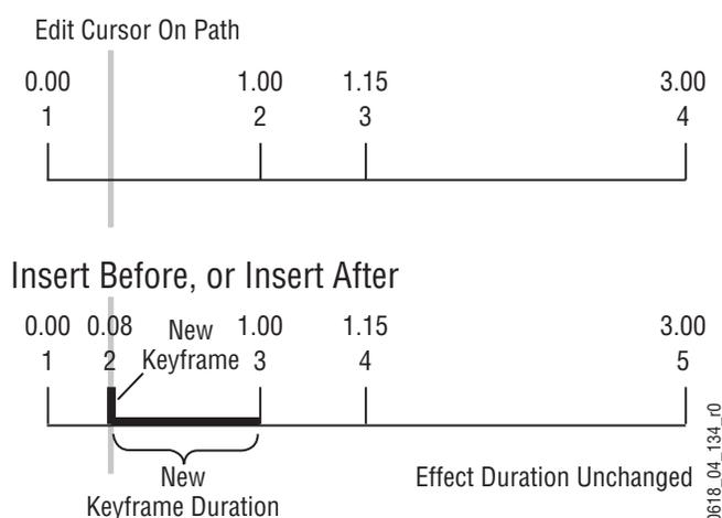
Note that after inserting on the path, the preceding keyframe's duration is shortened and the new keyframe's duration extends to the next keyframe. When keyframes are inserted on the path the overall effect duration does not change.
