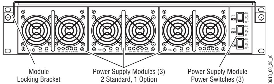
Though not required, we recommend each module be plugged into a separate AC circuit.
