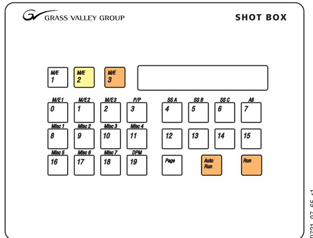
The Shot box operates with Release 5.0 and higher software versions using the Editor protocol.
