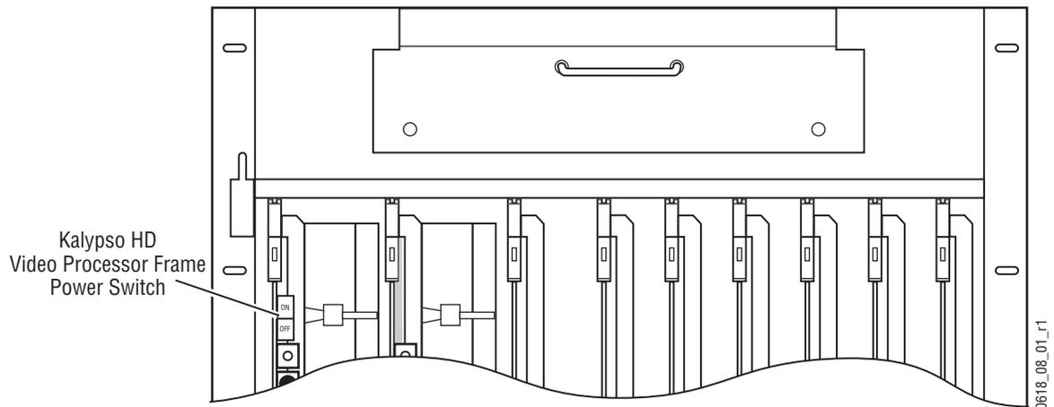
**CAUTION** The front door of the Kalypso Video Processor must remain closed during normal system operation for proper cooling airflow.
