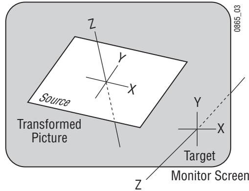
In this example the source space for the channel is referenced to the picture itself (tilted back at an angle) while the target space is referenced to the monitor screen (straight). X axis translations will move this picture differently, depending on whether source or target space is being used (Figure 90).
