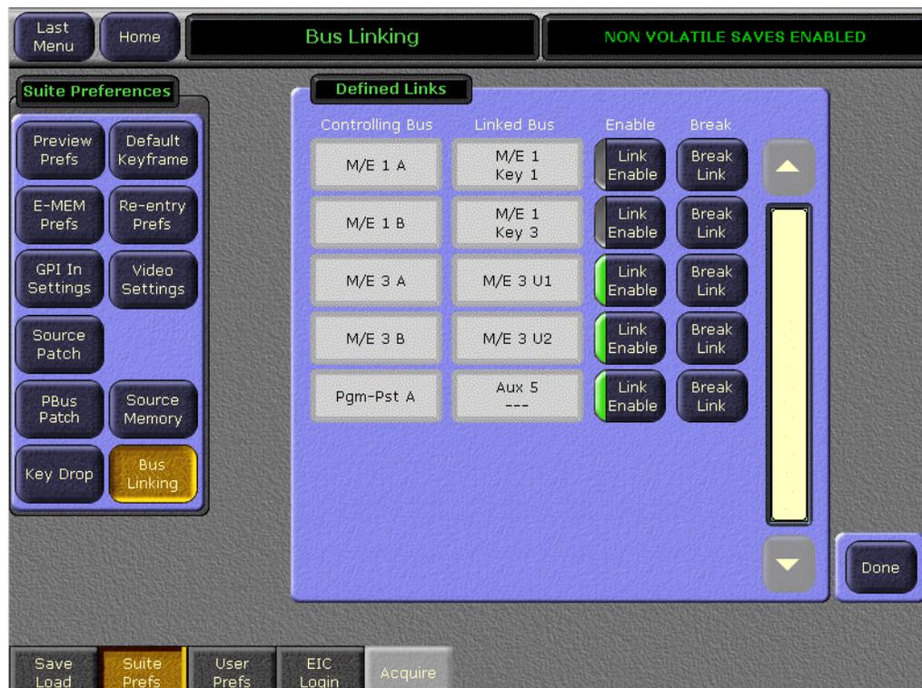
**Link Enable** – Enables the bus link, same as the Controlling bus **Link Enable** on the Bus Linking menu.
