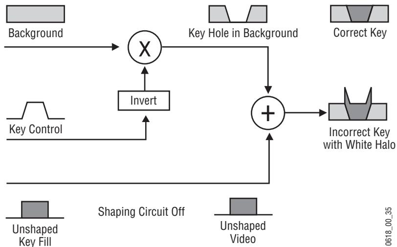
Recognizing the appearance of improperly shaped video helps you know how to correct the problem should it occur.
