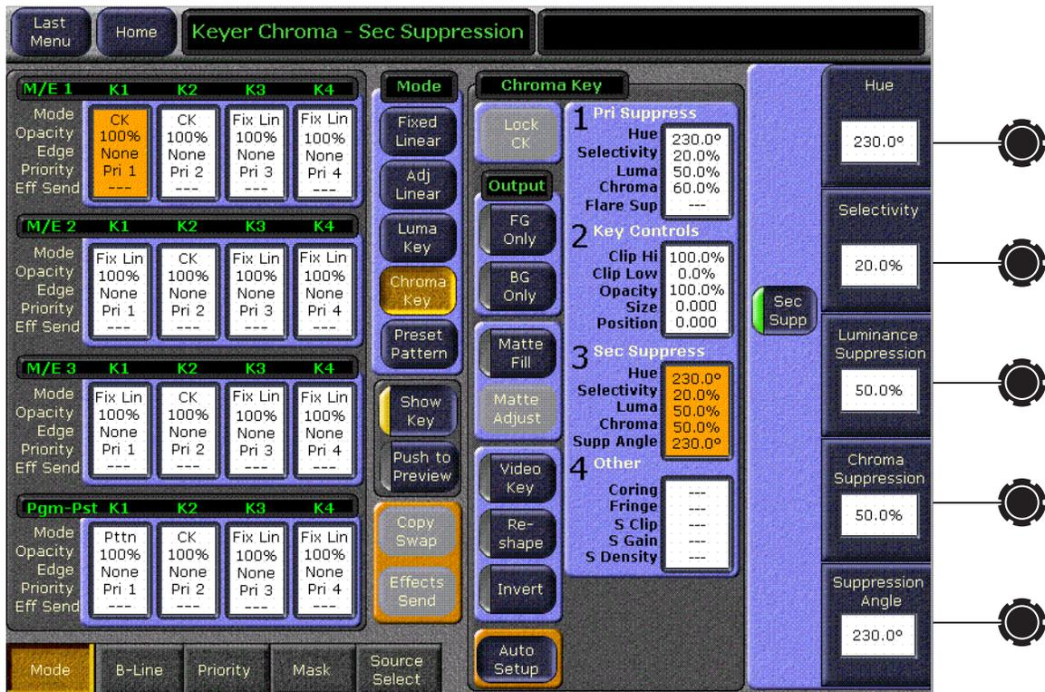
2. Adjust secondary suppression **Hue** and **Selectivity** so that the translucent area is affected, but opaque areas of the foreground are not. The final hue will lie somewhere between the backing color (primary suppression hue) and the uncorrupted foreground color.
