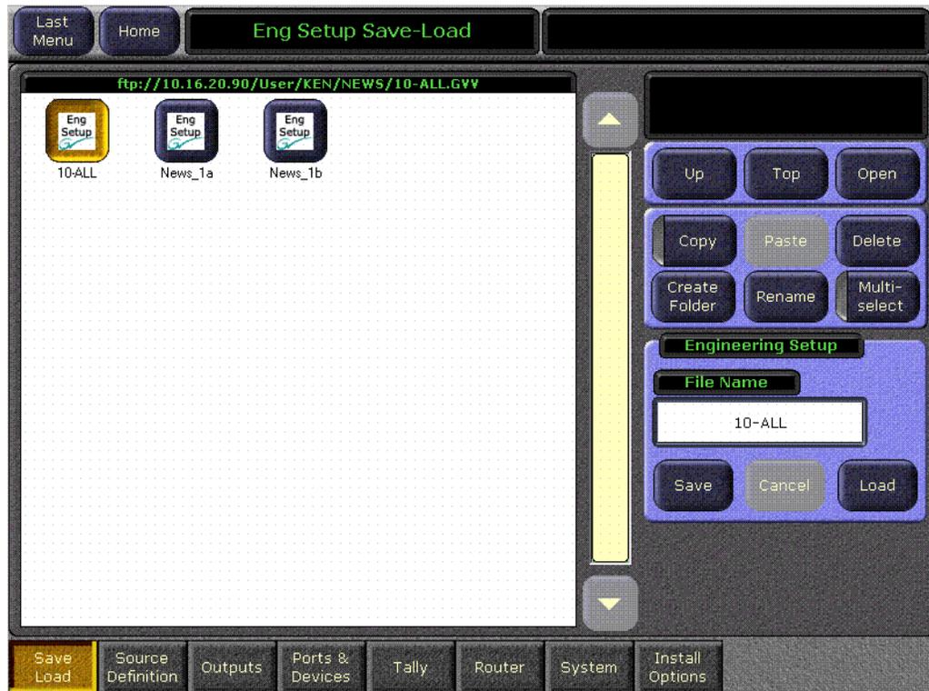
The Eng Setups Save-Load menu is similar to the Daily Setups Save-Load menu (page 164) and operates in the same way, except there is only one type of Engineering Setup file.
