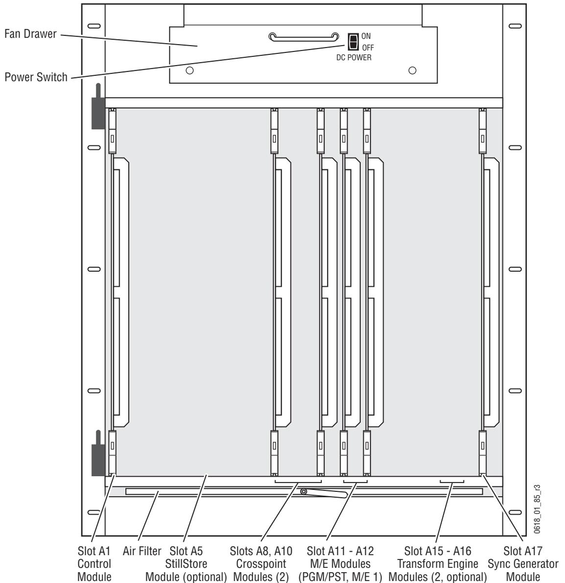
**CAUTION** The front door of the Kalypso Video Processor must remain closed during normal system operation for proper cooling airflow.
