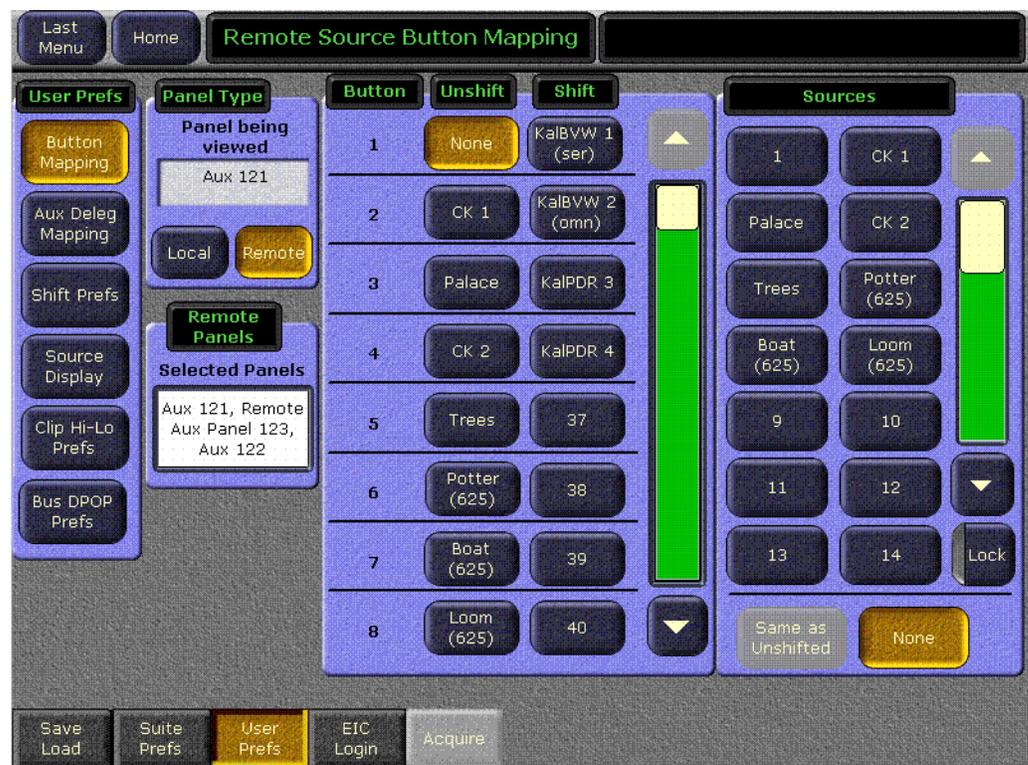
2. Touch the Remote Panels data pad to bring up a selection menu, permitting the selection of one or more Remote Aux panels (Figure 125).
