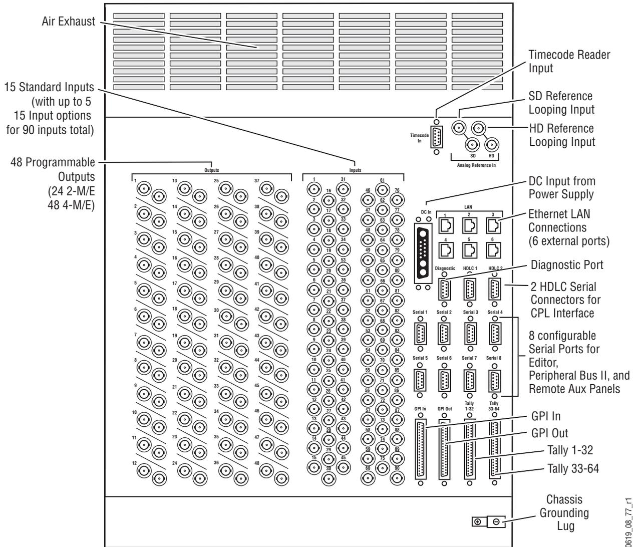
The Kalypso system has been designed for easy maintenance. All modules of the same type are identical, and can be swapped with one another. Modules can be removed and replaced safely with the power on, simplifying troubleshooting to the module level.
