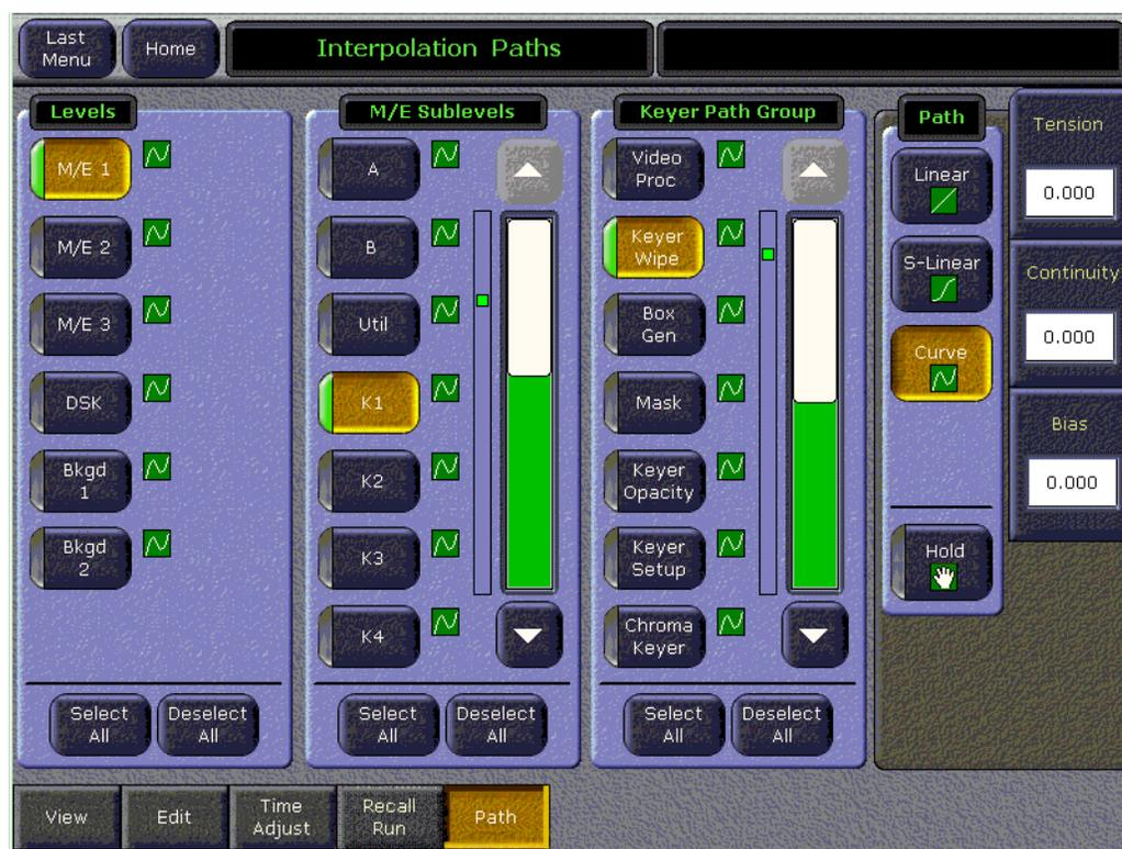
3. Choose the desired Path type (**S-Linear**, **Linear**, or **Curve**). If **Curve** is selected, you can use the soft knobs or data pads to change the values for **Tension**, **Continuity**, and **Bias**.
