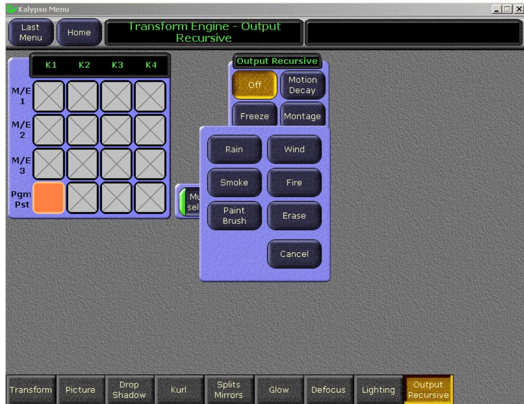
Parameters for multiple Transform Engines can be adjusted simultaneously on the Transform Engine menus, rather than having to change them separately for each Transform Engine. In addition, Effects Send for Transform Engines can be activated or deactivated directly on the Transform Engine menu by double touching their delegation buttons.
