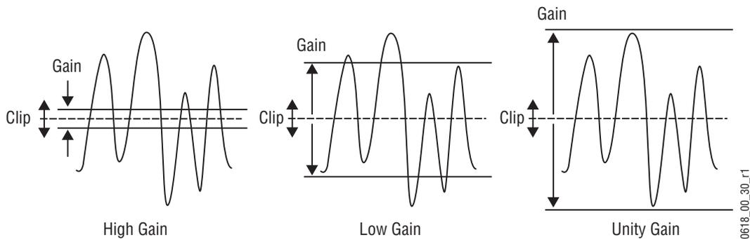
On the Kalypso system, Gain has a percentage value. A Gain value of 50% requires a luminance change of 50% of the distance between black and white to produce a keying signal ranging from transparent to opaque. A gain value of 100% (unity gain) uses the entire range between black and white for this transparent to opaque transition. A gain value of 0% produces the hard key edges (a high gain key).
