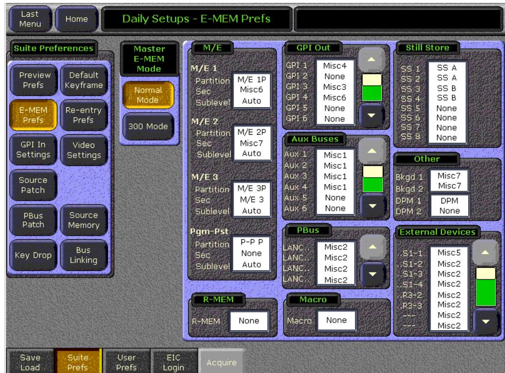
The M/E and Pgm Pst data pads display the current partition control parameters for that element. On a new Kalypso system the default settings assigns the partition boundary to the Primary partition level, and has the Secondary partition unattached (set to **None**) as shown in Figure 211.
