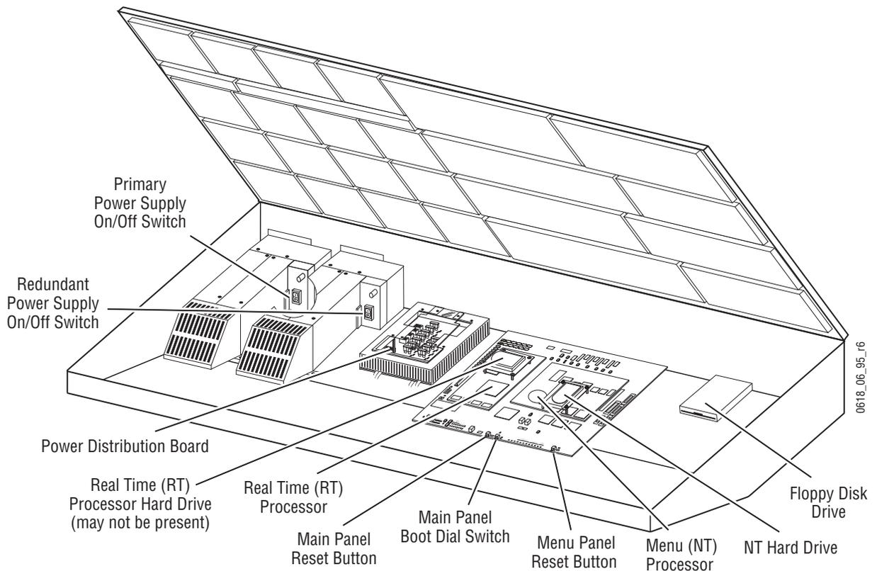
The actual type and location of equipment installed in early model Main panels varies, depending on date of manufacture. Some earlier designs used Hard Disk drives with the Real Time (RT) processor, and some used Disk on Chip hardware. Also, drives may be mounted directly on the processor boards or on separate brackets. If modified for Enhanced Menu panel operation, unnecessary hardware is removed and some rear connectors become inactive.
