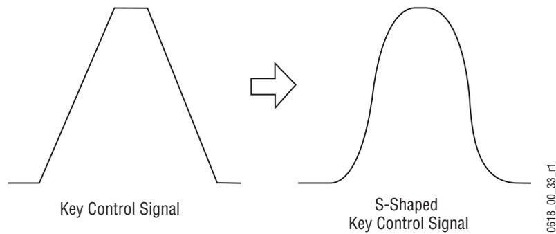
S-shaping is generally not applied to linear keys because the external device usually applies an S-shaping function when it generates the key cut and key fill signals. S-shaping should not be applied twice.
