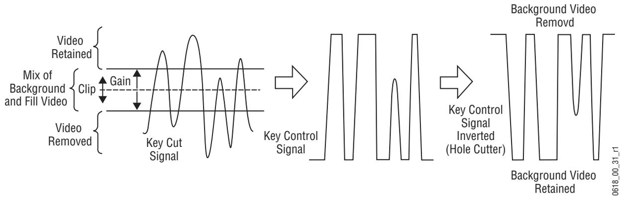
Clip and Gain control is appropriate for high gain keys (see below), to easily adjust where the relatively hard transition from background to fill occurs. In this mode, changing the Clip control moves the threshold up and down without affecting Gain, which is adjusted separately with its own Gain control.
