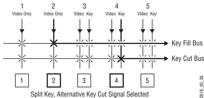
Note that if the key fill video has been shaped by an external device, this previously shaped video will not match the different key cut signal selected
