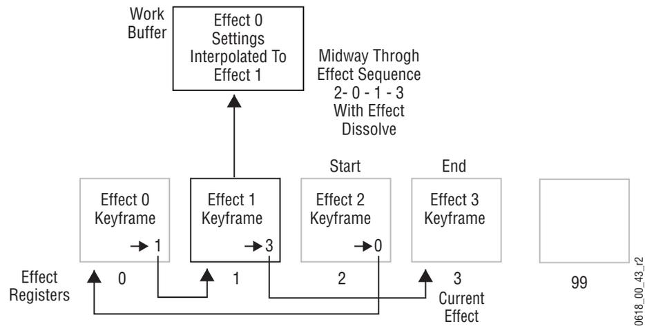
In the above example, recalling effect 2 as a sequence will proceed from register 2 to register 0 to register 1 to register 3. A sequence can begin from any of the effect registers in the sequence. For example, in the above example if register 0 is recalled, the sequence will proceed from register 0 to register 1 to register 3.
