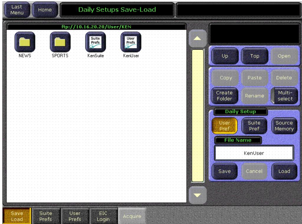
The Daily Setups Save-Load menu is similar to the File Operations All Files menu, with a file display pane on the left and some of the same navigation and action buttons on the right. An additional Save and Load pane of controls is on the lower right.
