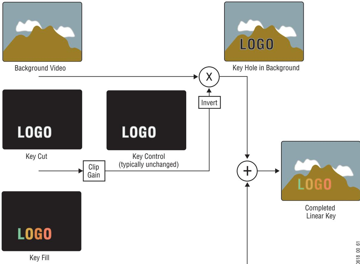
**Note** The soft edges in the illustrations in this part of the manual are simulated. The key edges are actually gradients, which allows these edges to blend smoothly with the background.
