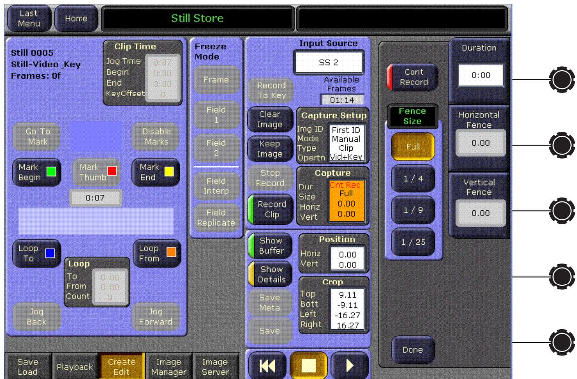
**CAUTION** Long duration recordings can uncache a lot of other Still Store material, and saving long recordings can fill the cache with locked items, making other Still Store material inaccessible.
