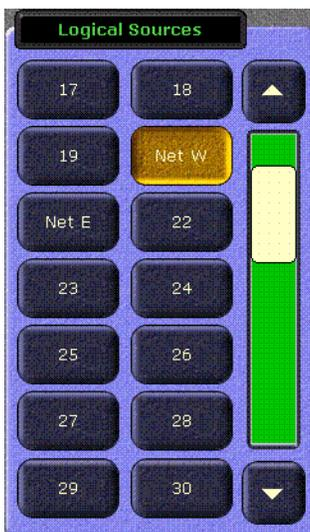
When multiple items are available for selection, scrolling lists are used (Figure 115). On most menus, touching the up and down triangle buttons scrolls the list up or down one item. When the top or bottom of the list is reached, that button goes gray. Touching the green area above or below the white handle scrolls the list up or down one group of items. You can also drag the white handle to quickly scroll through the entire list on some menus.
