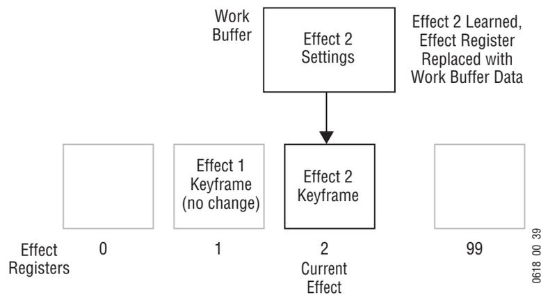
Effect registers can be locked to prevent them from being altered, and they can be saved to disk and reloaded and recalled for use at a later time.
