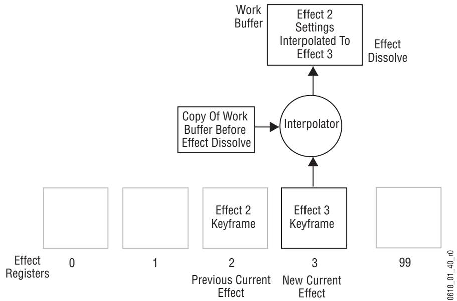
Note that the effect dissolve does not occur directly between two registers, and the transition aspect is handled separately from the interpolated parameter values. If work buffer parameter settings are changed before an effect dissolve, the current modified work buffer values (but not the source and button settings) will be smoothly interpolated to the new register values.
