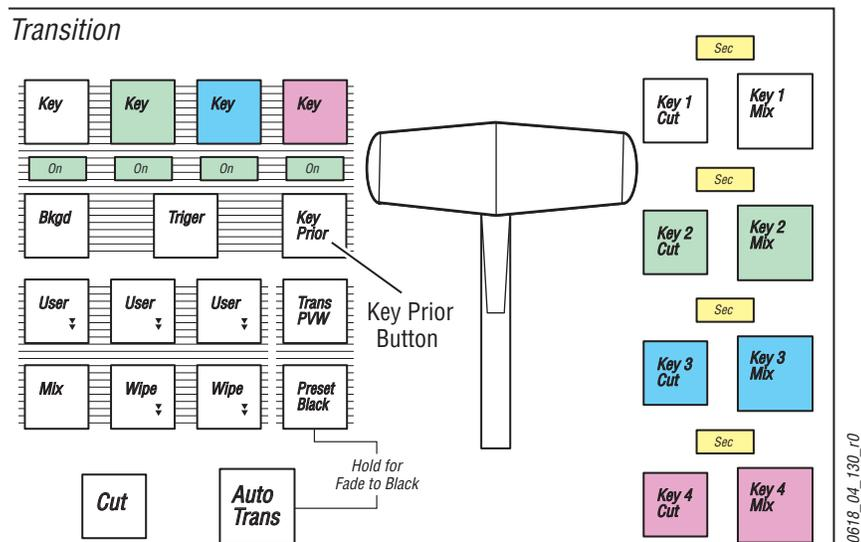
2. If not already set up, turn on the desired keys and arrange them so they overlap, observing the Program monitor. This will make the changes in key priority visible. For demonstration purposes, you can use four preset pattern keys.
