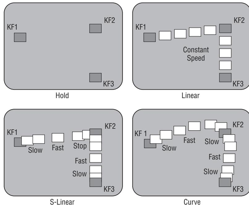
The path concept can also be applied to functions that do not move a picture across the screen, like matte hue changes. For these functions, the rate of change of the parameter follows the same path types above. For example, an S-Linear hue rotation will accelerate and decelerate the speed of the hue change at the beginning and end of the keyframe.
