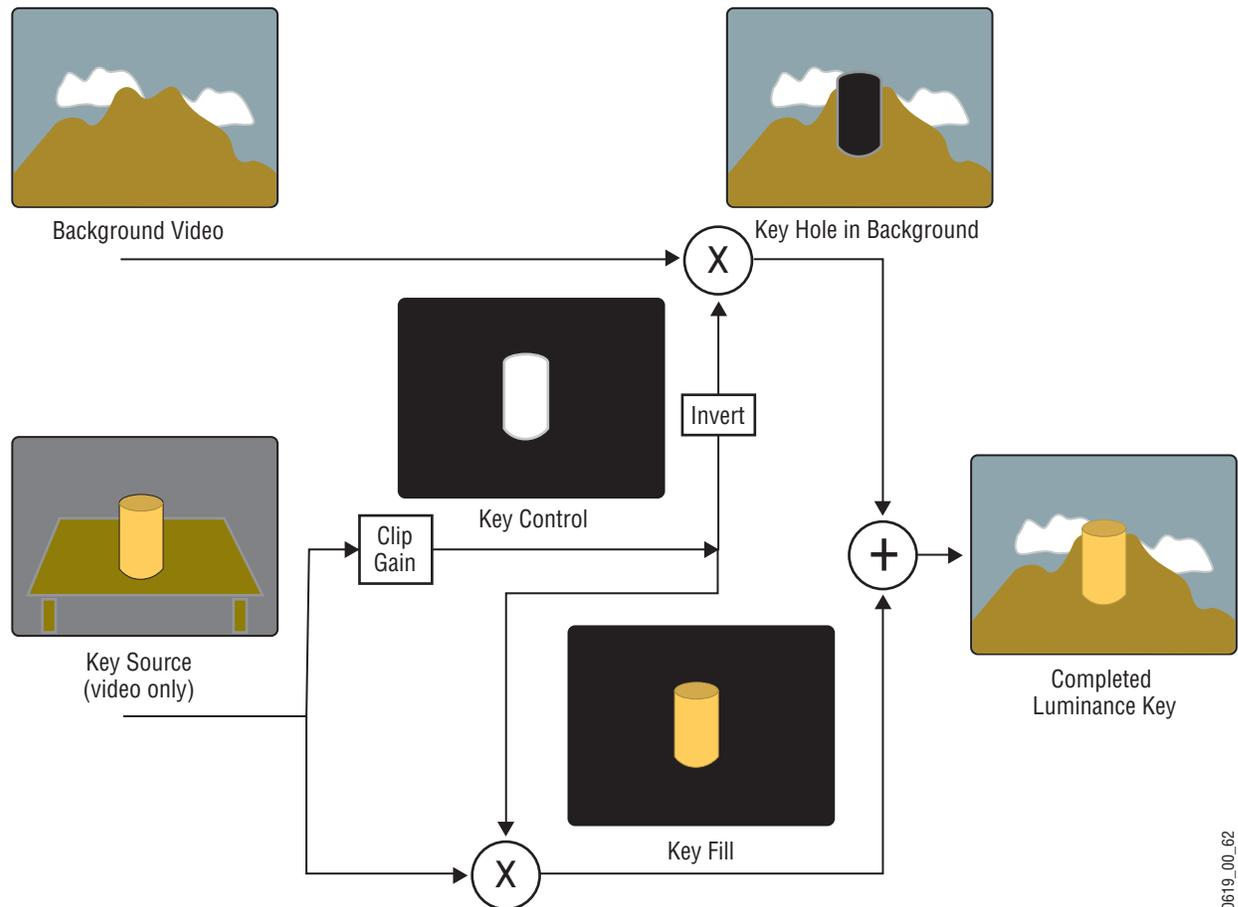
Clip and Gain (or Clip Hi/Lo) controls for luminance keys offer wide adjustment ranges. On the Kalypso system, an S-shaping function is also applied to the edges of luminance keys.
