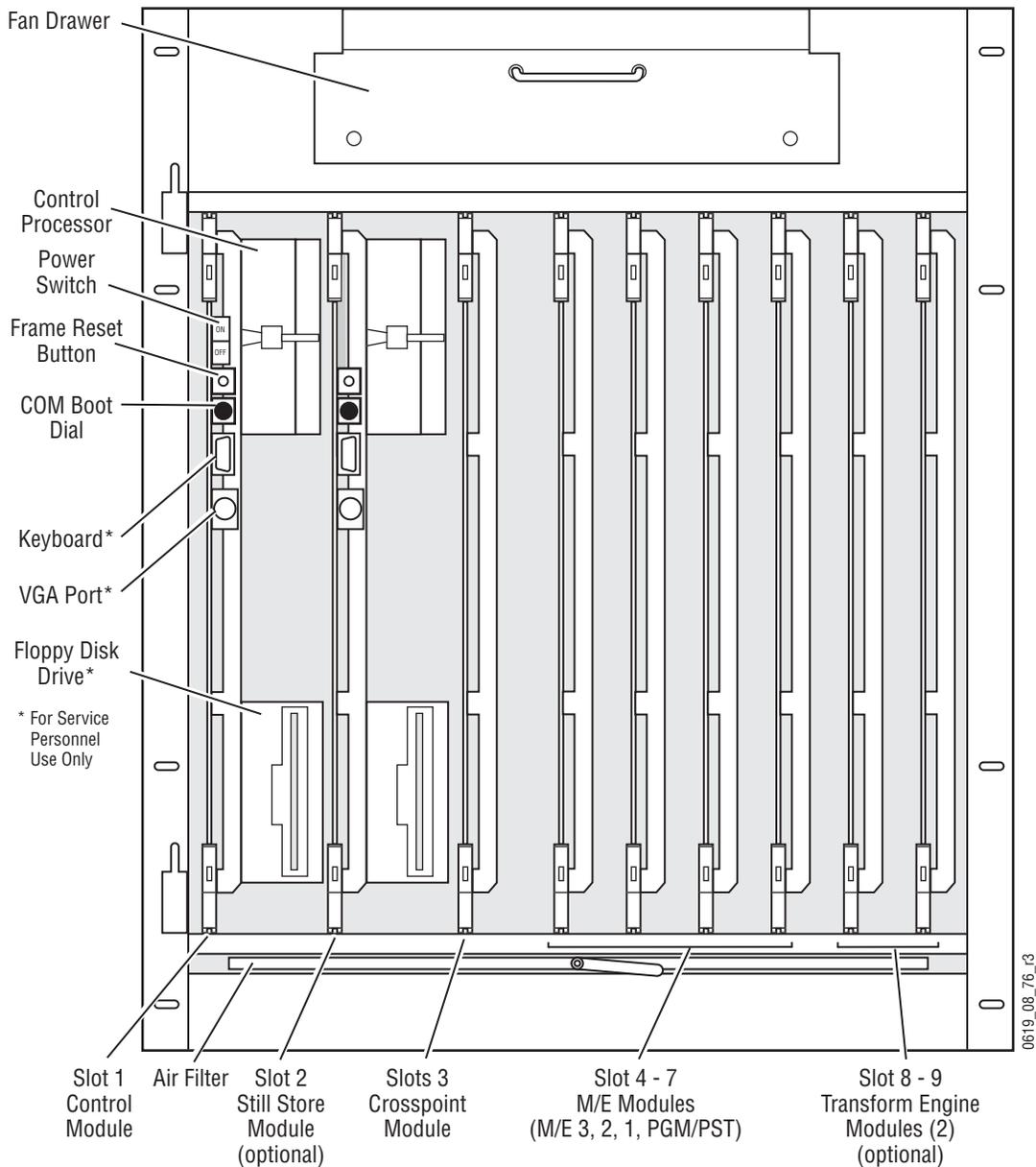
**CAUTION** The front door of the Kalypso Video Processor must remain closed during normal system operation for proper cooling airflow.
