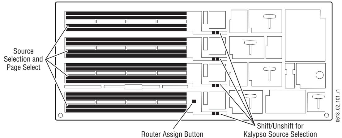
The **Router Assign** button on the Main panel is held down to place and keep the Main panel in Router Assign mode. When held down all normal panel operation is disabled, replaced with Router assign functions. Releasing the **Router Assign** button returns the Main panel to normal operation.
