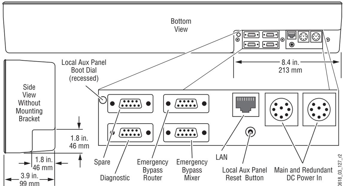
The Local Aux panel is generally installed directly above the left side of the Main panel so the Source Select buttons are aligned, though it can be mounted in any convenient location.
