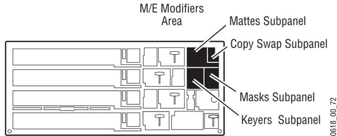
Delegation determines which M/E and keyer, or matte is being controlled at any given time by the M/E Modifiers controls. Delegation is available on the individual subpanels, via the M/E Keyer delegation buttons, and can be configured to occur automatically. See the *Kalypso User Manual* for more information on Delegation.
