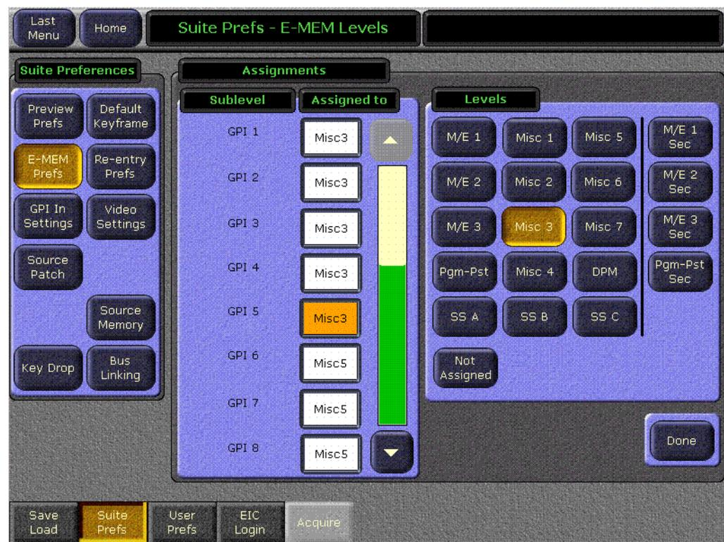
On the left individual levels can be selected for assignment (the selected level is yellow). Touching one of the E-MEM Enable buttons will assign that level to that button. Click on **Done** to return to the previous menu, from which you can access other levels to change.
