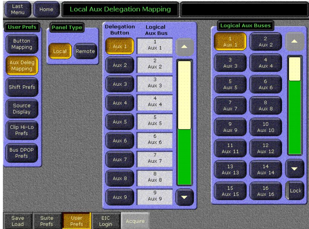
The Kalypso Local Aux panel has 13 Aux bus delegation buttons that can be used to control 13 Aux buses at a time. Multi destination Remote Aux panels also have Aux bus delegation buttons. More than 13 Aux buses are available on the Kalypso system, however. With this menu you can assign specific Aux buses to individual delegation buttons.
