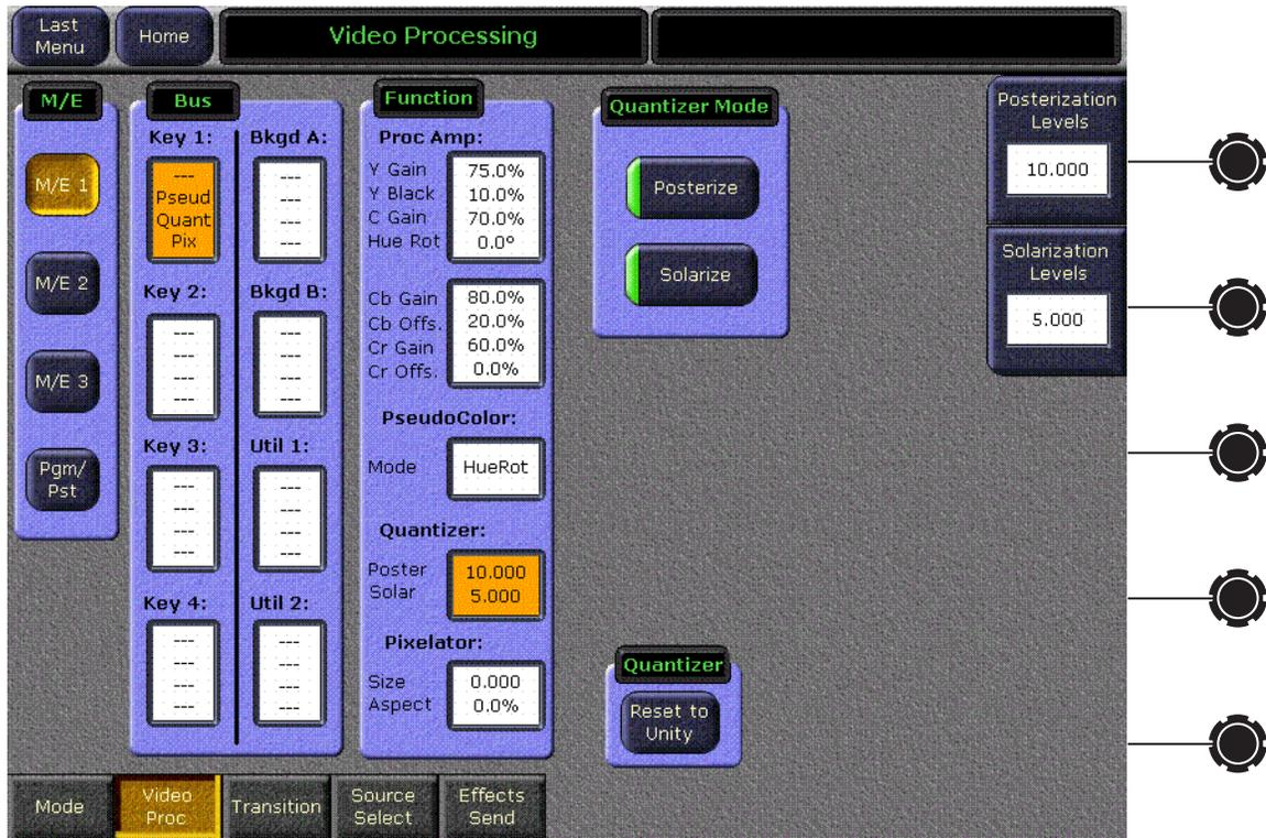
Separate on/off controls for **Solarize** and **Posterize** in the Quantizer Mode pane allow activation of any combination of the two features.
