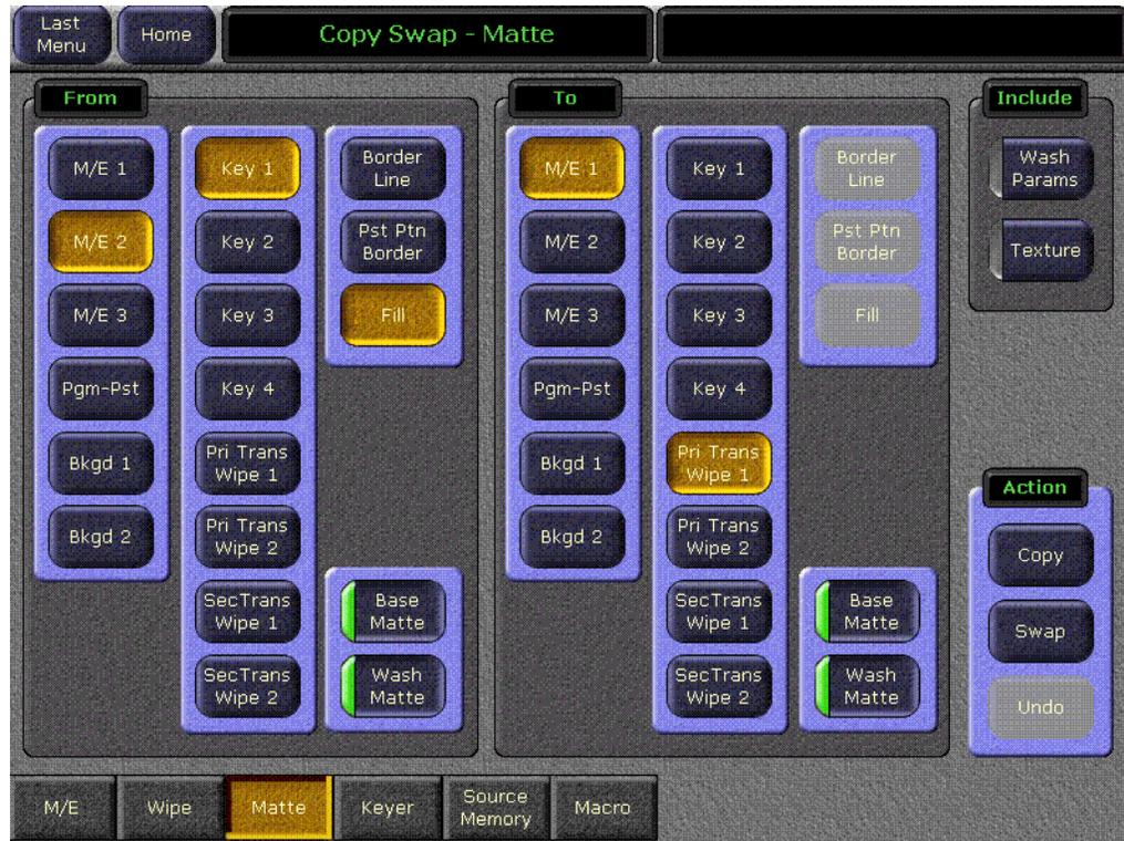
Some combinations of M/E level, Key level, and matte generator level do not exist. For example, in Figure 203, the destination matte is M/E 1's Trans Wipe. Pst Ptn Border, and Fill are grayed out because they only apply to keyer mattes. Similarly, if Bkgd 1 had been chosen, no further delegation would be needed, so all of the keyer related selections would be grayed out.
