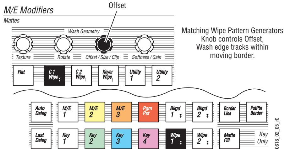
Selecting a different wash geometry gives the knob Size control, and this wash pattern will not move as the transition is performed. In Figure 63 **C2 Wipe** has been selected, though selecting **Keyer Wipe** will also gives the knob size control.
