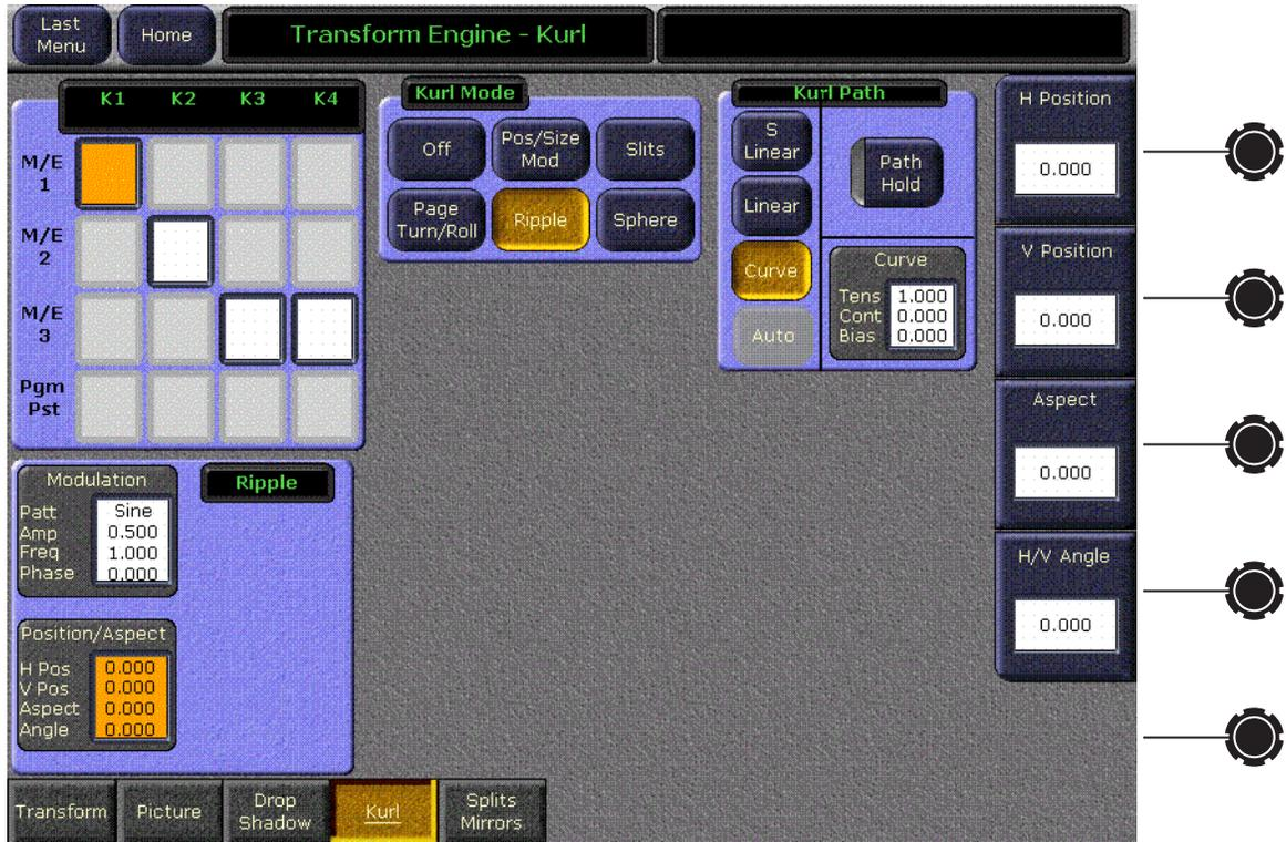
Soft knob controls are provided to control various attributes of the Ripple pattern.
