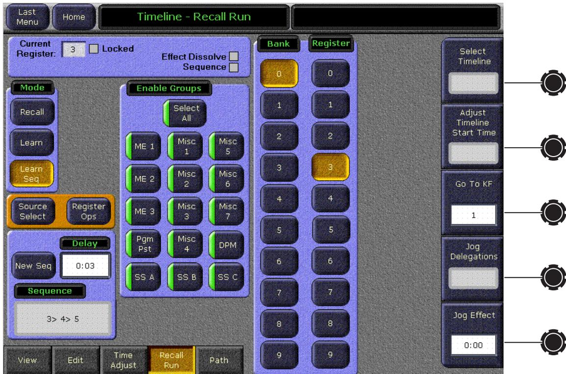
In this mode, pressing Bank and Register buttons on the right will immediately update the registers with their sequence links. The registers involved are reported in the Sequence pane below. To complete a sequence, either touch last register number a second time, or select one of the Mode buttons (Recall, Learn, or Learn Seq).
