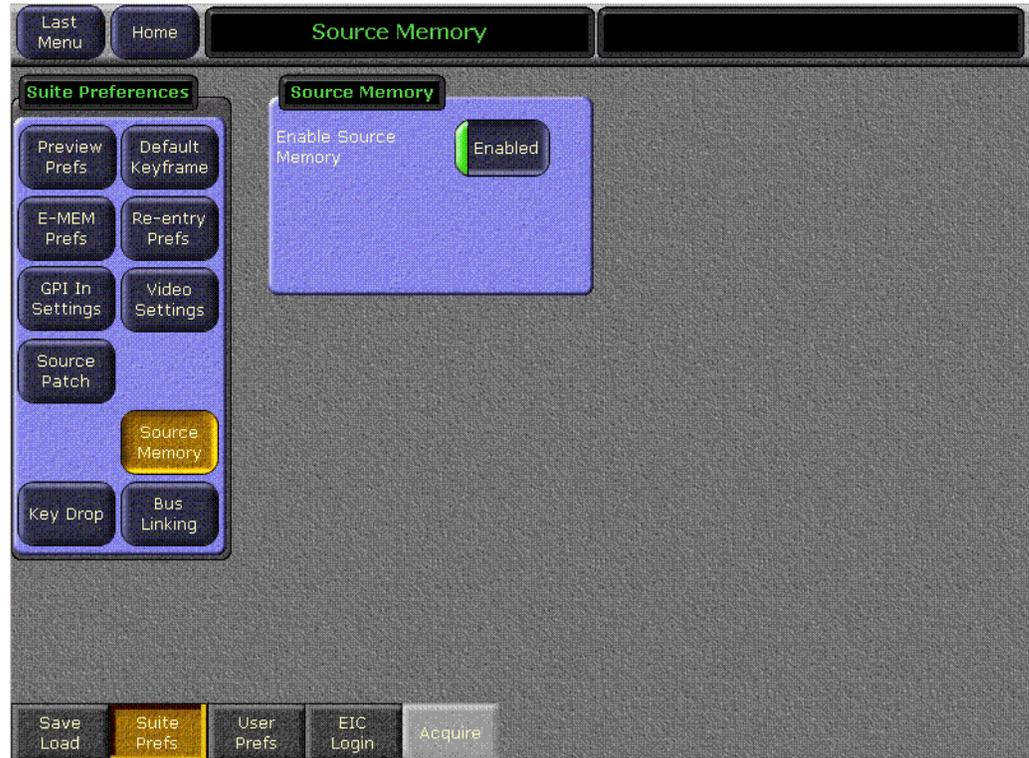
When **Enabled** (green indicator on the button is illuminated), key type and source memory settings will change as different sources are selected on that bus. When disabled (green indicator off), the current key type and source memory settings will not change when different sources are selected on that bus.
