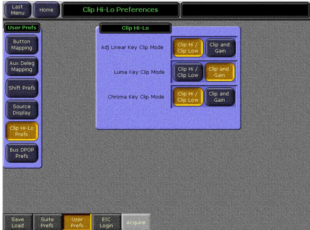
The Clip and Gain knobs on the Kalypso system Main panel and Menu panel can control either Clip and Gain, or Clip Hi and Clip Low, depending on the preference set. Different knob preferences can be applied to Adjustable Linear Keys, Luminance Keys, and Chroma Keys. The chosen settings for each key type are applied universally across the Main and Menu panels, wherever that type of key is used. Touch the button of the preference you wish to use for the listed key type.
