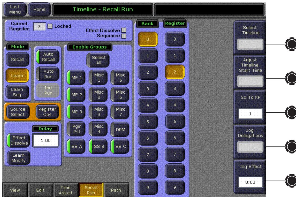
The **Effect Dissolve** button is used to specify the setting of this attribute when the register is learned.
