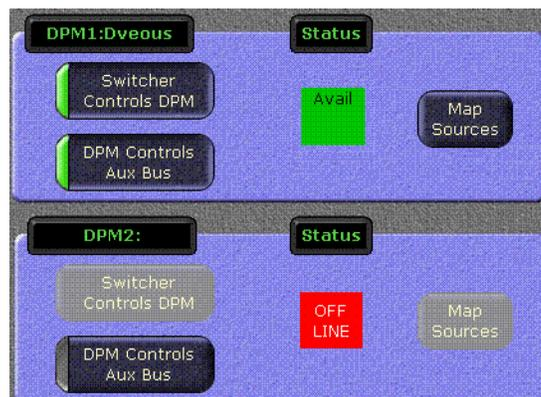
The **Switcher Controls DPM** and the **DPM Controls Aux Bus** buttons toggle on and off. The three possible combinations are:
