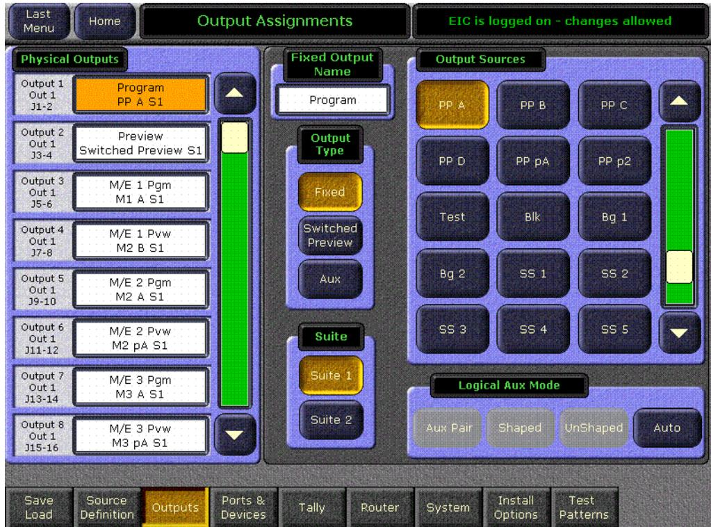
The **Suite 1** and **Suite 2** buttons are used to assign the currently selected output to a suite. The default setting is Suite 1.
