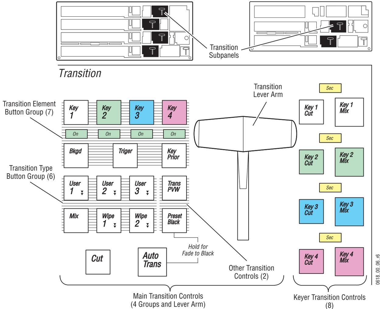
Each transition subpanel actually incorporates five transition systems. Each subpanel has one set of main transition controls, and also has individual cut and mix transition controls for each of the four keyers.
