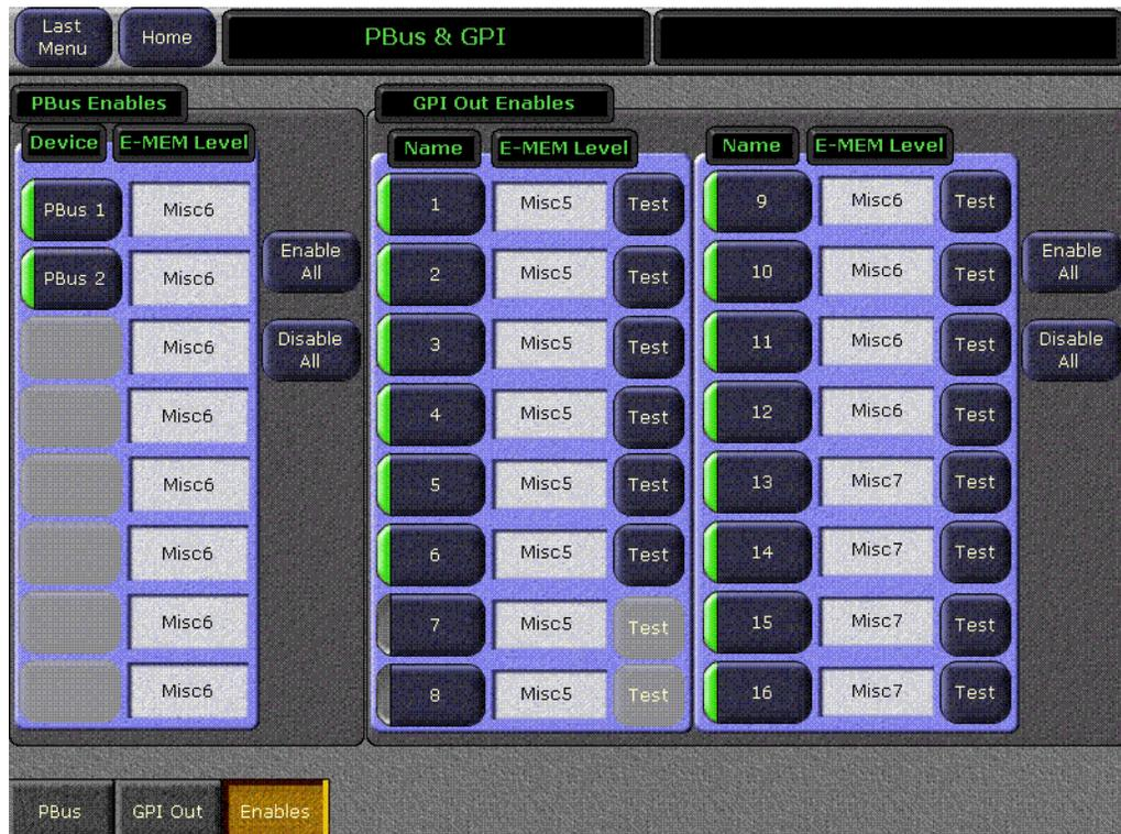
The **Enable All** and **Disable All** buttons allow enabling or disabling all enables for PBus or GPI Out.
