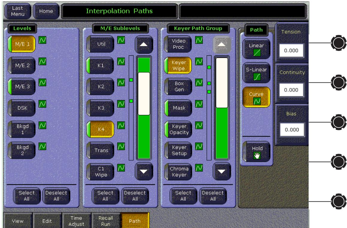
When operating in Multi-Suite mode, a special symbol with a curve and arrow is displayed if the level has not been acquired by that suite (**Bkgd 2** has this state in the illustration above).
