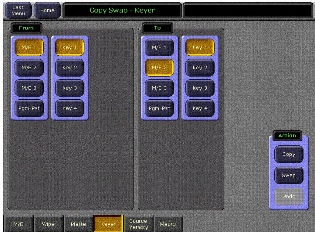
The menu enables the copying and swapping of entire keyers, including the mapping of key cutter and key fill sources. It is a direct copy of what is currently in the chosen From keyer, including key type, key split condition, and all parameters describing the key's behavior.
