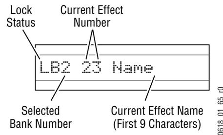
The E-MEM readout display prompts the operator for time entry during Transition Rate operations. The readout can also display messages to the operator. For example, if an attempt is made to alter a locked register the readout will display **Reg is locked** for five seconds. Typical readout displays are shown in ([Figure 69](#)).
