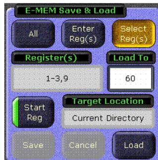
You cannot specify a number that would make the system write beyond the last register. For example, specifying a range of 1-10 with 99 as a Load To register causes an error because 99 is the last Register.
