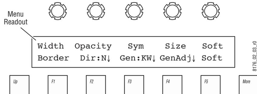
The readout display labels the functions of the soft knobs above and the soft buttons below. Seven characters of the display are used for each knob and button.
