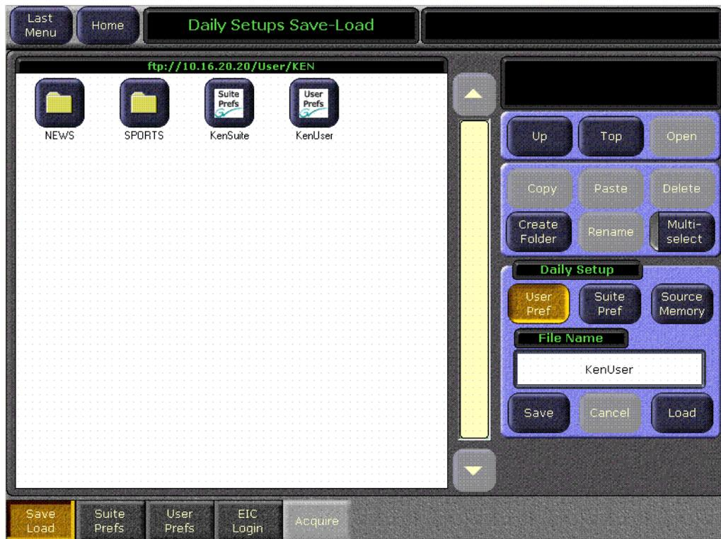
User Pref files contain user preference settings that can change the behavior of a control surface to match the personal preferences of an operator. Controls for these settings reside in the User Prefs menus.
