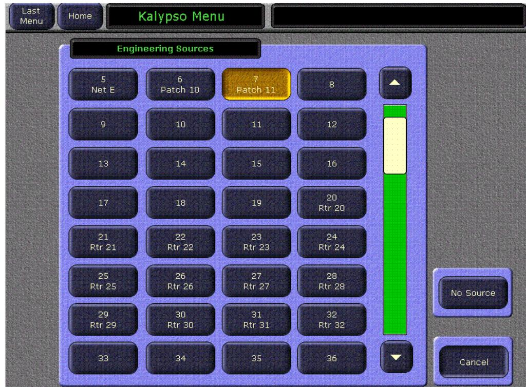
Touching an Engineering source button associates that source to the currently selected Logical source. You can also select **No Source**, in which case the system substitutes black whenever that Logical source is selected.
