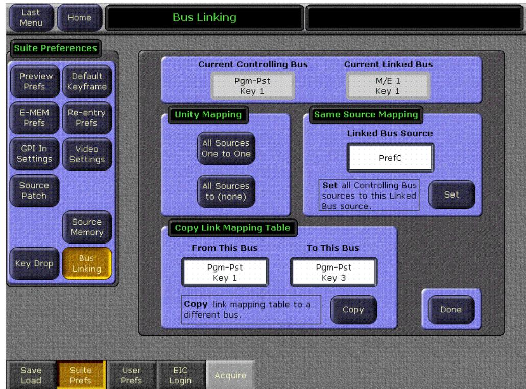
The current Controlling Bus and Linked Bus are identified in the data pads at the top of the pane.
