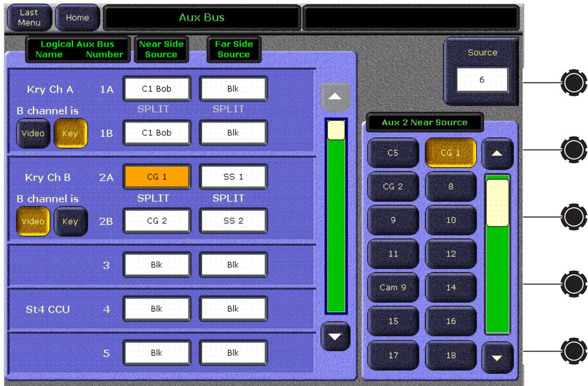
Aux bus sources are selected by choosing an aux bus data pad on the left scrolling pane, and then selecting the switcher source in the right scrolling panel. The Scroll soft knob can also be used to scroll through the available switcher sources.
