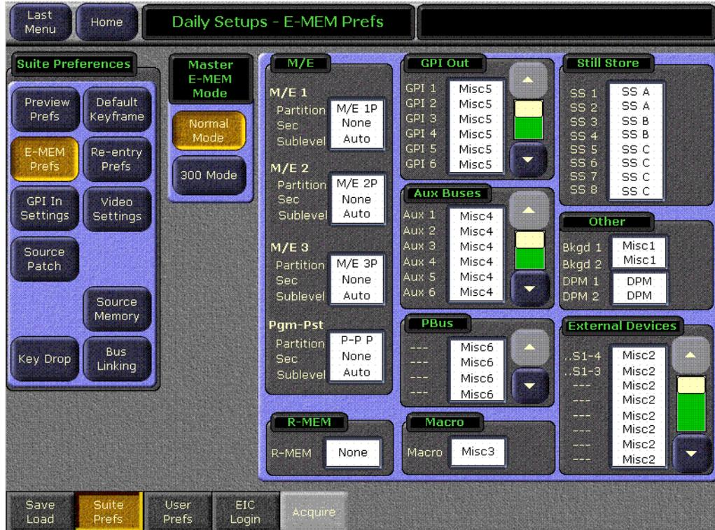
The Kalypso E-MEM system has 19 levels and many sublevels. Fifteen of these levels have Enable buttons in the Master E-MEM subpanel (M/E 1-3, PGM PST, Misc 1-7, etc.). The other four levels are used for M/Es split with the DoubleTake option.
