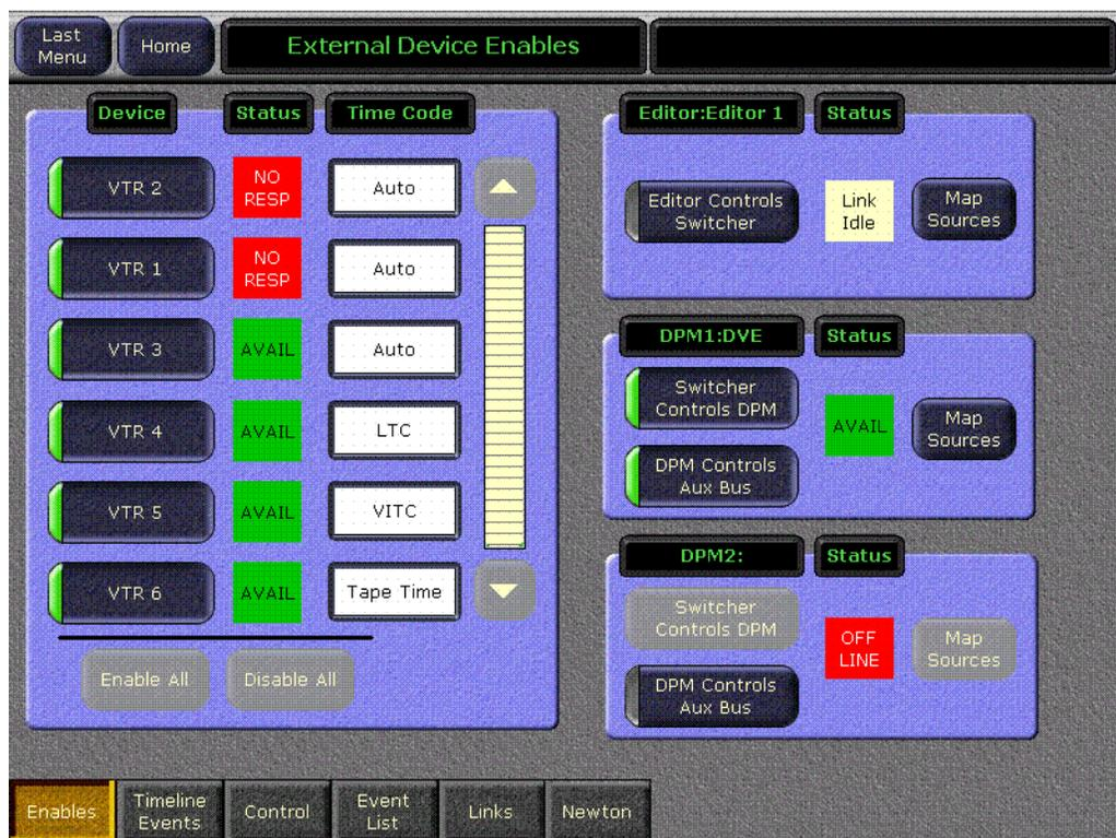
Disabling device control temporarily can be useful. For example, during a rehearsal you may not want to cue or roll VTRs. With the External Device Enables menu you can control which devices will respond without having to rebuild effects or change engineering configuration.
