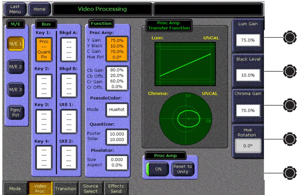
Menu delegation panes (M/E, Bus) on the left permit selecting which bank and bus the menu's video processing controls will be delegated to control. A central Function pane selects the video processing function. Controls for the selected function appear on the right. Soft knobs are available for continuously variable parameters, and touching a soft knob data pad permits entry of exact values.
