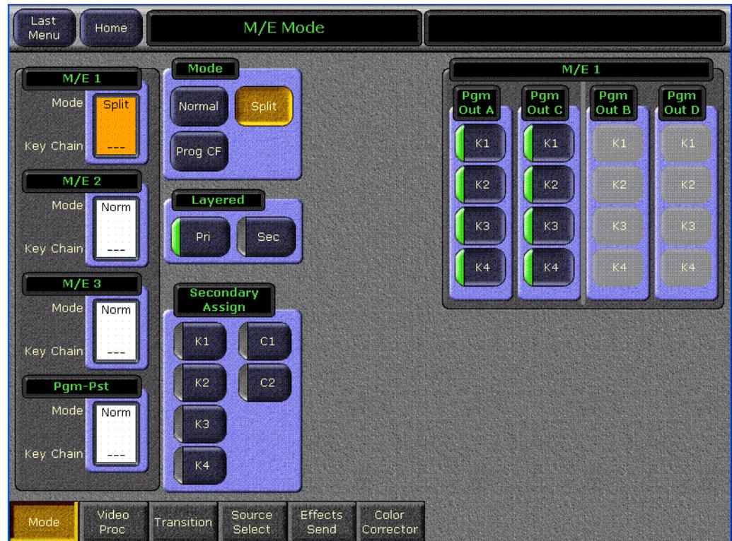
In **Normal** operating mode an M/E provides a main program output, a preview output, and a totally clean feed output (no keys).
