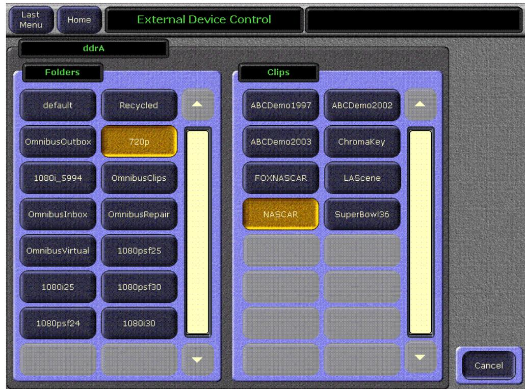
The Kalypso Machine Control subpanel always shows the clip list of the last selected folder. If you change a clip locally on the Profile DDR, that clip name will be updated on the Kalypso External Device menus. If the folder list or clip list are incomplete, re-enabling the device will fetch the entire folder and clip list.
