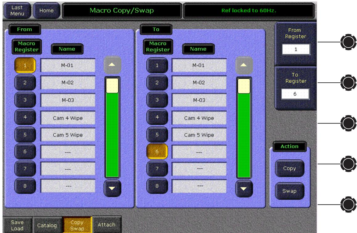
Macro register information can be moved from one register to another with this menu by selecting the registers in the From and To scrolling panes, then touching the **Copy** or **Swap** action buttons on the lower right. The soft knobs and data pads on the upper right can be used to quickly select specific register numbers in each pane.
