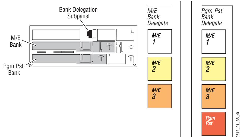
The buttons in the **M/E Bank Delegate** section delegate the M/E bank to control that selected M/E. The M/E bank cannot control PGM PST.
