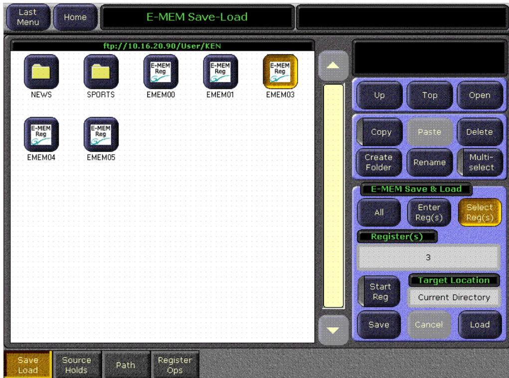
The pane on the left and the navigation and other controls on the upper right side of the screen operate the same the File Ops All Files menu (see page 232).
