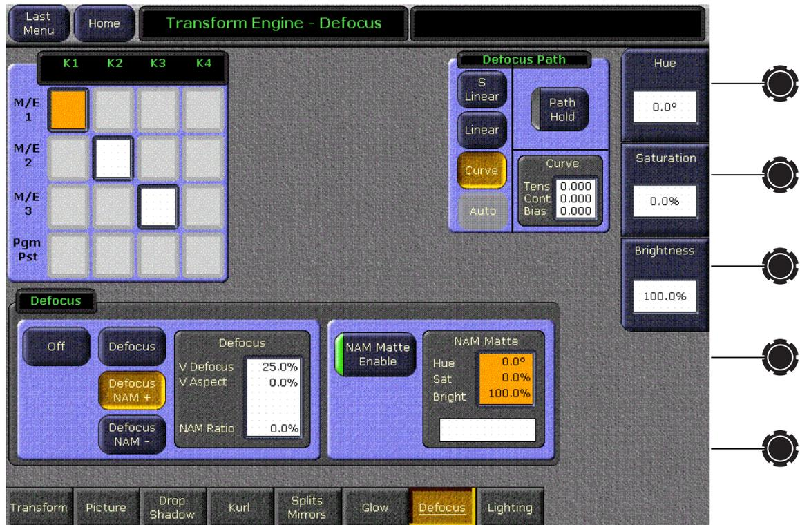
When the NAM Matte pane is activated, knob controls for matte **Hue**, **Saturation**, and **Brightness** become available. An approximation of the color of the matte is shown at the bottom of the pane.
