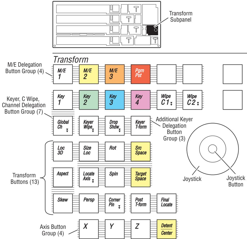
Operating the Transform subpanel involves delegating a resource and a set of associated parameters to the Joystick. The Joystick then provides control of the delegated parameter values. Parameters can also be delegated to the Master E-MEM subpanel for exact value entry.
