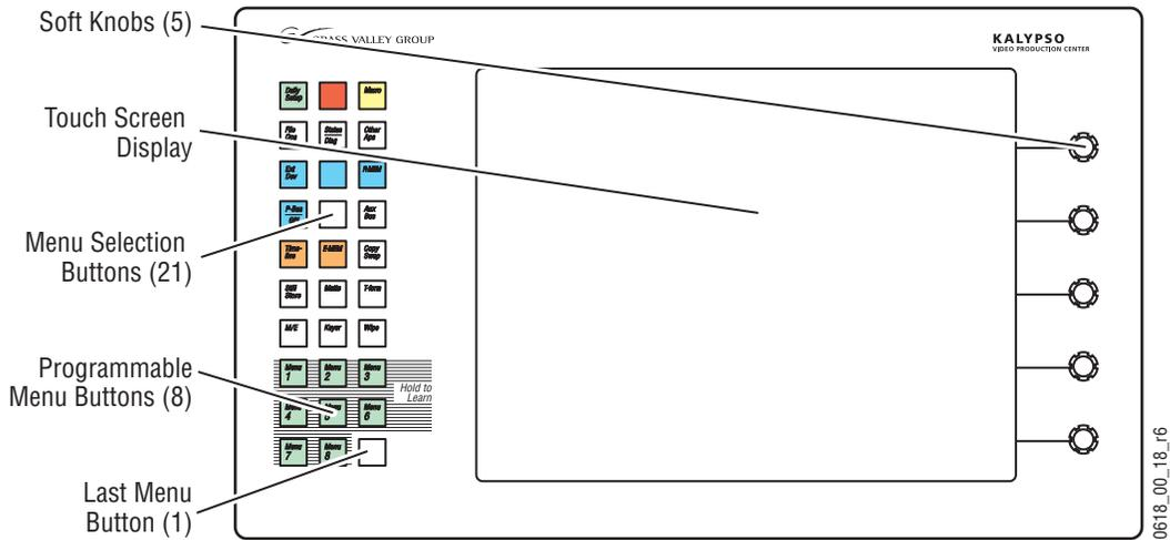
The Menu Selection buttons on the left side of the original Menu panel are used to display various menus on the touch screen. Only one menu button can be selected at a time. The menu state as it was last used will be dis-
