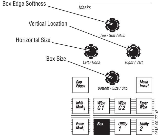
**CAUTION** The horizontal and vertical position controls in the Masks subpanel actually control the position of the selected wipe pattern generator. If the generator being adjusted is shared with other points of use, all these points will be affected by the change.
