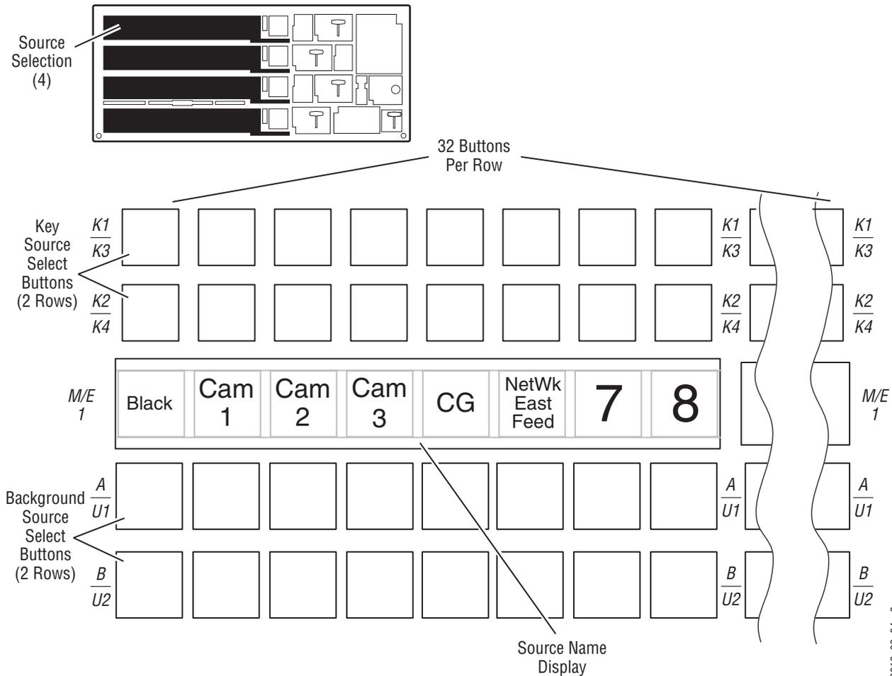
Pressing a button on an M/E row selects the source mapped to that button on the controlled bus, and the source button will go high tally if on-air, or low tally if not. Of 128 available sources, up to 32 can be mapped to the unshifted source selection buttons, and 32 to those shifted buttons. The remaining 56 available sources can be selected via an E-MEM recall or using the Source Select menu. The reentry buttons are fixed and cannot be mapped.
