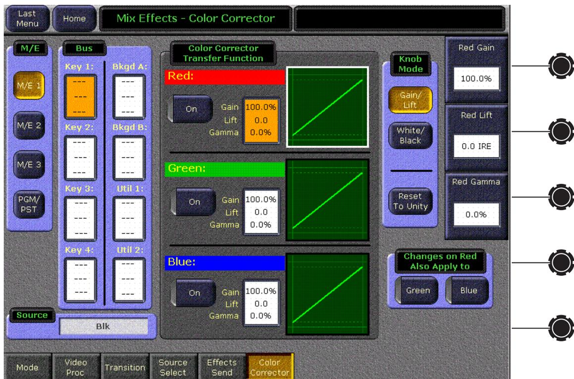
The M/E pane button group selects the M/E. The Bus data box group selects the bus layer within the M/E. The data boxes for the Bus delegation contain **Red**, **Green**, **Blue**, or - - -. A color component in the data box indicates that color correction is being applied to the component(s). For components not enabled, the - - - is shown as a placeholder.
