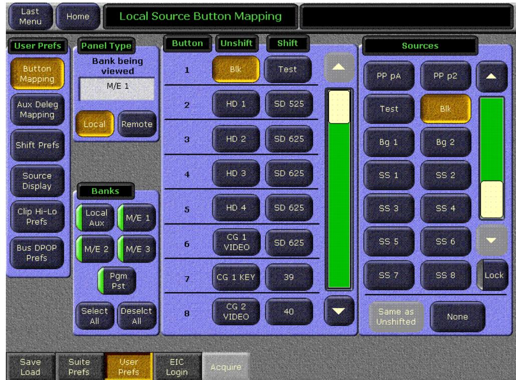
The Button Mapping menu can be delegated to configure Local panels (Main Panel and Local Aux Panel), or Remote Aux panels. On the Kalypso system, each bank on the Main Panel can have its own independent source to button mapping, if desired. The Local Aux panel can also have different button mappings, as well as each Remote Aux panel.
