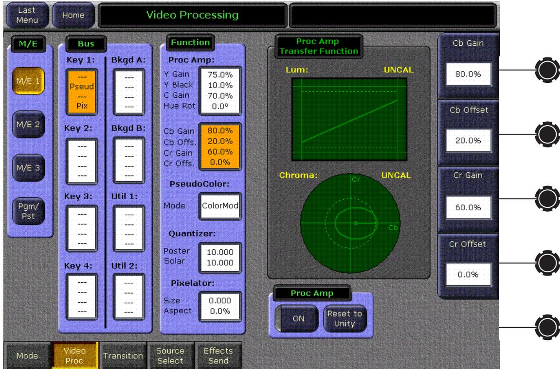
**CAUTION** When adjusting Proc Amp controls, illegal colors could be generated. Illegal colors have equivalent red, green, and blue color components that take on negative values. Illegal colors can cause problems in picture monitors and other equipment downstream of the switcher. The amount of adjustment that can cause this problem depends on the original picture content. This problem does not occur for typical small adjustments.
