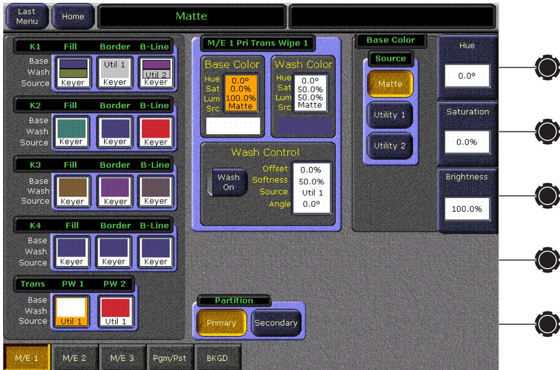
To use a matte as intermediate video, select the **Matte** button in the Base Color – Source pane on the right of the menu. Use the matte controls to set the desired matte settings for the intermediate video.
