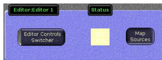
The **Editor Controls Switcher** button toggles on and off to indicate whether the Editor can control the switcher.
