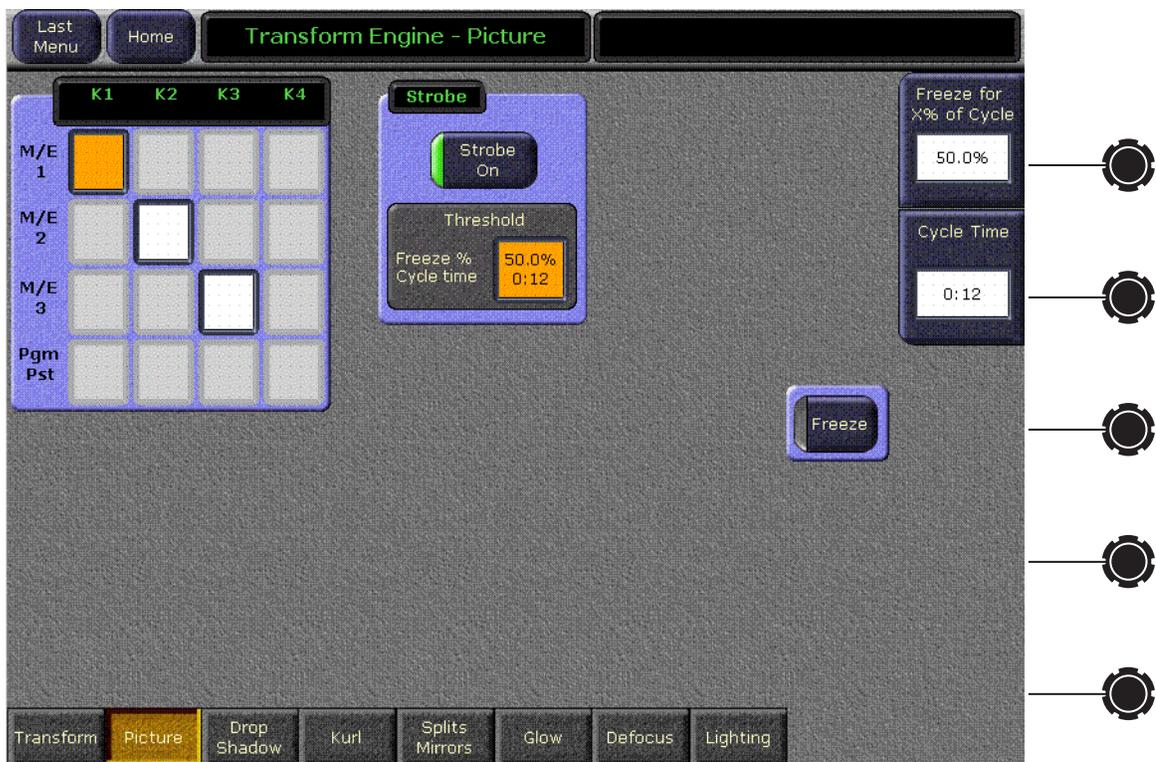
For example, 12 frames of frozen video with a 100% frozen duty cycle can be specified. The Transform Engine would then grab a frame and freeze it for 12 frames, and grab a new frozen video image every 12 frames. With a 50% frozen duty cycle using the same setting for 12 frames of frozen video, a still-frame would be displayed for 6 frames of video, followed by 6 frames of motion video. Then the cycle would repeat.
