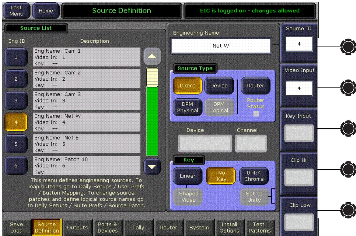
The soft knobs on the right can be used to scroll through the source list and assign inputs. Touching these data pads allows direct numeric input. Input number connectors are listed in Table 9.
