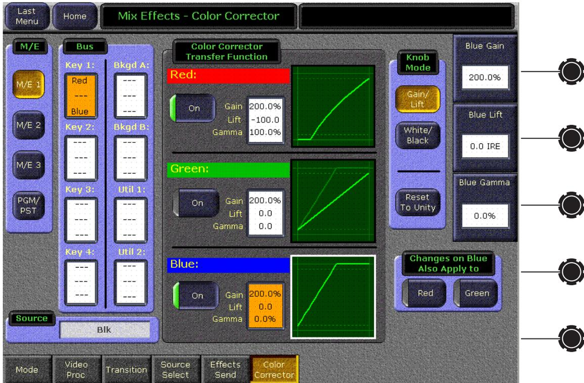
The three color components have individual **On** buttons, which are LED push on/push off type buttons. As shown in Figure 259, the Red and Blue components have been enabled but the Green component has not. If a com-
