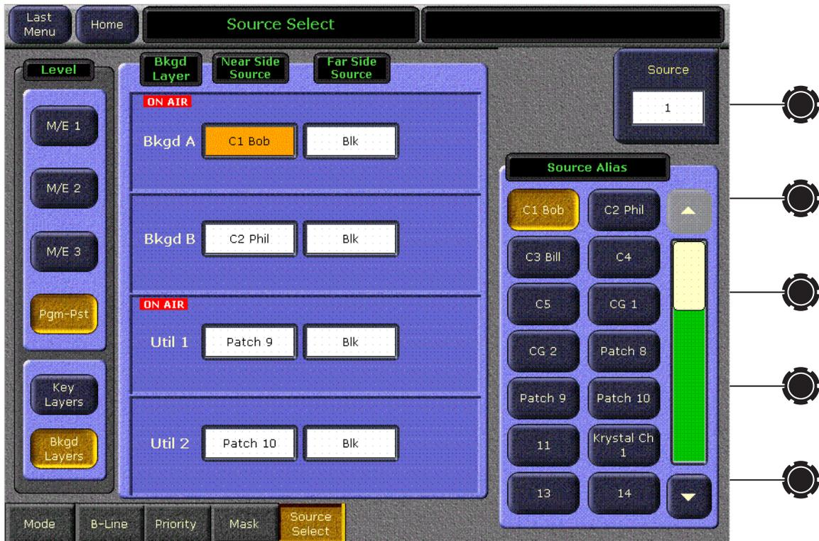
Sources are changed by choosing either the Key Layers or the Bkgd Layers, delegating the desired item (for example, M/E 1, Keyer 1 Fill, Near Side Source), and then selecting the source from the scrolling list on the right. You can tap the green area of the slider to display the next group of sources, and you can drag your finger on the slider handle to quickly scroll the list. Sources can also be selected with the Source soft knob.
