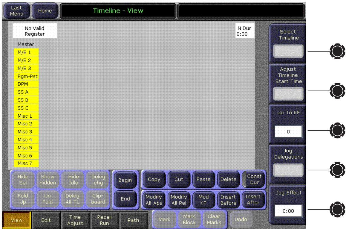
The Timeline – View menu is intended to provide different ways to display the effect information. Release 12.0 supports a single view of the data.
