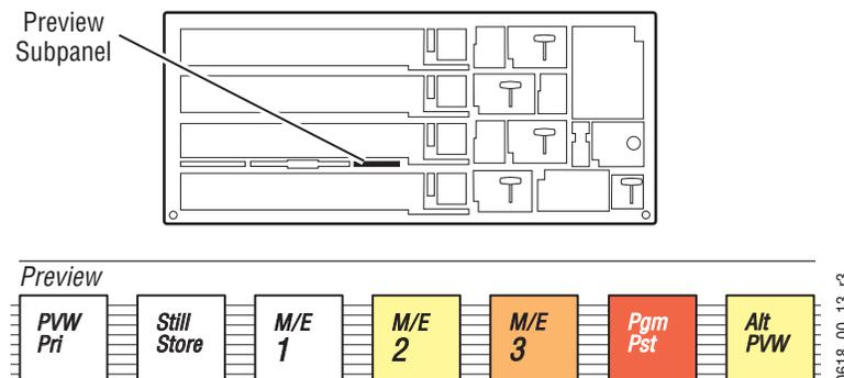
The Preview subpanel also works with the Local Aux panel, which provides a selection mechanism for viewing sources and program outputs of the M/Es on the switched preview output. Note that the switched preview will automatically show the appropriate signal during Hold to Preview, Show Key, Color Pick and Auto Key Setup operations, replacing whatever signal may have been selected for previewing.
