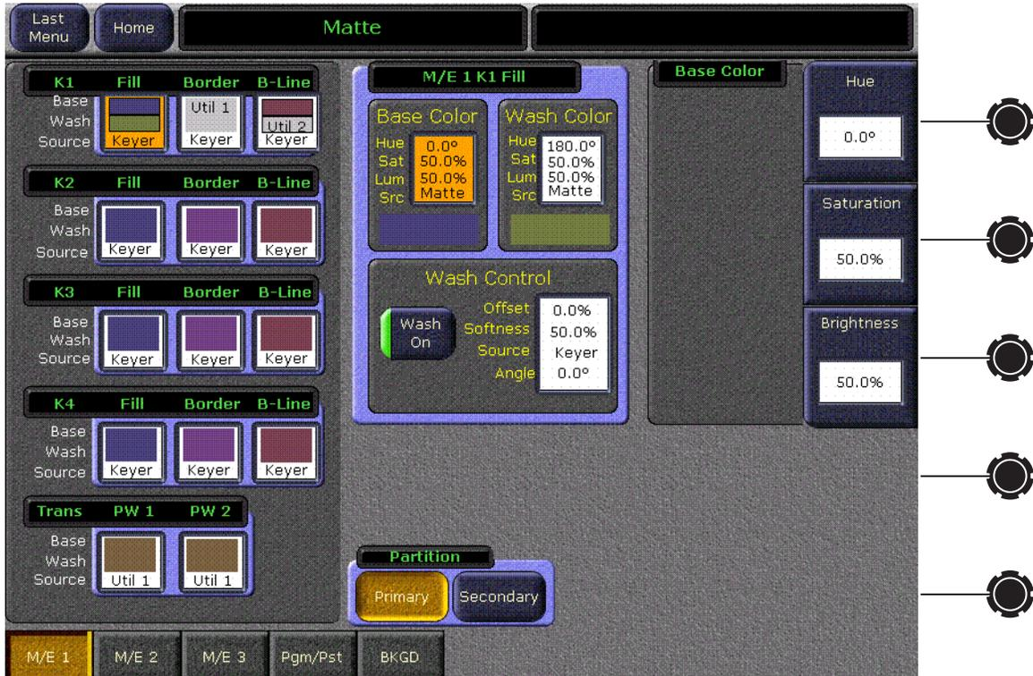
**Primary** and **Secondary** partition delegation buttons provide independent control of the mattes used in the Primary and Secondary partitions of a split M/E (available with the DoubleTake option). See the separate *Kalypso User Manual* for more information about DoubleTake split Mode M/E partitions.
