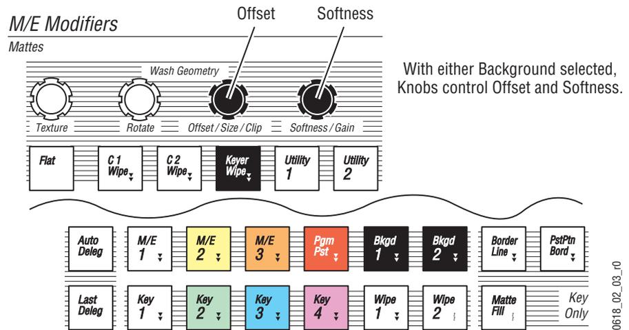
When either **Utility 1** or **Utility 2** is selected the two knobs control Clip and Gain of the video that specifies the wash (Figure 65).
