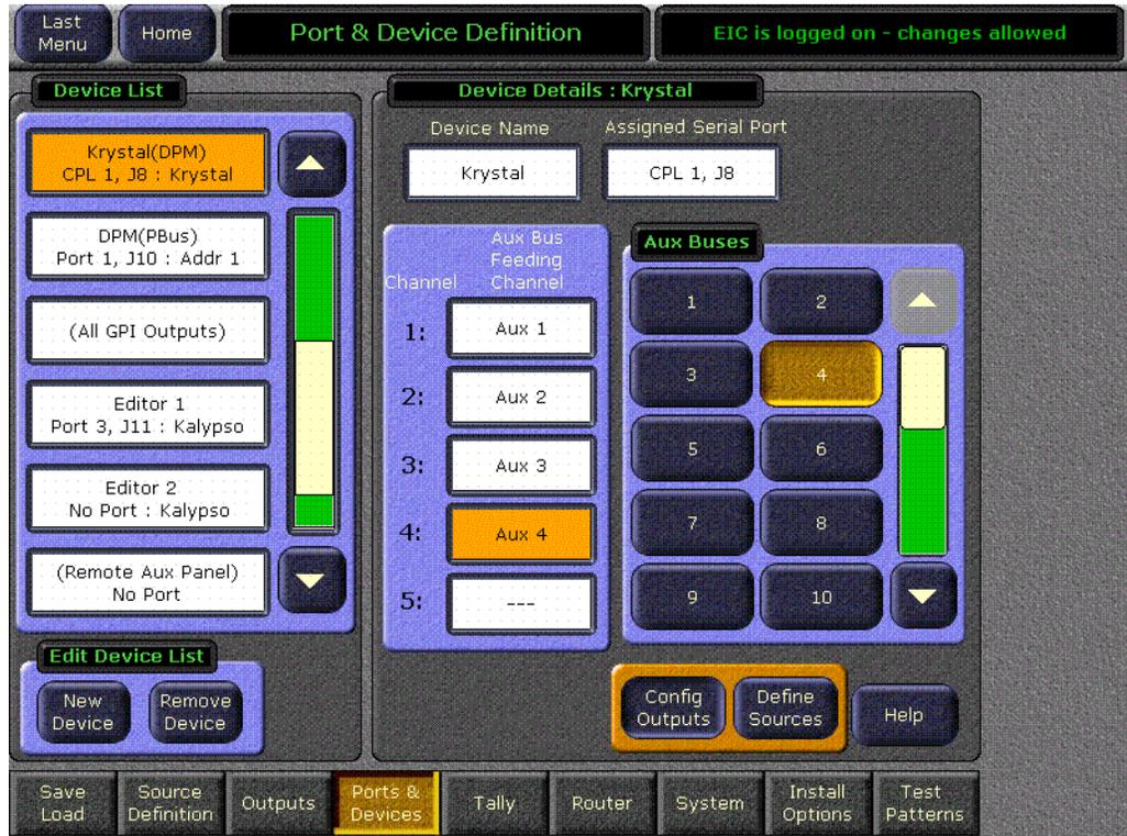
Touching the **New Device** button brings up a menu used to create a new device definition (Figure 137).
