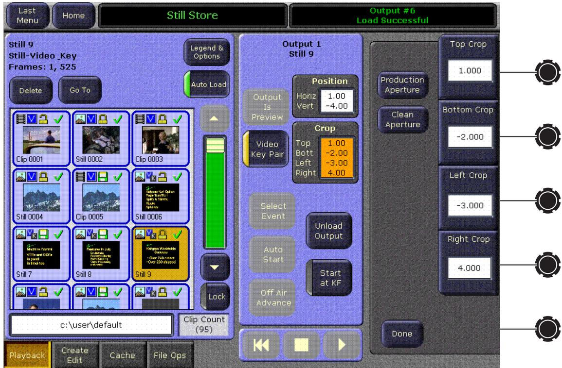
The **Production Aperture** button sets crops slightly wider than Clean Aperture, to meet the SMPTE recommended practice. This permits passing the maximum amount of image data down the signal chain, which can help hide edge artifacts during subsequent image processing.
