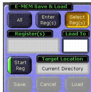
Clicking on the **Load To** datapad opens the Load To keypad (Figure 195). Enter the number for a single register to which you would like to begin loading registers.
