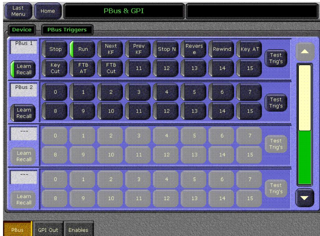
Up to 16 PBus triggers (0-15) can be associated with each external device on the PBus. When a device is defined (Eng Setups), names can be given to the device and each of its triggers. The actual action performed when a particular trigger is sent is determined by the external device. For user convenience, in Eng Setups each trigger can be given a descriptive name.
