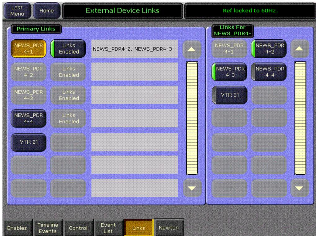
The External Device Links menu has two panes with scrolling lists, each listing the devices setup for Kalypso system control. A primary device is selected in the Primary Links pane on the left, and the devices that are to be linked to that primary device are selected in the pane on the right.
