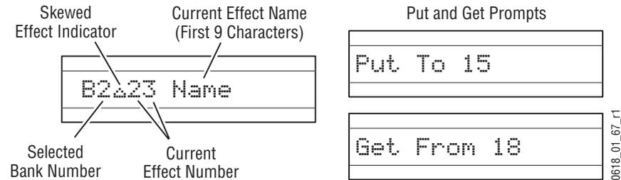
If there is more than one current effect register (different E-MEM levels were independently recalled from different registers, also called a *skewed effect*) a triangle symbol is displayed between the current bank number and the current register number. The locations of the contributing registers can be determined by turning on one enable at a time.
