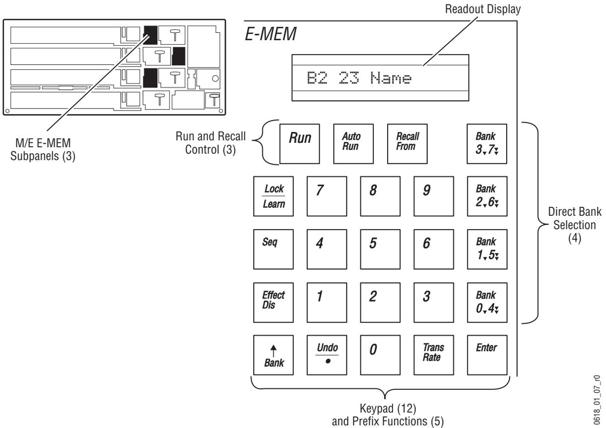
All the functions of an individual E-MEM subpanel are also available on the Master E-MEM subpanel, via enables (see *Master E-MEM Subpanel on page 110*).
