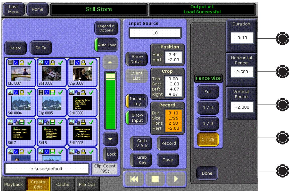
The **Duration** data pad and soft knob determine the duration of the recording. The parameter value is in frames.
