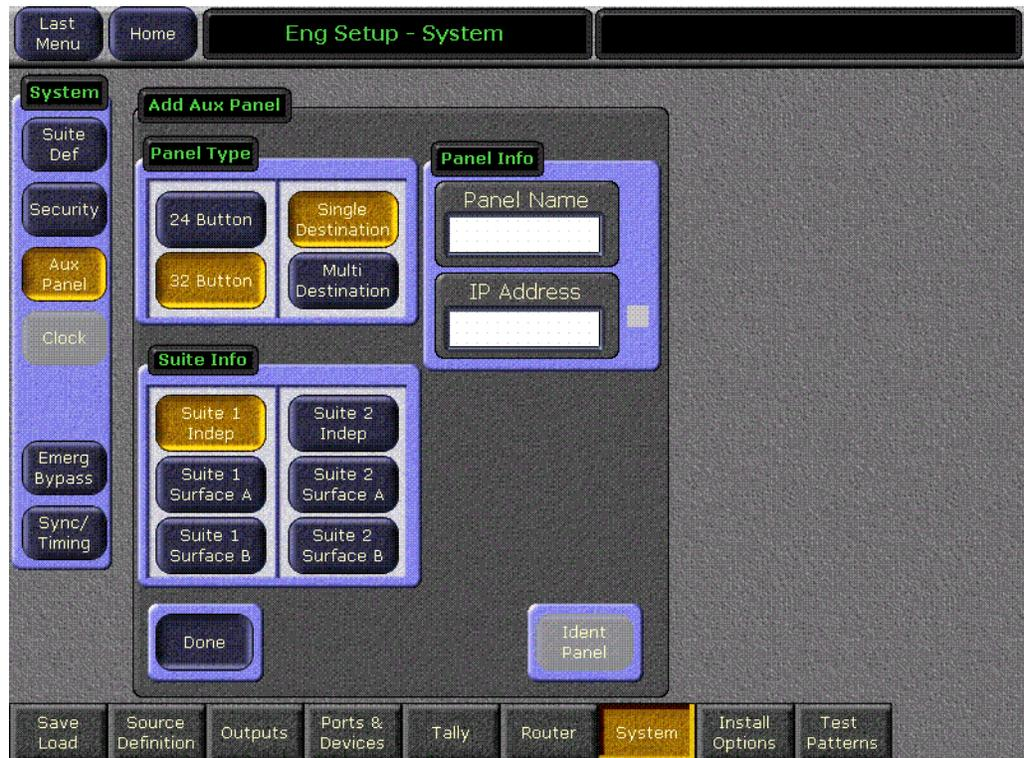
The **Suite 1 Indep** and **Suite 2 Indep** buttons assign that Aux panel to control the Aux buses of that suite. The configuration settings for this Aux panel are saved with Eng setups, however, and so are independent from individual Suite and User Pref settings. This setting is generally used for Aux panels that reside outside a local workspace, for example a machine room or video operations area.
