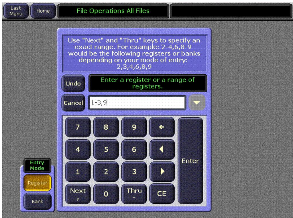
For example, in Figure 192 clicking on the Enter key will enter Registers 1 through 3 and also register 9. If the **Bank** button were selected clicking on the Enter key will enter Registers 10-39, 90-99.
