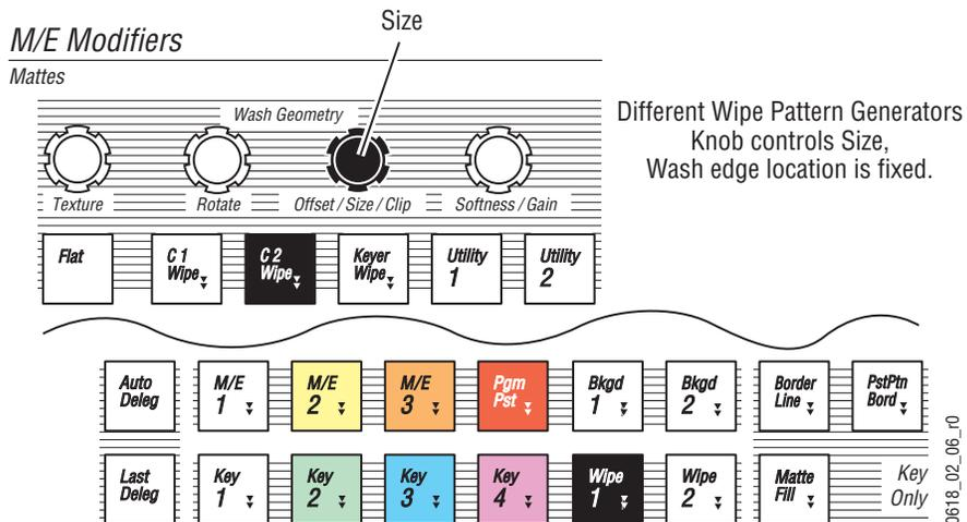
The above also applies to preset patterns. Selecting **PstPtn Border** as the Key Only delegation and selecting **Keyer Wipe** for Wash Geometry (the same wipe pattern generator) gives the knob Offset control. With a **Pst Ptn Border** delegation, selecting either **C1 Wipe** or **C2 Wipe** gives Size control.
