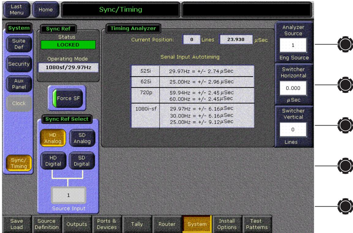
A Timing Analyzer is available, as well as controls to select the sync reference that switches the system between HD and SD operating modes. See the separate *Kalypso HD/Duo Installation and Service Manual* for information about these additional controls.
