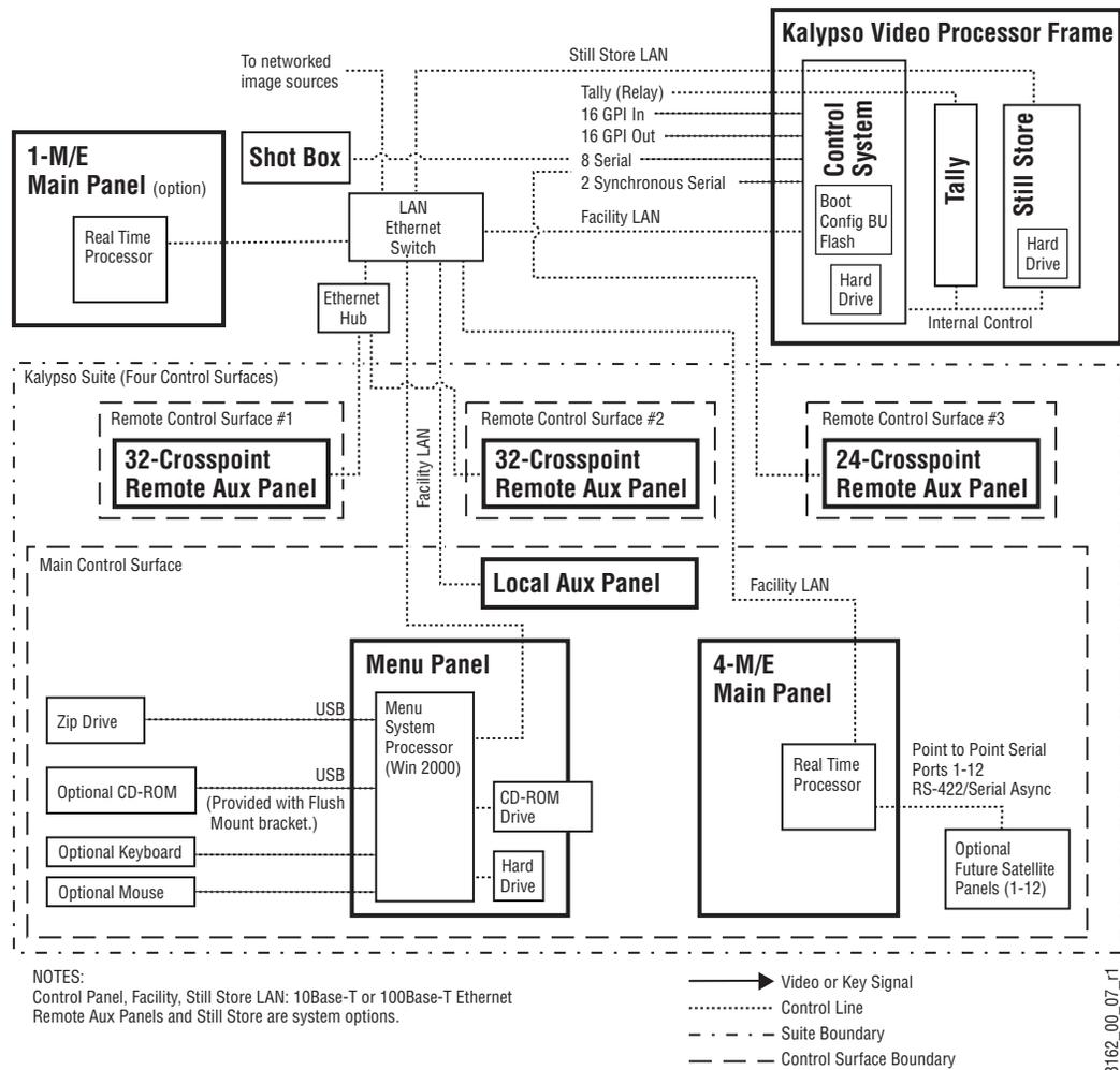
Late model 2-M/E Kalypso system control is the same as the 4-M/E Kalypso system, except the Local Aux panel is built into the 2-M/E Main panel (Figure 41).
