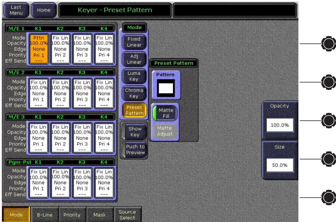
The 4 x 4 grid of data pads on the left are used to delegate one of the 16 keyers (four M/Es, each with four keyers) for control by the menu. The selected keyer is colored gold.
