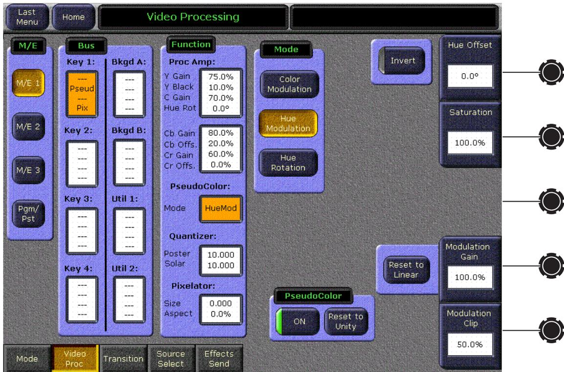
**Hue Modulation** (Figure 248) operates like Color Modulation, but instead of mixing between two color mattes, the modulating signal maps incoming luminance to matte hue. As the instantaneous luminance value of the incoming video changes from black to white, the instantaneous hue of the processed picture changes in hue angle. As the luminance increases, the hue value increases toward magenta, red, etc., counterclockwise on the vectorscope.
