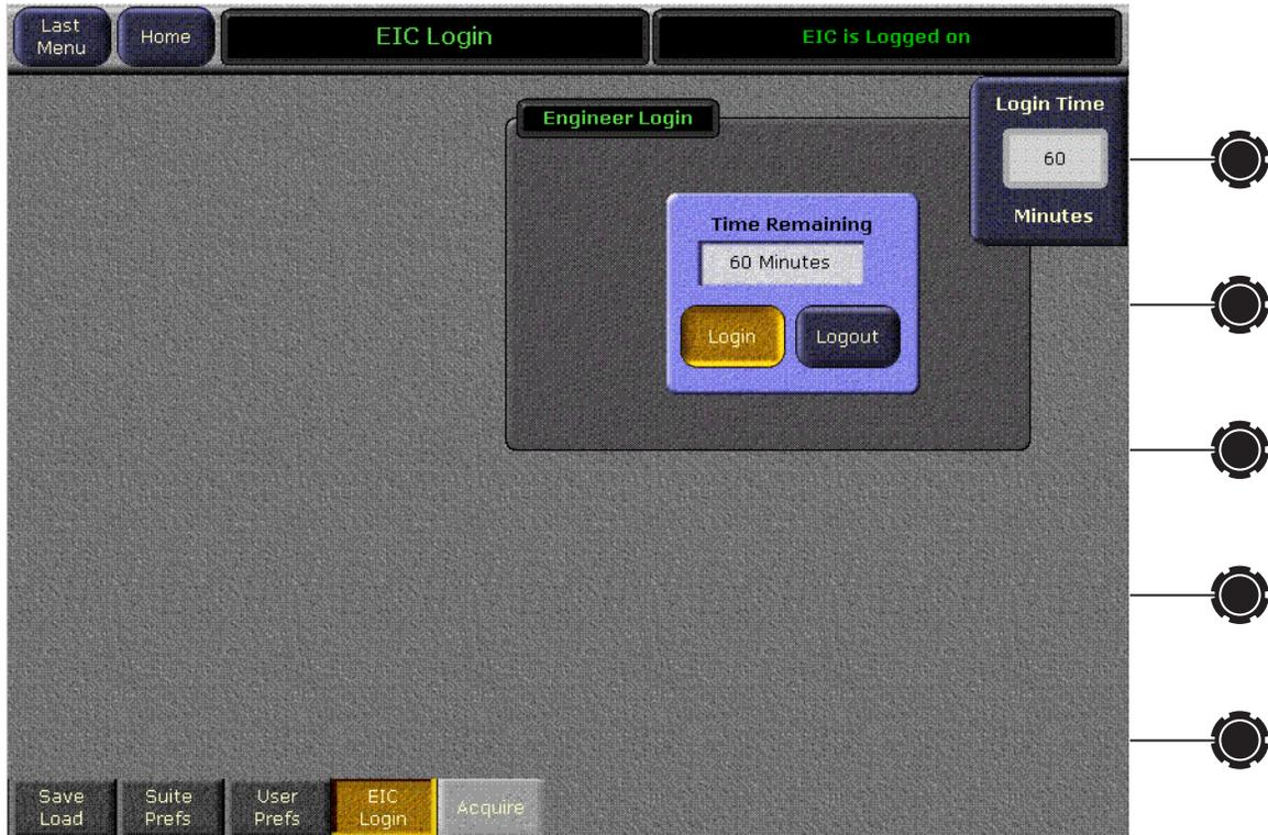
A password may be required to log in, depending on the security account settings. When logged in, changes can be made to the Kalypso system Engineering Setups and loading an Eng Setup file will be permitted.
