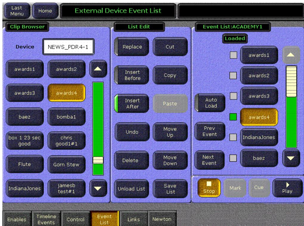
**CAUTION** If an Event List is loaded that has the names of clips that have been deleted from the DDR, there is no advance notification that clips are missing, commands for the missing clips will be ignored, and those clips will not play.
