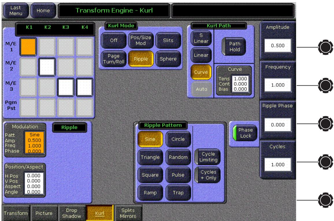
The Ripple soft knob controls and wave patterns are the same as Position/Size, except there is no H/V Angle control (see [Modulation Pane](#) on page 326 and [Figure 229](#) on page 328).
