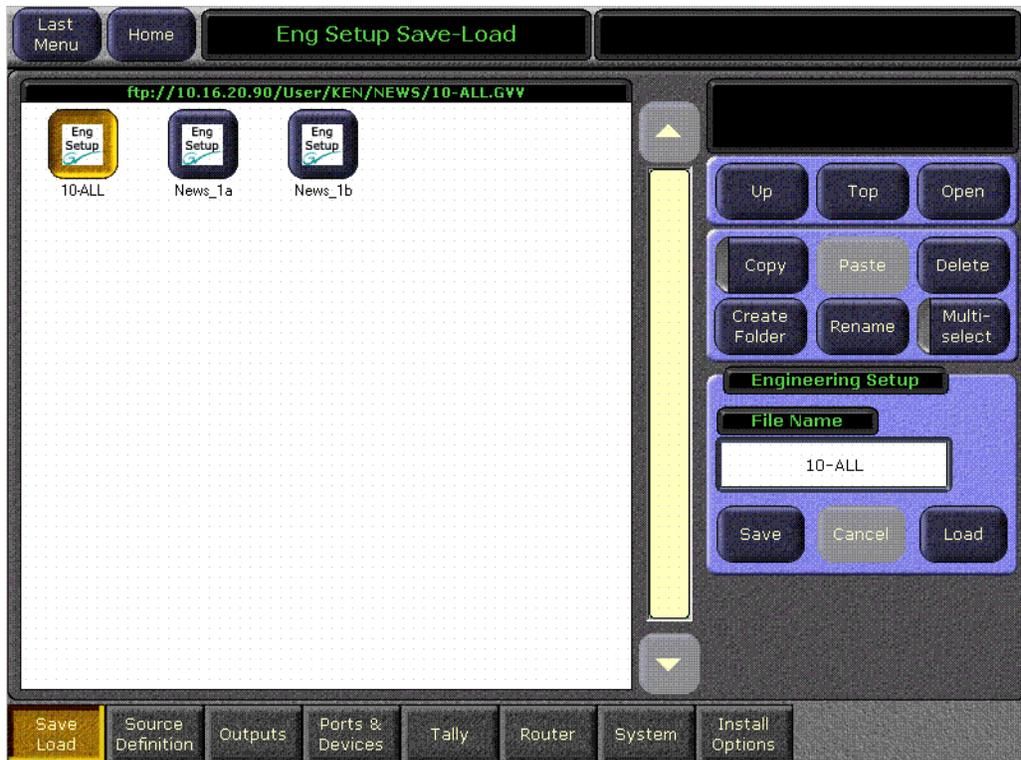
On the left side of the Eng Setup Save-Load menu is a file display pane equipped with a scroll bar. This pane shows icons and names of the files, folders, and drives contained in the currently selected directory. The
