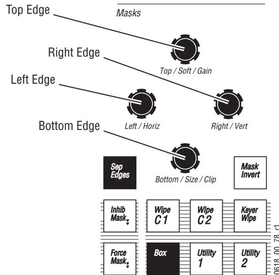
When **Utility 1** or **Utility 2** is selected the following knobs are available (Figure 60). **Joystick** control is not available for utility masks.
