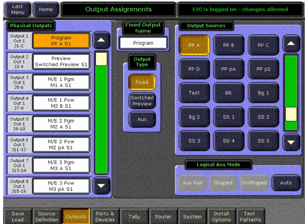
Eight data pads at a time are displayed in the left Physical Outputs area. Each data pad is associated with a specific pair of physical output connectors on the frame. Touching a data pad selects it, colors it gold, and the rest of the screen will show information and settings for only the selected item.
