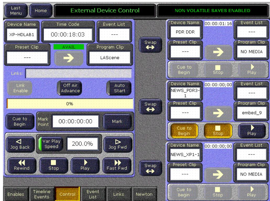
The pane on the left provides full control of one device. The three panes on the right provide limited control of each of those devices. Any limited control device can be swapped with the full control device by touching the **Swap** button. This gives any device access to the additional control functions available in the larger pane.
