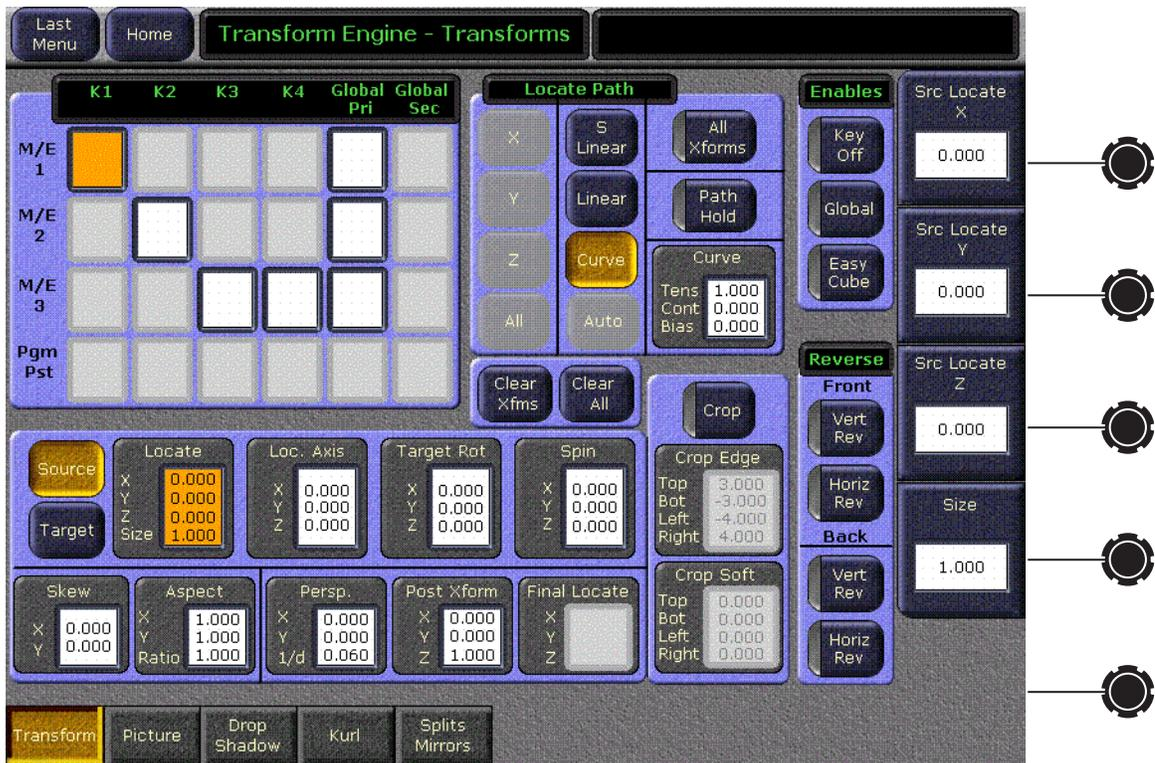
The Transform Engine menu has all the transform controls on the Main panel's Transform subpanel except the Joystick (soft knobs or keypad entry are used instead). The Transform Engine menu also has additional controls not present on the Main panel, including **Crop** and **Reverse** and **Easy Cube**.
