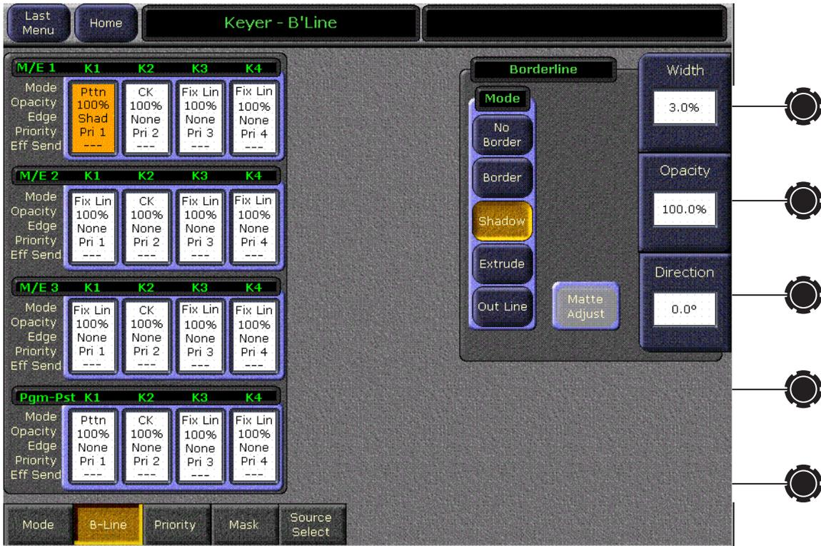
The 4 x 4 grid of data pads on the left are used to delegate one of the 16 keyers. The Borderline controls displayed for the delegated keyer on the right side match the button and knob controls on the Main panel.
