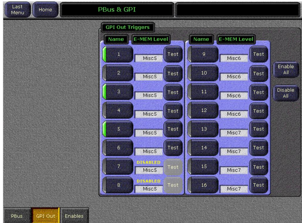
In Eng Setups, each GPI trigger can be given a descriptive name that appears on the buttons in this menu. The actual action performed when a GPI trigger is fired is determined by how it is wired to the external device.
