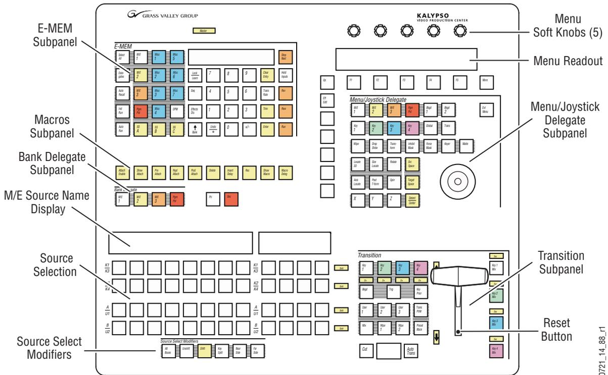
The 1-M/E Main panel has a reset button on the rear and one inside the lever arm slot, to permit easy reset when installed in a console.
