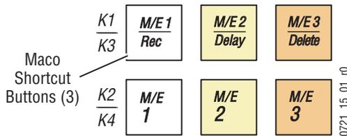
Holding down **M/E 1/Rec** initiates macro Record mode and delegates the keyer row to macro operation. With the button held down, select a macro register button to record into and then release the **M/E 1/Rec** button. Perform the operations to be recorded, and when done press the flashing Rec or macro register button to terminate the recording. Pressing the button twice and holding it down after the second press activates macro Append mode (as long as the button is held down).
