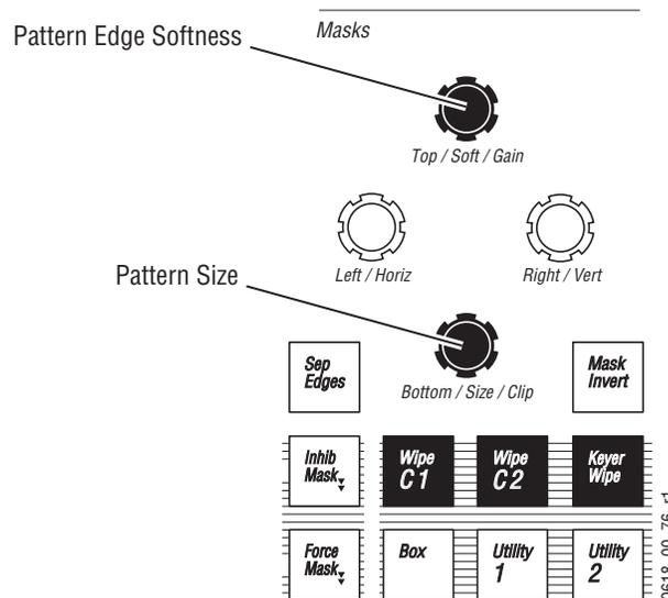
When **Box** is selected with **Sep Edges** off, the following knobs are available (Figure 58). Preset Pattern can also be adjusted using these mask controls.
