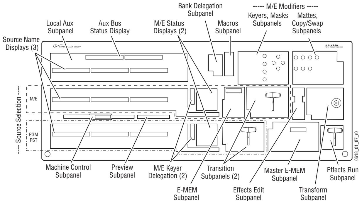
The controls on the 2-M/E Main subpanel are essentially identical to those on a 4-M/E panel, though they may be placed at different locations on the panel. Only differences in these controls will be discussed here. Refer to the 4-M/E subpanel descriptions for more information.
