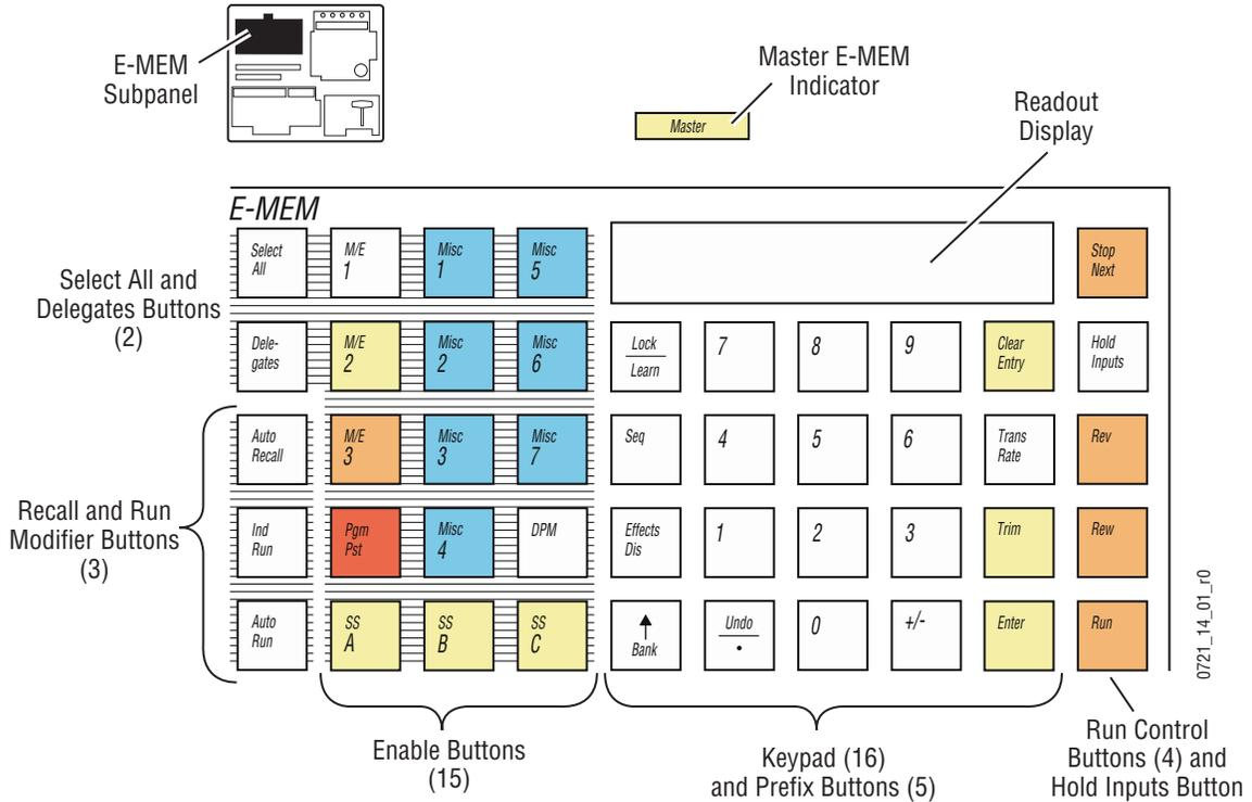
The E-MEM subpanel operates as either an individual M/E E-MEM subpanel or as a Master E-MEM subpanel, depending on delegation.
