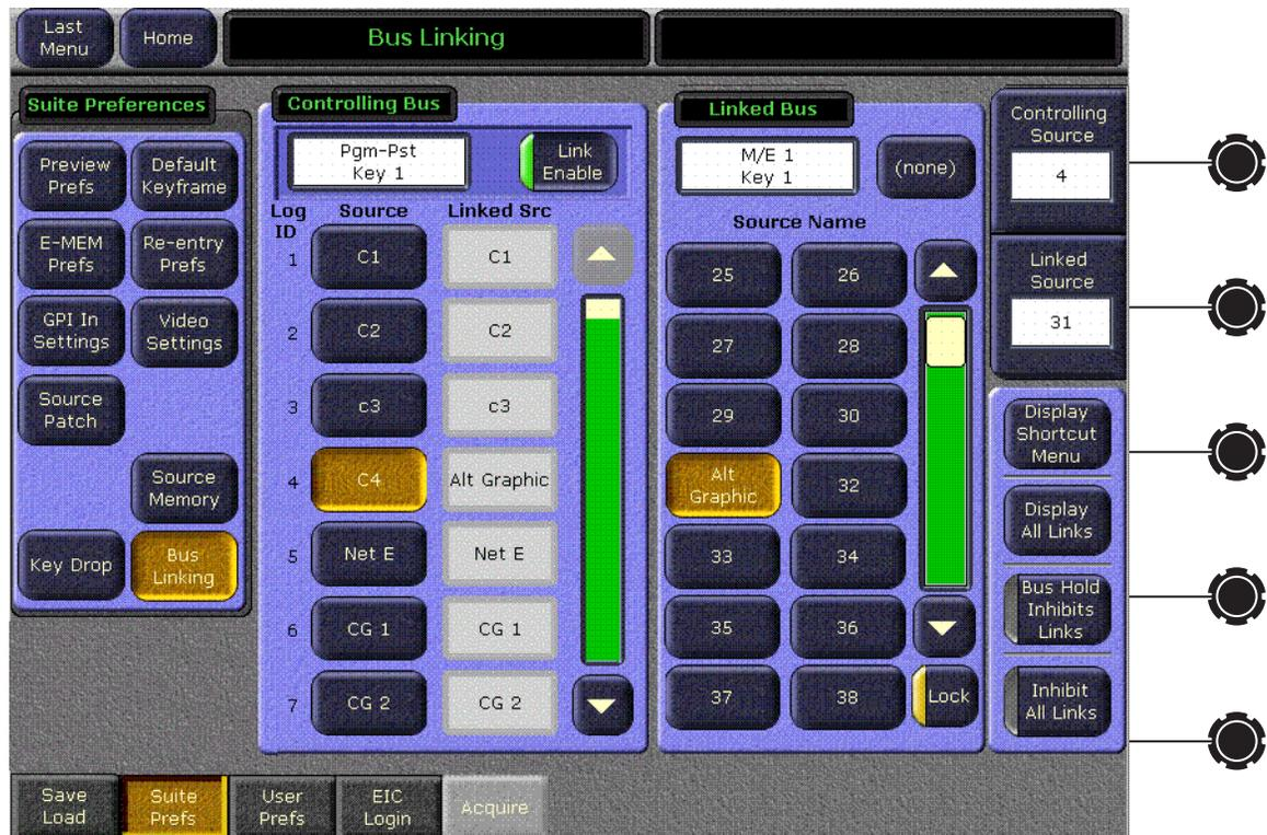
The Bus Linking menu has two main panes, a Controlling bus pane on the left and a Linked bus pane on the right. Controls in these panes are used to select the buses to be linked and associate the sources between those buses. The Controlling bus pane shows the current source associations. Controls outside these panes on the right side of the menu are also available for making source associations and managing bus links.
