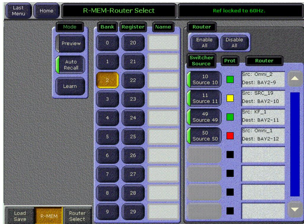
When **Preview** mode is turned on, recalling a register will only display the R-MEM settings stored in that register. No switcher sources will change. This allows you to see what switcher sources will be affected by a register recall, and what the router sources and destinations will be after the recall. When **Preview** is turned off, the right pane returns to displaying the current status, including any previously set enables.
