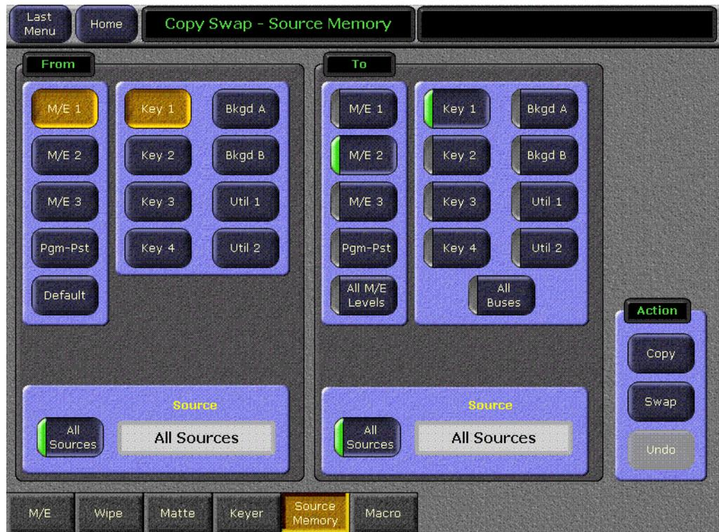
The user delegates the M/E level, the keyer within the M/E, and the numbered input source to the keyer. Each source on each keyer has its own source memory, which is a collection of keyer settings specific to that particular intersection (point of use) of the keyer and its input.
