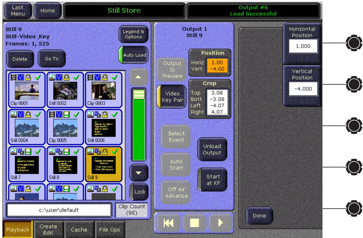
Touching the **Crop** data pad brings up a similar menu with **Top Crop**, **Bottom Crop**, **Left Crop**, and **Right Crop** controls (Figure 212). The image can be cropped to any rectangular shape. These controls are keyframeable but resolution is limited to pixels and lines so interpolated motion may not appear smooth. For smooth motion use a Transform Engine.
