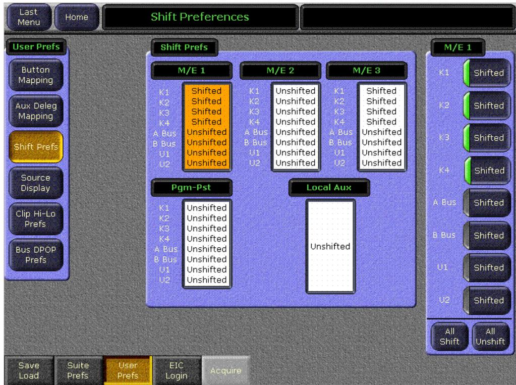
**Note** The **Shift Prefs** and **Source Display** menu settings should match, so each shifted bank displays shifted source names by default, and vice versa. In these two menus select both shifted or both unshifted for each bank that is not using Split Mode. See the next page for related information.
