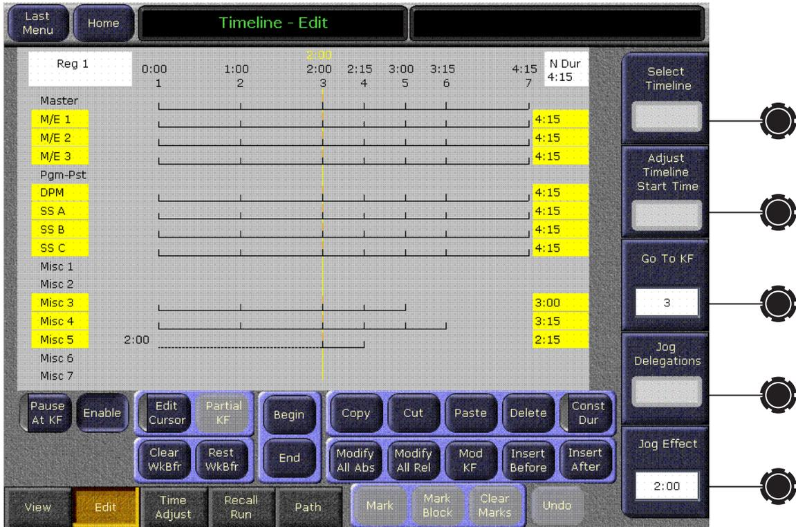
The number of the currently loaded register appears at the upper left corner of the menu. Below are the names of E-MEM level groups, and to the right of each name is an area for displaying its timeline. Only Enabled level groups are displayed. The names of level groups that are delegated for editing are highlighted in yellow. Only these highlighted timelines are affected by edit operations.
