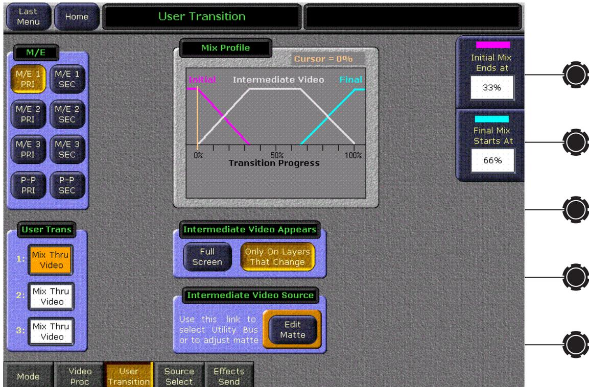
The M/E pane on the left delegates the rest of the menu to that M/E. The User Trans pane below that represents the **User 1**, **User 2**, or **User 3** User Transition buttons on the selected M/E's Transition subpanel. Selections in both of these panes are required to delegate the menu controls for a specific User Transition. The three Transition subpanel User buttons DPOP to the User Transition menu properly delegated to that button.
