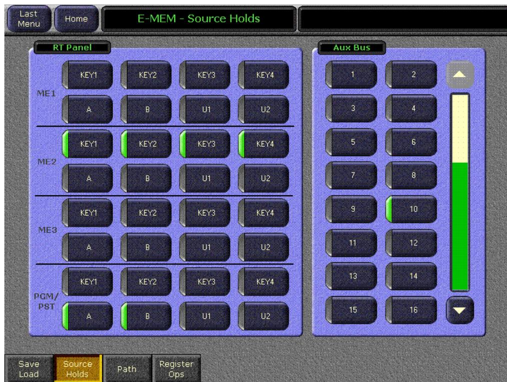
During E-MEM recalls and effect runs sources can be programmed to change. Sometimes this is not desired, as an effect may be designed to run on the currently selected sources, not the particular sources used when the effect was built.
