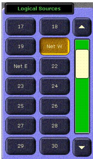
When multiple items are available for selection, scrolling lists are used (Figure 100). On most menus, touching the up and down triangle buttons scrolls the list up or down one item. When the top or bottom of the list is reached, that button goes gray. Touching the green area above or below the white handle scrolls the list up or down one group of items. You can also drag the white handle to quickly scroll through the entire list on some menus.
