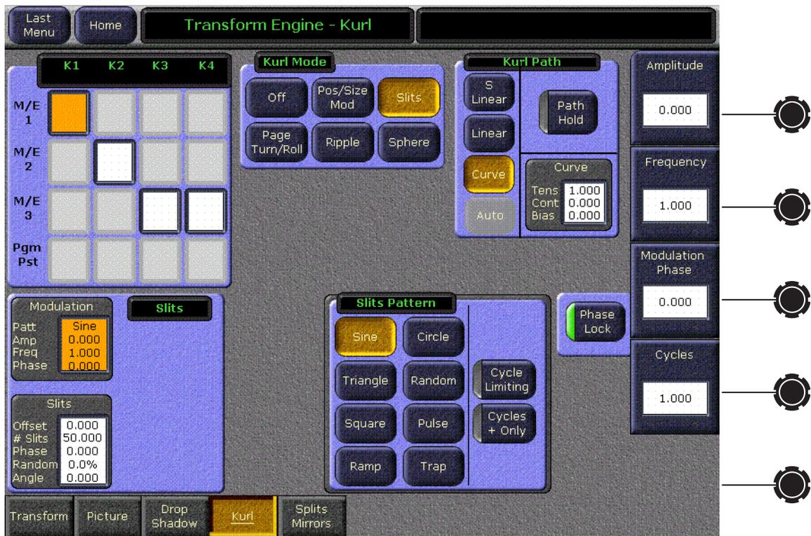
The Slit modulation soft knob controls and wave patterns are the same as Position/Size (see [Modulation Pane](#) on page 326 and [Figure 229](#) on page 328).
