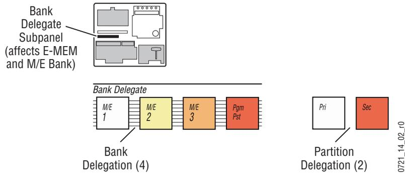
When **M/E 1**, **M/E 2**, or **M/E 3** is selected, that Kalypso system M/E is controlled by the 1-M/E panel, and the E-MEM subpanel operates the same as an individual M/E E-MEM on a 2 or 4-M/E Kalypso Main panel.
