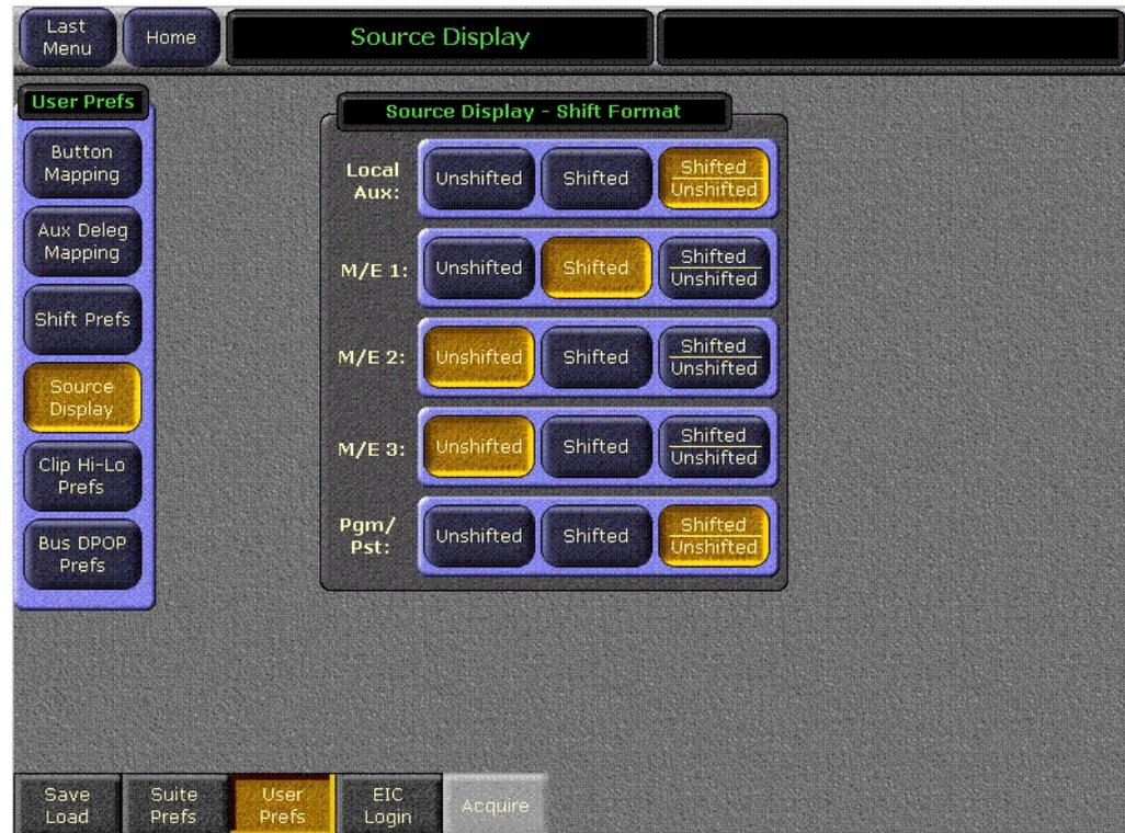
**Note** The **Source Display** and **Shift Prefs** menu settings should match, so each shifted bank displays shifted source names by default, and vice versa. In these two menus select both shifted or both unshifted for each bank that is not using Split Mode. See the previous page for related information.
