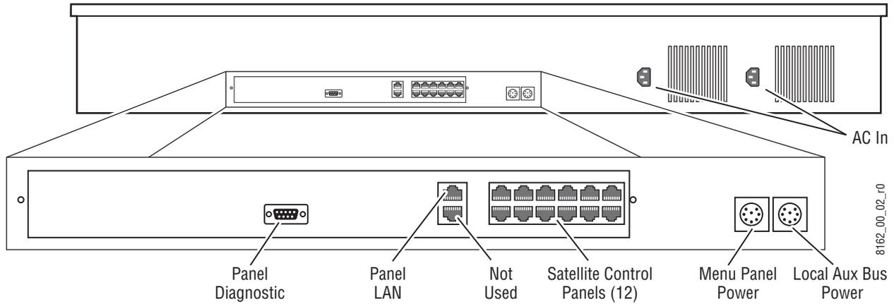
Main panel power switches and the Main panel reset button are accessed by lifting the top of the Main panel ([Figure 5](#)). A redundant power supply can be installed into the tub of the Main panel as an option. The Main panel provides power to the separate Menu panel and Local Aux panel.
