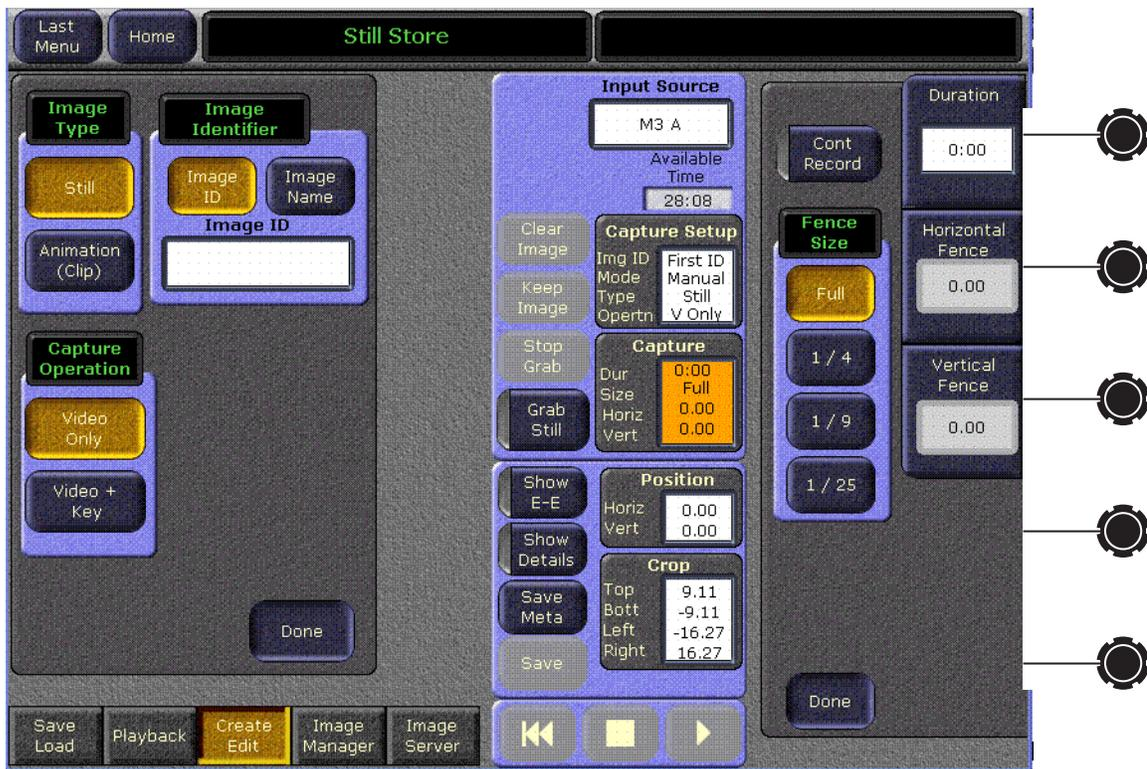
The middle touch button group contains the **Show Buffer**, **Show Details**, and **Save Meta** parameter selection buttons, the **Save** touch button, and the **Position** and **Crop** data pads.
