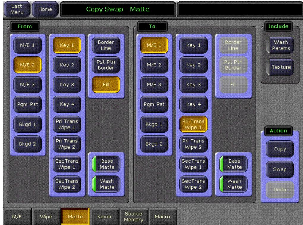
Some combinations of M/E level, Key level, and matte generator level do not exist. For example, in [Figure 209](#), the destination matte is M/E 1's Trans Wipe. Pst Ptn Border, and Fill are grayed out because they only apply to keyer mattes. Similarly, if Bkgd 1 had been chosen, no further delegation would be needed, so all of the keyer related selections would be grayed out.
