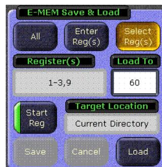
You cannot specify a number that would make the system write beyond the last register. For example, specifying a range of 1-10 with 99 as a Load To register causes an error because 99 is the last Register.
