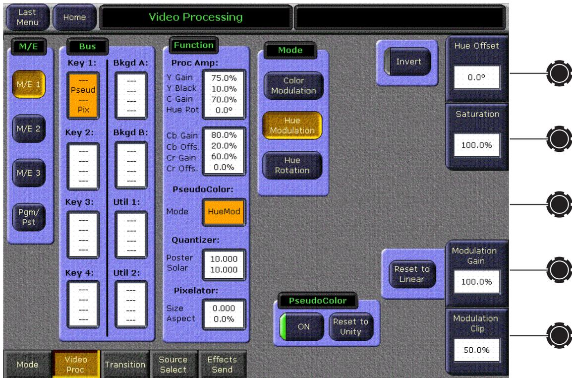
**Hue Modulation** (Figure 265) operates like Color Modulation, but instead of mixing between two color mattes, the modulating signal maps incoming luminance to matte hue. As the instantaneous luminance value of the incoming video changes from black to white, the instantaneous hue of the processed picture changes in hue angle. As the luminance increases, the hue value increases toward magenta, red, etc., counterclockwise on the vectorscope.
