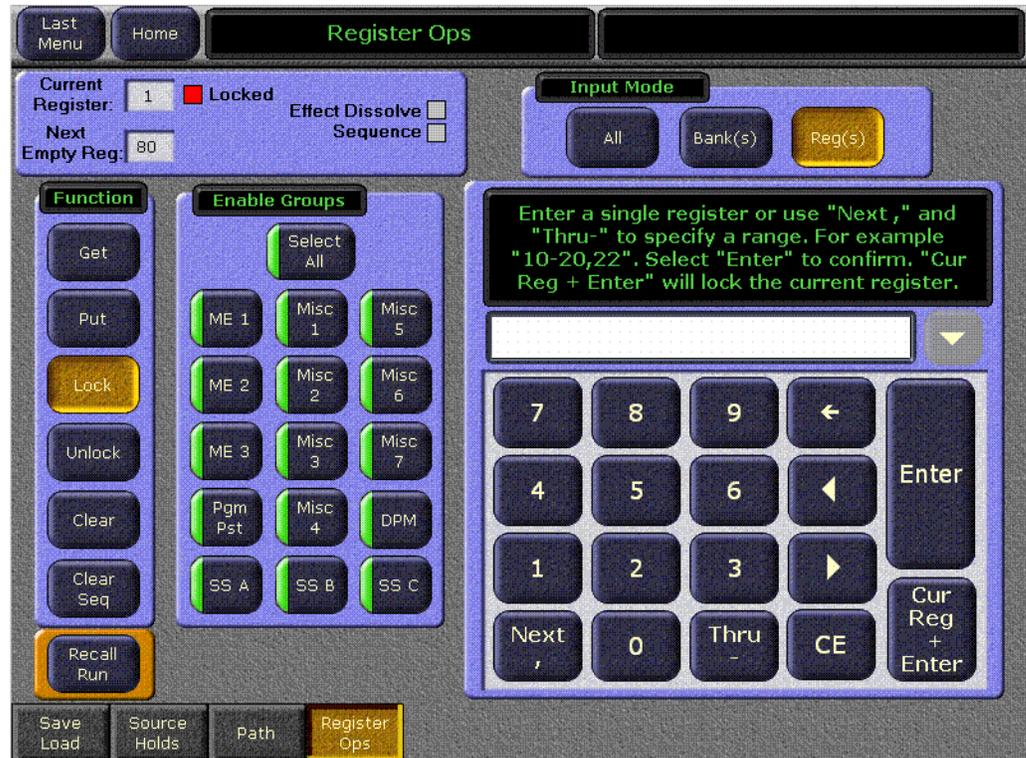
The Input Mode pane is used to specify the scope of the action to be performed.
