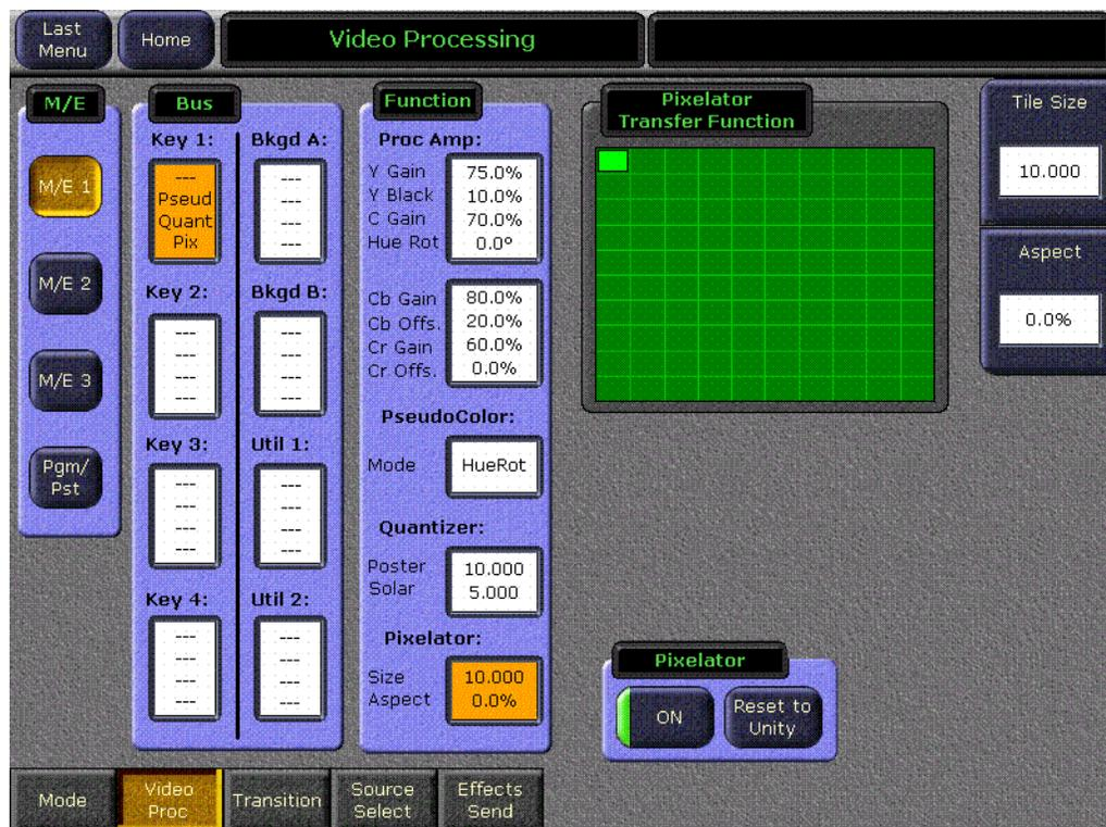
The **Tile Size** soft knob adjusts size of the tiles, in pixels. (The reading is actually overly accurate, to accommodate interpolation. The actual width in pixels of a tile is rounded upward to the nearest multiple of 4).
