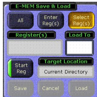
Clicking on the **Load To** datapad opens the **Load To** keypad (Figure 201). Enter the number for a single register to which you would like to begin loading registers.
