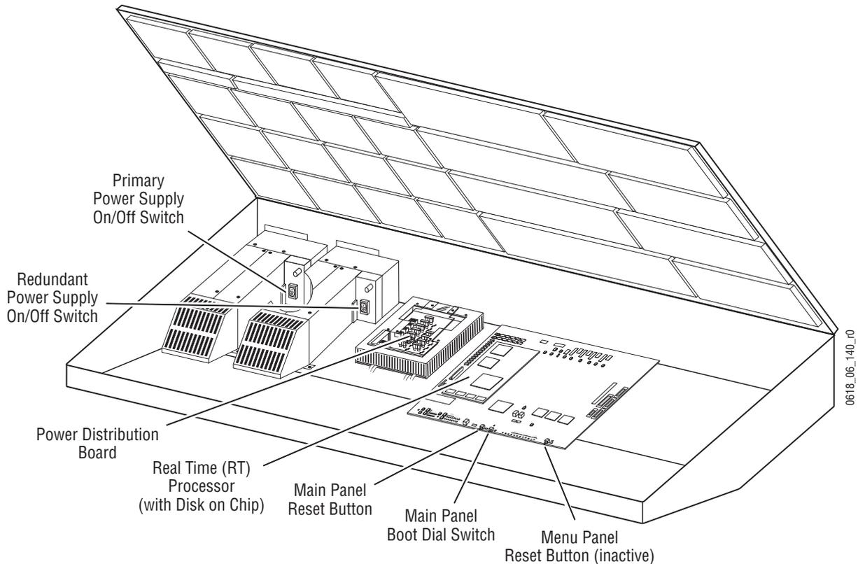
Earlier model 4-M/E Main panels have additional connectors (Figure 6) used with the original Kalypso Menu panel. If this model is modified for Enhanced Menu panel operation, the indicated connectors are inactive.
