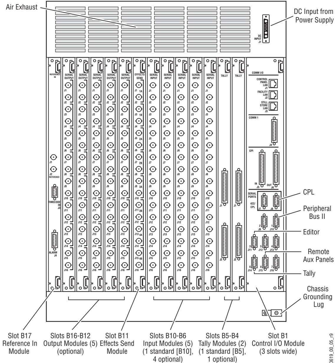
The Kalypso system has been designed for easy maintenance. All modules of the same type are identical, and can be swapped with one another. Modules can be removed and replaced safely with the power on, simplifying troubleshooting to the module level.
