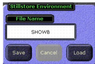
The **File Name** button displays a keyboard for the operator to enter a name for the environment to be saved.
