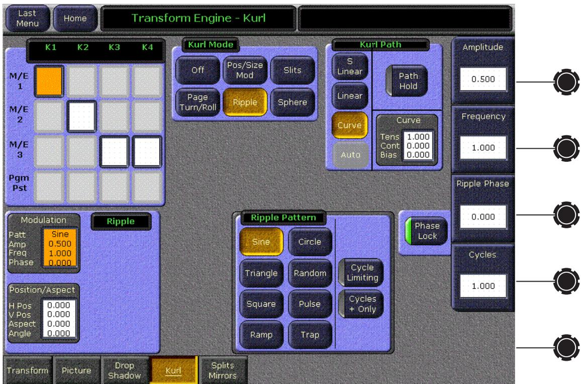
The Ripple soft knob controls and wave patterns are the same as Position/Size, except there is no H/V Angle control (see [Modulation Pane on page 347](#) and [Figure 246 on page 349](#)).
