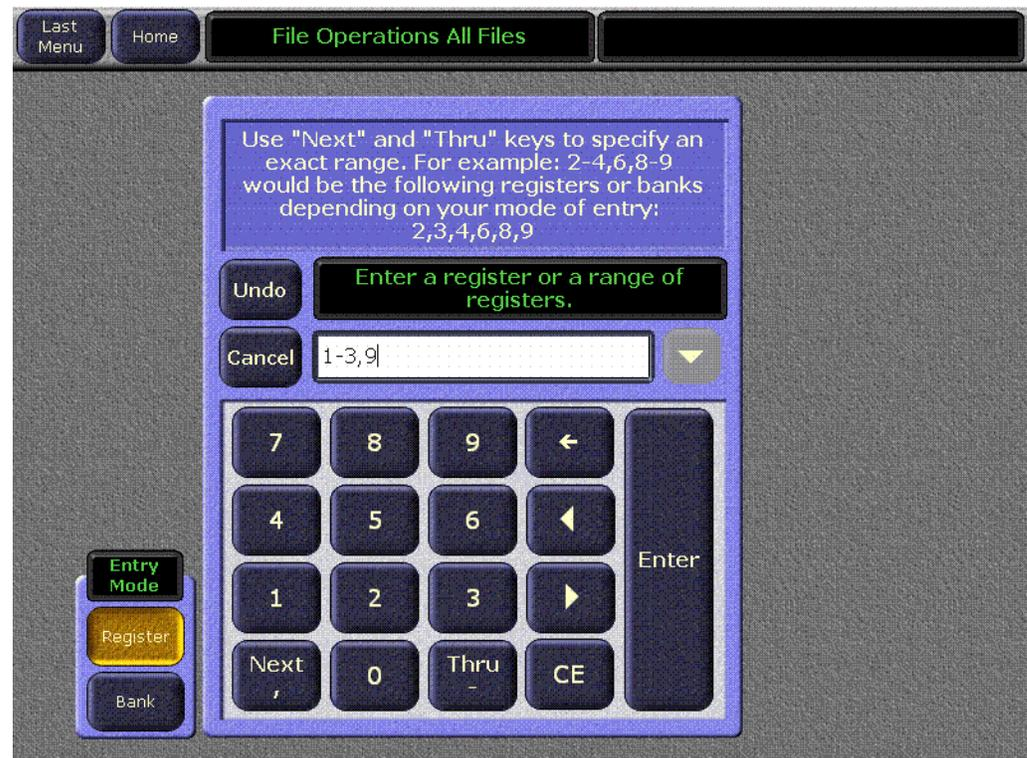
For example, in Figure 198 clicking on the Enter key will enter Registers 1 through 3 and also register 9. If the **Bank** button were selected clicking on the Enter key will enter Registers 10-39, 90-99.
