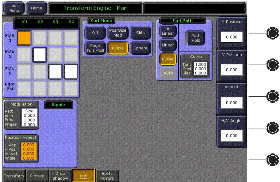
Soft knob controls are provided to control various attributes of the Ripple pattern.
