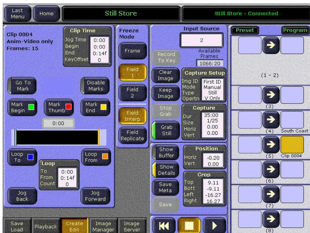
Selecting the **Save Meta** touch button saves meta data changes to an image in output to the (cropping, fence size, etc.) meta data file on the hard disk.
