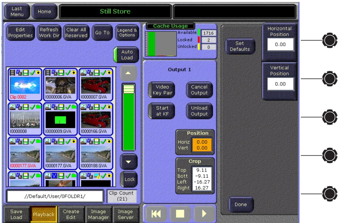
Touching the **Crop** data pad brings up a similar menu with **Top Crop**, **Bottom Crop**, **Left Crop**, and **Right Crop** controls (Figure 218). The image can be cropped to any rectangular shape. These controls are keyframeable but resolution is limited to pixels and lines so interpolated motion may not appear smooth. For smooth motion use a Transform Engine.
