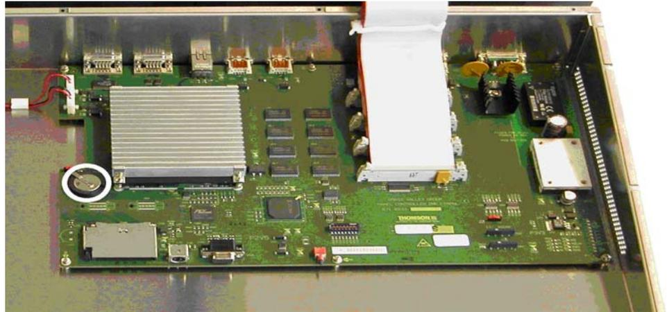
3. Remove the old battery by lifting the clip holding it in place.
