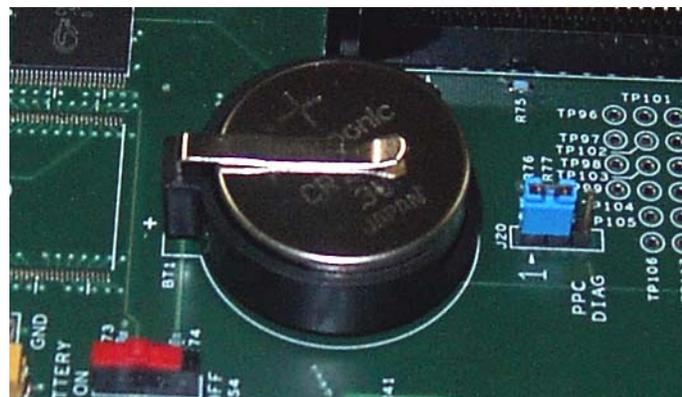
3. Remove the old battery by lifting the clip holding it in place.
