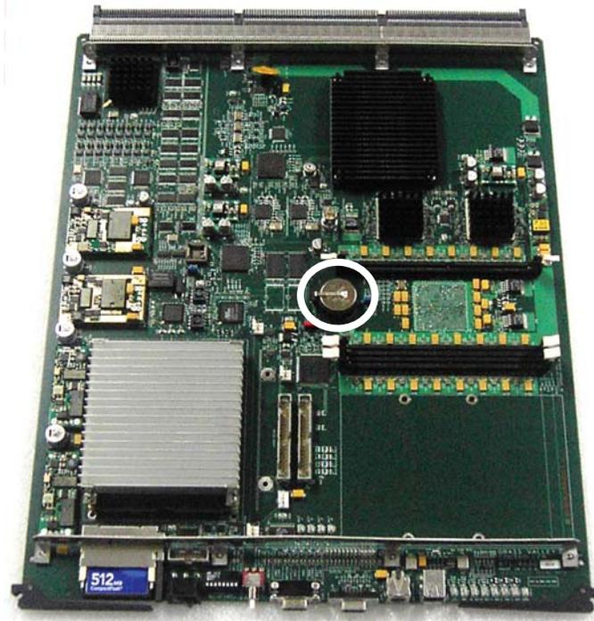
Figure 58. Kayak HD Frame Controller Board Battery
