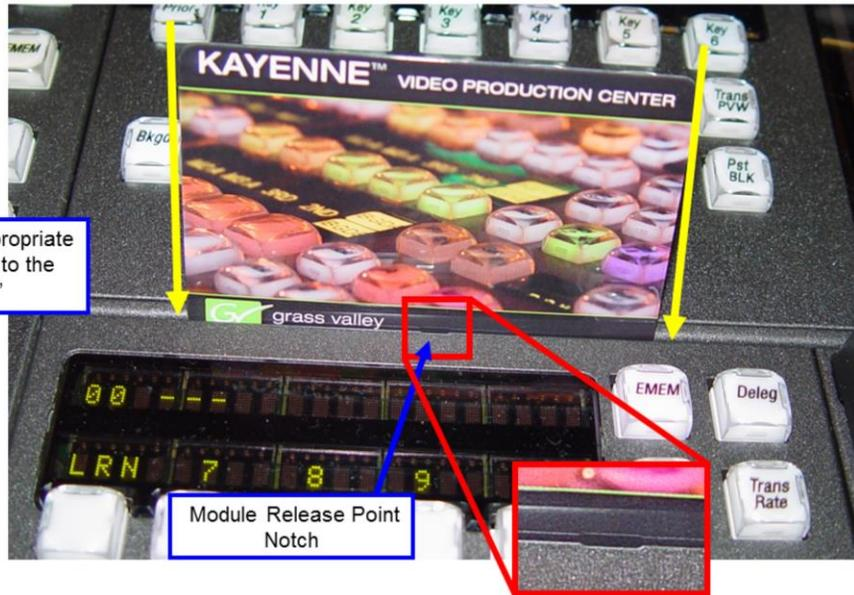
Locate and Press Appropriate Card Straight Down to the Release "Click"
