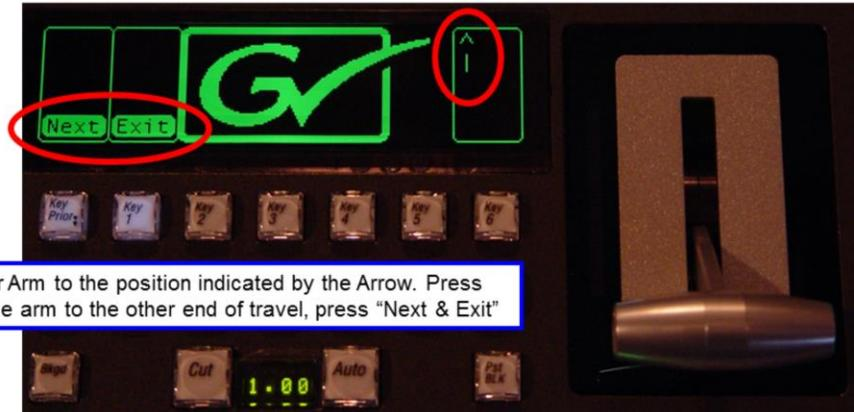
Move the Lever Arm to the position indicated by the Arrow. Press "Next". Move the arm to the other end of travel, press "Next & Exit"
