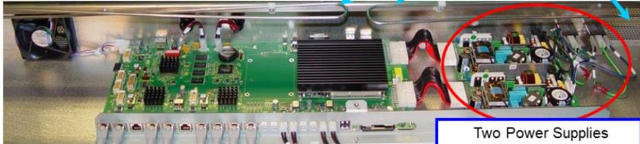
Two Power Supplies Standard. Power Supplies and fans are replaceable items from GV.
