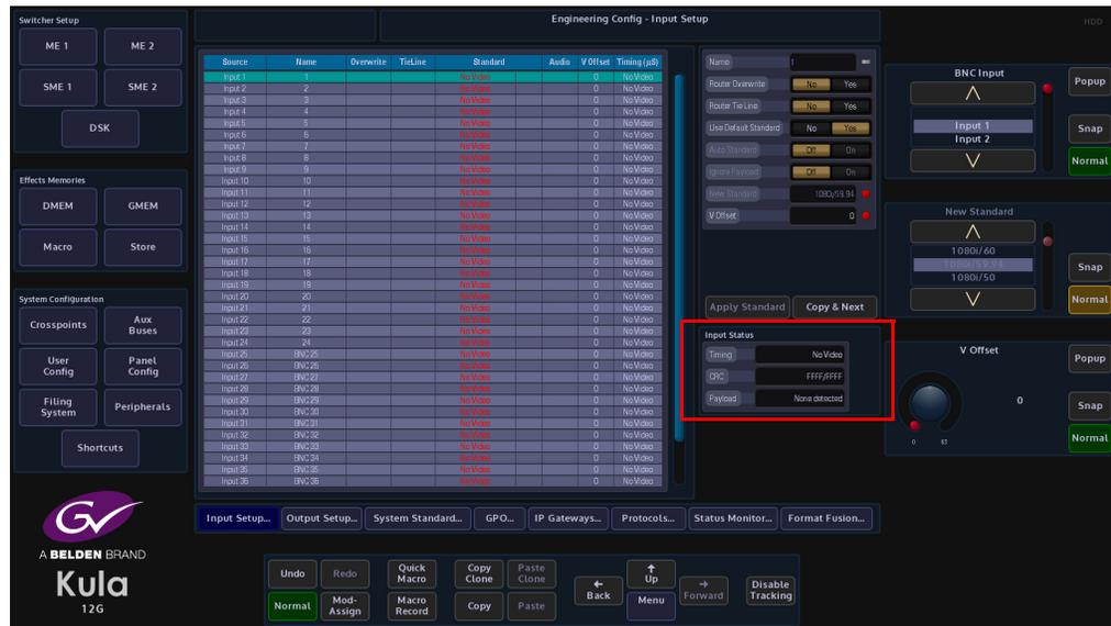
The Timing Parameter indicates the Offset in Micro seconds (or Milli Seconds) between the Reference input and the selected source. To Clean switch or avoid a Line offset (e.g. a vertical shift) the Timing has to be within +/- half a line of the current standard. e.g. for 1920x1080i59.94 +/-14uS).
