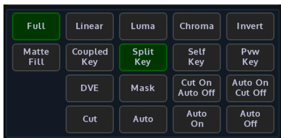
**DVE** - This turns on the DVE function. When entering the DVE menu, the DVE function will be enabled.
