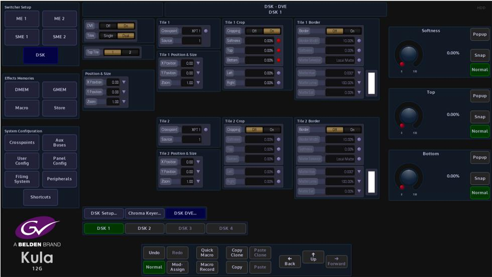
**Cropping On/Off** - Switches the crop facility On or Off. Press the On/Off buttons in the parameter control area of the menu.
