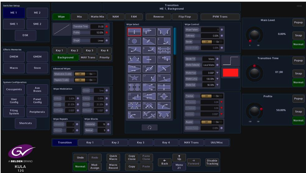
If a Wipe transition is required, touch the **{Wipe}** button in the Transition area of the control surface, or in the transition menu, The type of transition wipe required can be selected using the **“Wipe Pattern”** parameter, use the associated rotary control to scroll through the wipe patterns. Move the T-bar from end stop to end stop. Notice that the Key Layer will now transition with a wipe pattern over the A/B background.
