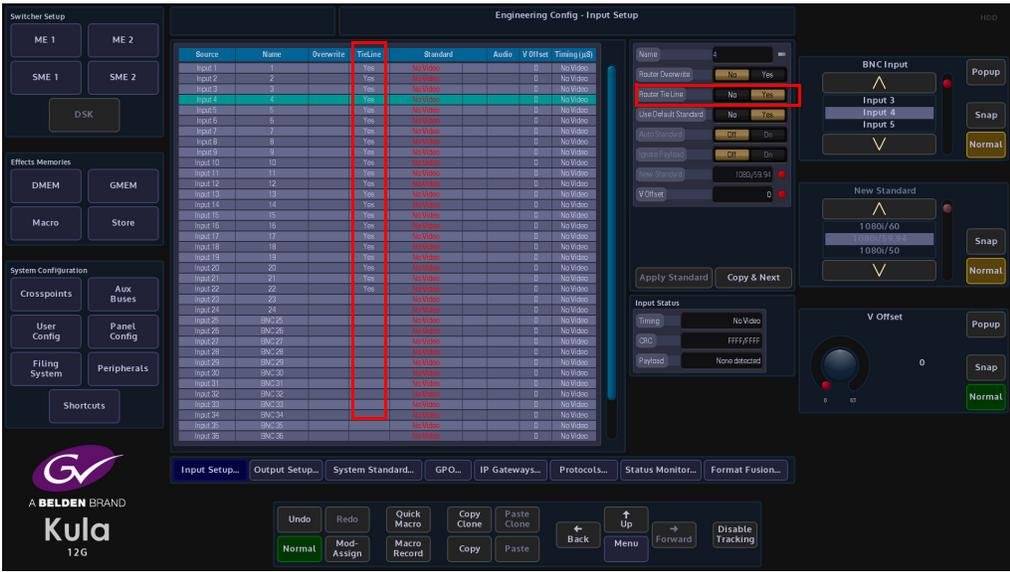
Note: For inputs that are set as “Tie Lines”, it is recommended that the “Source Standard” parameter (in the Eng Config - Inputs menu) is set to “Auto Standard”.
