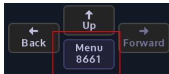
At a basic level (on the Kula control surface GUI), the only level), you can discover/learn the unique numeric menu code (like a phone number) of any menu by navigating to it in the normal way. Once there, the menu number can be seen in one of two places, depending on the GUI in use. For the large touch screen GUI, it is shown on the **{Menu Jump}** button under the 'UP' button. On the Kula control surface GUI, it is shown on the numeric keypad, accessed by touching the "Star" pop-up button.
