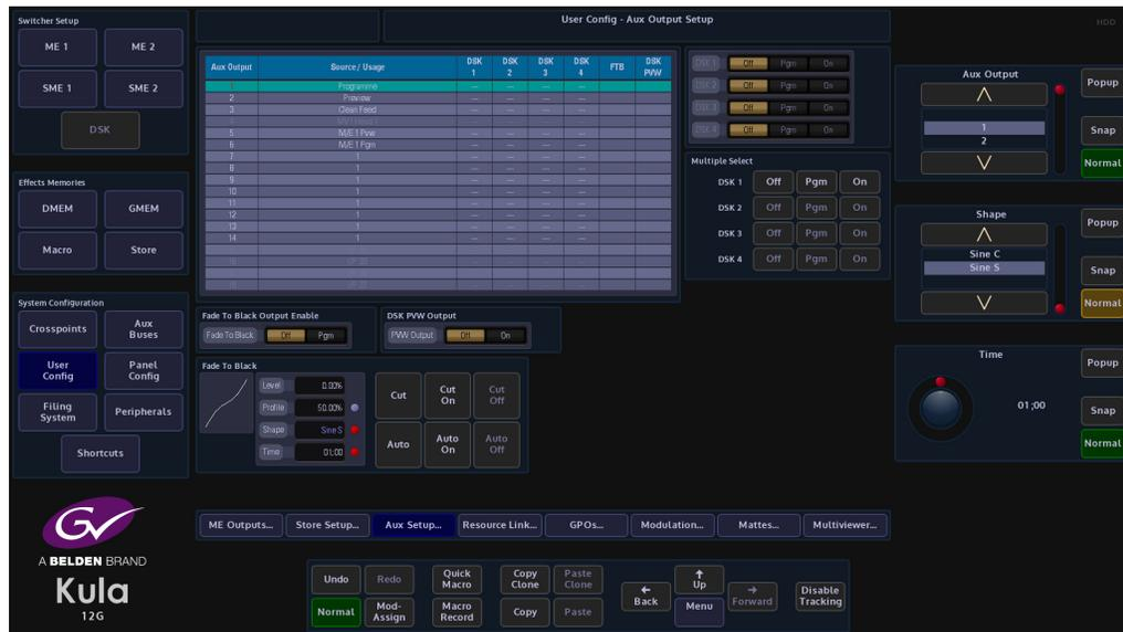
The table in the menu displays what is setup on each output from the mainframe. The Source/Usage column displays the type of signal output that is on each BNC, i.e. PGM, PWV, Clean or Multiviewer Head etc. The 4 DSK columns display which outputs the DSKs are enabled on, by default DSK 1 is always selectable, DSKs 2 to 4 are only available to select if they are enabled in the Eng Config - Outputs menu.
