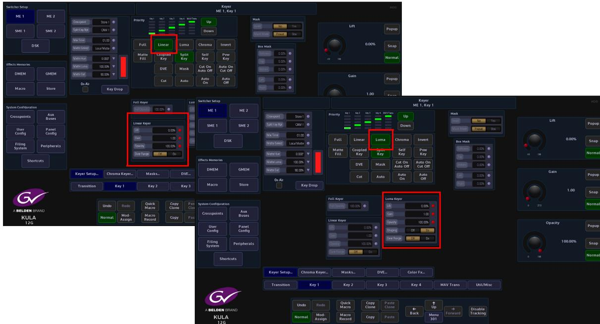
**Lift** - sets the Luma level at which the Key operates.
