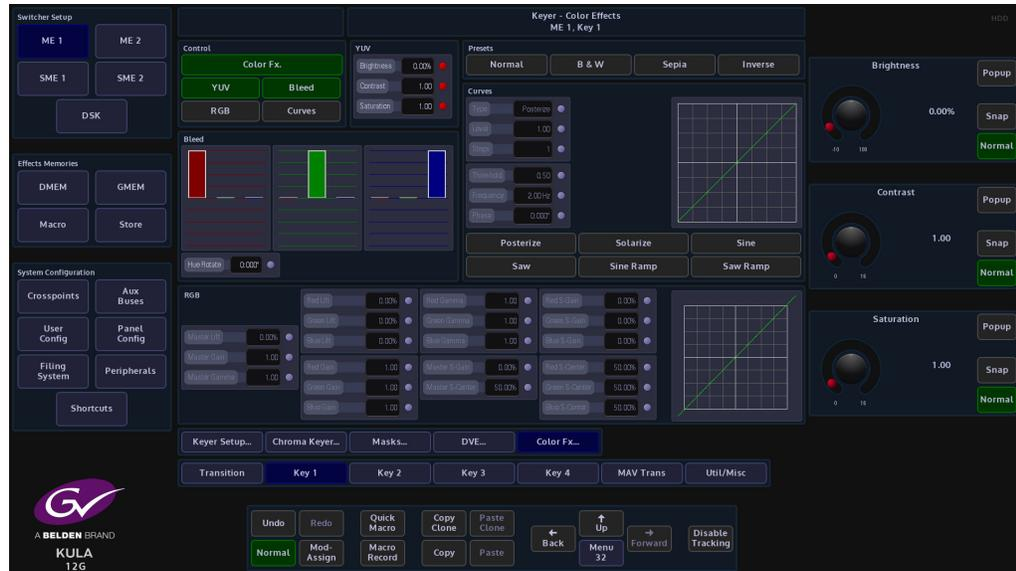
The initial menu has a default state where a single adjustment for each parameter menu is active; this will allow the adjustment of the main RGB bleed parameters:
