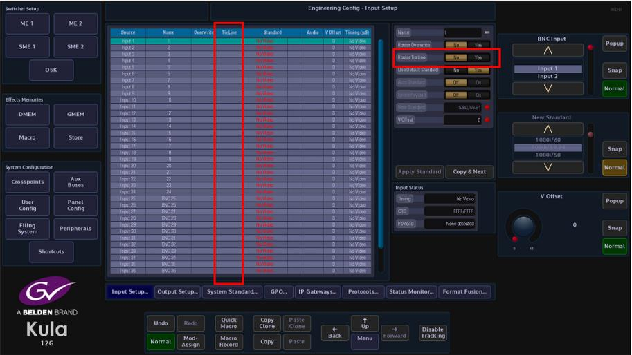
Using the **Router Overwrite** parameter in the **Eng Config - Input Setup** menu, Kula is able to receive UMD information from any of the BNC inputs. This information will then be displayed in the input menu’s and can also be used for the mnemonic displays on the control surface for selecting sources.
