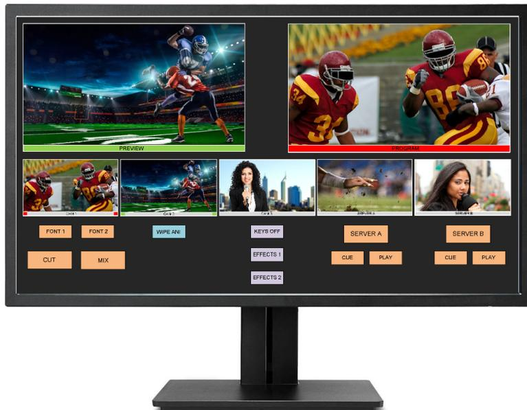
With K-Touch the user can cut sources to the program, or select them to the preview, recall effects on the M/E banks, control the clip stores and select sub-clips. example of other functions are wipes, Clip transitions and mixes all by using customized buttons on the touch screen.
