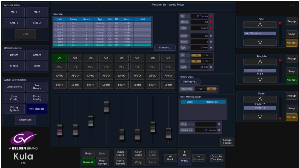
You should be able to slide faders via the Visual or Fader Module and see corresponding faders move on Yamaha Audio Mixer for communication test.
