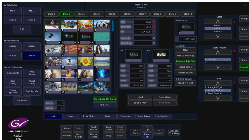
In the **Store Load** main menu, the Stills, Clips and Audio Clips are sequenced in numerical order. This number appears on the bottom left of the mini pic starting with 0 and ending at 999 depending on the number given to the still or clip in the K-Manager software.
