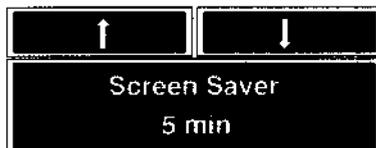
The screen saver switches off the display in order to avoid burn-ins when the control panel is inactive for a given period. This period can be set with the arrow soft-keys.
