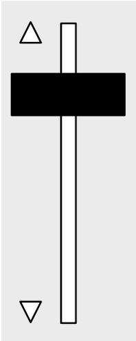
The fader enables sensitive manual transitions. The yellow arrows to the left of the fader show the moving direction to the next contribution which is shown on the preview monitor.
