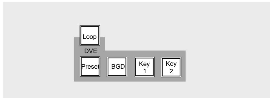
If **Loop** is not actuated, the respectively selected video signal is switched through to the DVE. The manipulated signal of the DVE is available on the input routing switcher and can be processed in the same way as a normal video signal.
