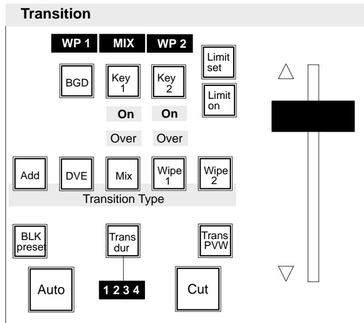
For picture design, selection can be made between the transition modes **Add**, **Mix**, **DVE**, and **Wipe**, providing up to two wipe generators. The individual picture components can be simultaneously faded with different transition types. Control of the mixing stage is facilitated by the consequently realized next transition principle.
