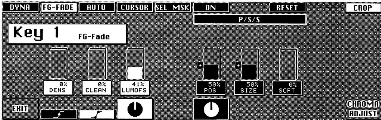
**LUMOFS** positive luminance offset to the subtractive key color luminance (only in the FG Fade mode).
