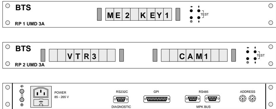
Connection to the MPK bus is made in the same way as for the AUX panels. Power supply can be universally with line voltages of 85 V ... 265 V AC. The respective use of the UMDs can be adjusted with the two rotary switches **ADDRESS** on the terminal panel.
