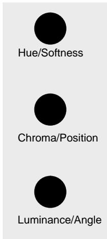
The **Hue** control adjusts the color. The **Chroma** control adjusts the intensity of the color. The **Luminance** control adjusts the brightness of the color.
