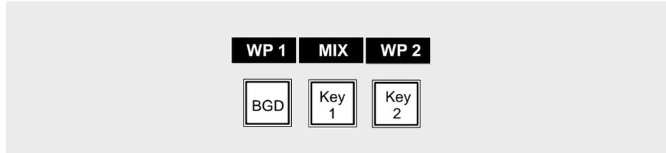
The selected keys light and indicate which picture components are affected during the next transition. The result can be looked at the preview monitor.
