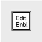
**Edit Enable** enables the switcher to be controlled by an external editing system. In the activated state, the switcher can be switched from the control panels as well as from an editor.
