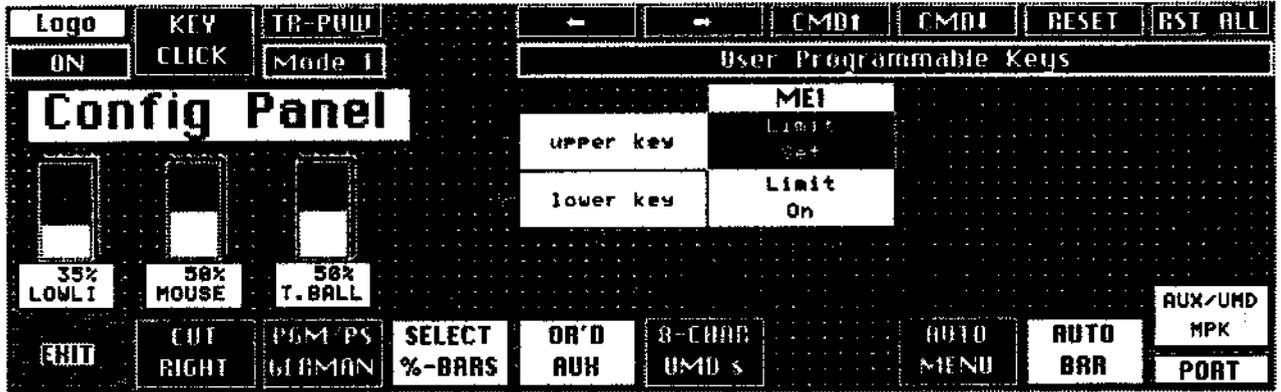
The CONFIG PANEL menu serves to set system parameters for the control panel of the switcher. Some analog parameters to optimize operation are also set in the INSTALL menu.
