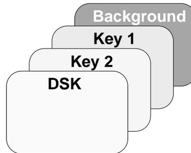
Beside the main outputs, the switcher additionally includes a clean-feed output which provides the picture in front of the downstream keyer.
