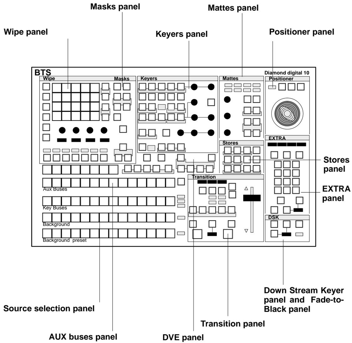
A detailed illustration of the control panel is shown on a fold-out page at the end of the manual.
