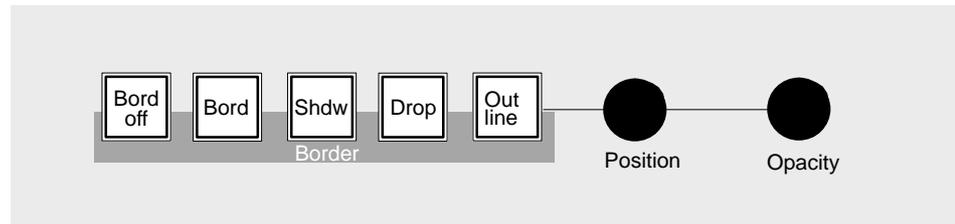
The Border key group enables the user to provide the key signals with a border effect which can be adjusted individually.
