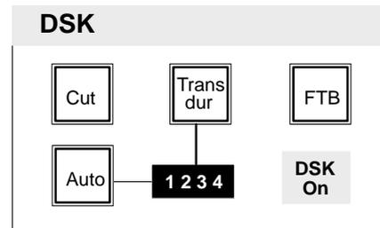
**FTB** switches the panel from downstream keyer control to fade-to-black control. The operational mode is indicated by lighting-up of **FTB**. When switching over, all settings of the Downstream Keyer panel are stored and automatically restored when returning to the DSK mode. If **FTB** has been pressed erroneously, press it again to deselect the function.
